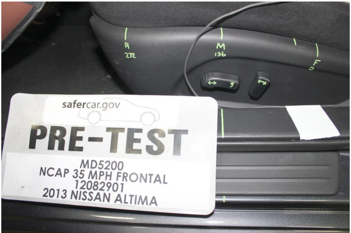
Pre-Test Driver's Seat Fore-Aft Markings
