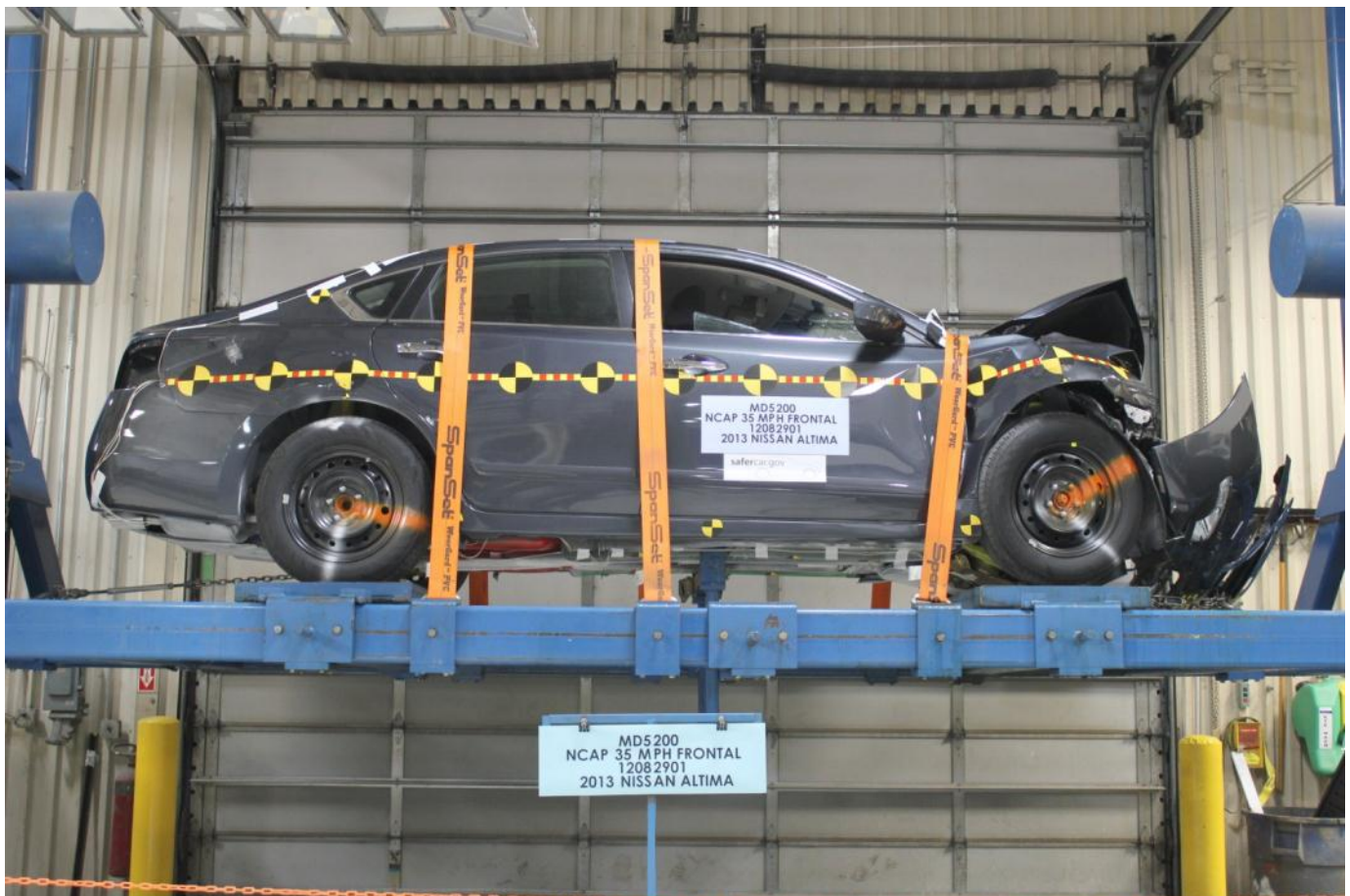
Vehicle at 0° on Static Rollover Device
