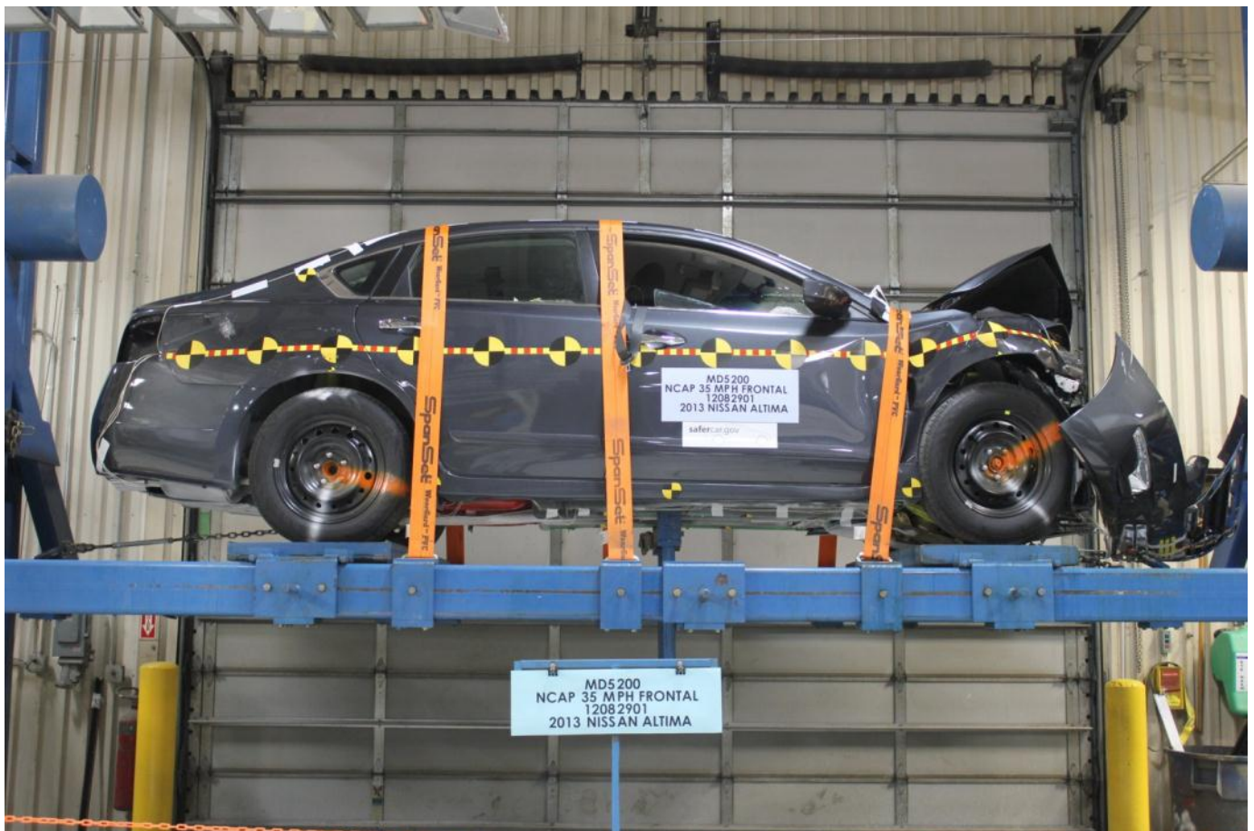
Vehicle at 360° on Static Rollover Device
