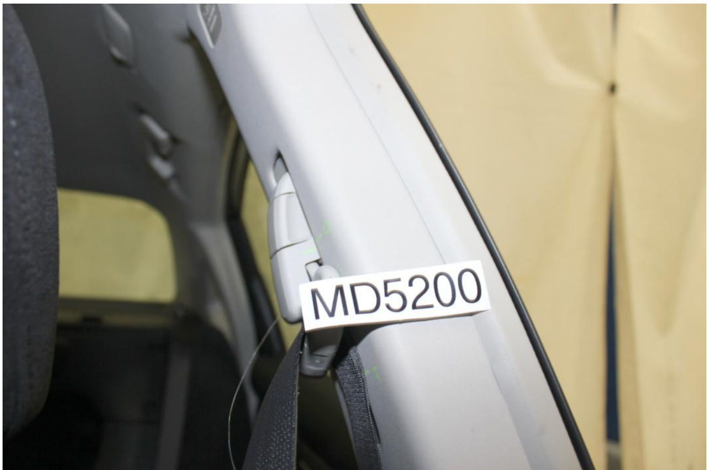
Post-Test View of Belt Anchorage for Driver Dummy
