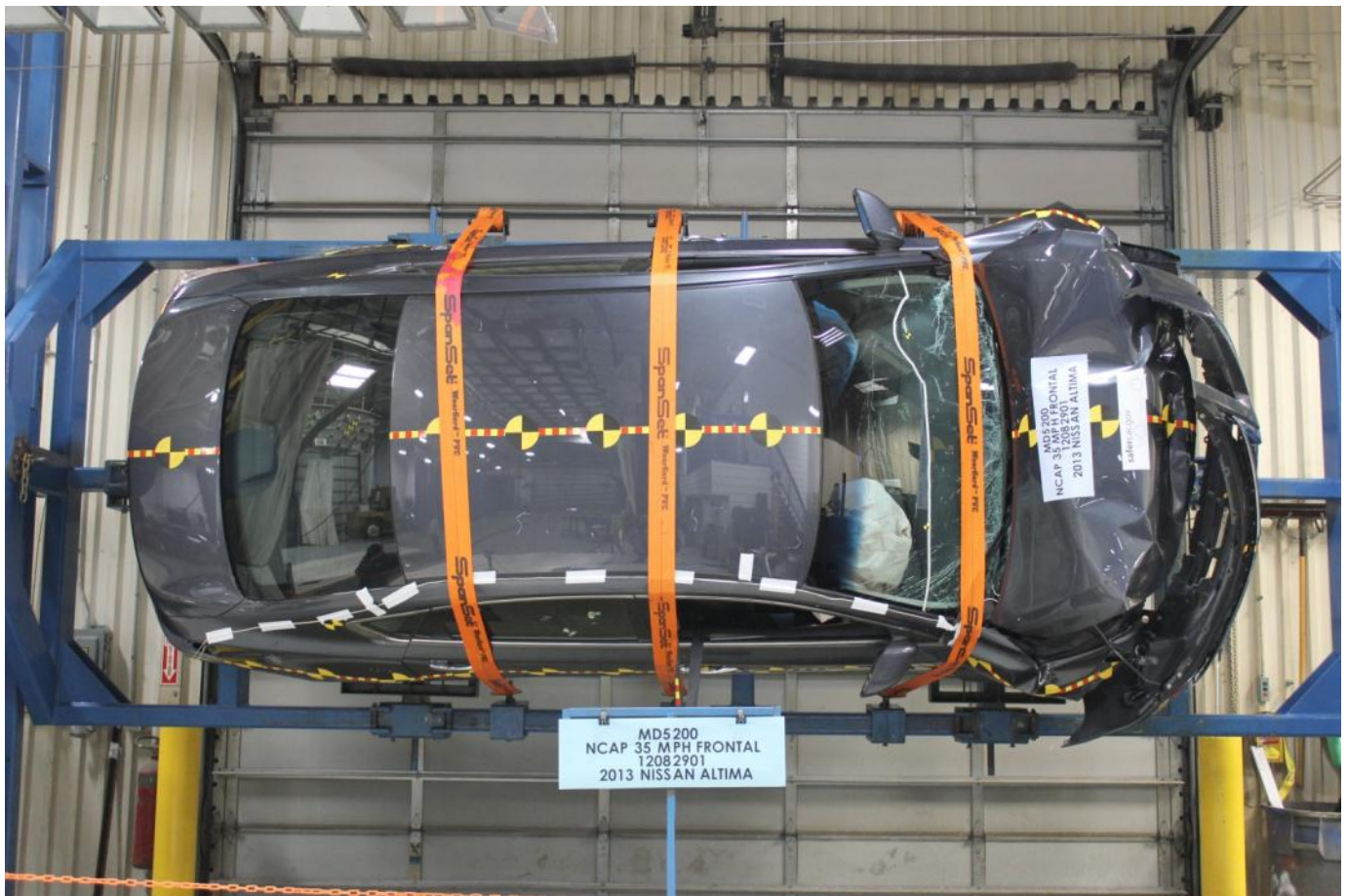
Vehicle at 270° on Static Rollover Device
