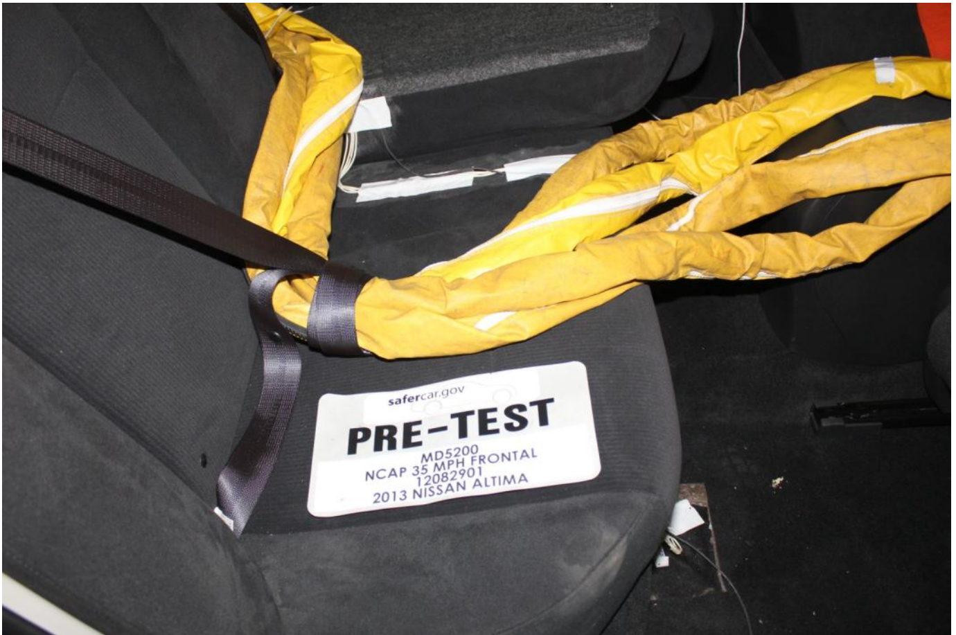
Pre-Test Dummy Cable Routing
