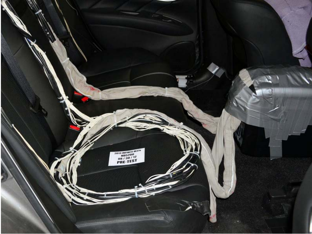
FIGURE 27. Pre-Test Dummy Cable Routing
