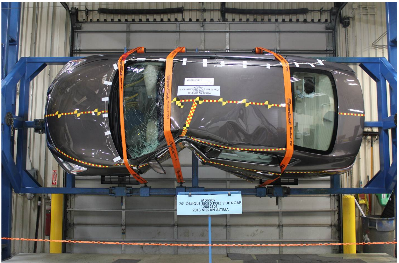
FMVSS No. 301 Static Rollover 90 Degrees
