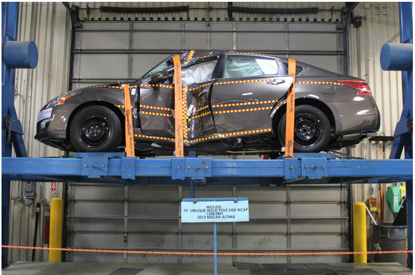
FMVSS No. 301 Static Rollover 0 Degrees
