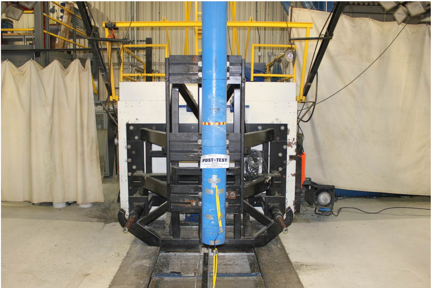
Post-Test Pole Barrier Front View
