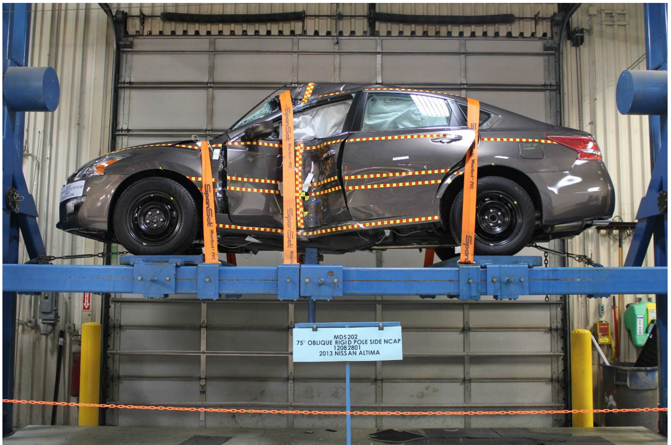
FMVSS No. 301 Static Rollover 360 Degrees
