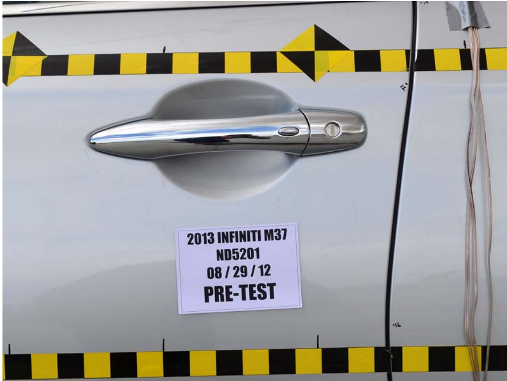
FIGURE 21. Pre-Test Left Front Door Latch Close-Up
