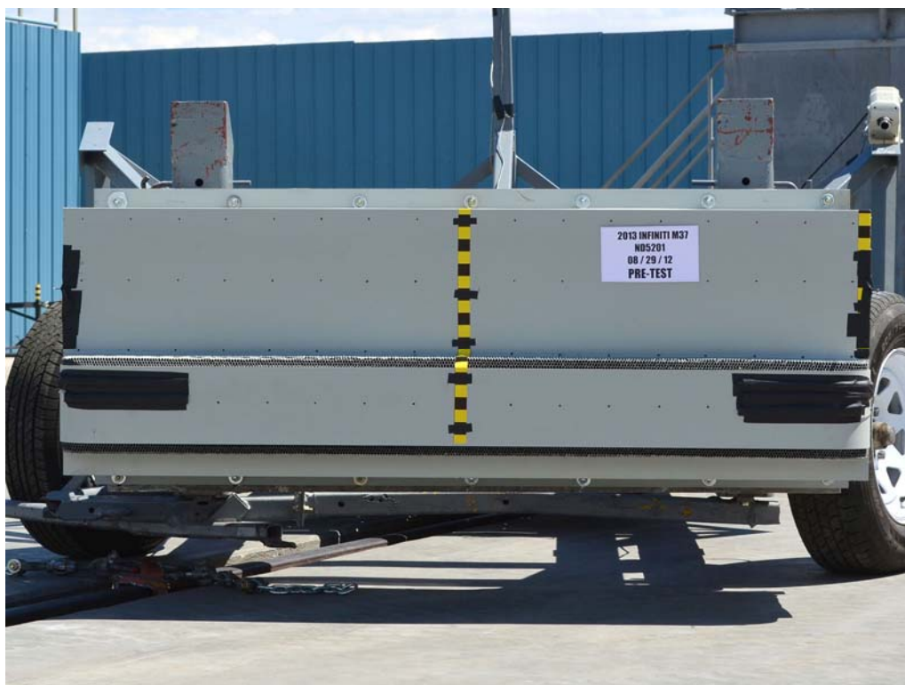
FIGURE 84. Pre-Test Front View of MDB Impactor Face
