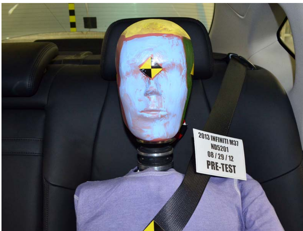
FIGURE 59. Pre-Test Frontal View of Rear Passenger Dummy Head and Shoulders in Relation to Head Restraint
