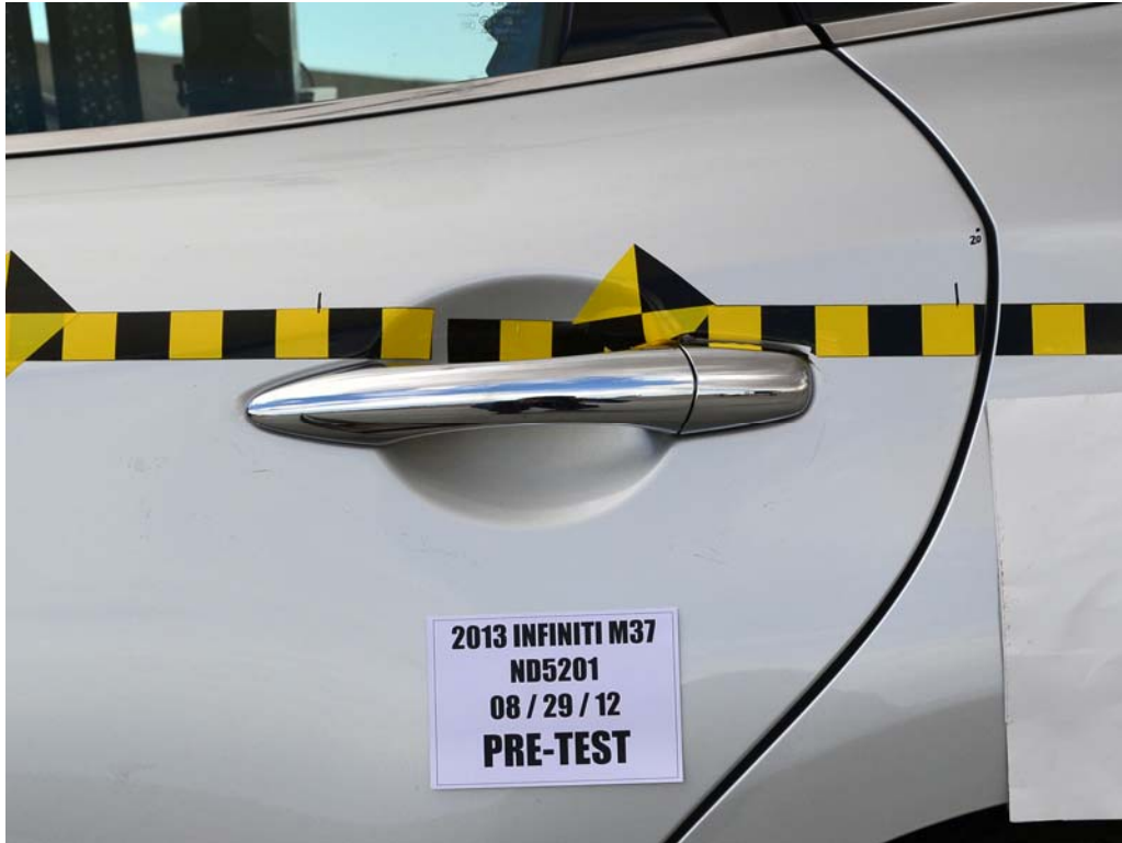
FIGURE 23. Pre-Test Left Rear Door Latch Close-Up
