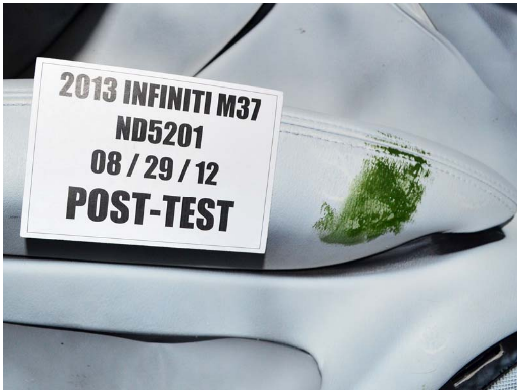
FIGURE 54. Post-Test Driver Dummy Close-Up Knee Contact View
