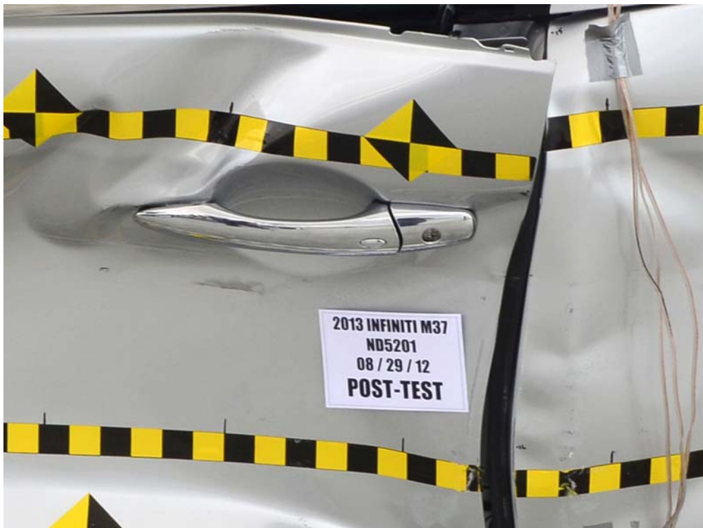
FIGURE 22. Post-Test Left Front Door Latch Close-Up
