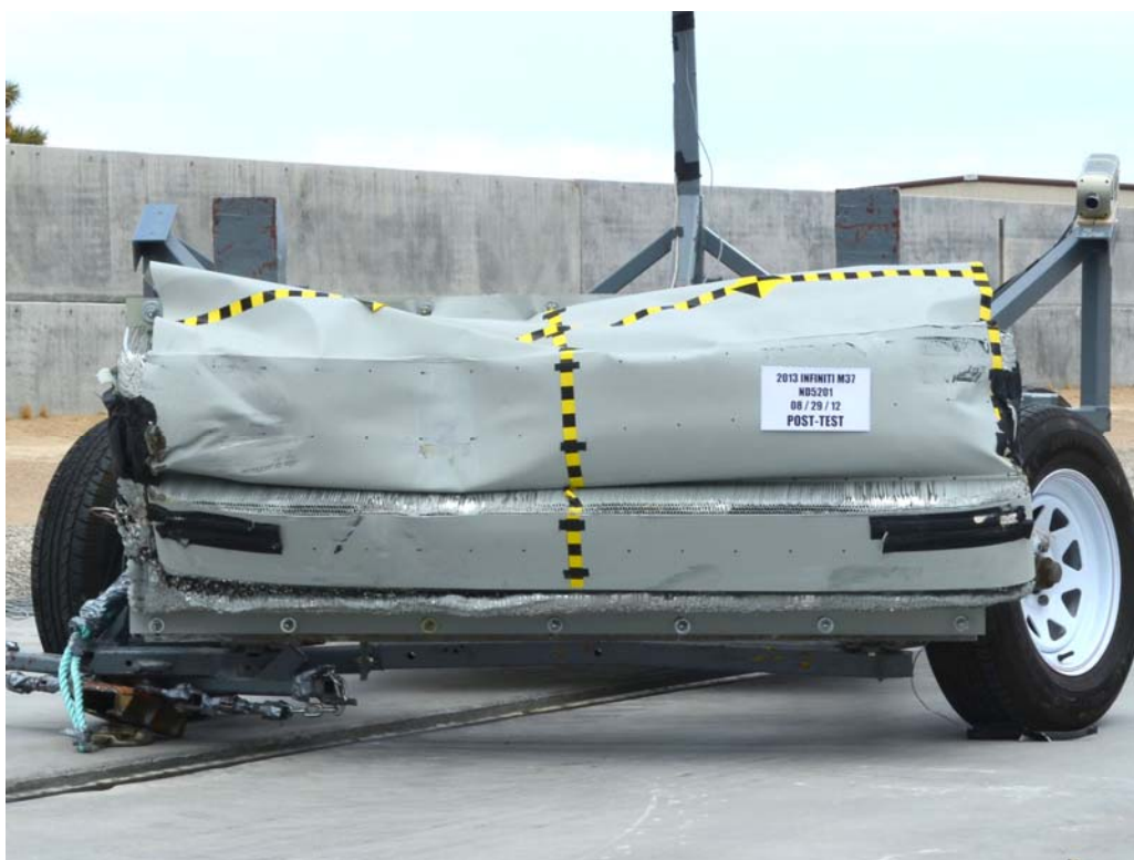
FIGURE 85. Post-Test Front View of MDB Impactor Face
