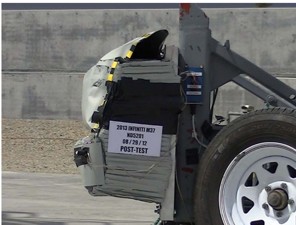
FIGURE 89. Post-Test Left Side View of MDB Impactor Face
