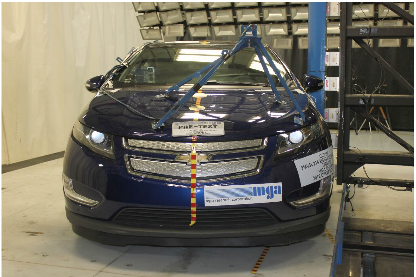
Pre-Test Frontal View of Test Vehicle
