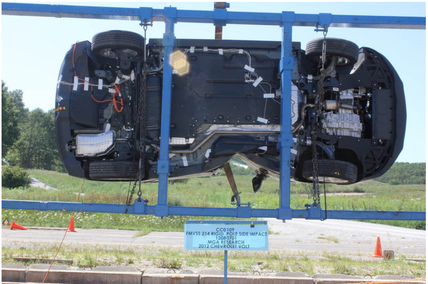
Post-Test Vehicle at 270 Degree Rollover
