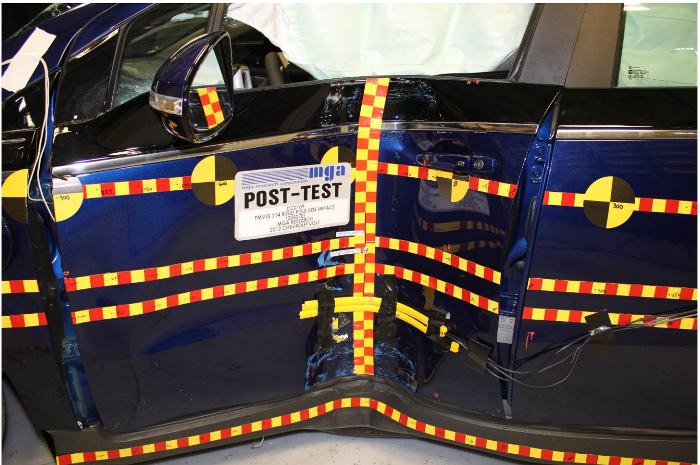
Post-Test Impact Zone Close-up View
