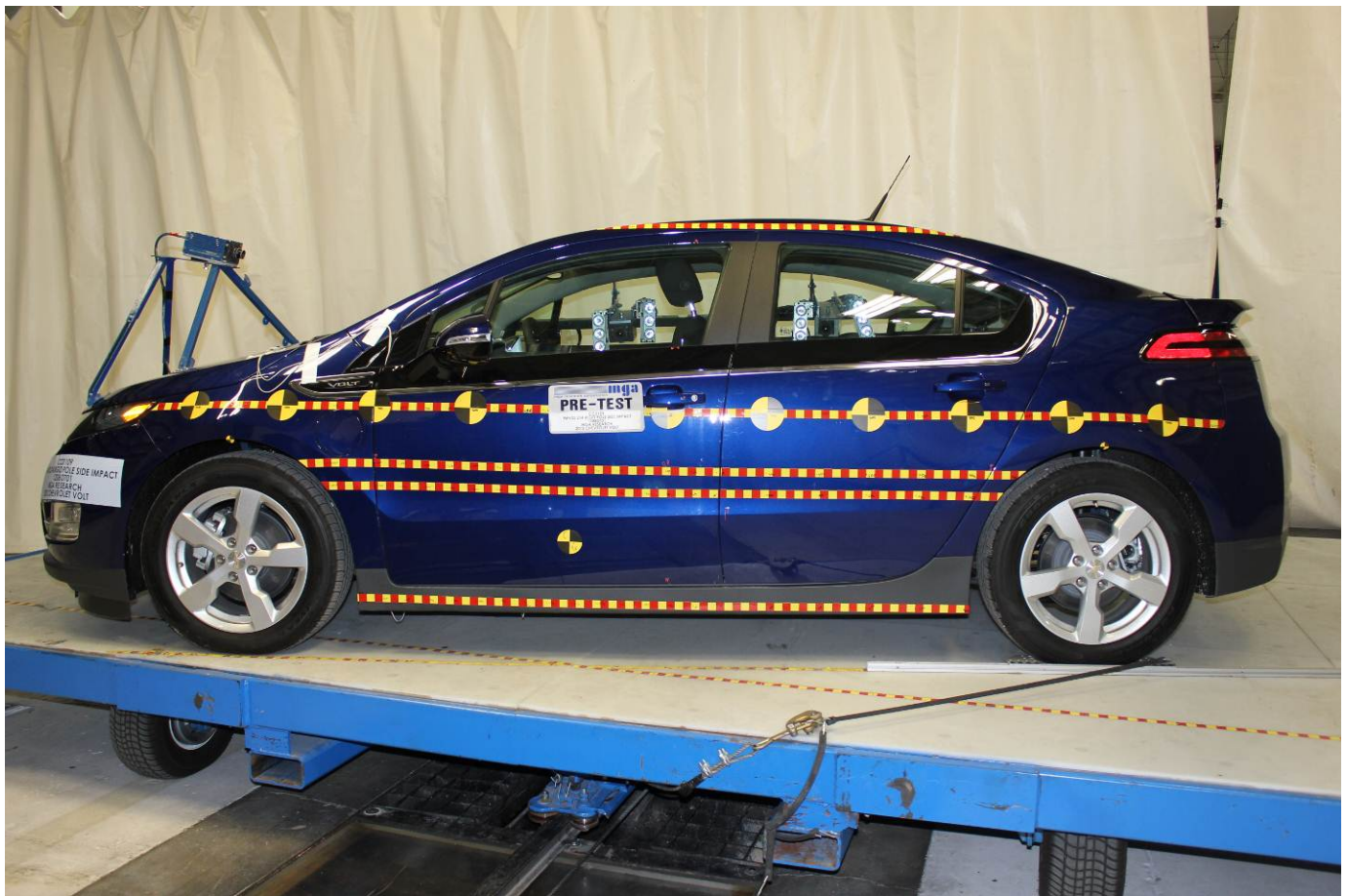
Pre-Test Impacted Side View of Test Vehicle
