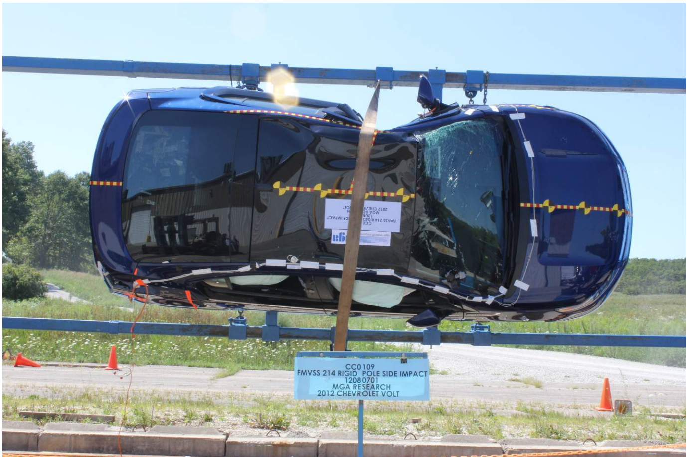
Post-Test Vehicle at 90 Degree Rollover
