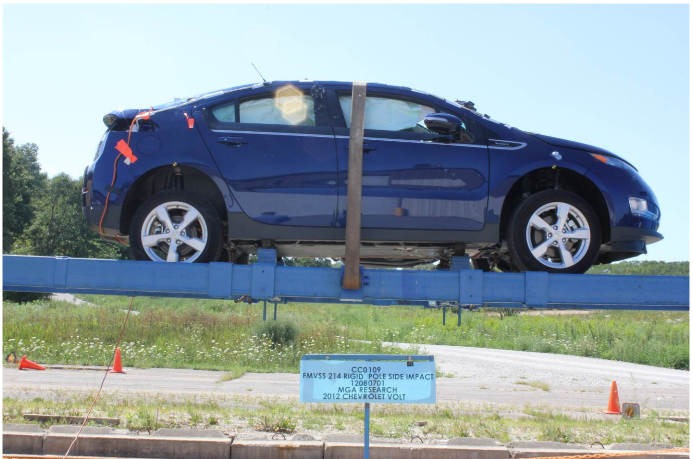
Post-Test Vehicle at 360 Degree Rollover
