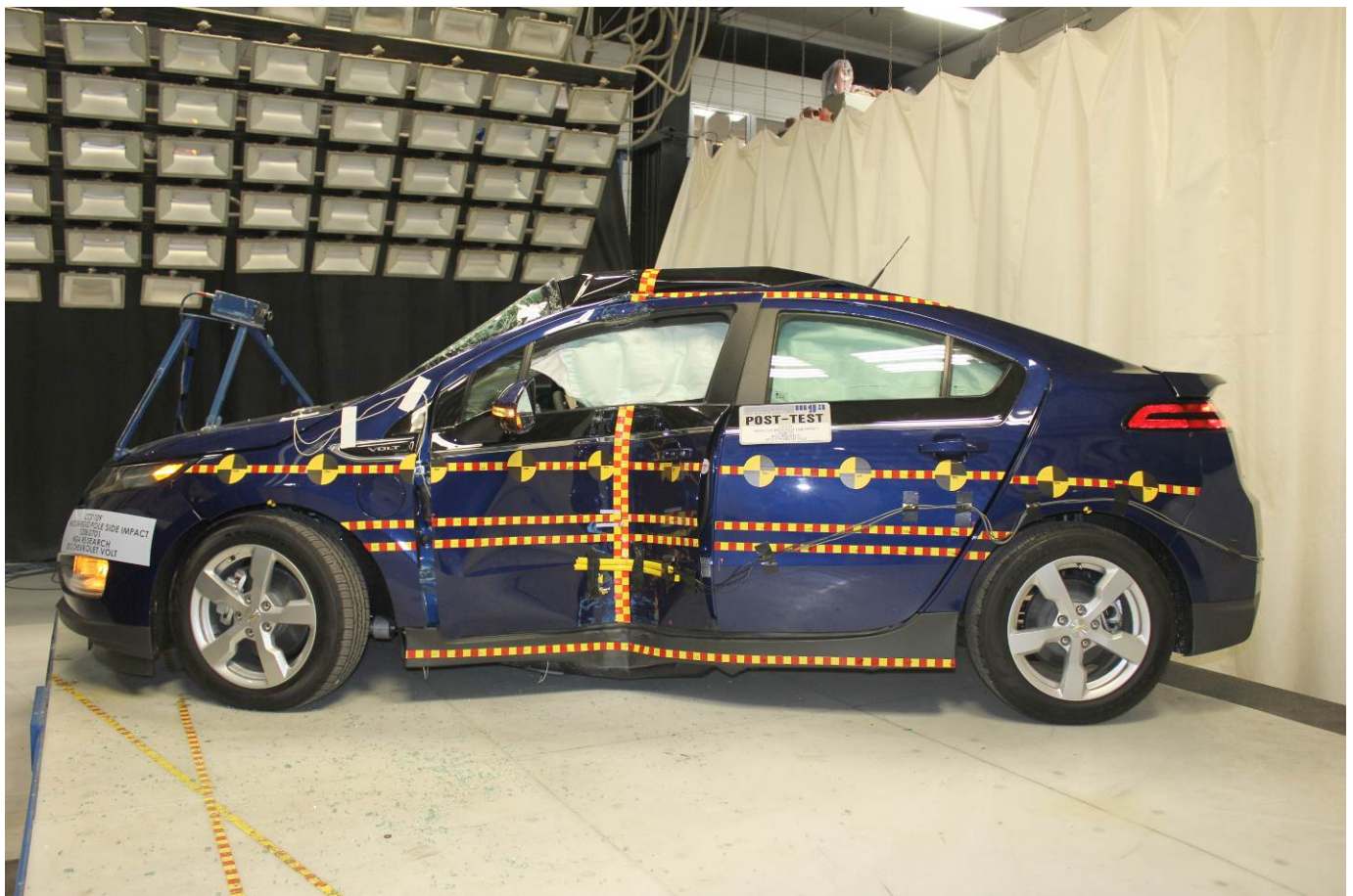
Post-Test Impacted Side View of Test Vehicle
