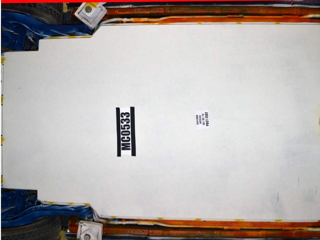
FIGURE 15. Post-Impact View of Propulsion Battery Module
