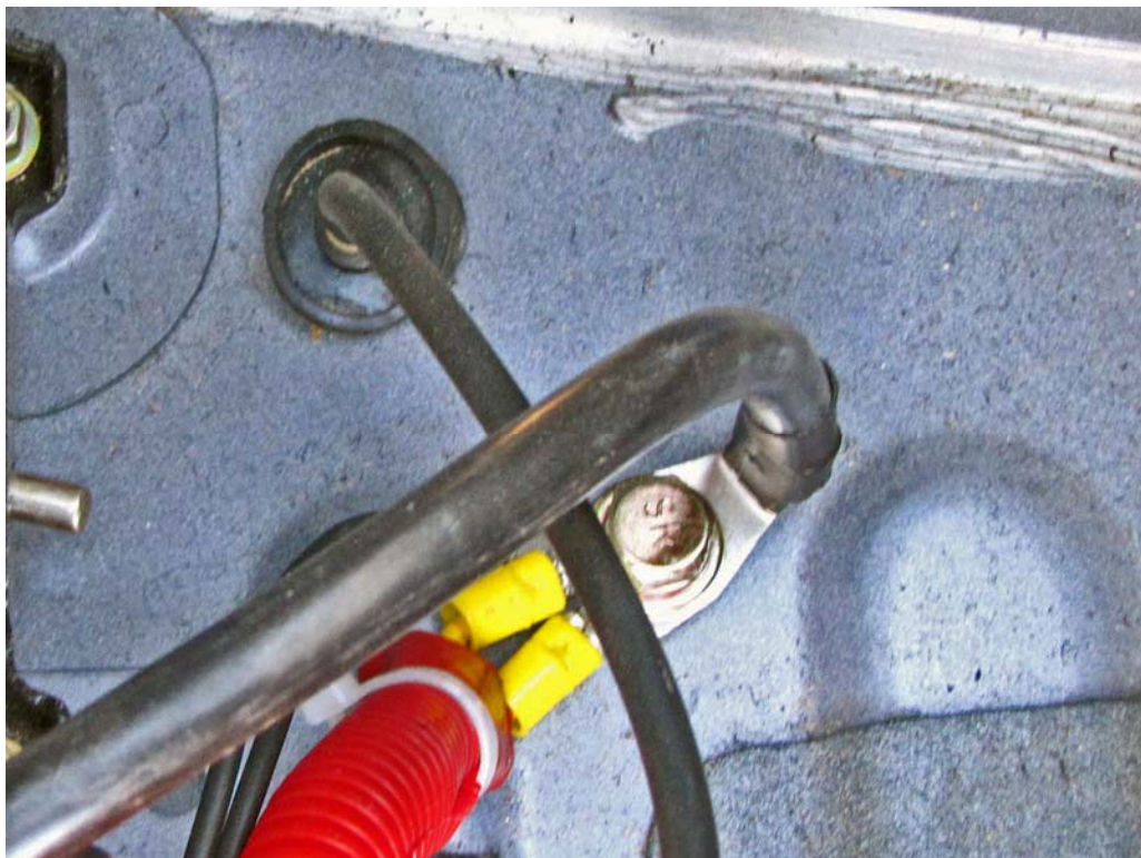
FIGURE 21. Pre-Impact View of Ground Lead Attached
