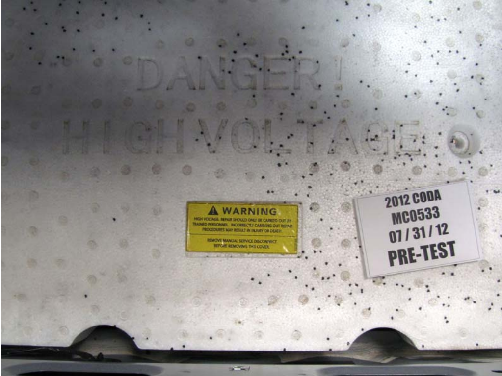
FIGURE 5a. Other Vehicle Label Related to Electrical Propulsion System
