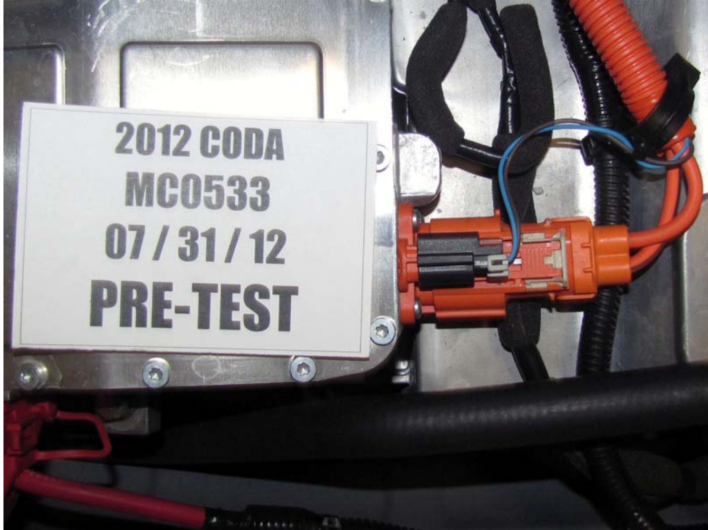
FIGURE 18a. Pre-Impact View of High Voltage Interconnect
