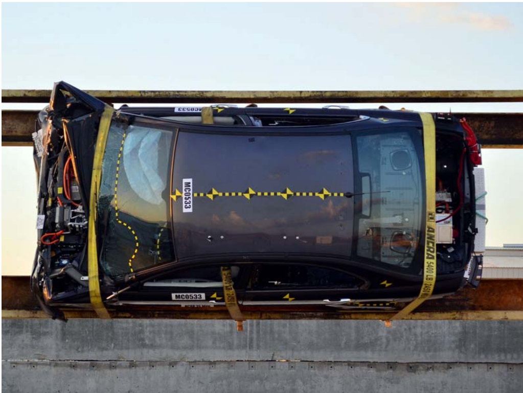
FIGURE 29. FMVSS No. 305 Static Rollover at 90 Degrees
