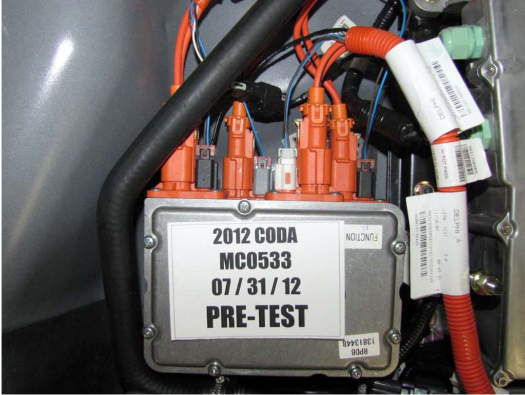
FIGURE 18e. Pre-Impact View of High Voltage Interconnect
