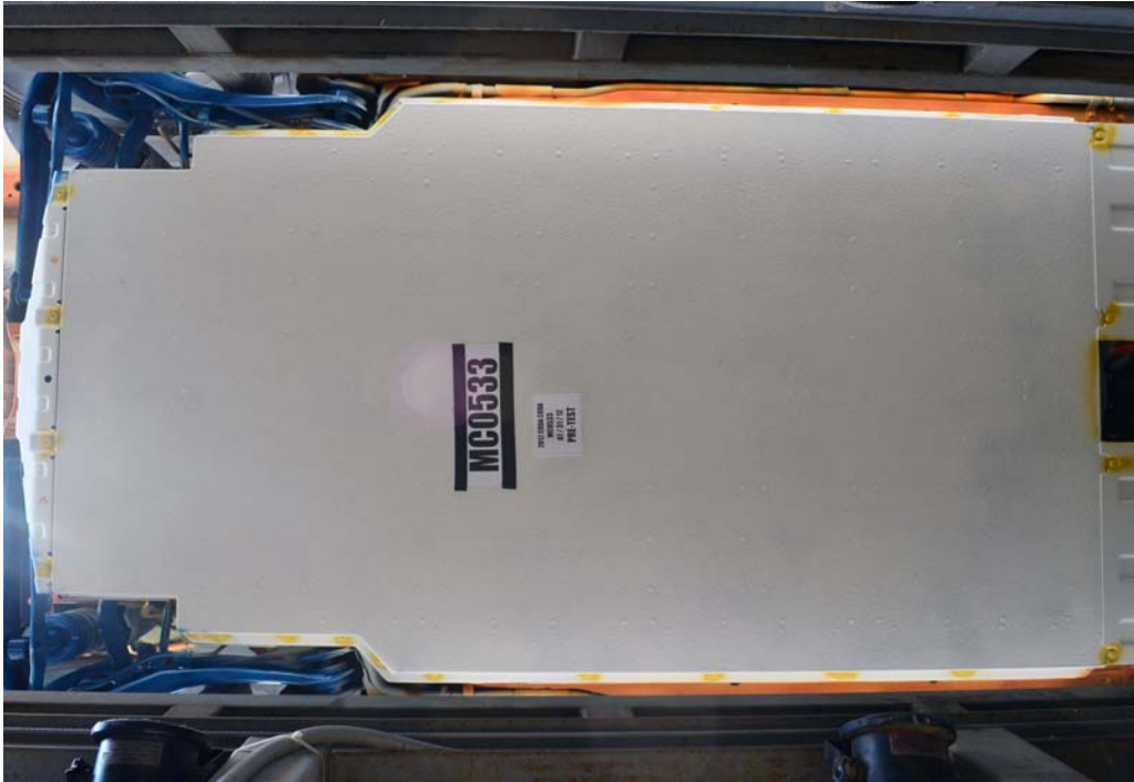
FIGURE 9. Pre-Impact View of Propulsion Battery
