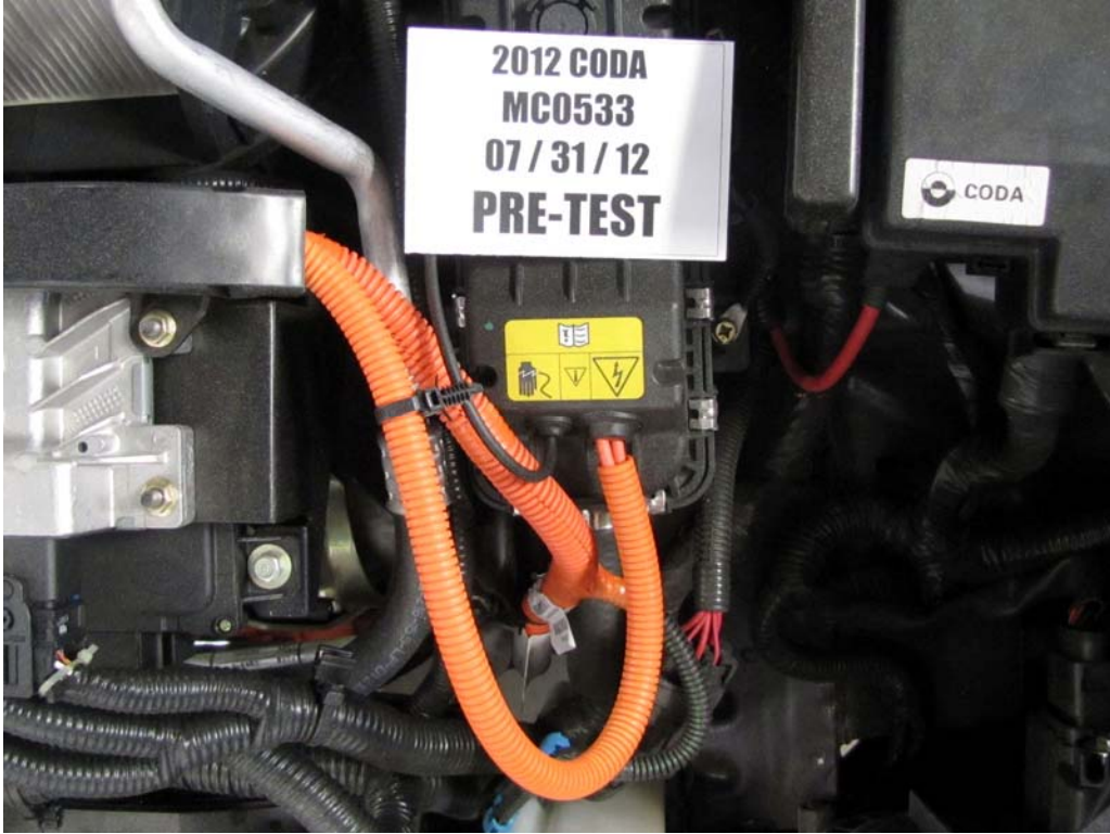
FIGURE 18i. Pre-Impact View of High Voltage Interconnect
