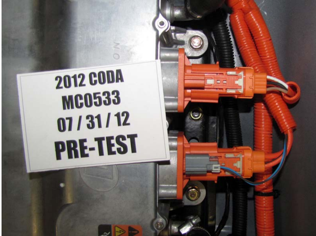
FIGURE 18c. Pre-Impact View of High Voltage Interconnect
