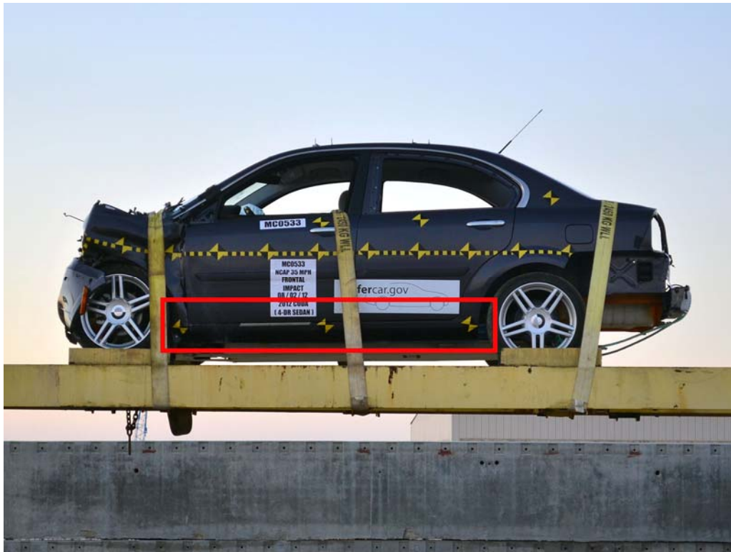
FIGURE 32. FMVSS No. 305 Static Rollover at 360 Degrees
