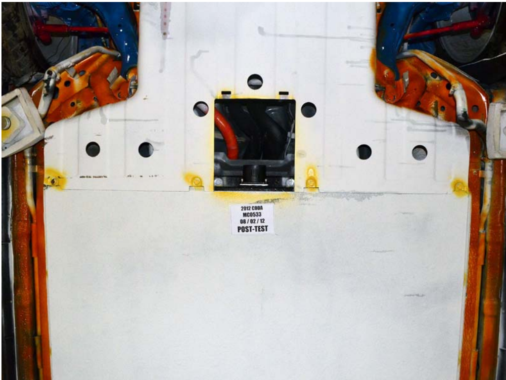
FIGURE 10. Post-Impact Front View of Propulsion Battery
