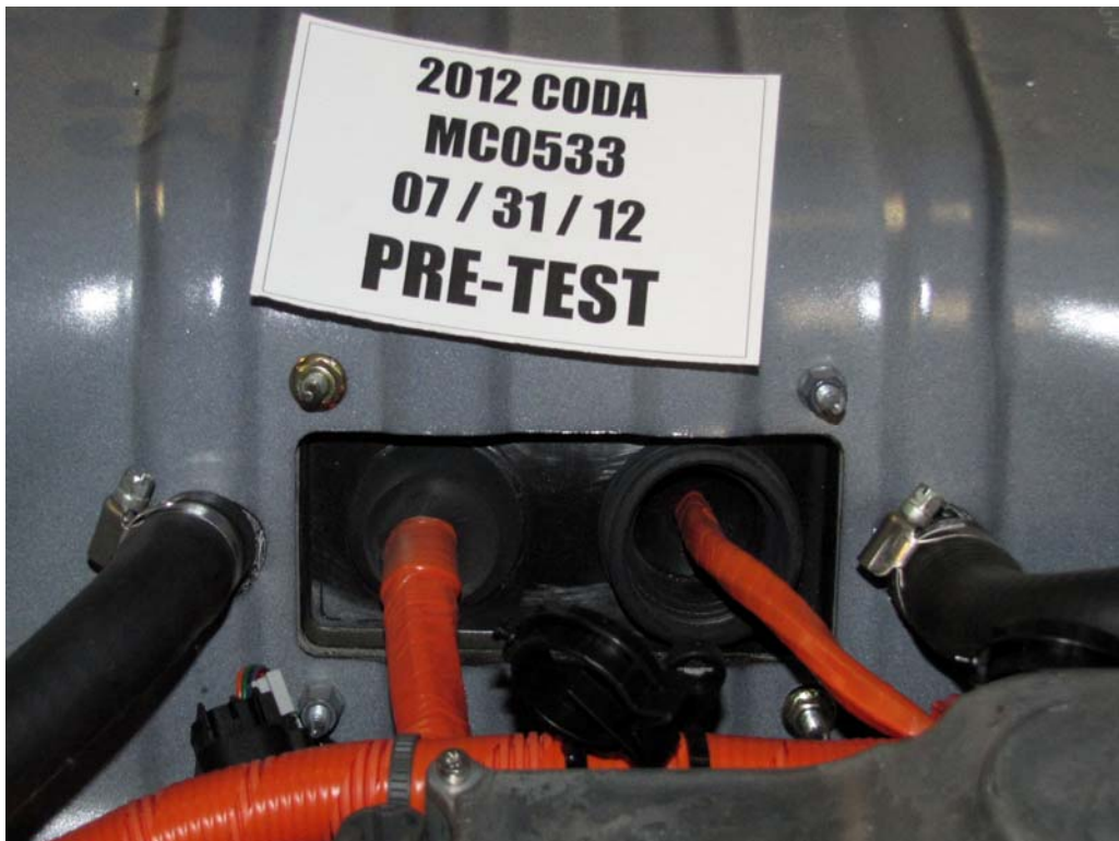
FIGURE 18d. Pre-Impact View of High Voltage Interconnect
