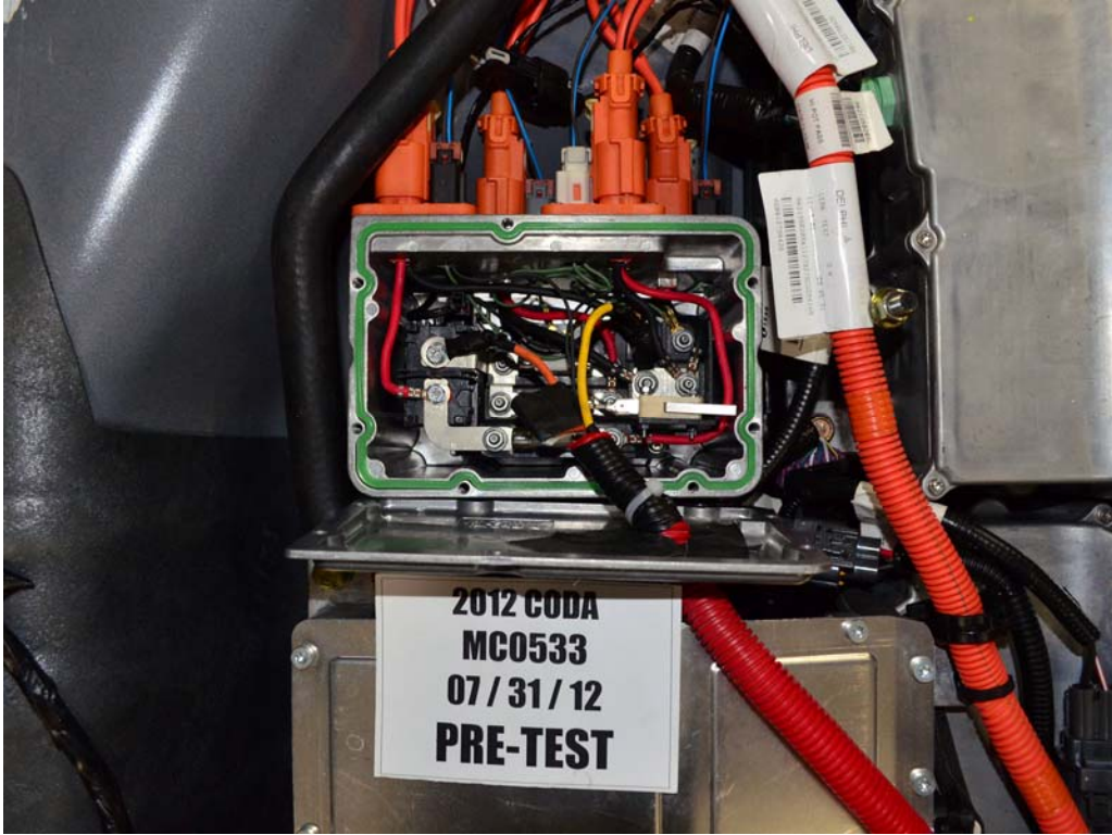
FIGURE 22. Pre-Impact View of High Voltage Leads Attached
