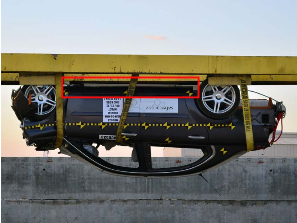
FIGURE 30. FMVSS No. 305 Static Rollover at 180 Degrees
