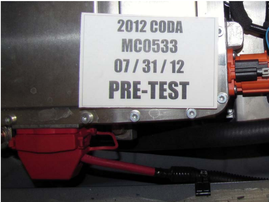
FIGURE 18. Pre-Impact View of High Voltage Interconnect
