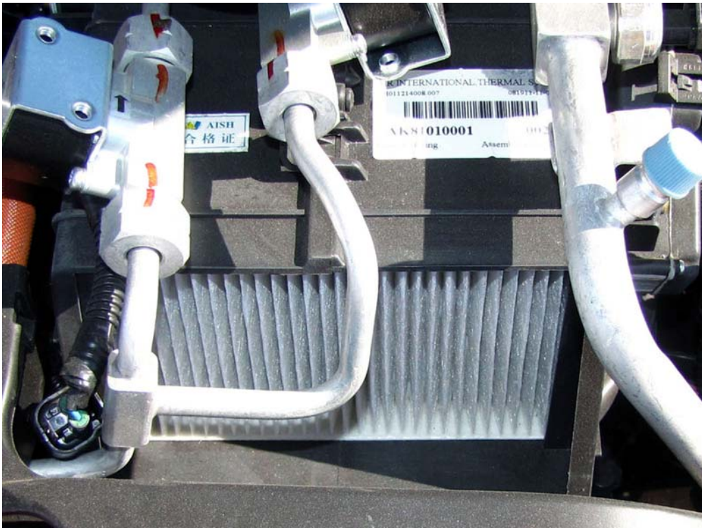
FIGURE 19. Pre-Impact View of Propulsion Battery Venting System
