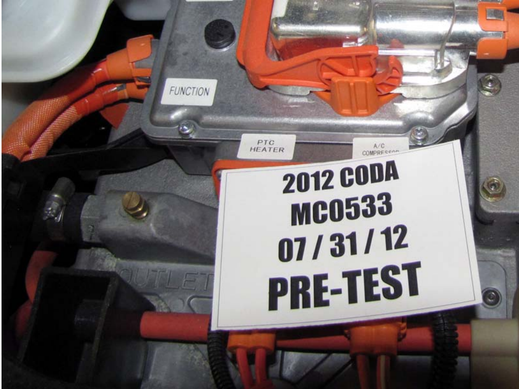
FIGURE 18g. Pre-Impact View of High Voltage Interconnect
