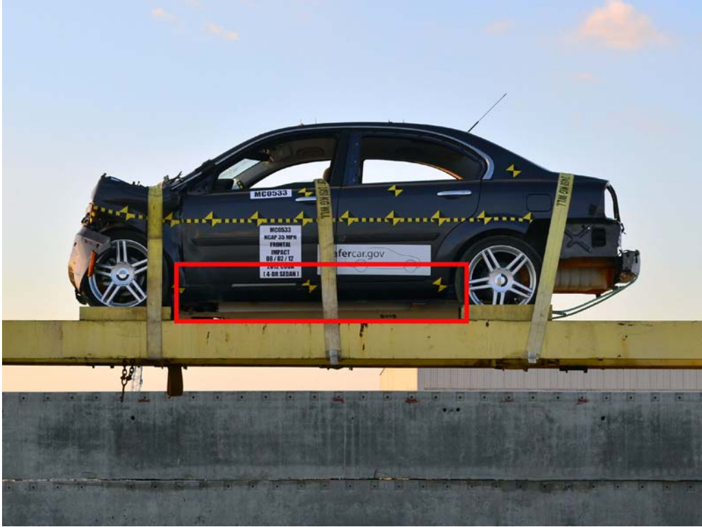
FIGURE 28. FMVSS No. 305 Static Rollover at 0 Degrees
