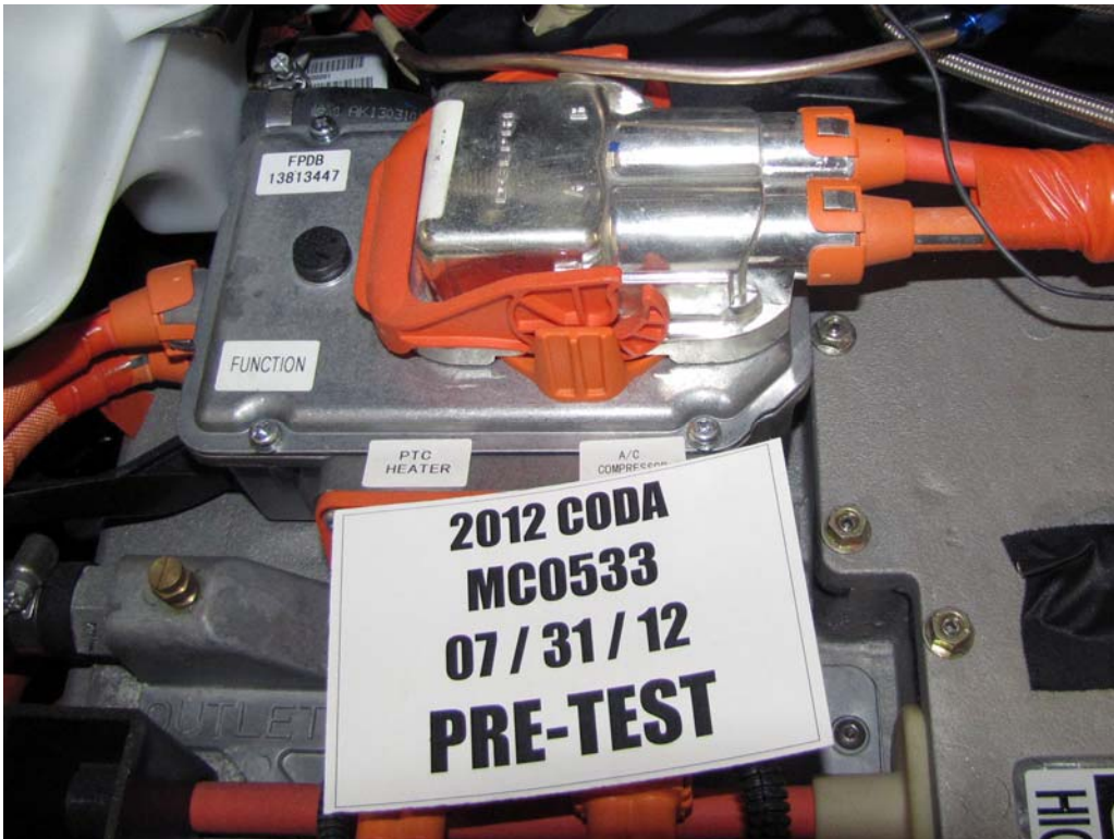
FIGURE 18f. Pre-Impact View of High Voltage Interconnect
