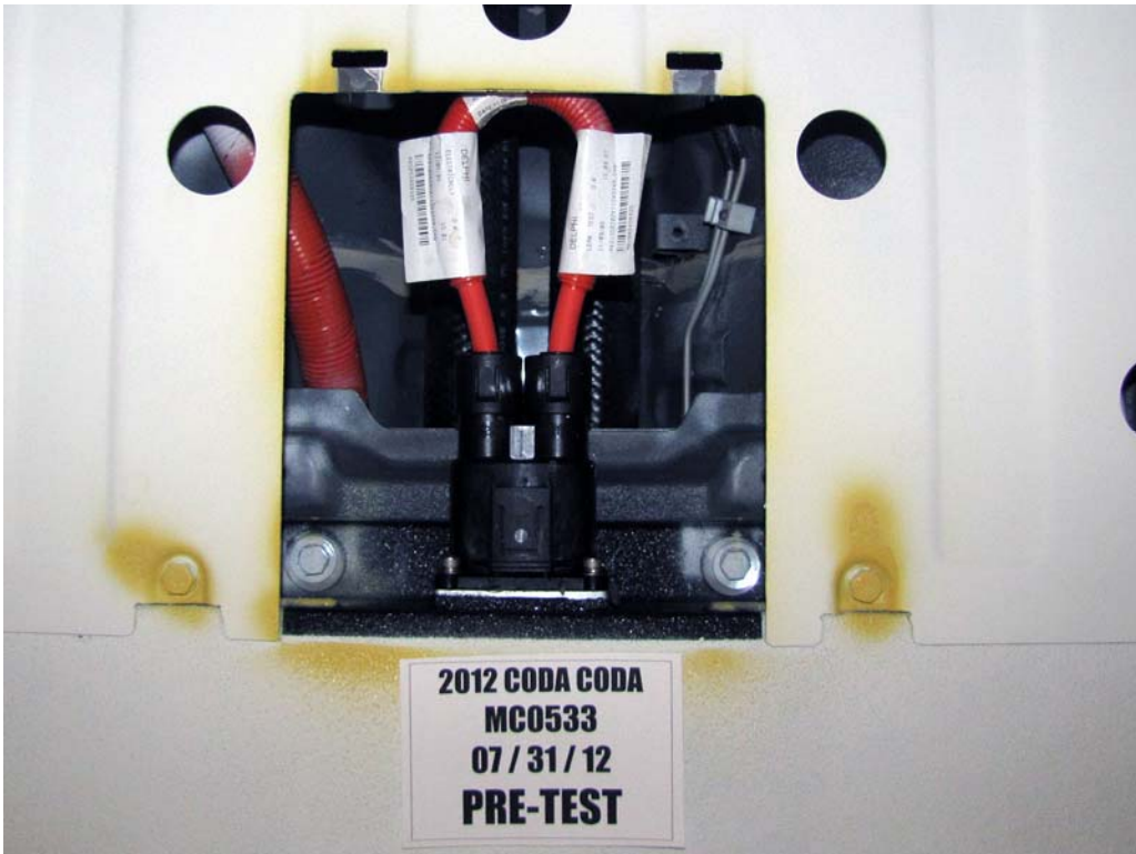
FIGURE 6. Manual High Voltage Disconnect in Place
