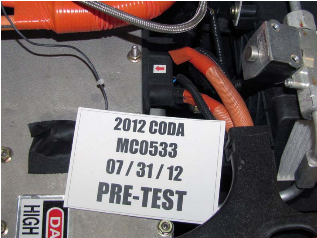
FIGURE 18h. Pre-Impact View of High Voltage Interconnect
