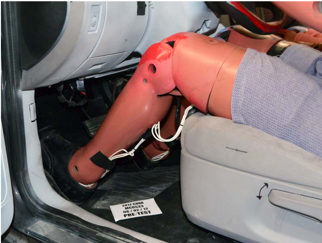
FIGURE 39. Pre-Test Driver Dummy Feet
