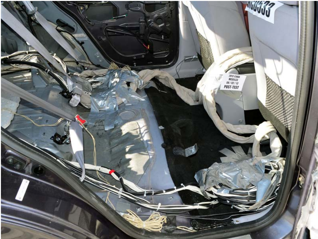
FIGURE 28. Post-Test Dummy Cable Routing
