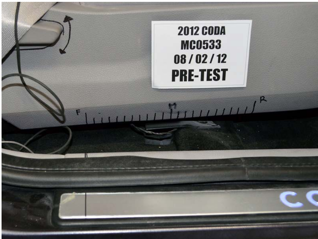
FIGURE 56. Pre-Test Passenger's Seat Fore-Aft Markings
