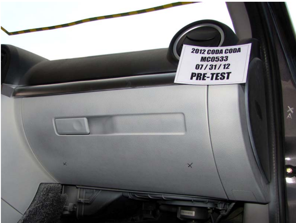
FIGURE 62. Pre-Test Passenger's Side Knee Bolster
