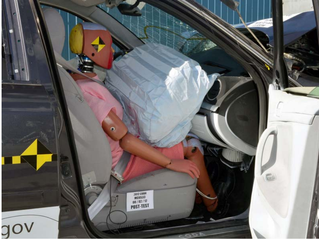
FIGURE 55. Post-Test Passenger Dummy and Vehicle Interior View
