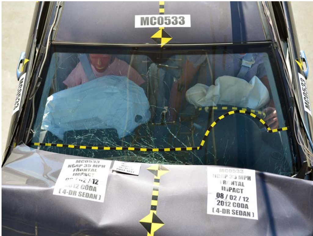
FIGURE 18. Post-Test Windshield View
