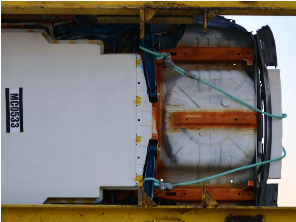
FIGURE 26. Post-Test Rear Underbody View
