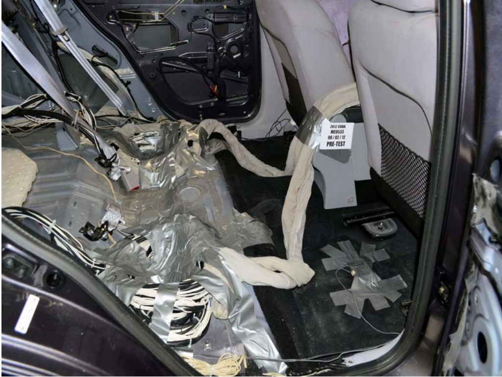
FIGURE 27. Pre-Test Dummy Cable Routing
