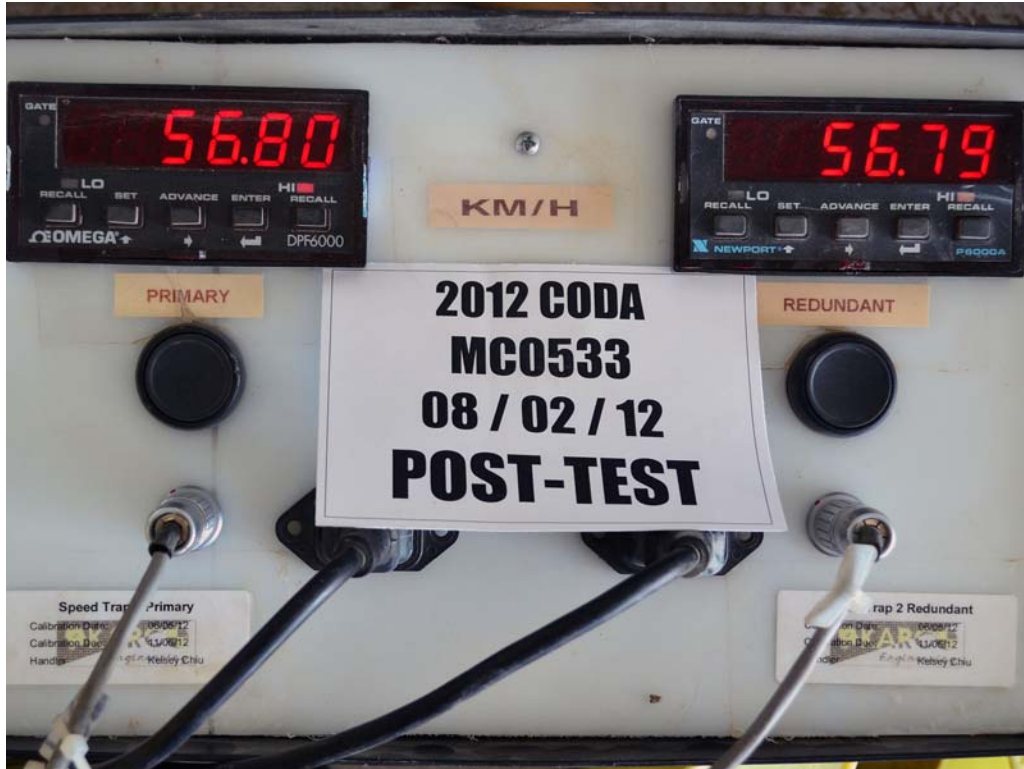
FIGURE 69. Post-Test Speed Trap Read Out
