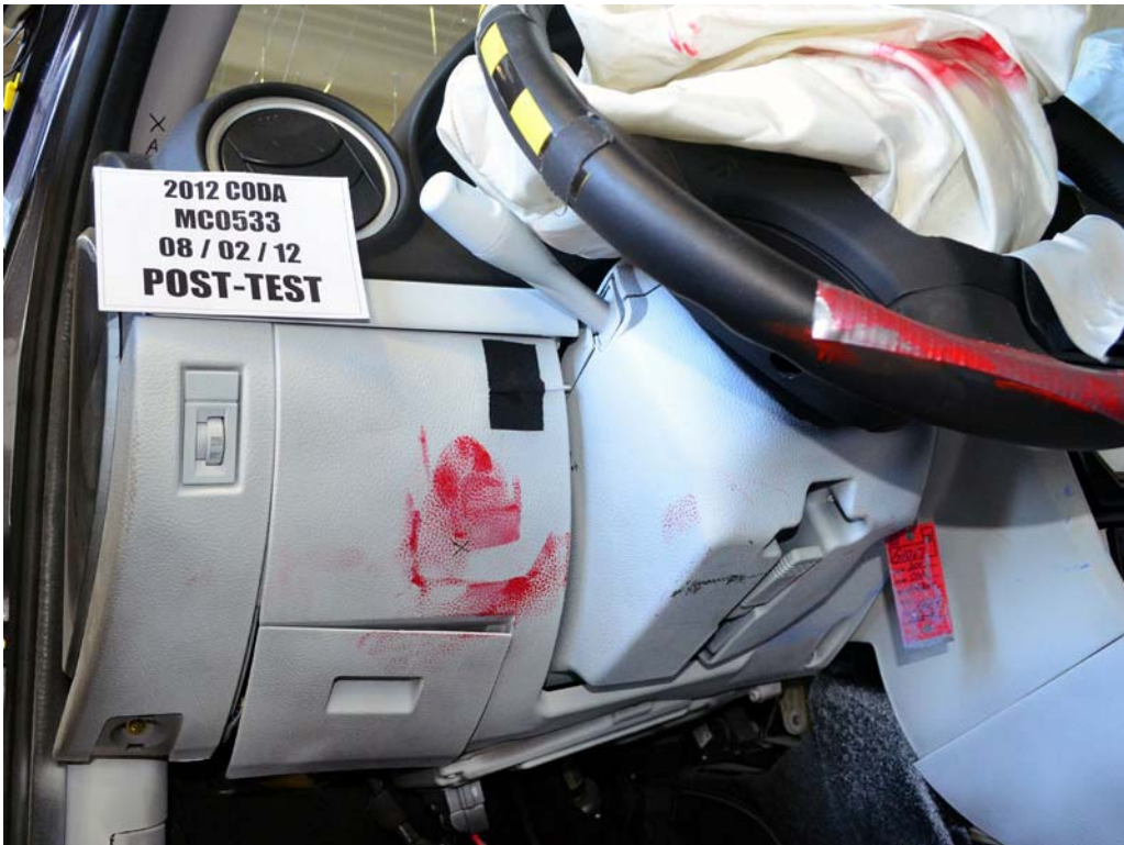
FIGURE 42. Post-Test Driver's Side Knee Bolster
