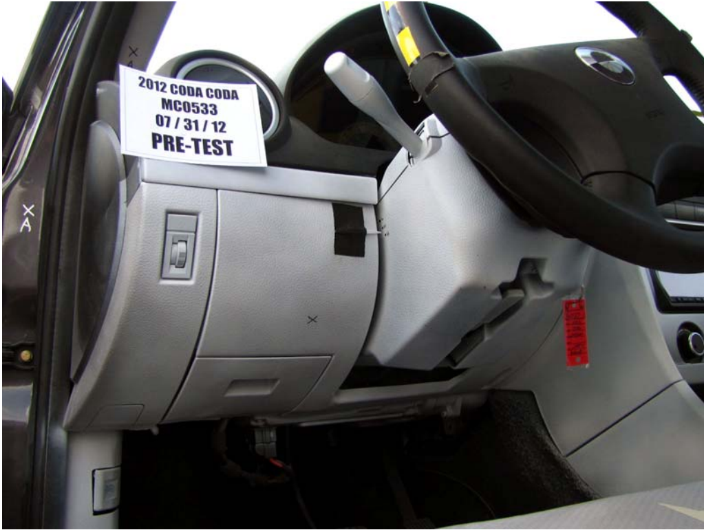
FIGURE 41. Pre-Test Driver's Side Knee Bolster
