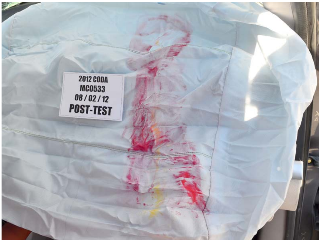
FIGURE 66. Post-Test Passenger Dummy Contact With Airbag
