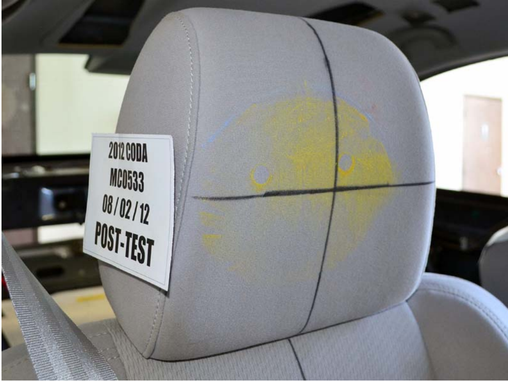
FIGURE 66a. Post-Test Passenger Dummy Contact With Headrest
