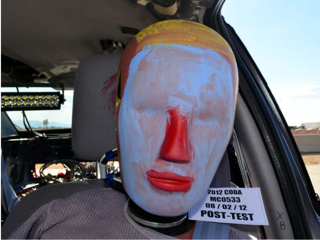
FIGURE 45. Post-Test Driver Dummy Face
