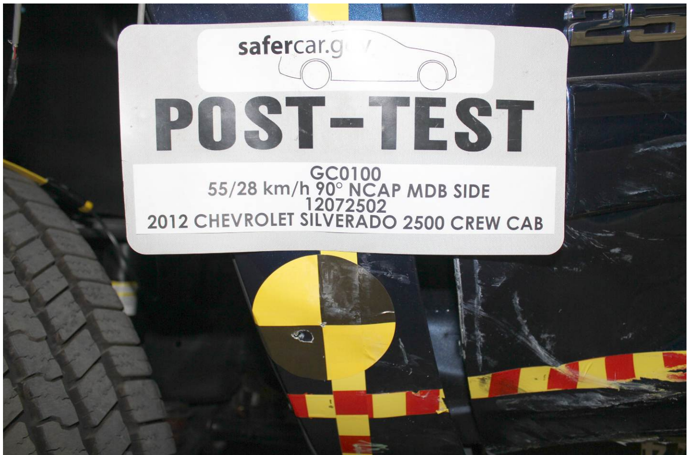
Post-Test Close-Up View of Impact Point Target
