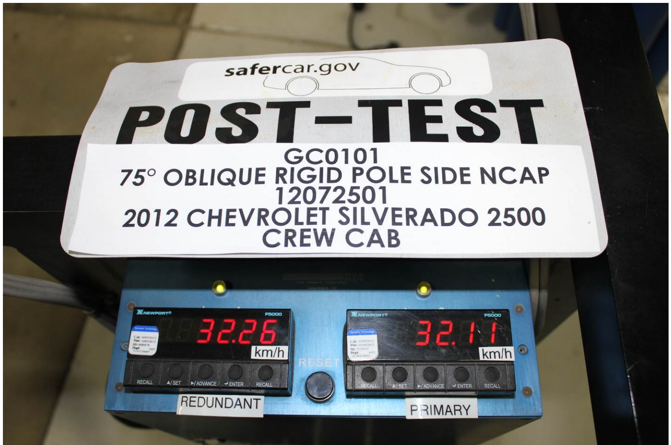
Post-Test Primary and Redundant Speed Trap Read-Out
