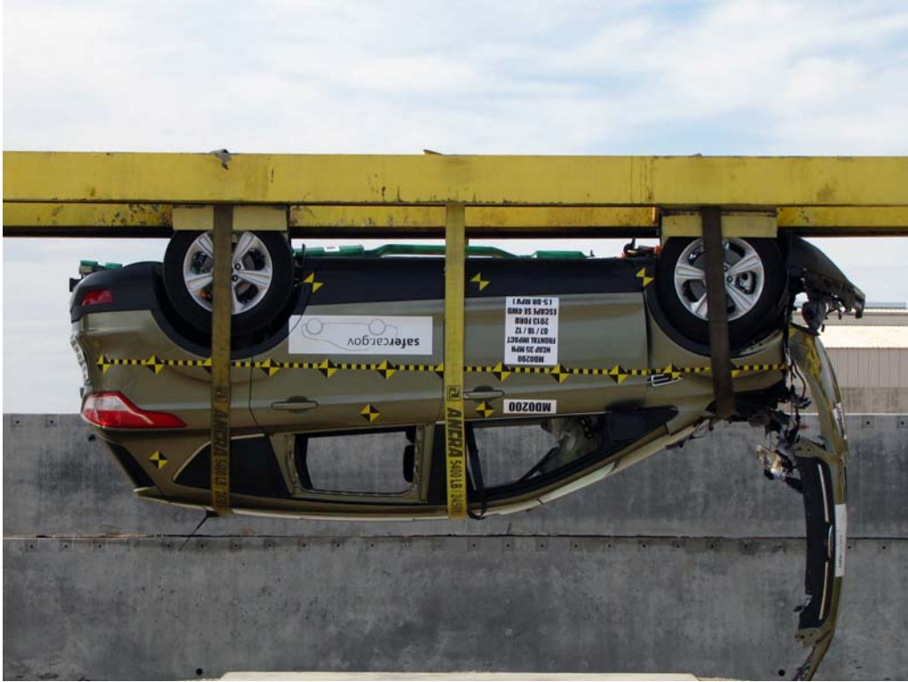
FIGURE 72. Vehicle at 180° on Static Rollover Device
