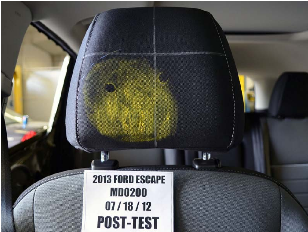
FIGURE 66a. Post-Test Passenger Dummy Contact With Headrest
