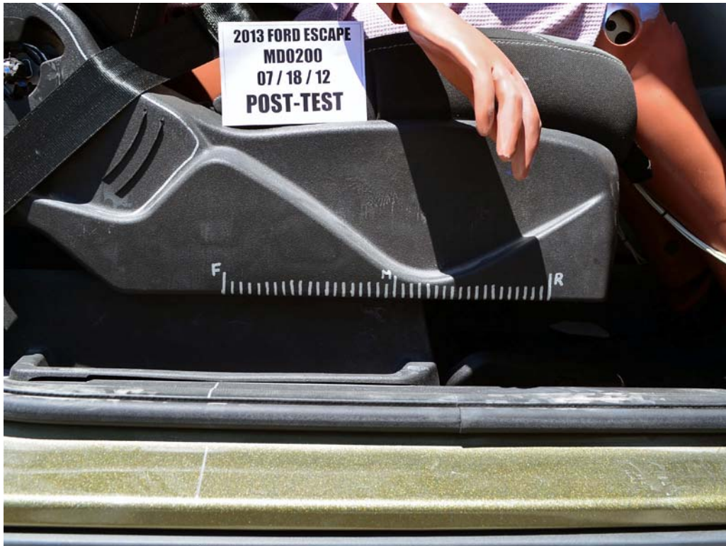
FIGURE 57. Post-Test Passenger's Seat Fore-Aft Markings
