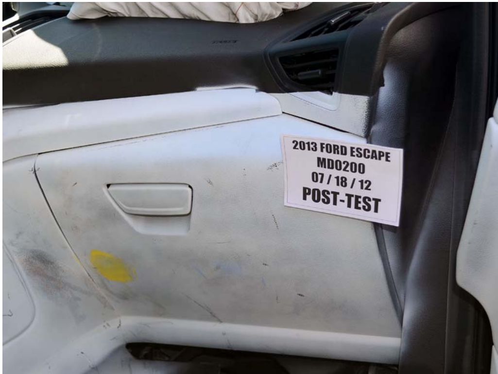
FIGURE 63. Post-Test Passenger's Side Knee Bolster
