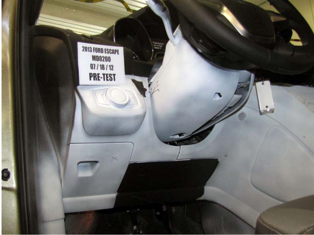
FIGURE 41. Pre-Test Driver's Side Knee Bolster
