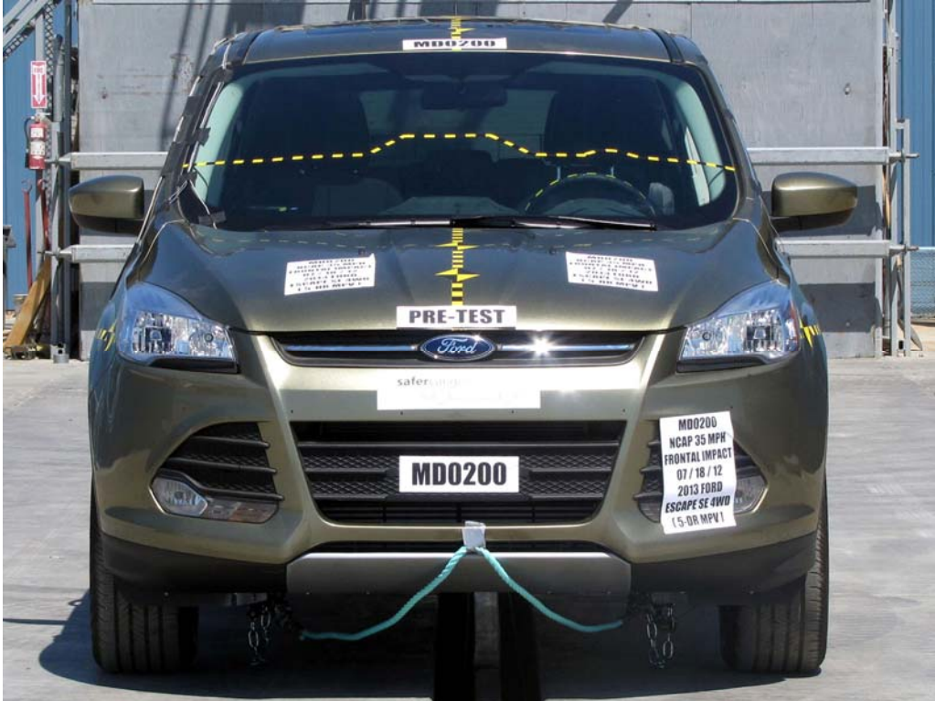
FIGURE 7. Pre-Test Front View of Test Vehicle
