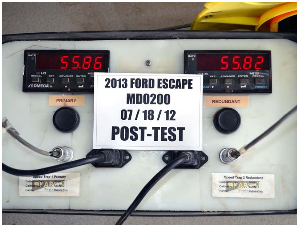
FIGURE 69. Post-Test Speed Trap Read Out
