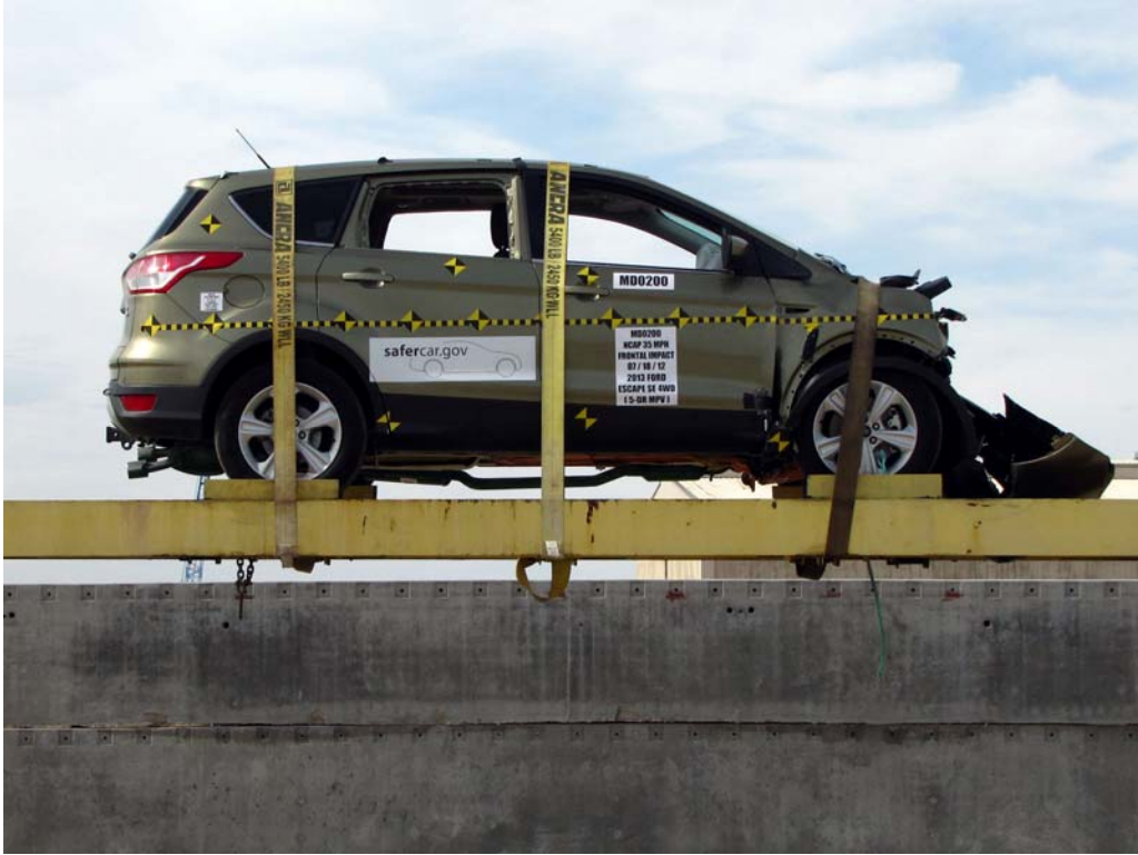
FIGURE 70. Vehicle at 0° on Static Rollover Device
