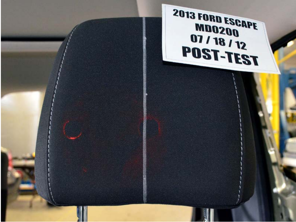
FIGURE 47. Post-Test Driver Dummy Contact With Headrest
