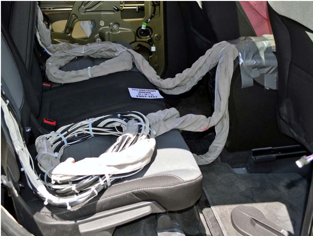
FIGURE 28. Post-Test Dummy Cable Routing
