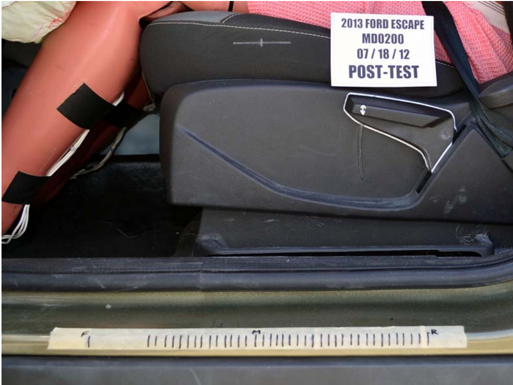
FIGURE 36. Post-Test Driver's Seat Fore-Aft Markings
