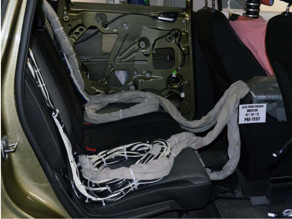
FIGURE 27. Pre-Test Dummy Cable Routing
