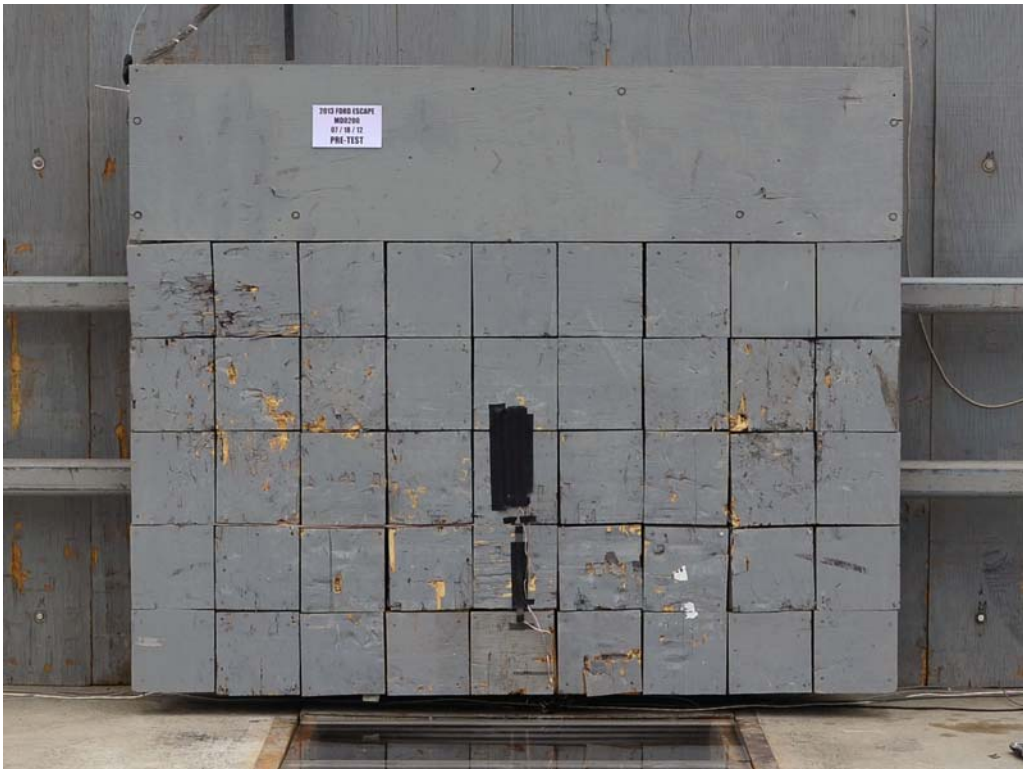
FIGURE 2. Load Cell Wall
