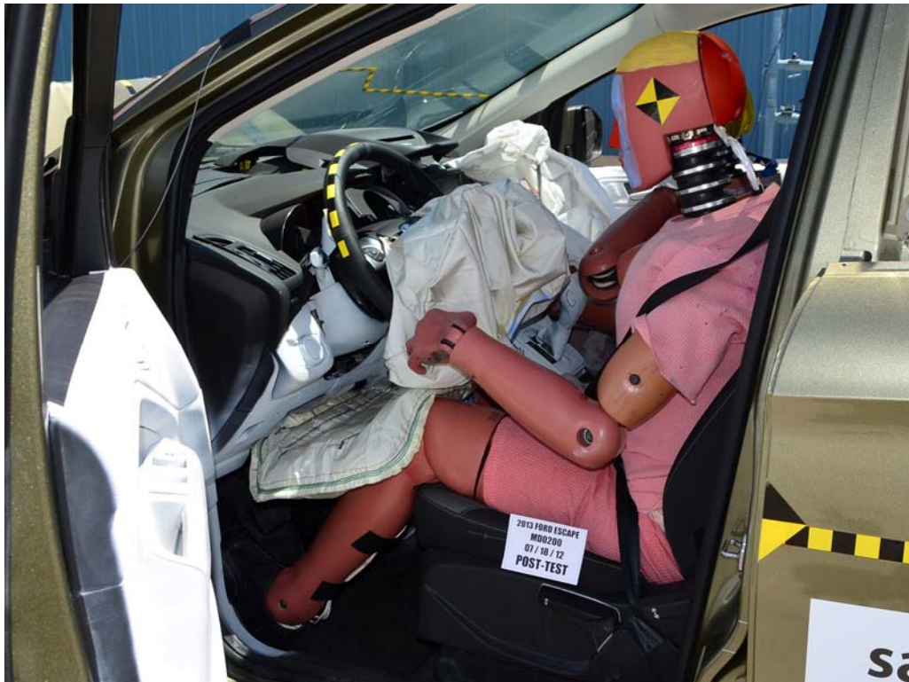
FIGURE 34. Post-Test Driver Dummy and Vehicle Interior View
