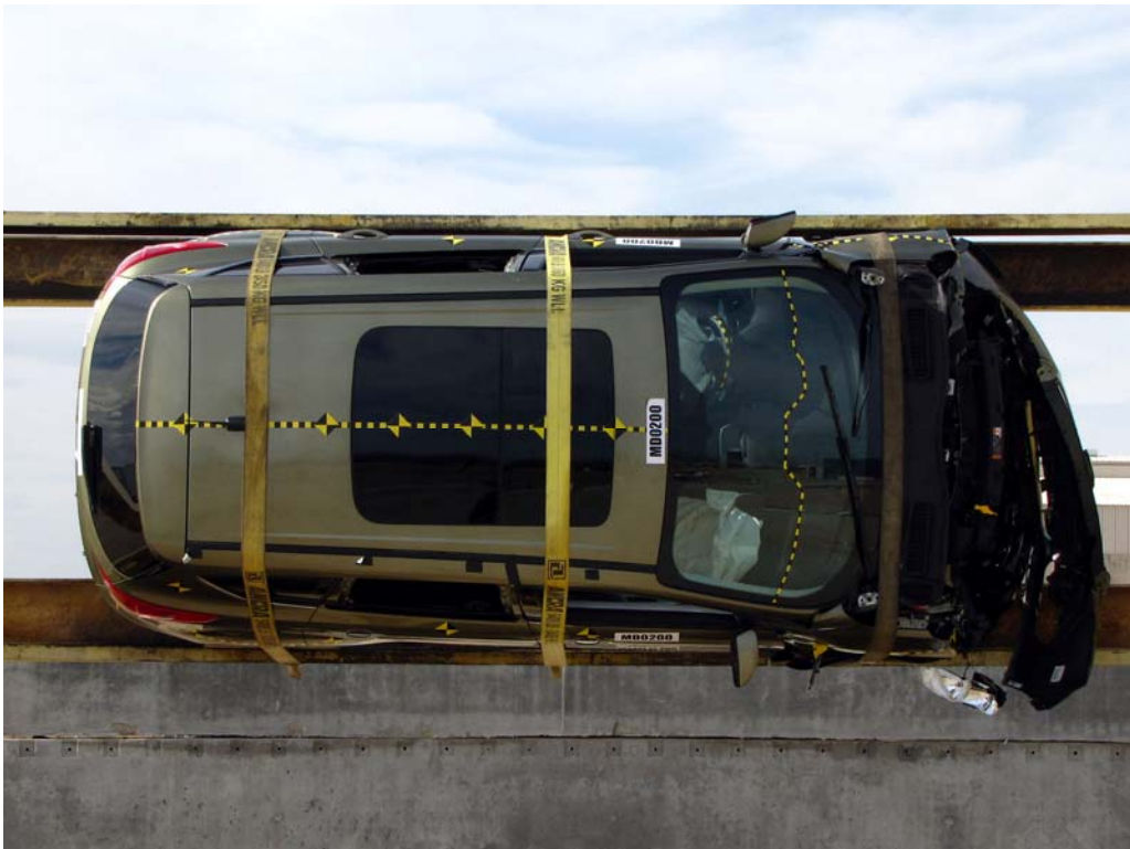
FIGURE 71. Vehicle at 90° on Static Rollover Device
