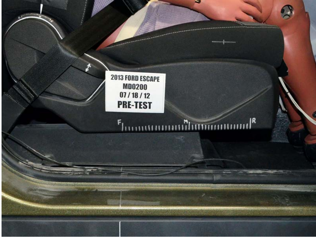
FIGURE 56. Pre-Test Passenger's Seat Fore-Aft Markings
