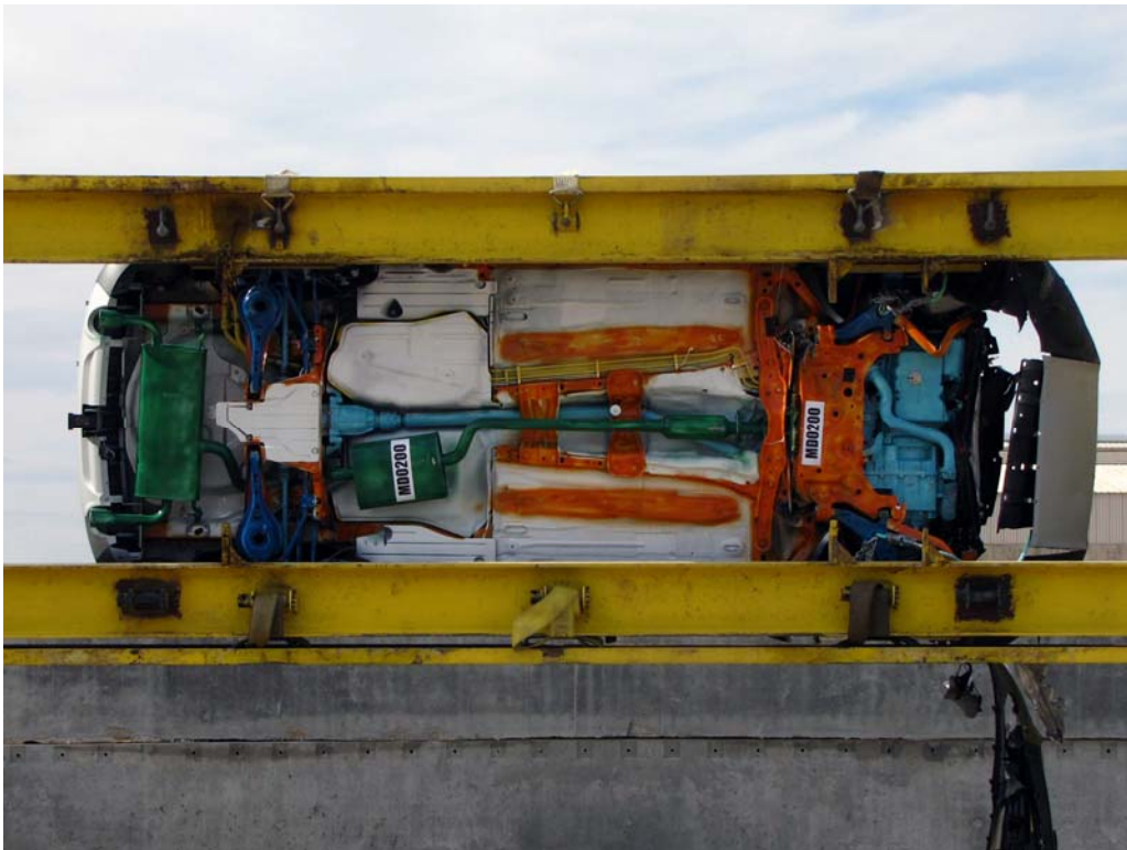
FIGURE 73. 2013 Vehicle at 270° on Static Rollover Device
