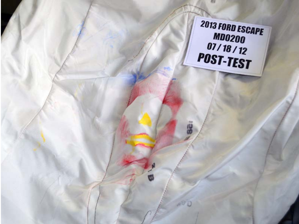
FIGURE 66. Post-Test Passenger Dummy Contact With Airbag
