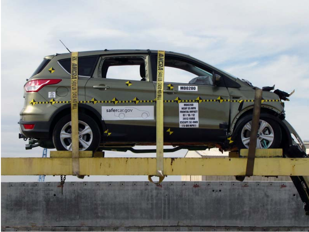
FIGURE 74. Vehicle at 360° on Static Rollover Device
