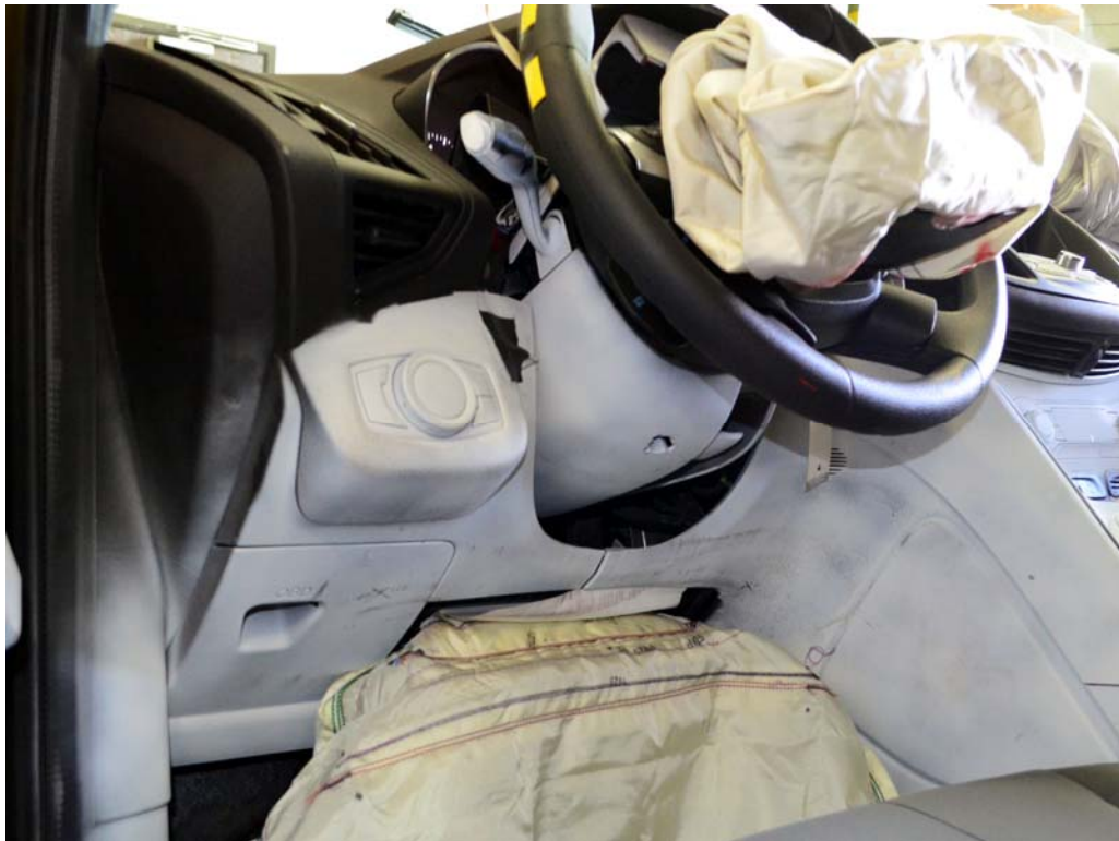
FIGURE 42. Post-Test Driver's Side Knee Bolster
