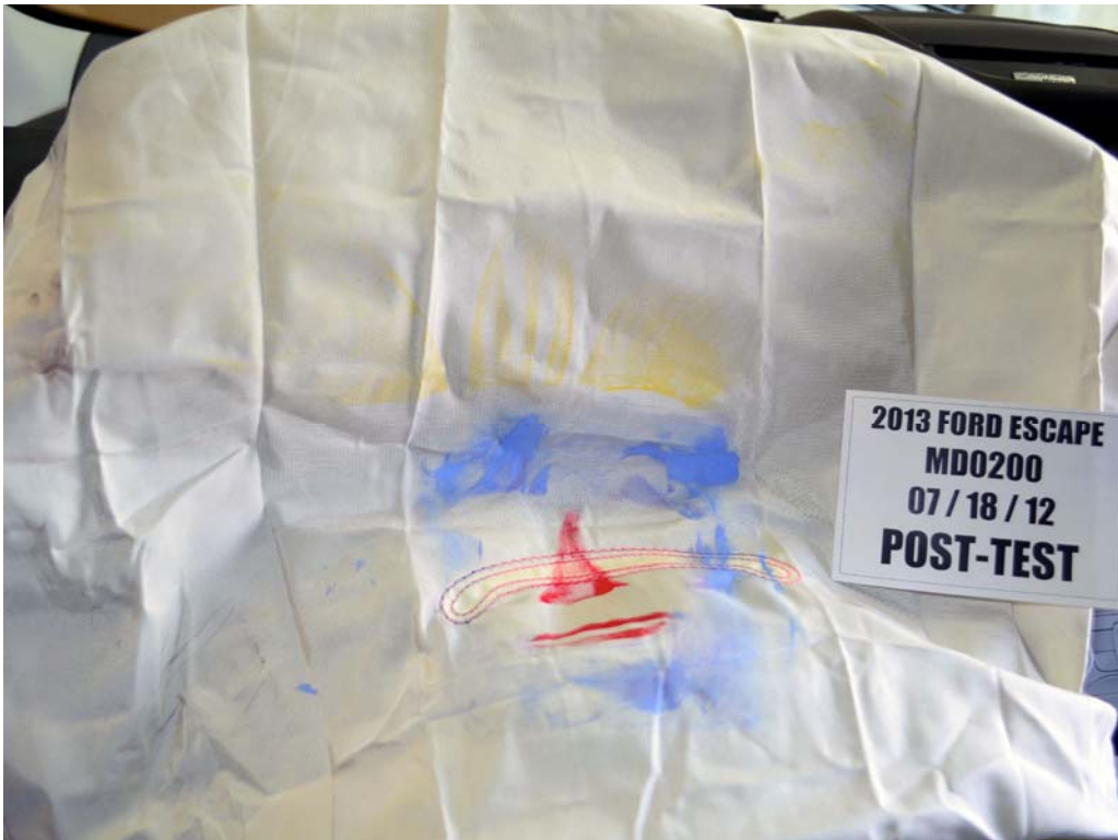
FIGURE 46. Post-Test Driver Dummy Contact With Airbag
