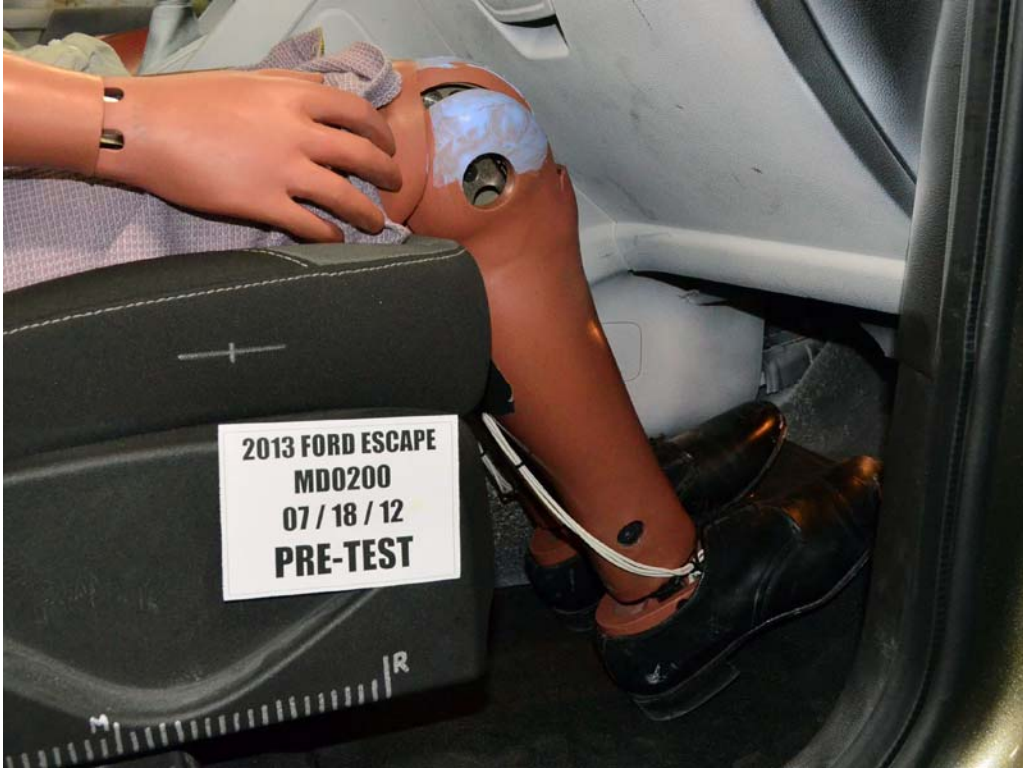
FIGURE 60. Pre-Test Passenger Dummy Feet
