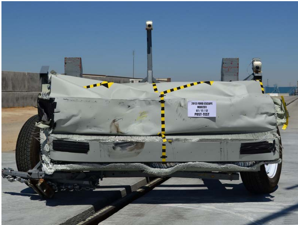
FIGURE 85. Post-Test Front View of MDB Impactor Face
