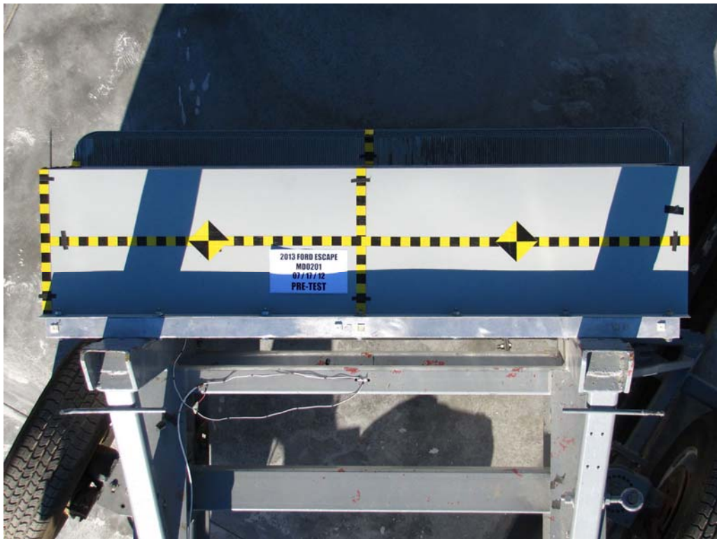
FIGURE 86. Pre-Test Top View of MDB Impactor Face
