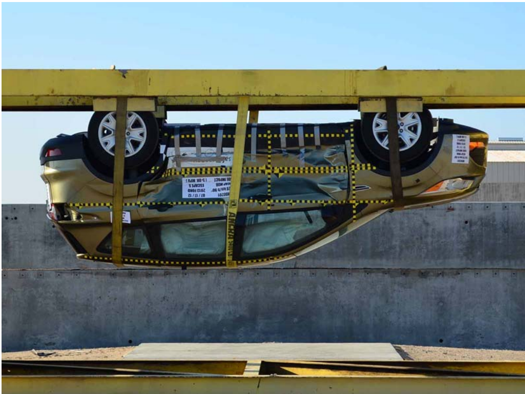
FIGURE 98. FMVSS No. 301 Static Rollover 180 Degrees
