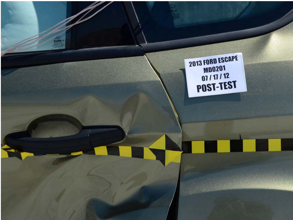
FIGURE 24. Post-Test Left Rear Door Latch Close-Up
