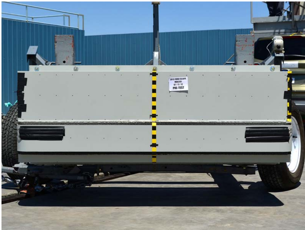
FIGURE 84. Pre-Test Front View of MDB Impactor Face
