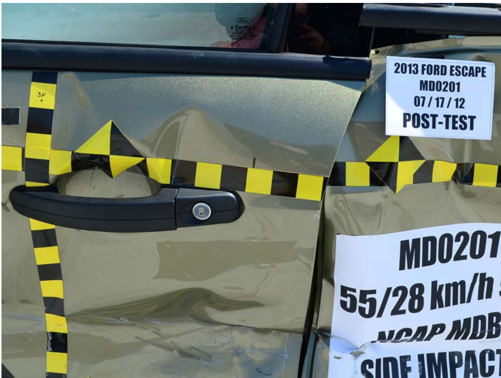
FIGURE 22. Post-Test Left Front Door Latch Close-Up
