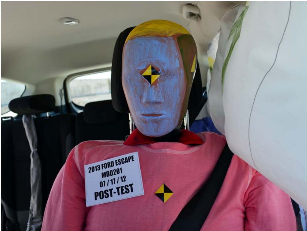
FIGURE 26. Post-Test Front Close-Up View of Driver Dummy
