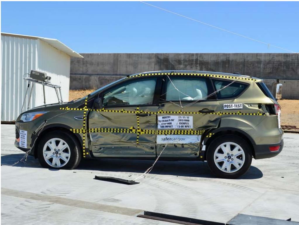
FIGURE 8. Post-Test Left Side View of Test Vehicle
