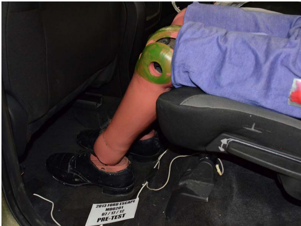
FIGURE 64. Pre-Test Placement of Rear Passenger Dummy's Feet
