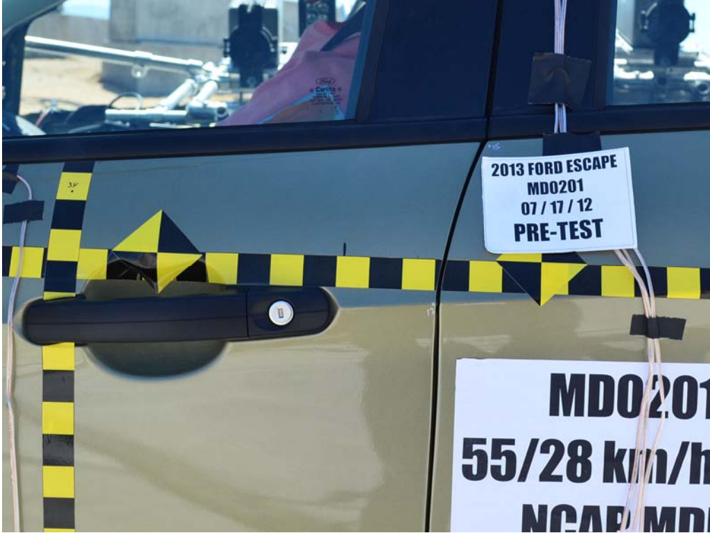
FIGURE 21. Pre-Test Left Front Door Latch Close-Up
