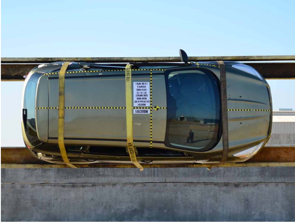
FIGURE 97. FMVSS No. 301 Static Rollover 90 Degrees
