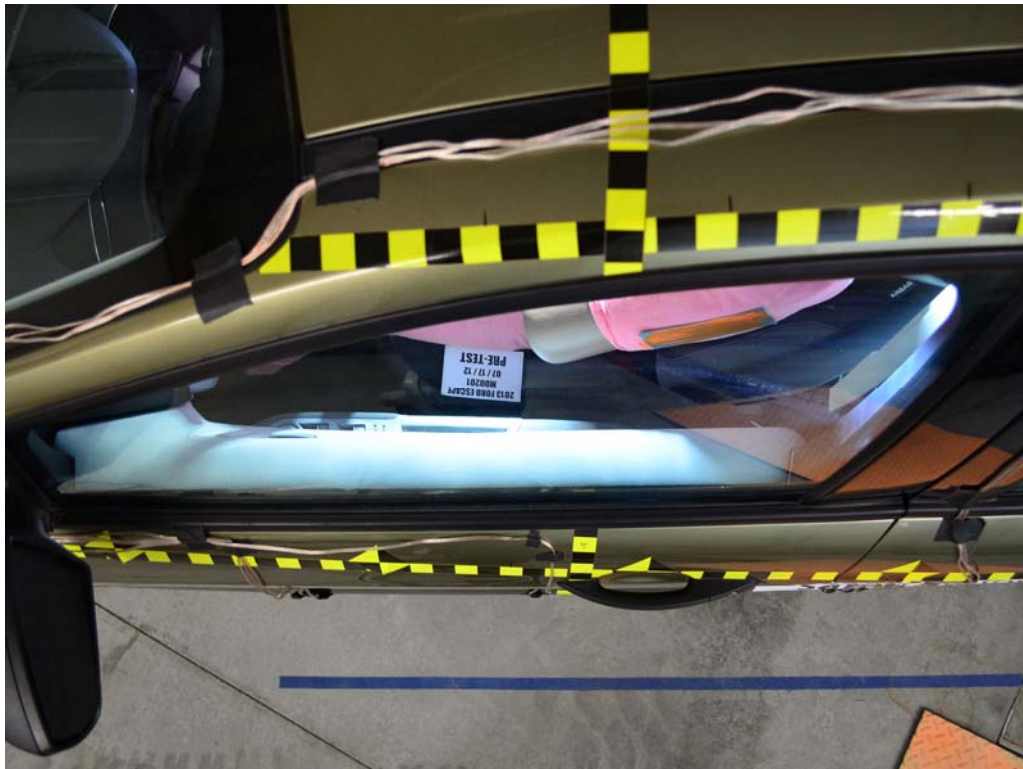
FIGURE 42. Pre-Test Driver Dummy and Door Clearance View
