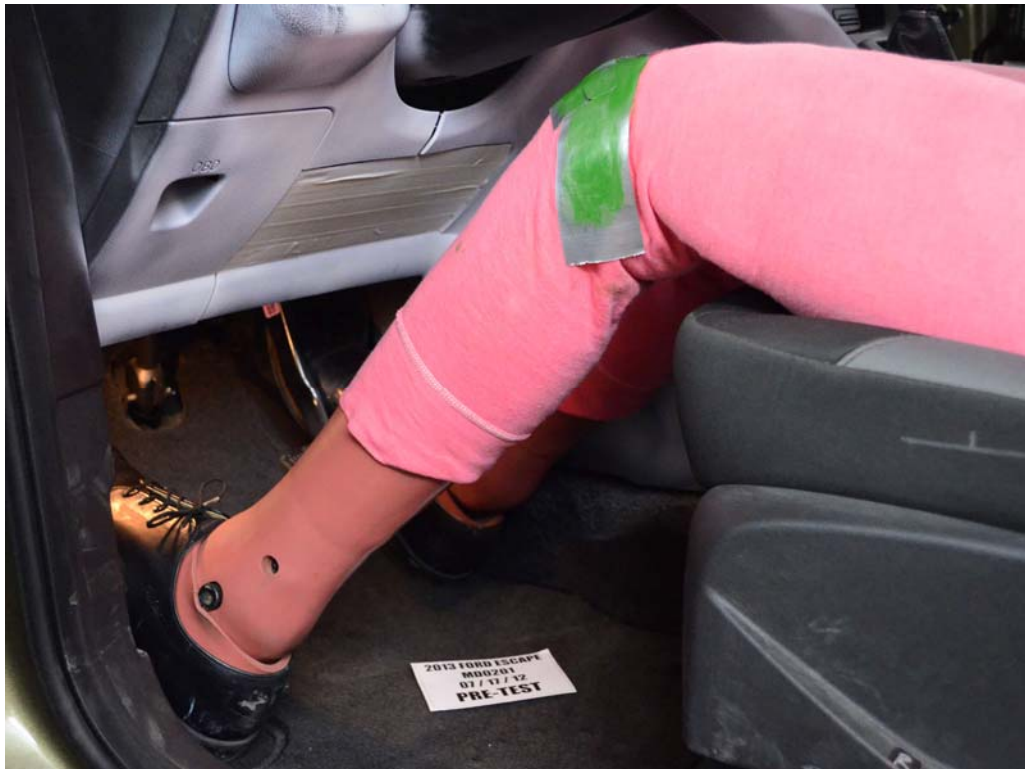
FIGURE 34. Pre-Test Placement of Driver Dummy's Feet
