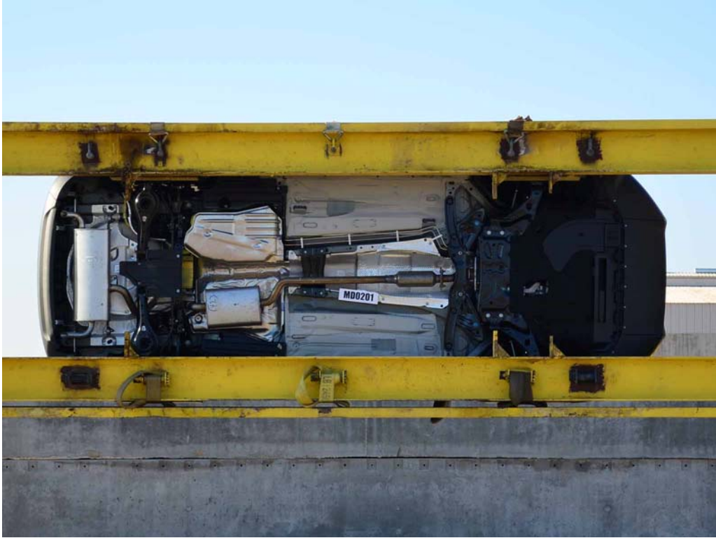
FIGURE 99. FMVSS No. 301 Static Rollover 270 Degrees
