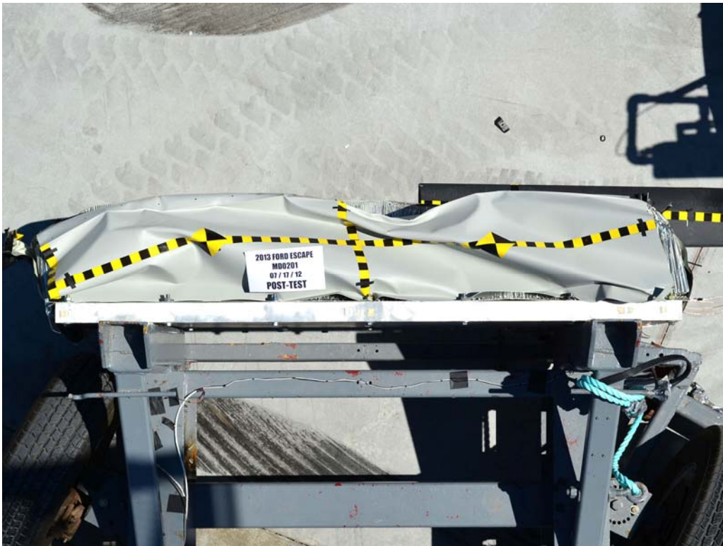
FIGURE 87. Post-Test Top View of MDB Impactor Face
