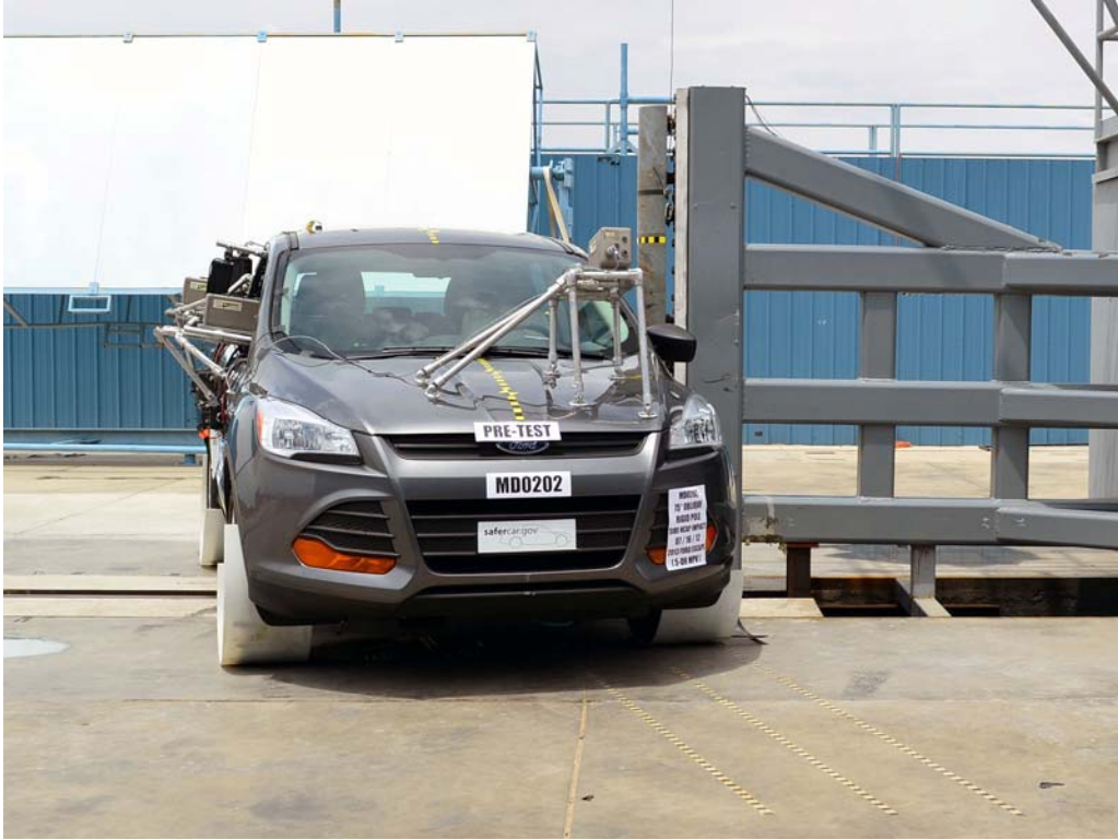
FIGURE 17. Pre-Test Left Side View of Pole Positioned Against Side of Vehicle at Impact Point
