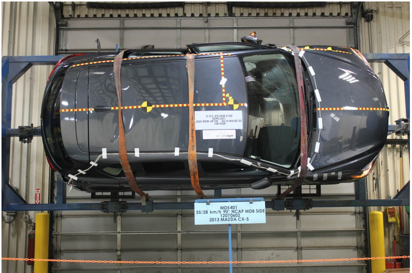
FMVSS No. 301 Static Rollover 270 Degrees
