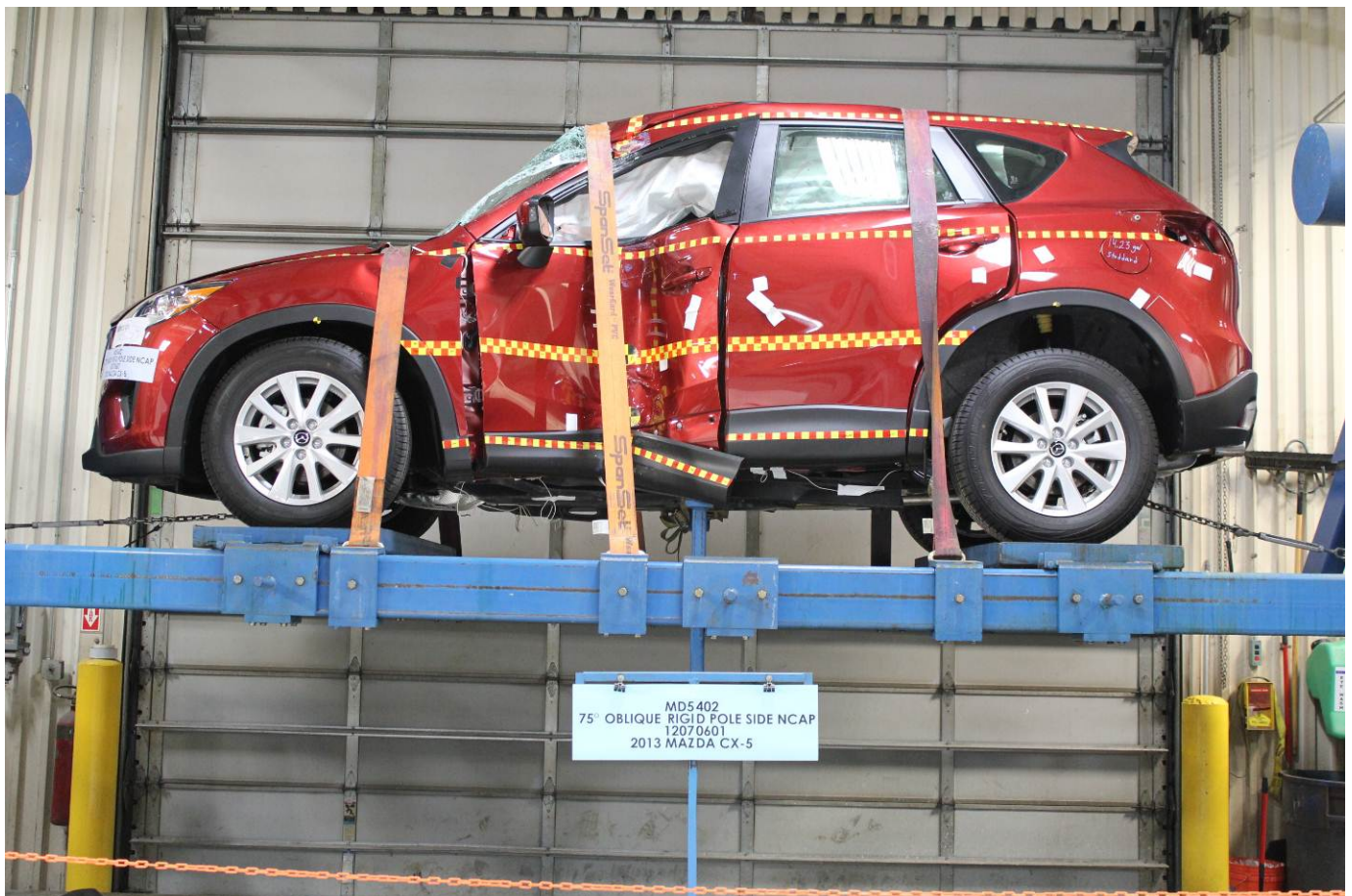
FMVSS No. 301 Static Rollover 360 Degrees
