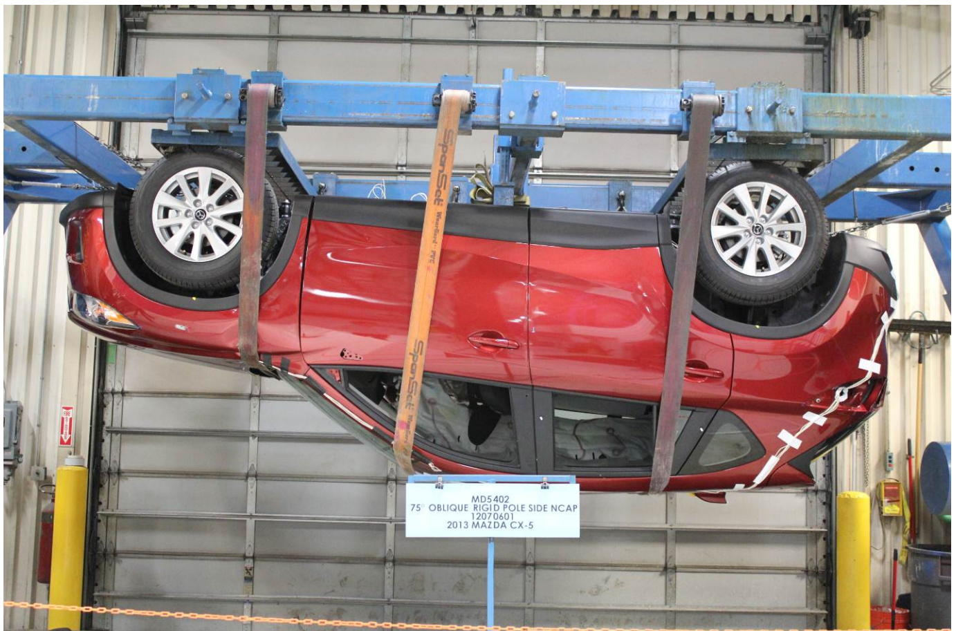
FMVSS No. 301 Static Rollover 180 Degrees
