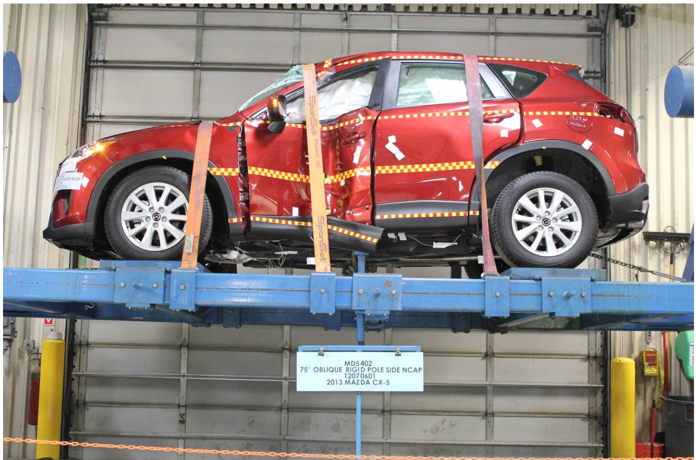
FMVSS No. 301 Static Rollover 0 Degrees
