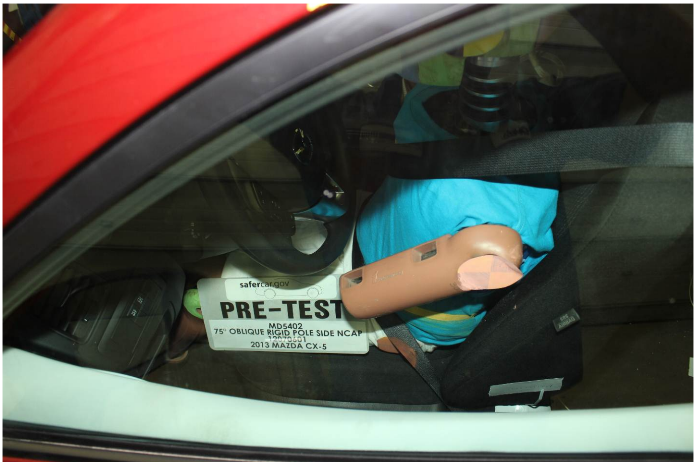
Pre-Test Dummy and Door Clearance View
