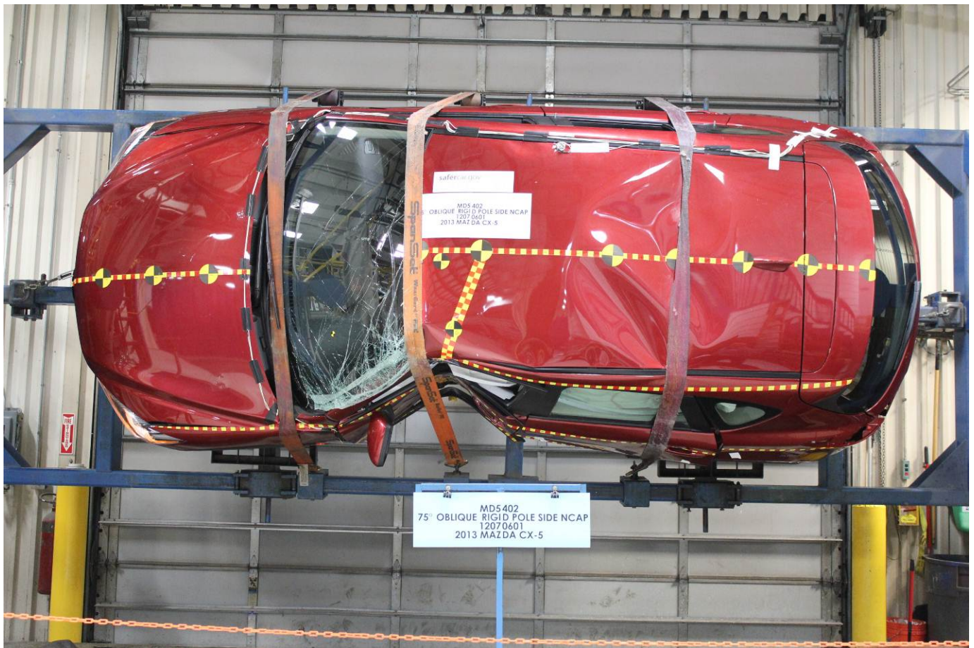
FMVSS No. 301 Static Rollover 90 Degrees
