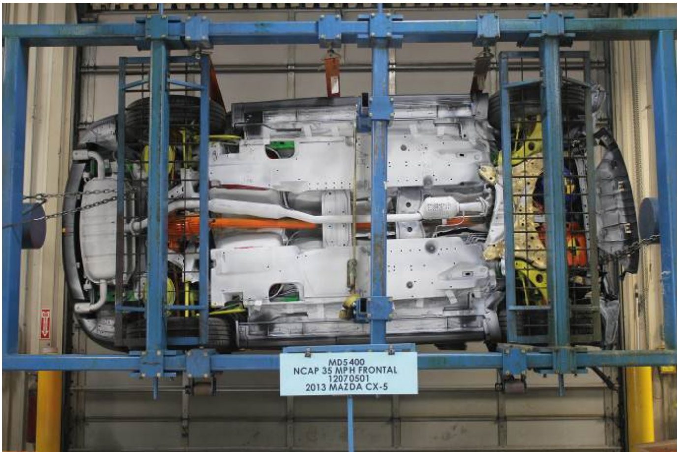
Vehicle at 90° on Static Rollover Device
