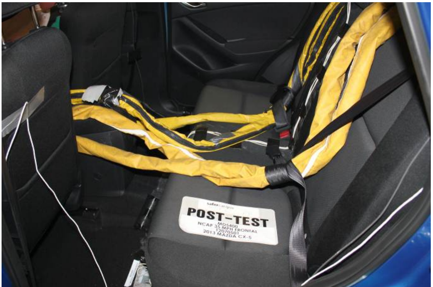
Post-Test Dummy Cable Routing
