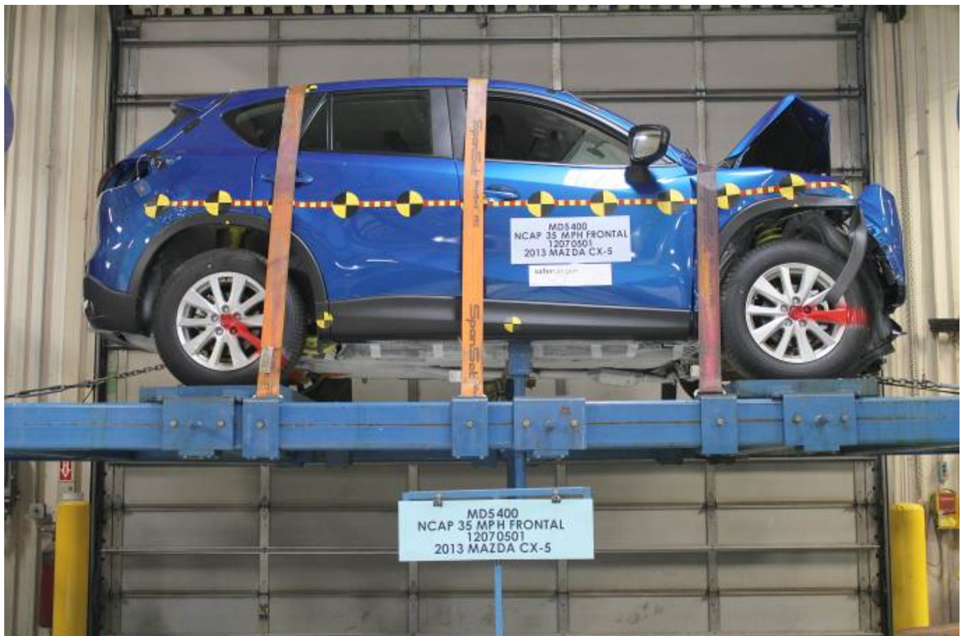
Vehicle at 0° on Static Rollover Device
