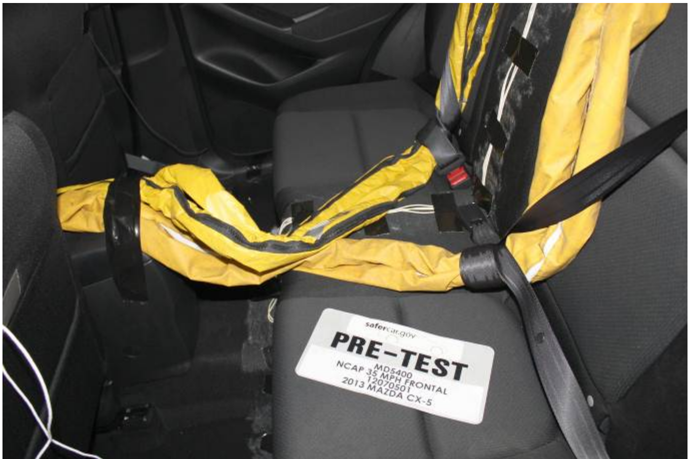
Pre-Test Dummy Cable Routing
