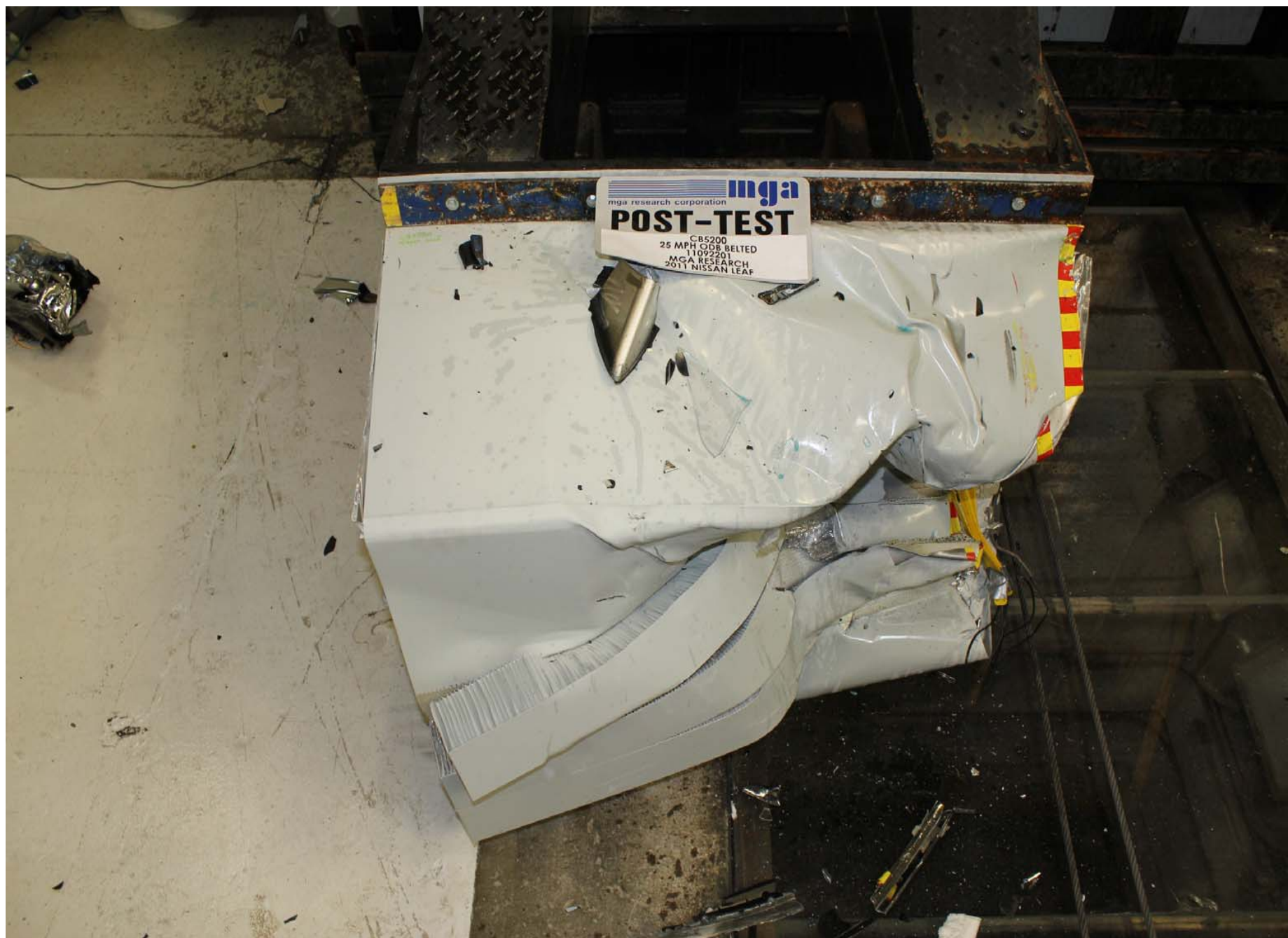
Post-Test Offset Deformable Barrier Top View
