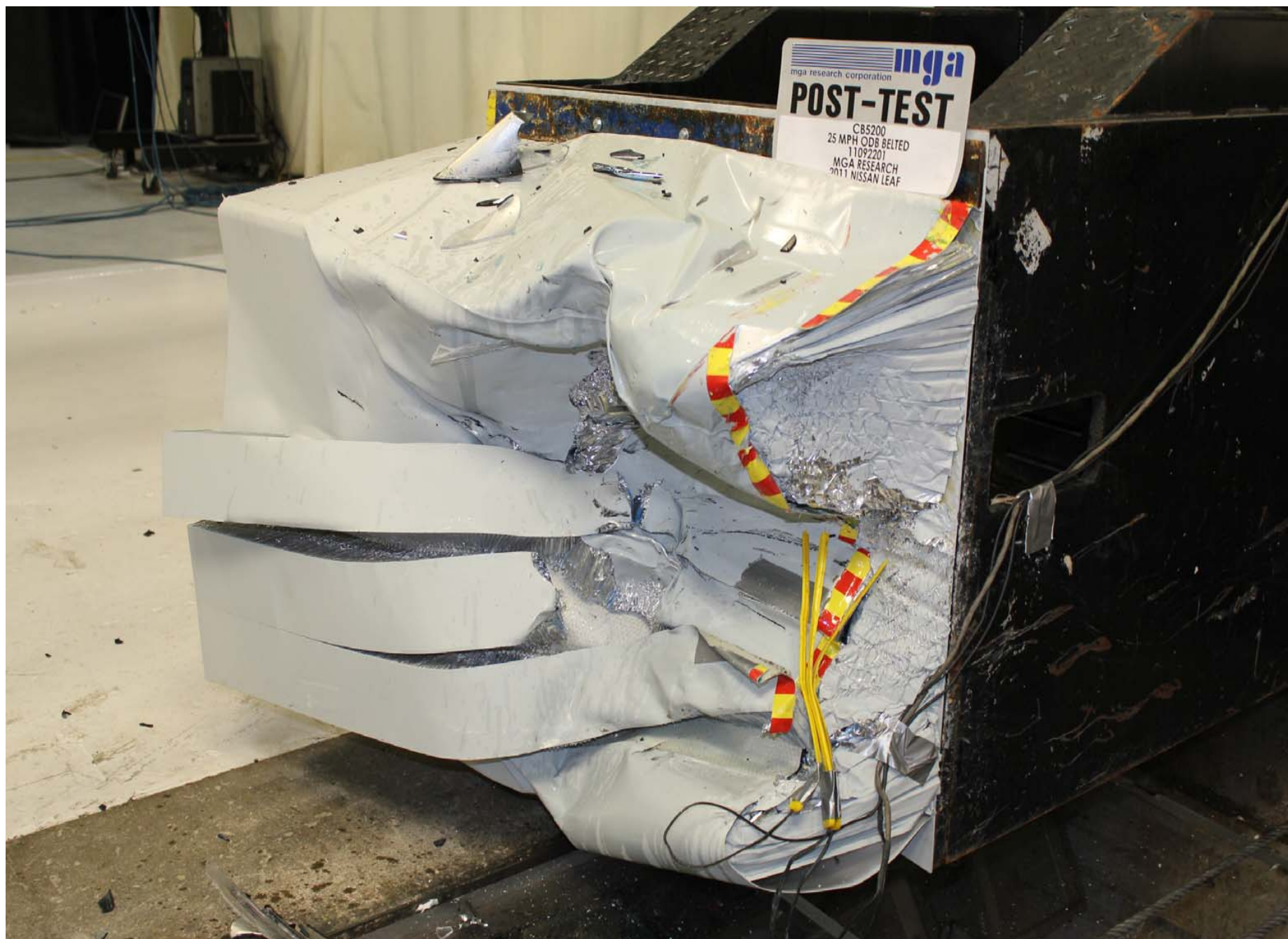
Post-Test Left Front Three-Quarter View of Offset Deformable Barrier
