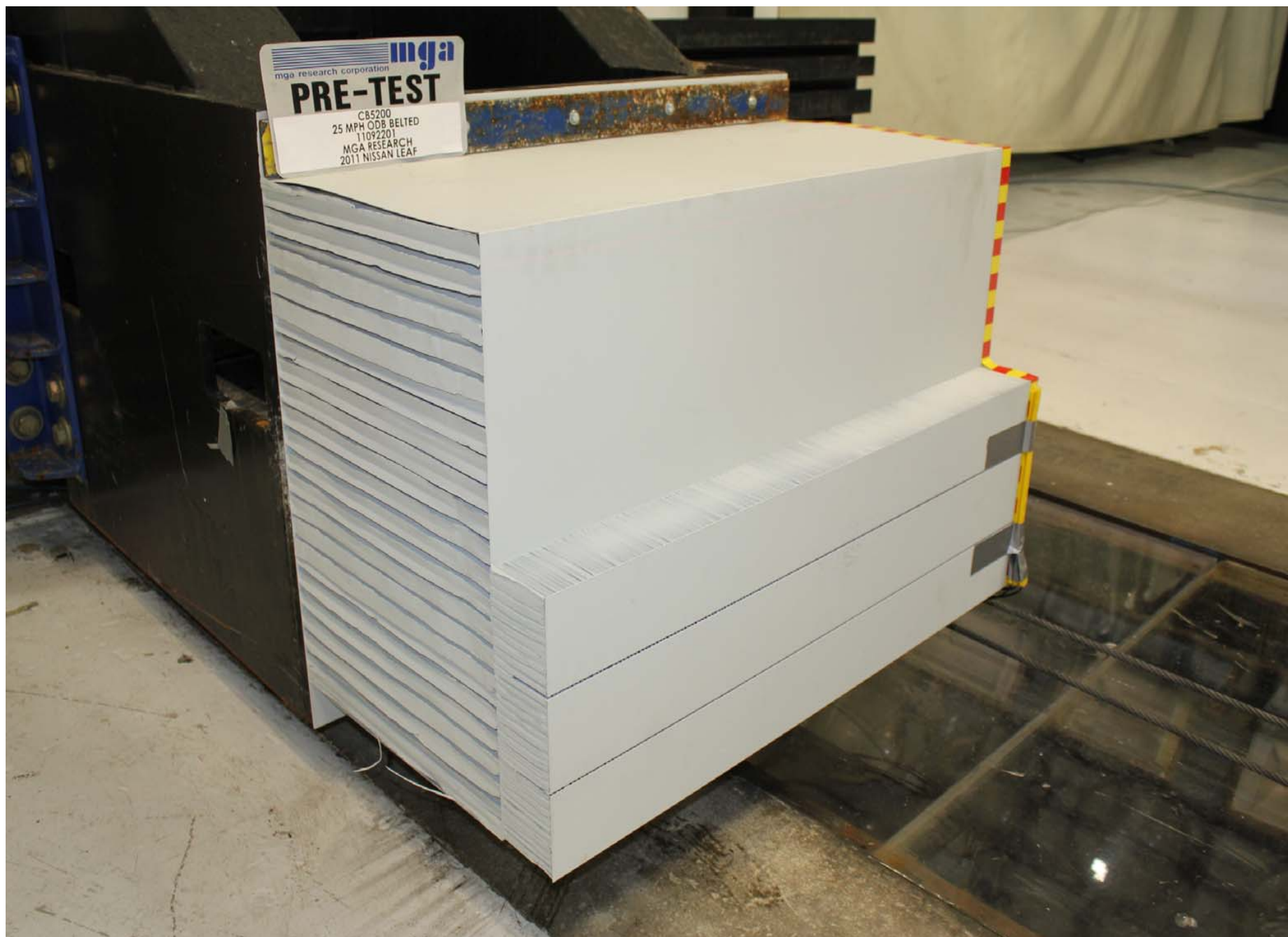
Pre-Test Right Front Three-Quarter View of Offset Deformable Barrier
