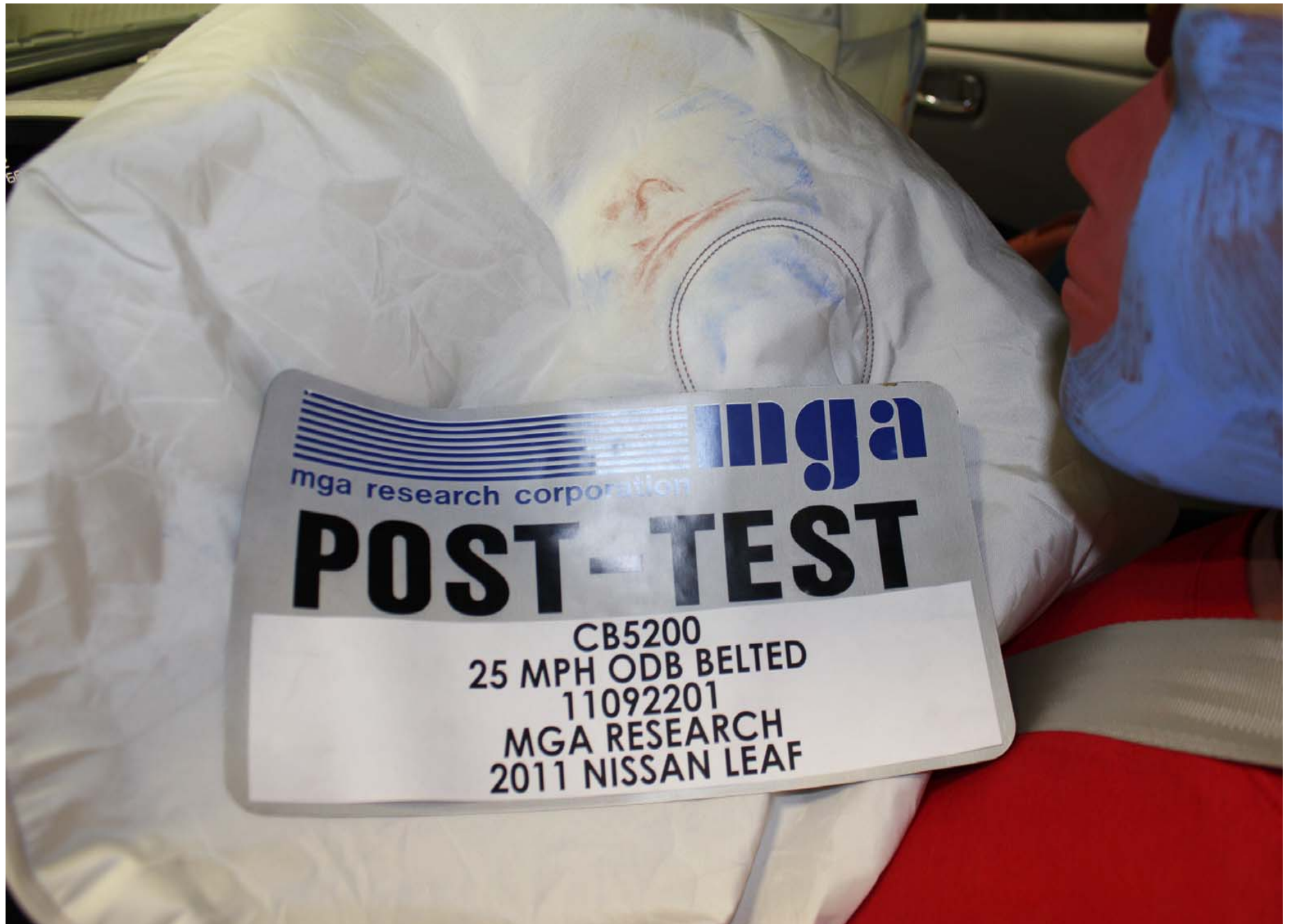
Post-Test Driver Dummy Airbag Contact
