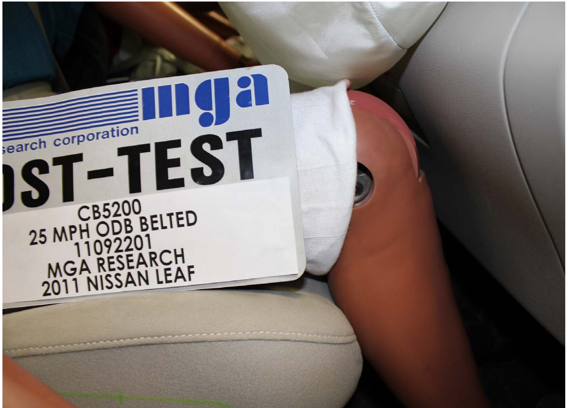
Post-Test Passenger Side Knee Bolster View
