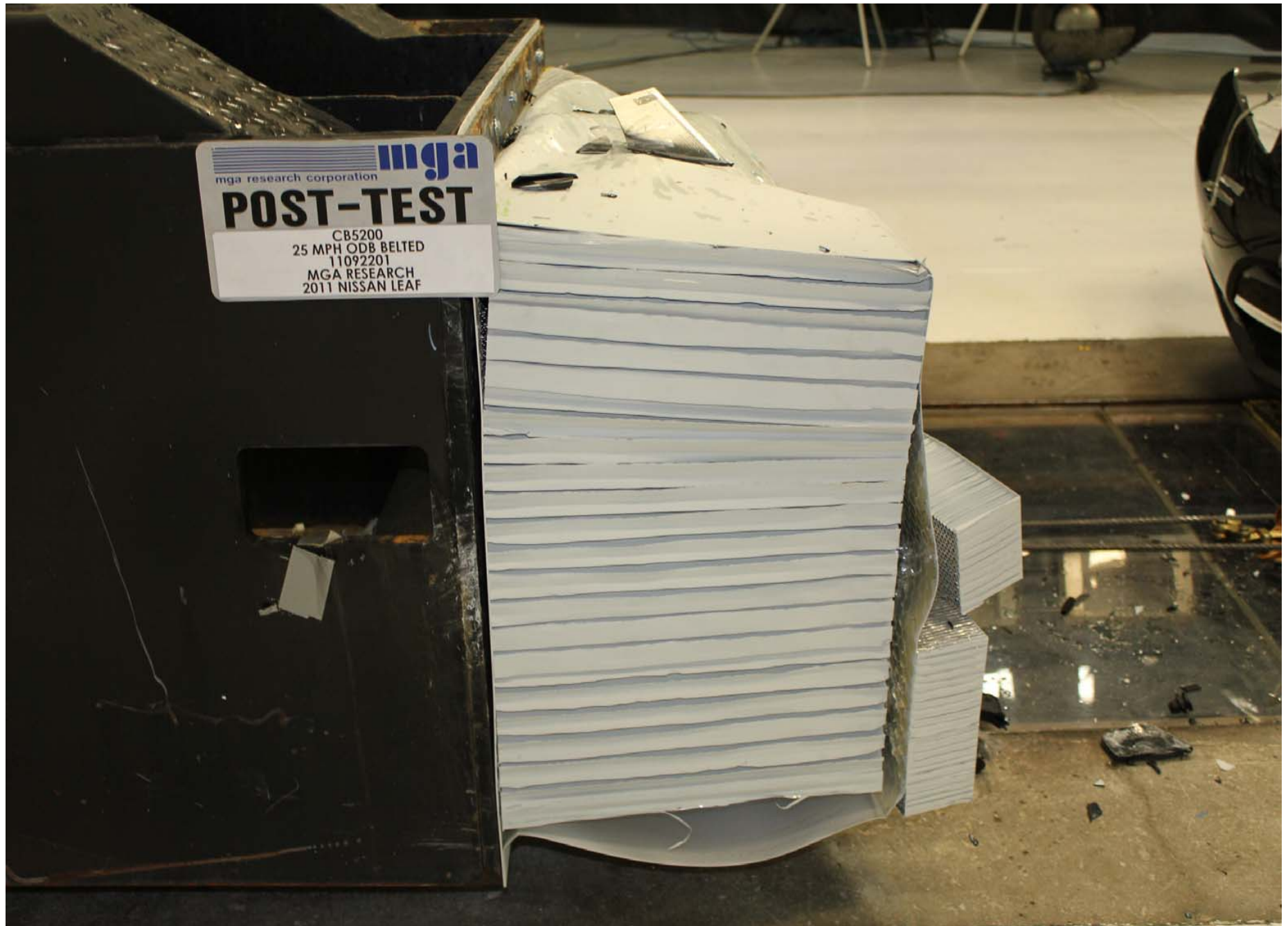
Post-Test Offset Deformable Barrier Right Side View
