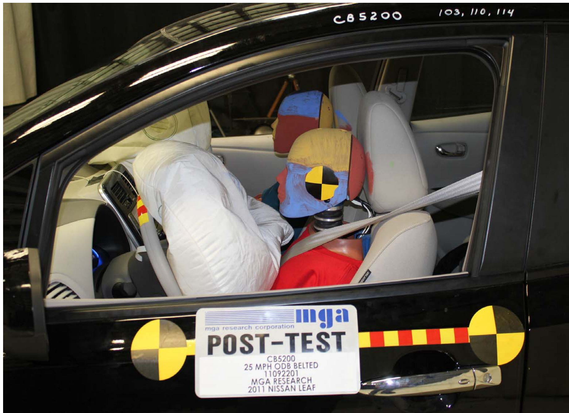
Post-Test Driver Dummy Position Left Side View
