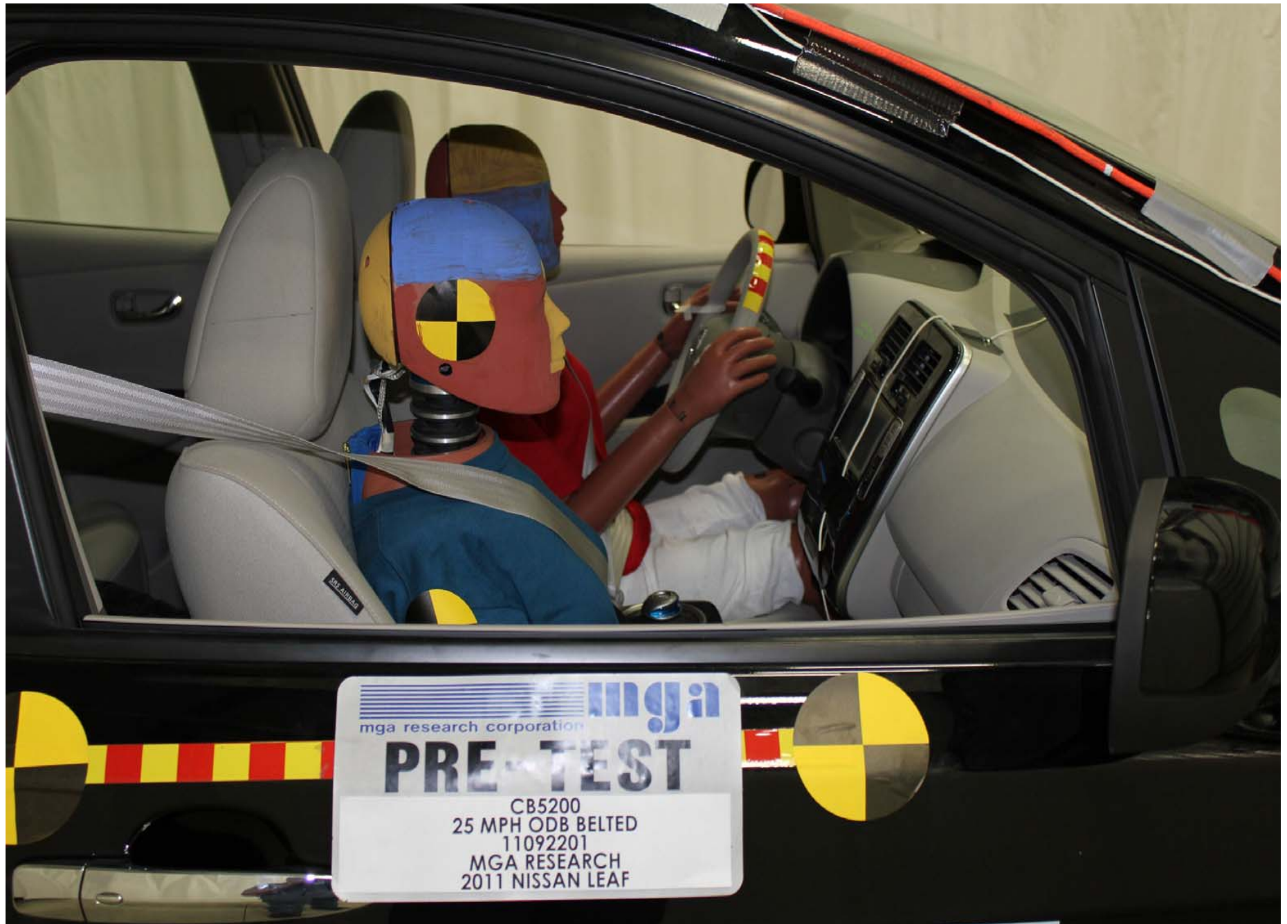
Pre-Test Passenger Dummy Position Right Side View
