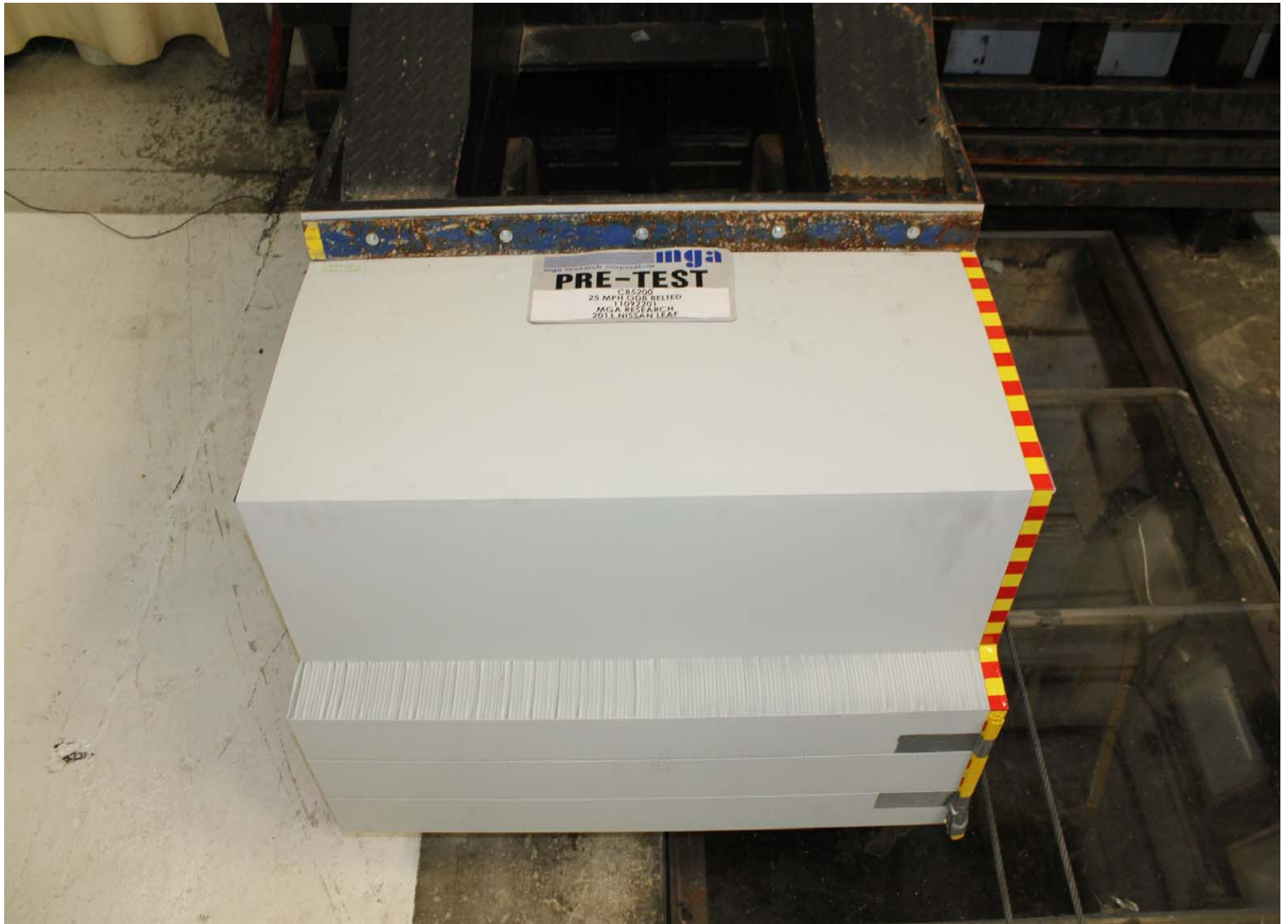
Pre-Test Offset Deformable Barrier Top View
