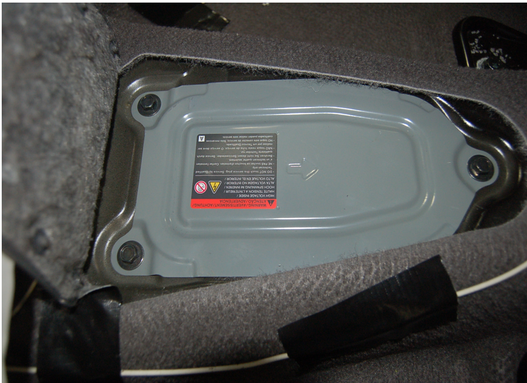
Manual High Voltage Service Disconnect Close-Up View
