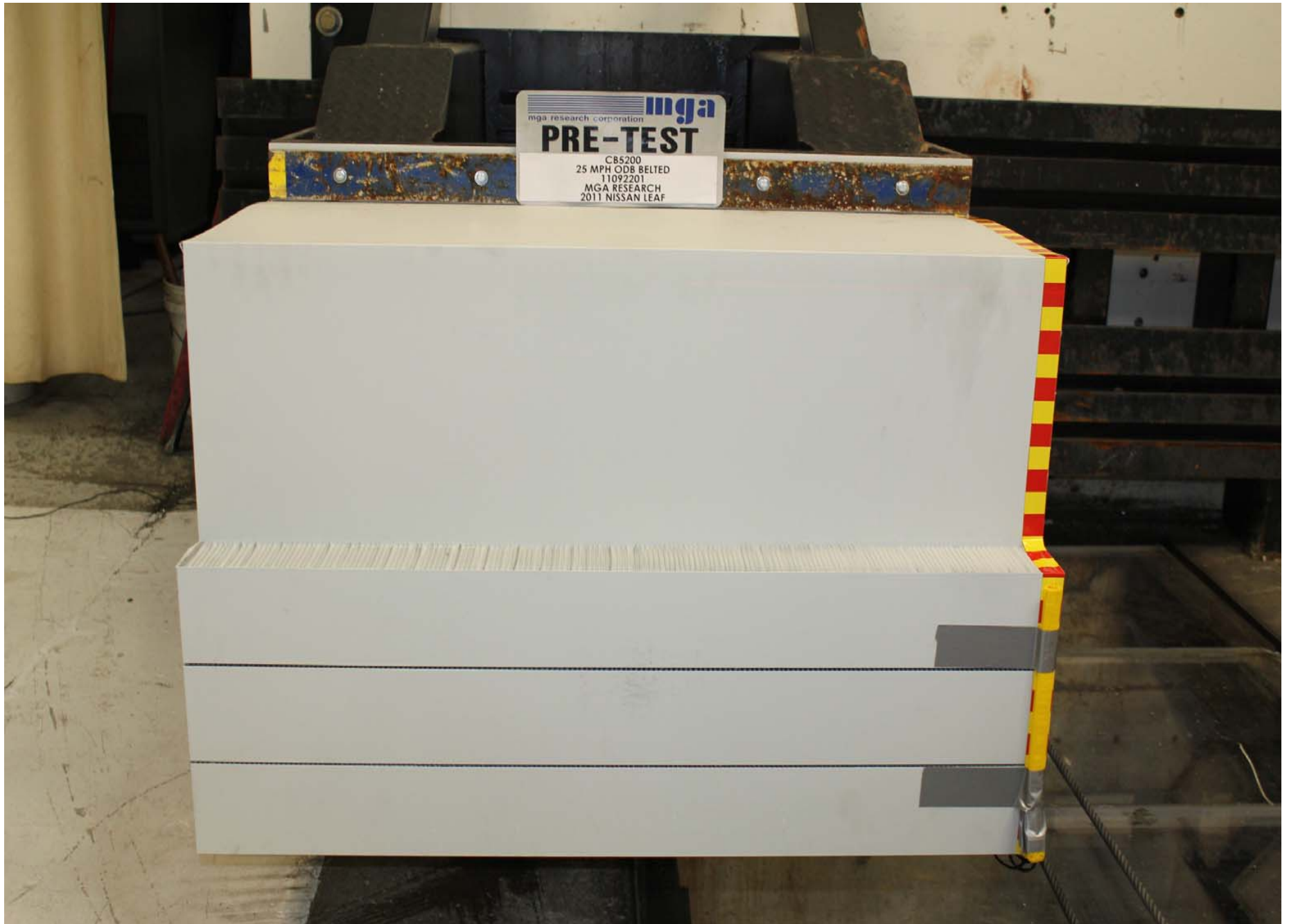
Pre-Test Offset Deformable Barrier Front View
