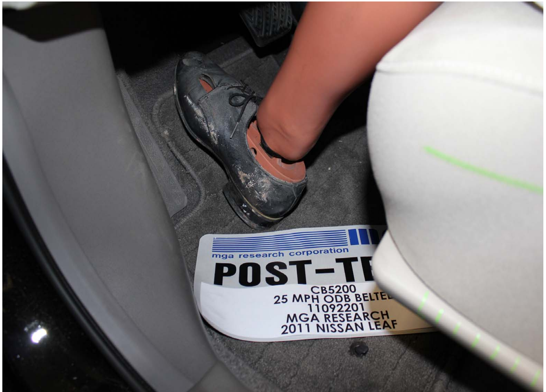
Post-Test Driver Dummy Feet Position
