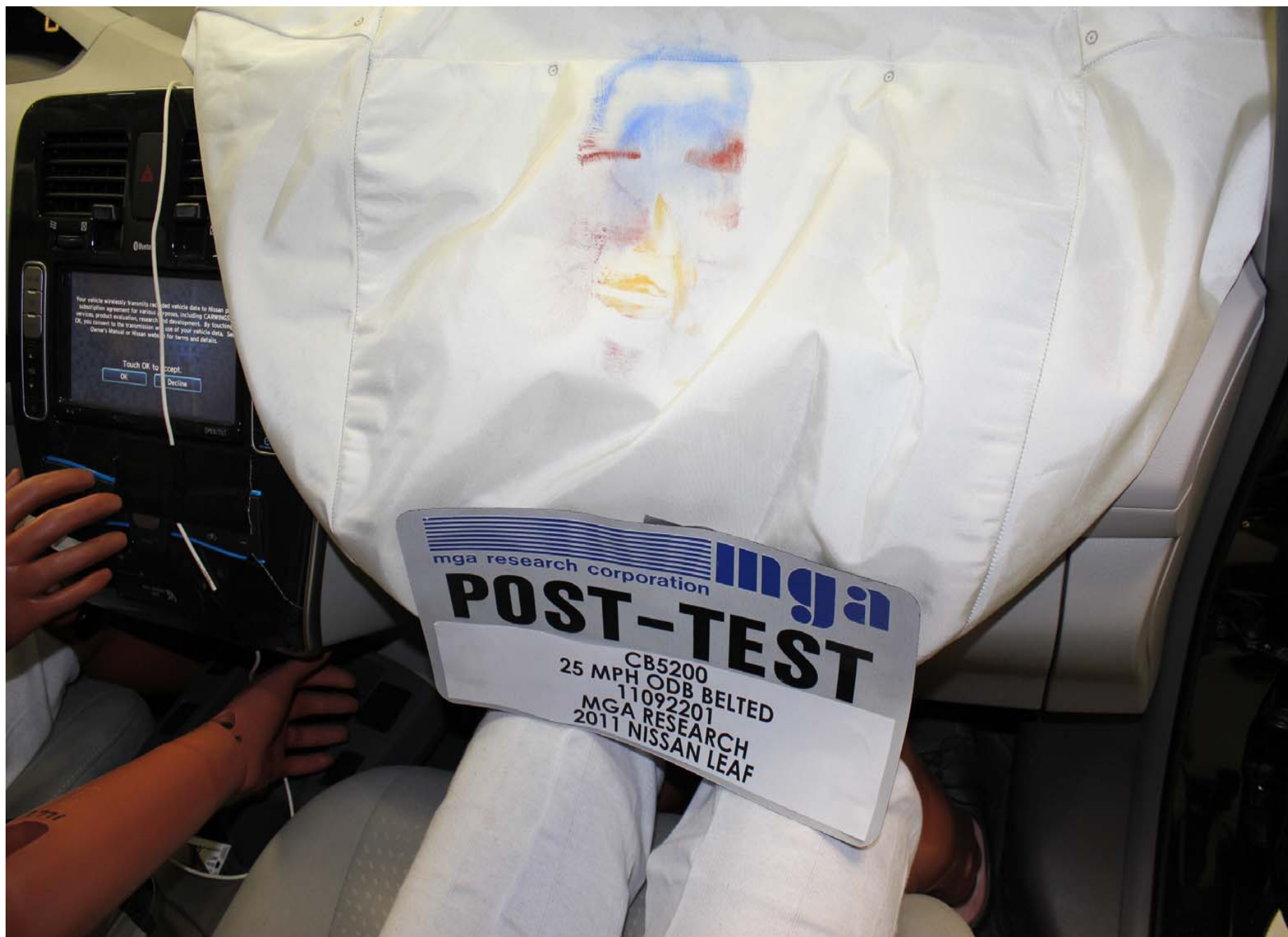
Post-Test Passenger Dummy Airbag Contact
