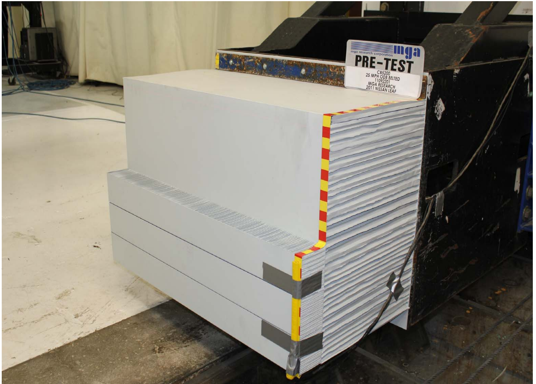
Pre-Test Left Front Three-Quarter View of Offset Deformable Barrier
