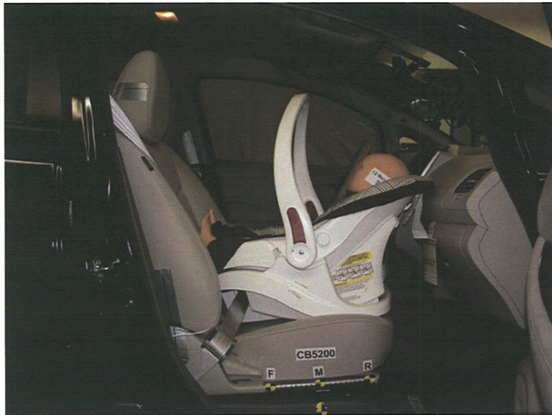
Cosco Arriva WBase, Belted, Rear Facing, Middle Seat Track
