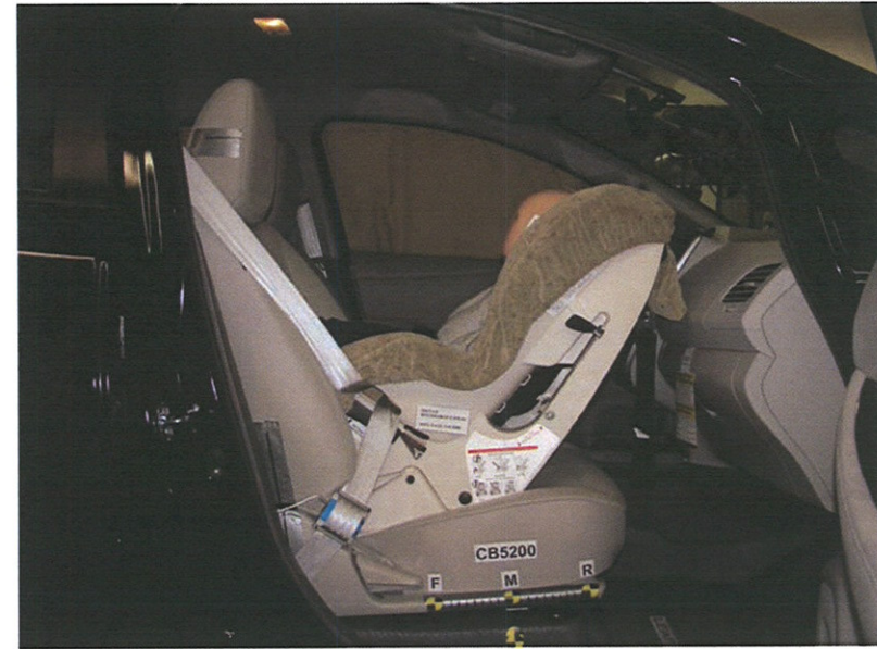
Britax Roundabout Rear Facing Belted, Middle Seat Track
