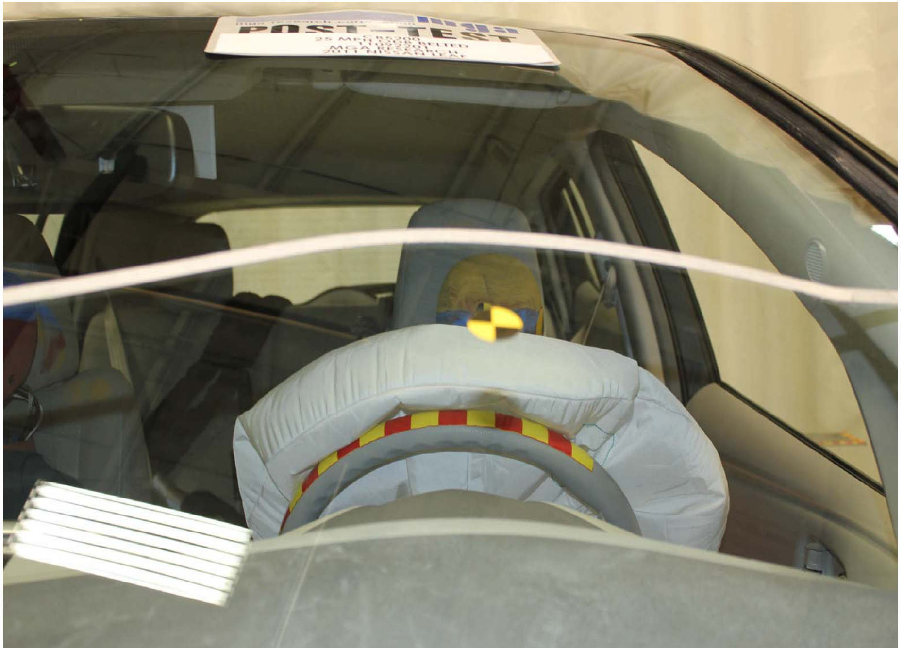
Post-Test Driver Dummy Front View (head position)
