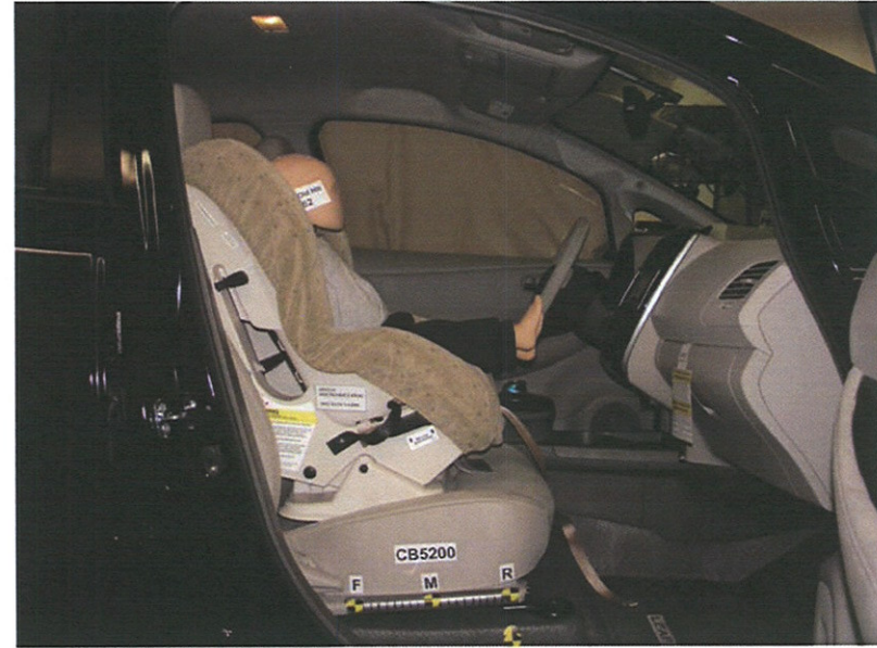
Britax Roundabout Forward Facing Unbelted, Rearward Seat Track
