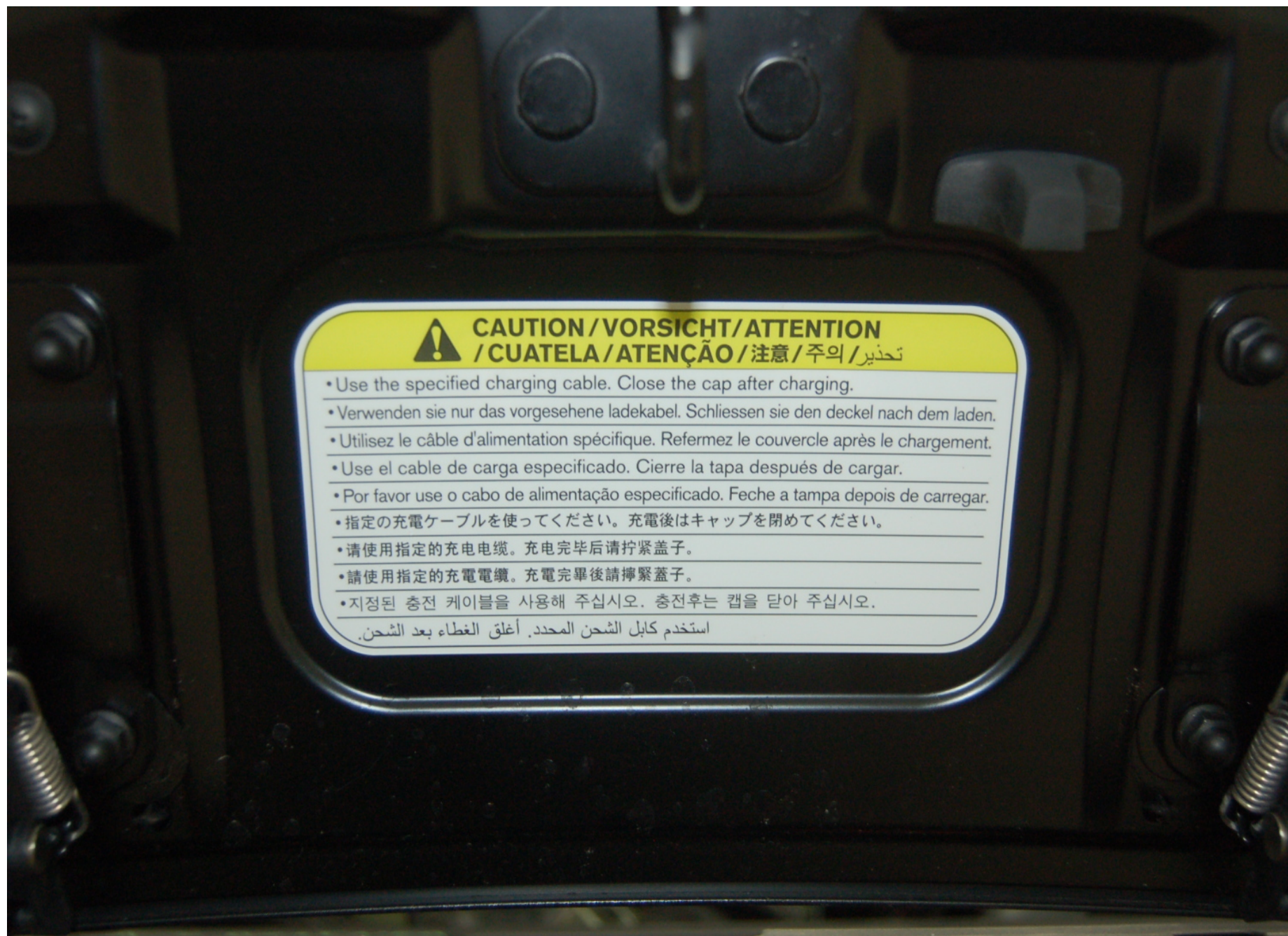
Auxiliary Power Module Warning Label
