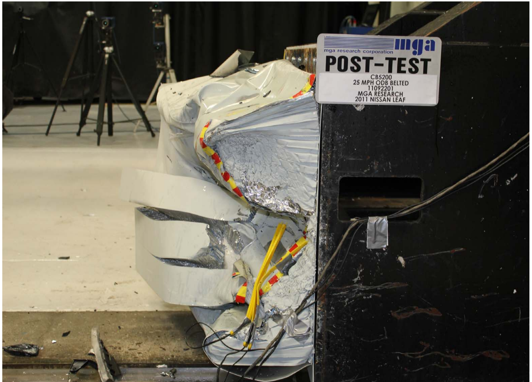
Post-Test Offset Deformable Barrier Left Side View
