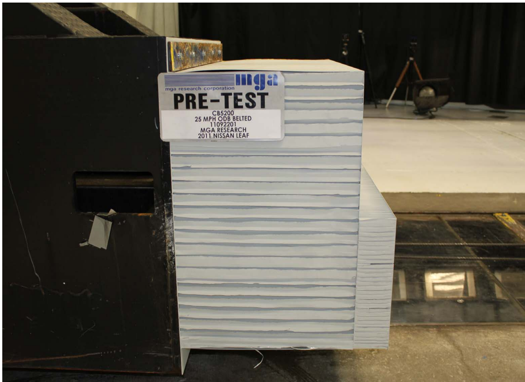
Pre-Test Offset Deformable Barrier Right Side View
