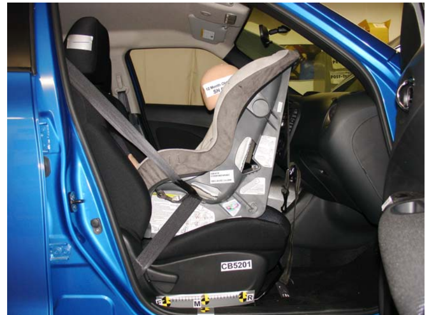
Graco Comfortsport Rear Facing Belted, Middle Seat Track
