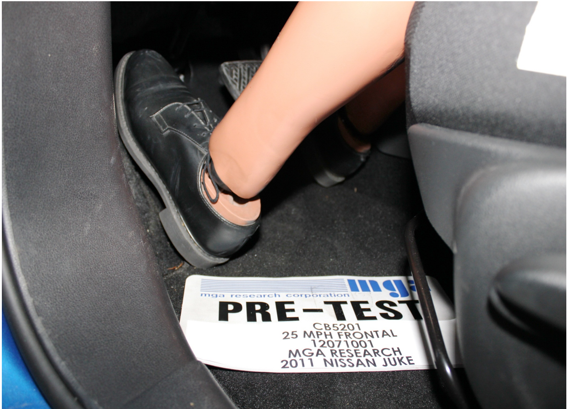
Pre-Test Driver Dummy Feet Position
