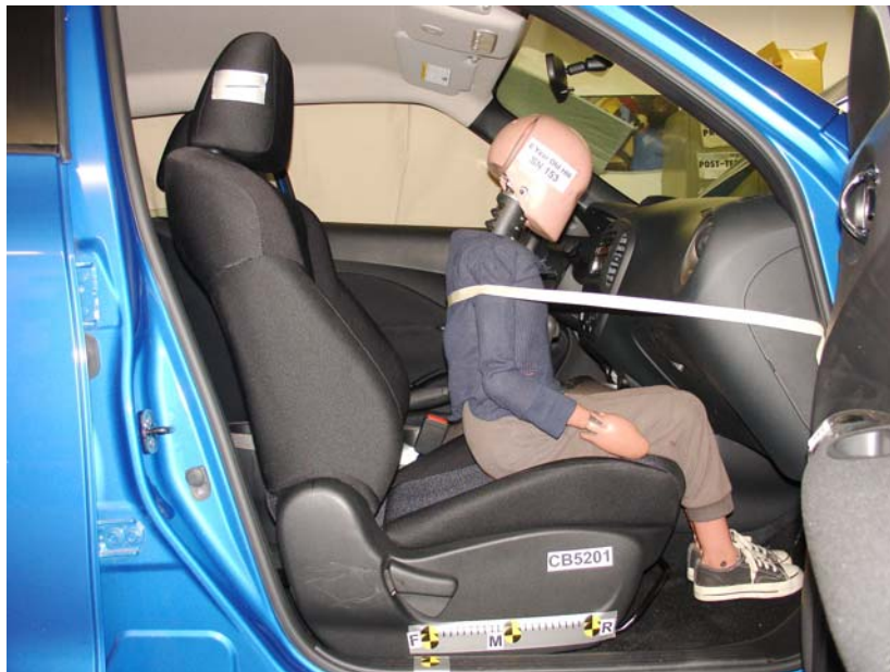
6-Year-Old Unbelted, Forward Seat Track, Position 3
