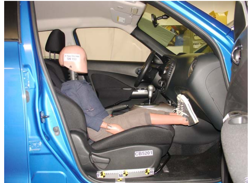
6-Year-Old Unbelted, Forward Seat Track, Position 2
