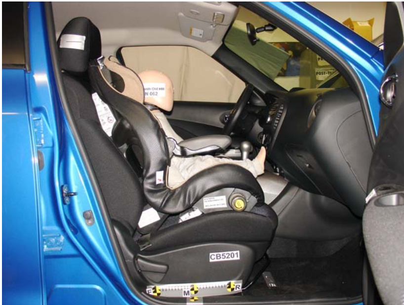
Evenflo Generations Forward Facing Unbelted, Middle Seat Track
