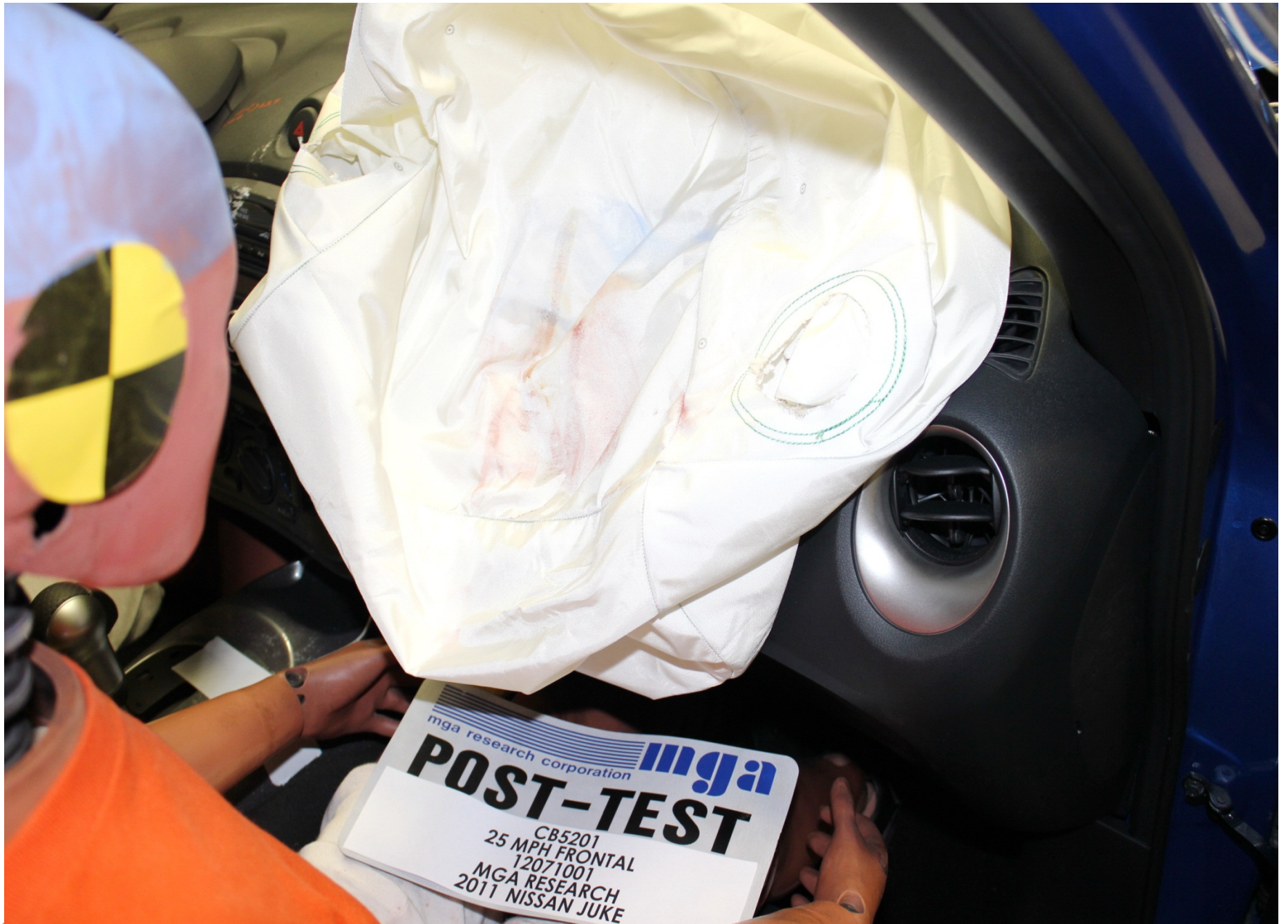
Post-Test Passenger Dummy Airbag Contact
