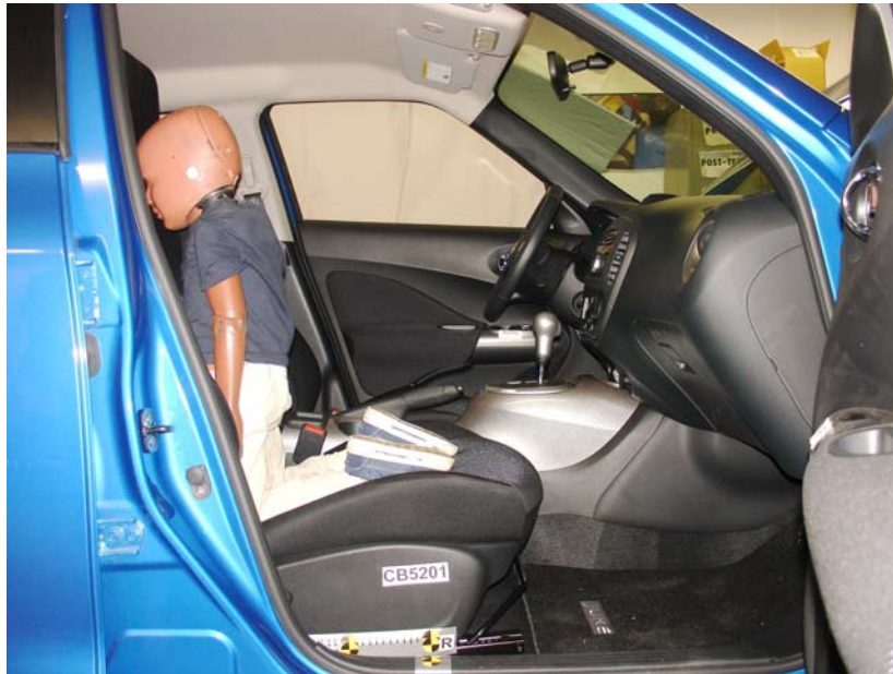
3-Year-Old Unbelted, Rearward Seat Track, Position 7
