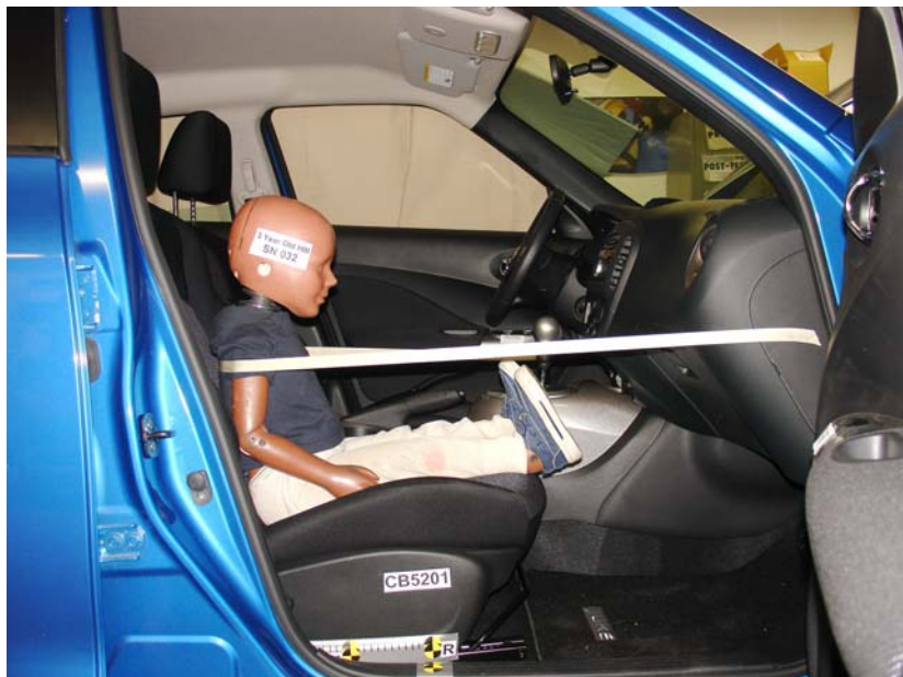
3-Year-Old Unbelted, Rearward Seat Track, Position 3
