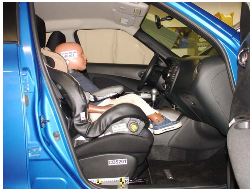
3-Year-Old Forward Facing Evenflo Generations Cinched With Harness, Rearward Seat Track
