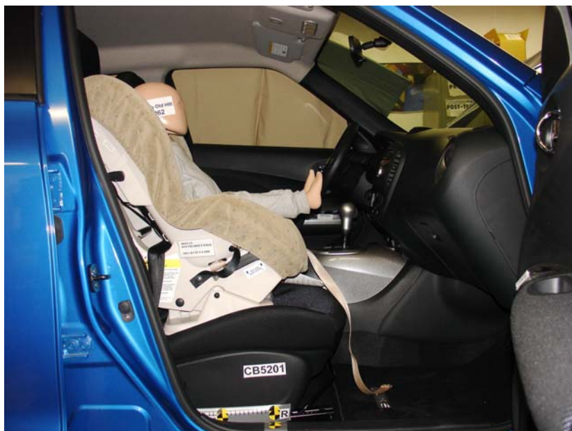
Britax Roundabout Forward Facing Belted, Rearward Seat Track
