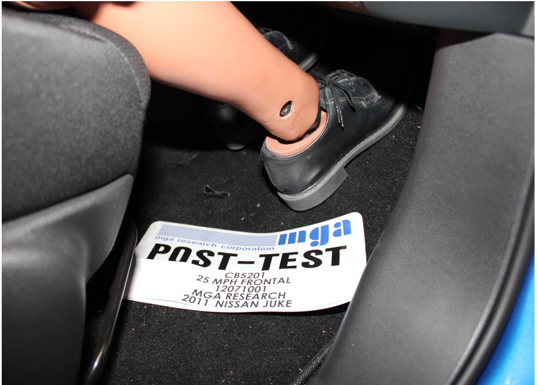
Post-Test Passenger Dummy Feet Position
