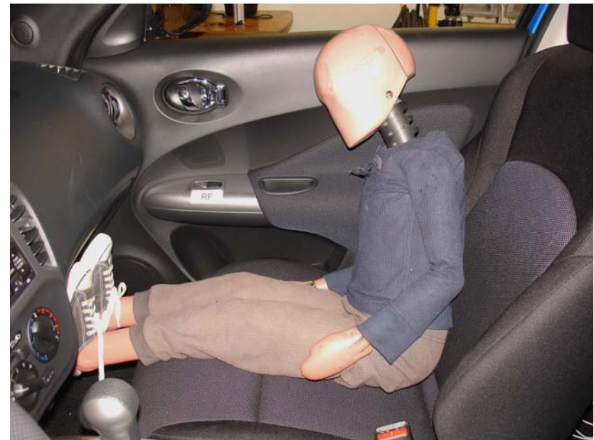
6-Year-Old Unbelted, Forward Seat Track, Position 4
