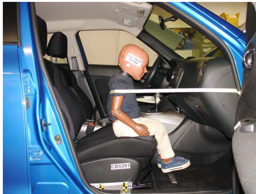
3-Year-Old Unbelted, Rearward Seat Track, Position 4
