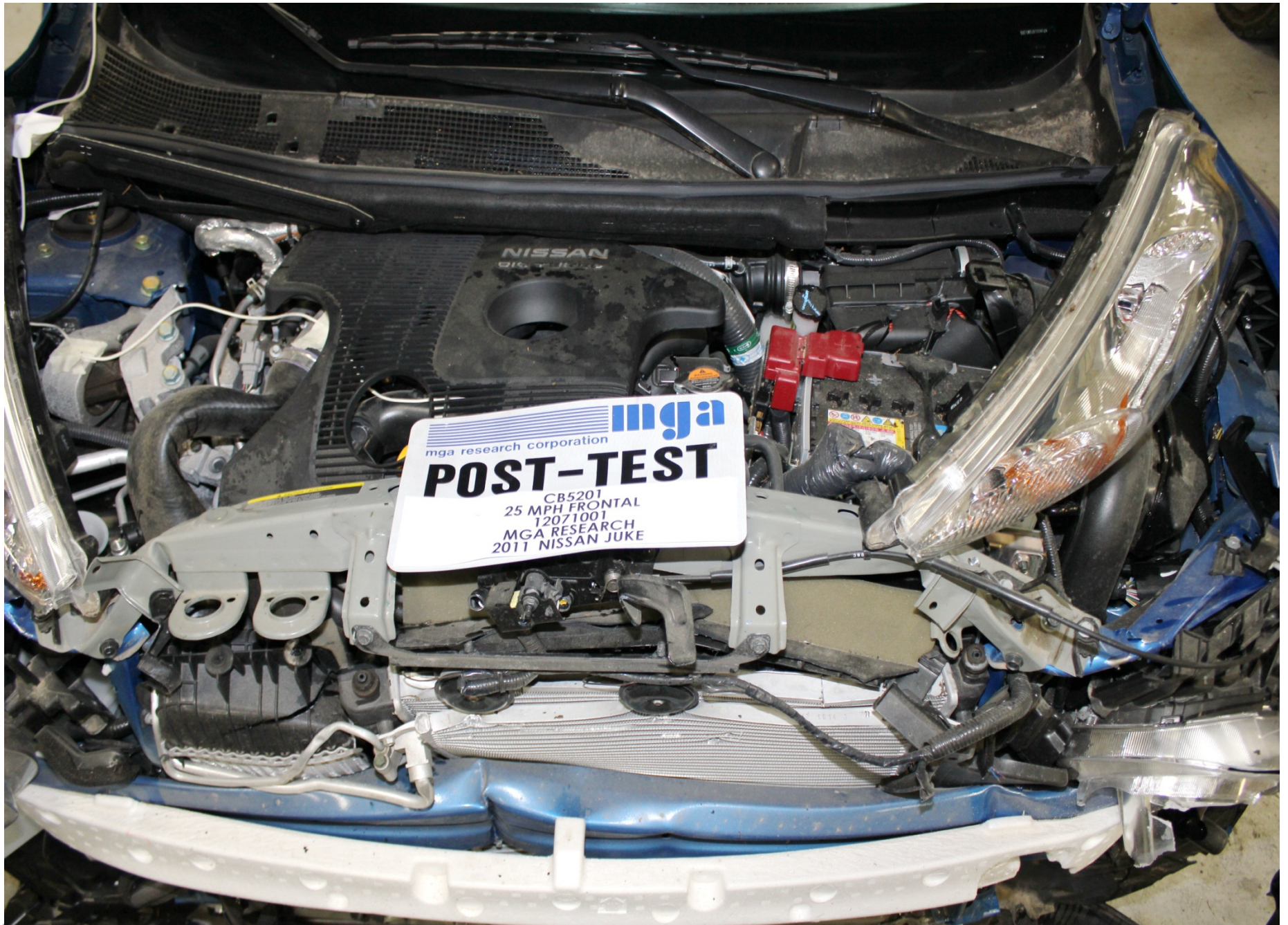
Post-Test Engine Compartment View
