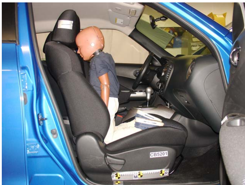
3-Year-Old Unbelted, Forward Seat Track, Position 7
