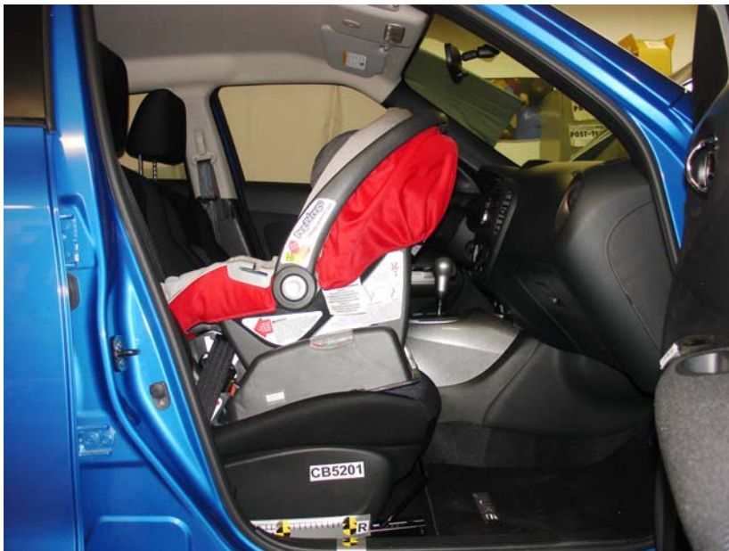
Peg Perego Viaggio WBase, Belted, Rear Facing, Rearward Seat Track
