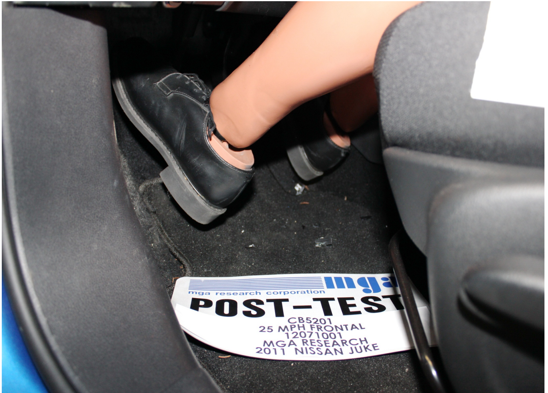
Post-Test Driver Dummy Feet Position
