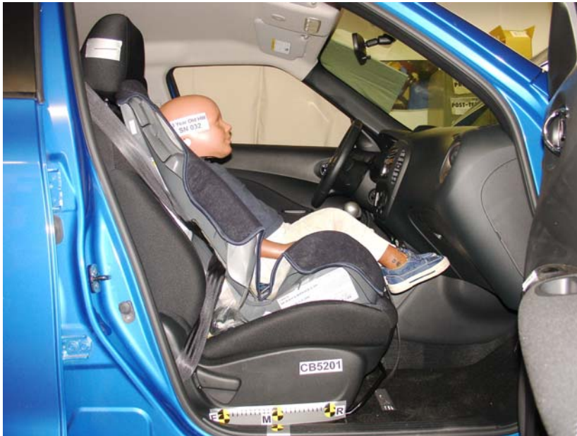
3-Year-Old Forward Facing Cosco High Back Booster Cinched With Harness, Middle Seat Track 3-Year-Old Forward Facing Cosco High Back Booster Cinched With Harness, Rearward Seat Track
