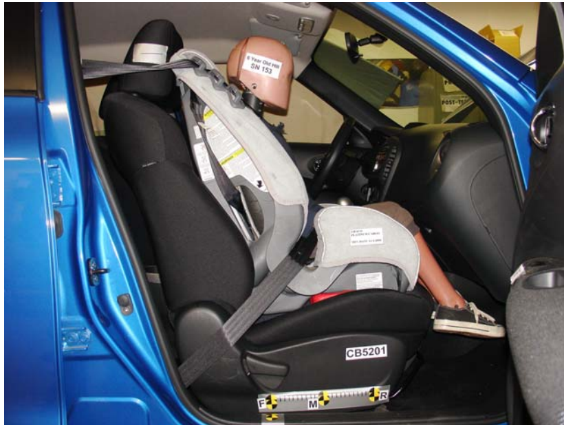
6-Year-Old Graco Platinum Cargo Belted, Forward Seat Track
