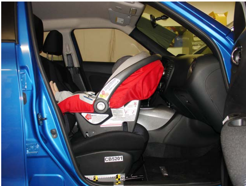
Peg Perego Viaggio WOut Base, Unbelted, Rear Facing, Rearward Seat Track
