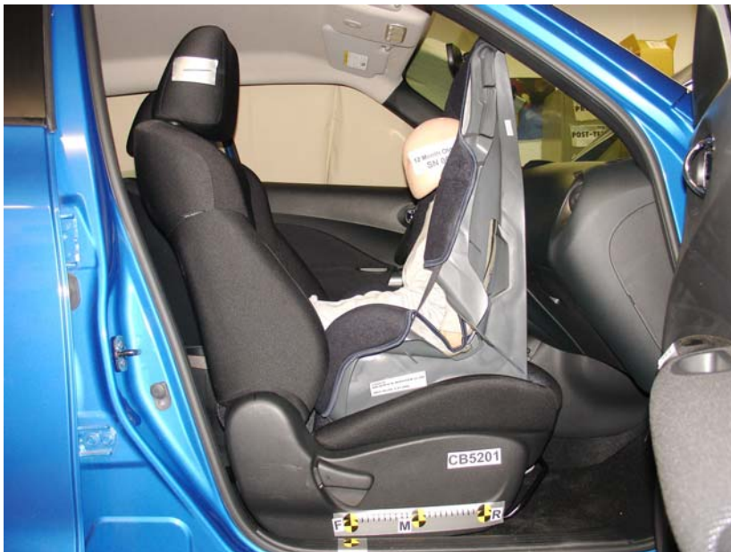
Cosco High Back Booster Rear Facing Unbelted, Forward Seat Track
