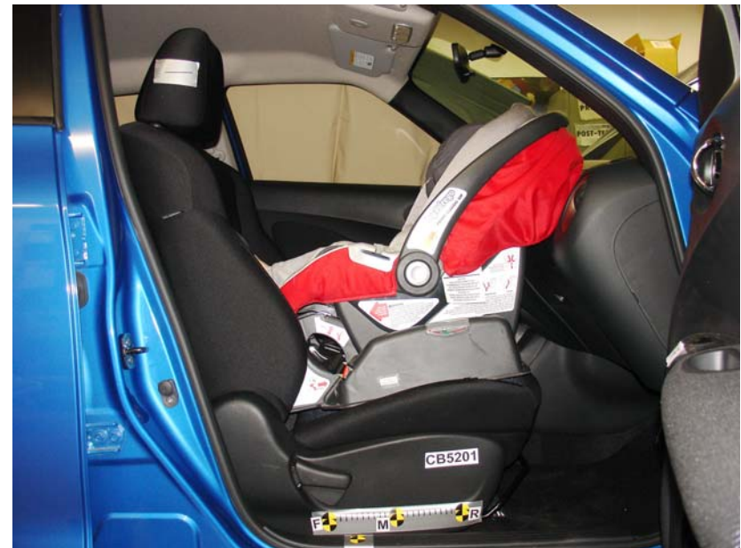
Peg Perego Viaggio WBase, Unbelted, Rear Facing, Forward Seat Track
