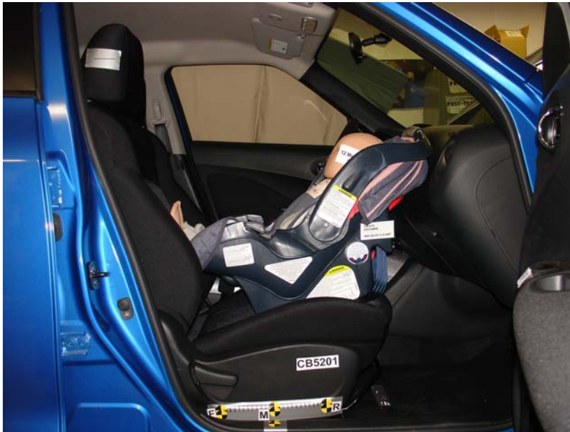
Graco Snugride WOut Base, Unbelted, Rear Facing, Middle Seat Track
