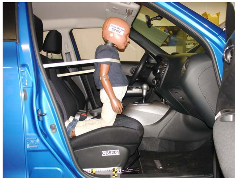
3-Year-Old Unbelted, Rearward Seat Track, Position 6
