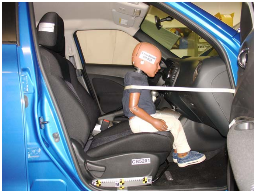
3-Year-Old Unbelted, Middle Seat Track, Position 4
