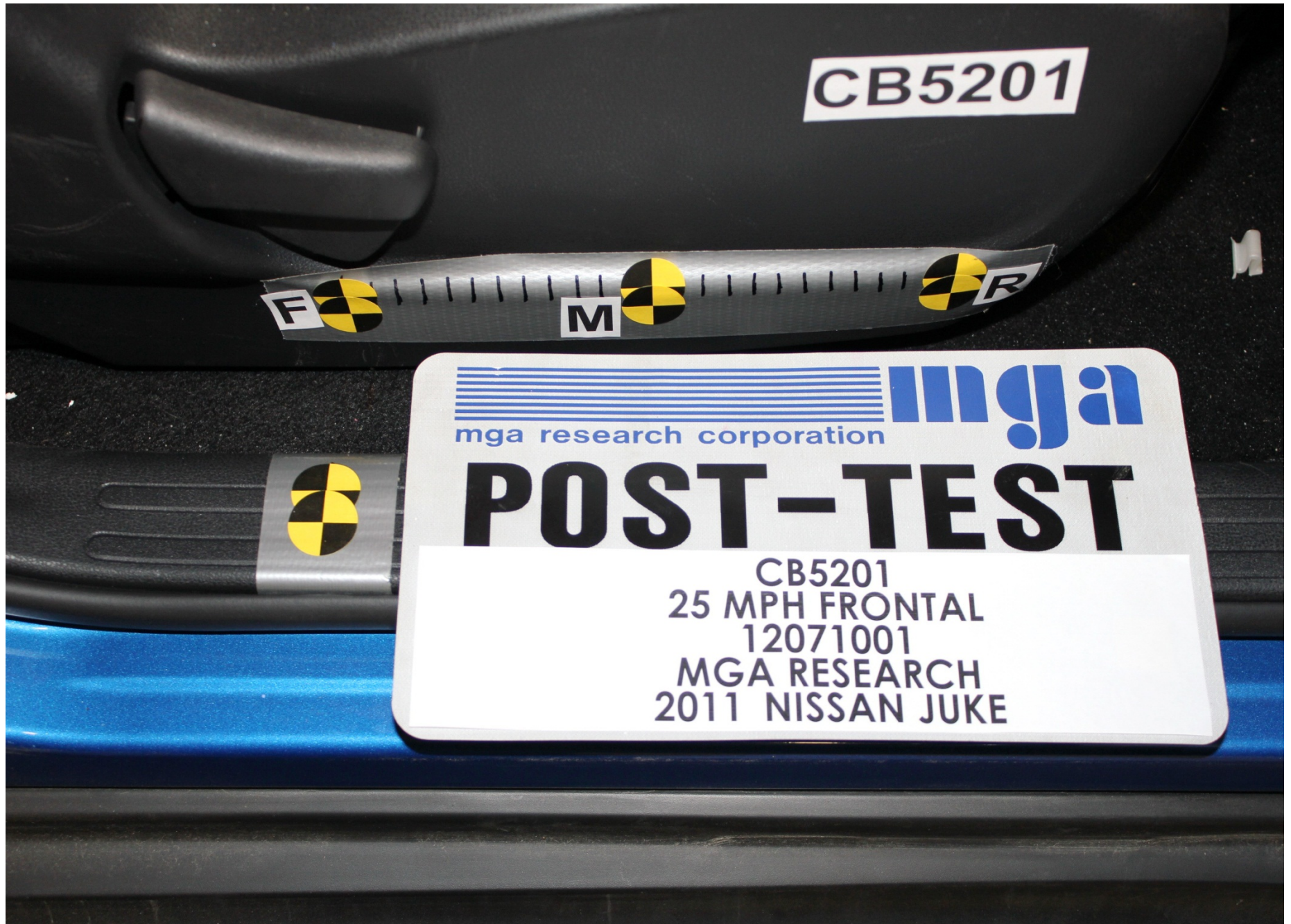
Post-Test Passenger Dummy Seat Position
