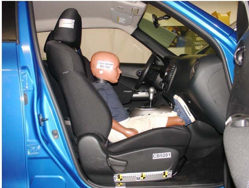
3-Year-Old Unbelted, Forward Seat Track, Position 1
