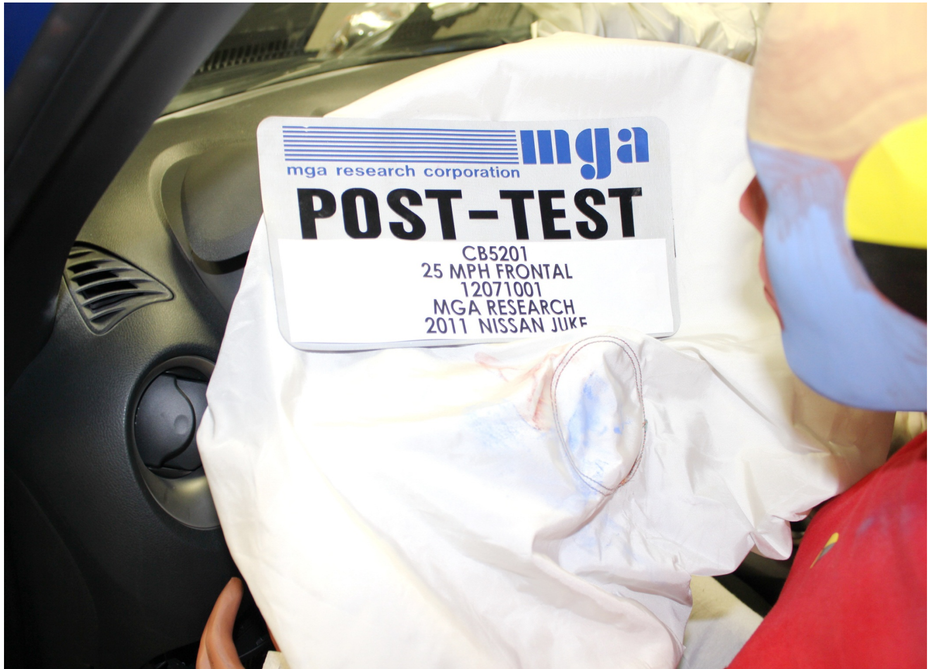
Post-Test Driver Dummy Airbag Contact
