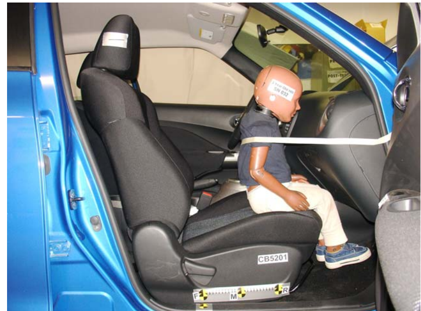
3-Year-Old Unbelted, Forward Seat Track, Position 4
