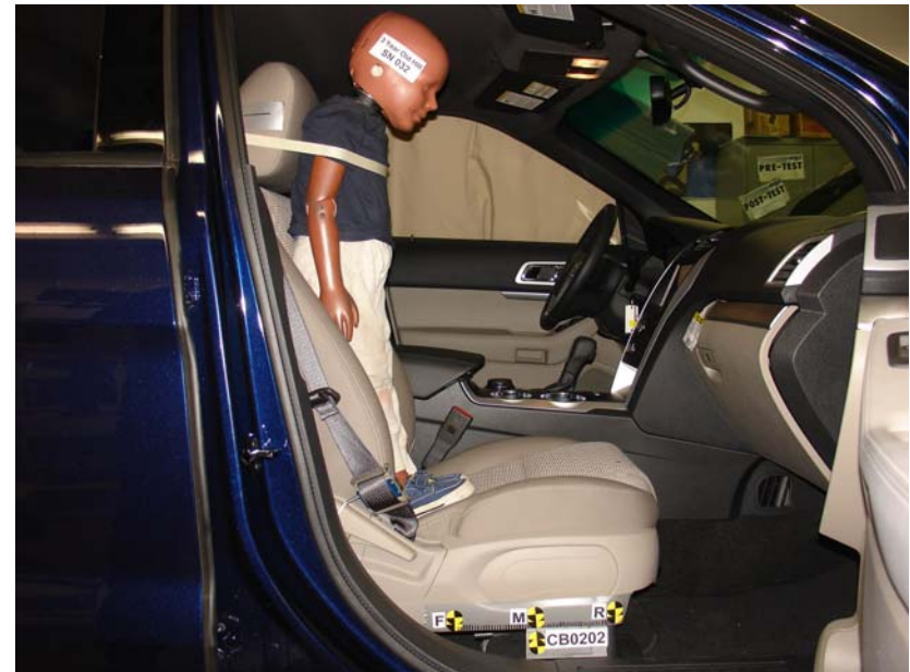
3-Year-Old Unbelted, Middle Seat Track, Position 5
