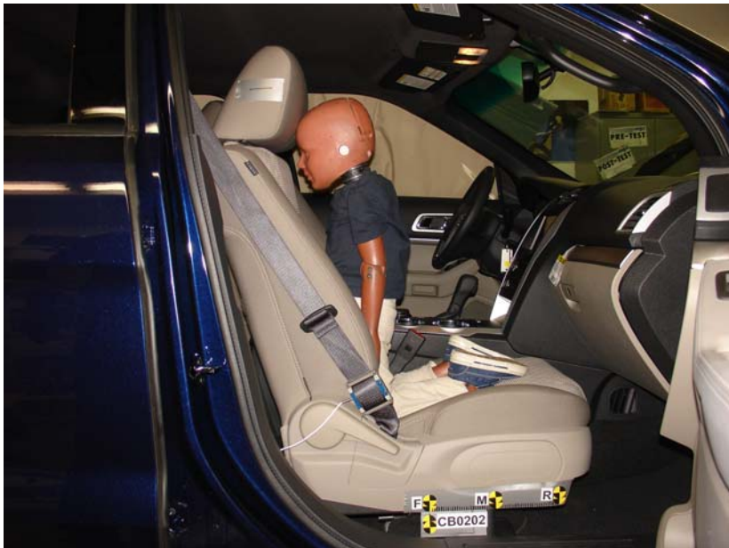
3-Year-Old Unbelted, Forward Seat Track, Position 7
