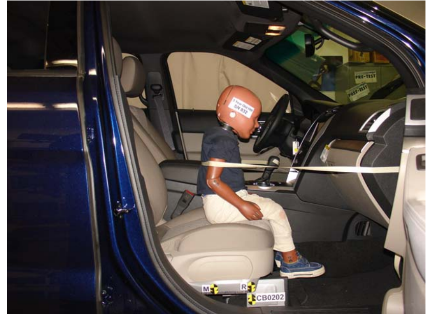
3-Year-Old Unbelted, Rearward Seat Track, Position 4
