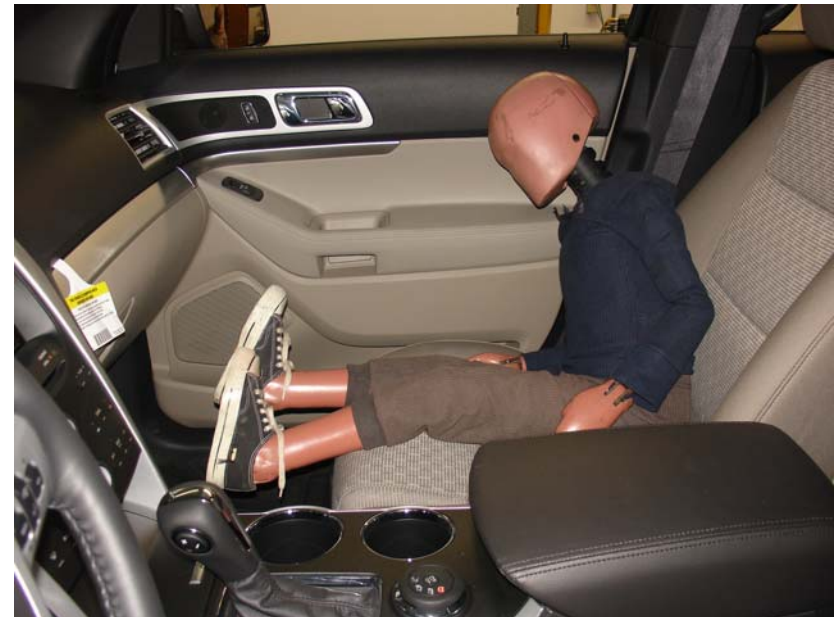
6-Year-Old Unbelted, Rearward Seat Track, Position 4
