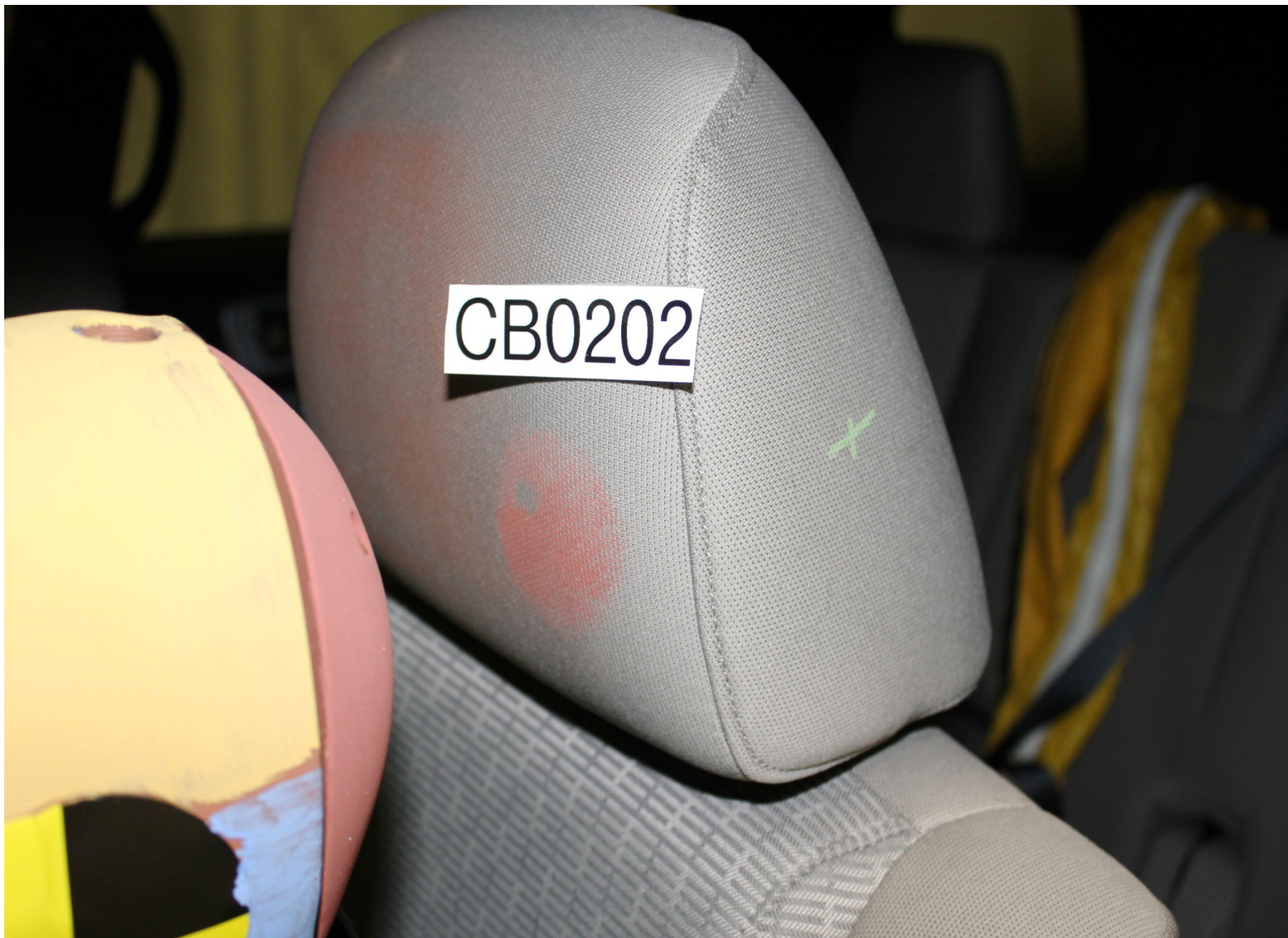
Post-Test Driver Dummy Head Contact (headrest)
