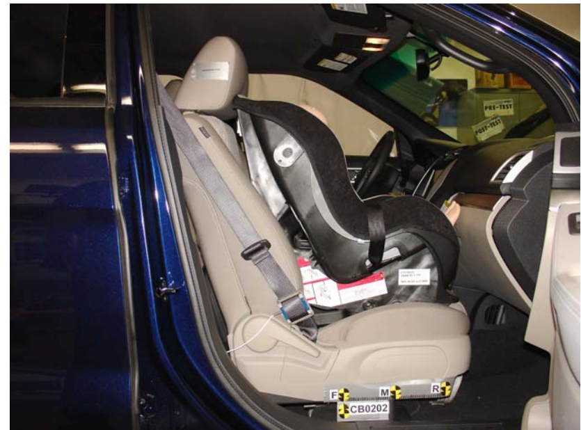
Evenflo Tribute Forward Facing Unbelted, Forward Seat Track
