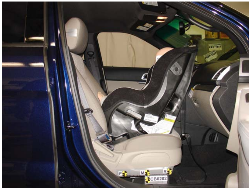
Evenflo Tribute Rear Facing Unbelted, Middle Seat Track
