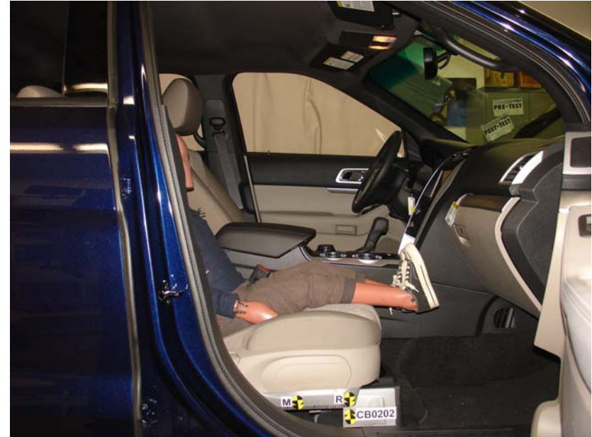
6-Year-Old Unbelted, Rearward Seat Track, Position 2
