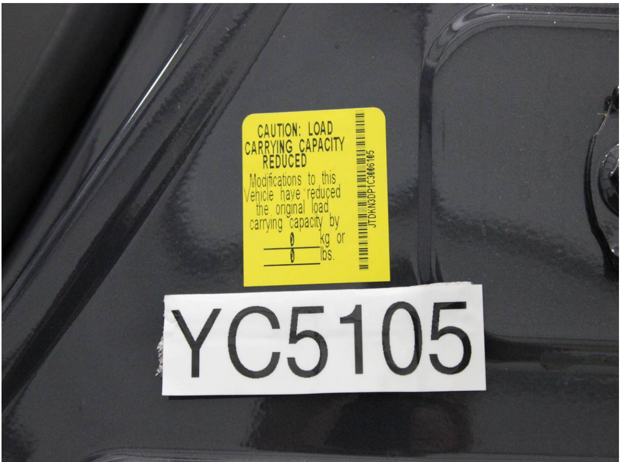
Load Carrying Capacity Reduced Label
