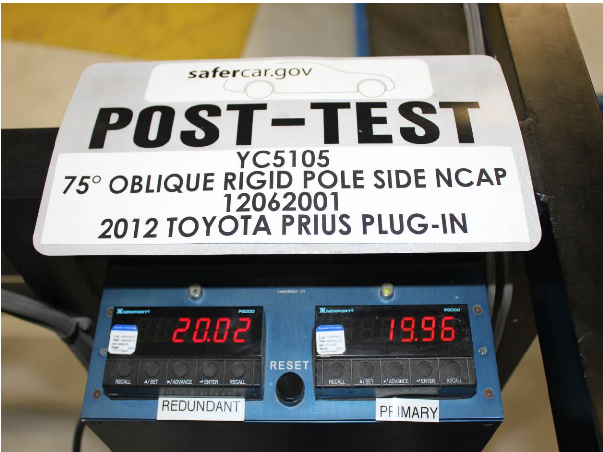
Post-Test Primary and Redundant Speed Trap Read-Out
