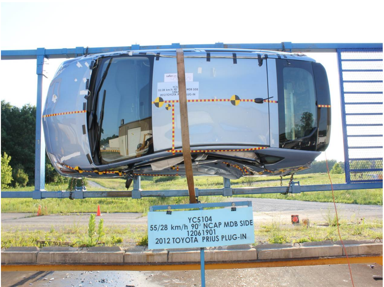
FMVSS No. 301 Static Rollover 90 Degrees
