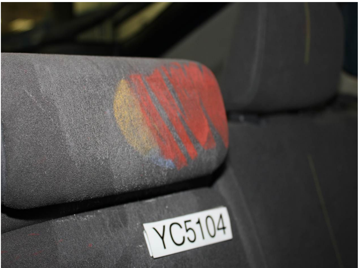
Post-Test Rear Passenger Dummy Close-up Head Contact with Vehicle Interior View
