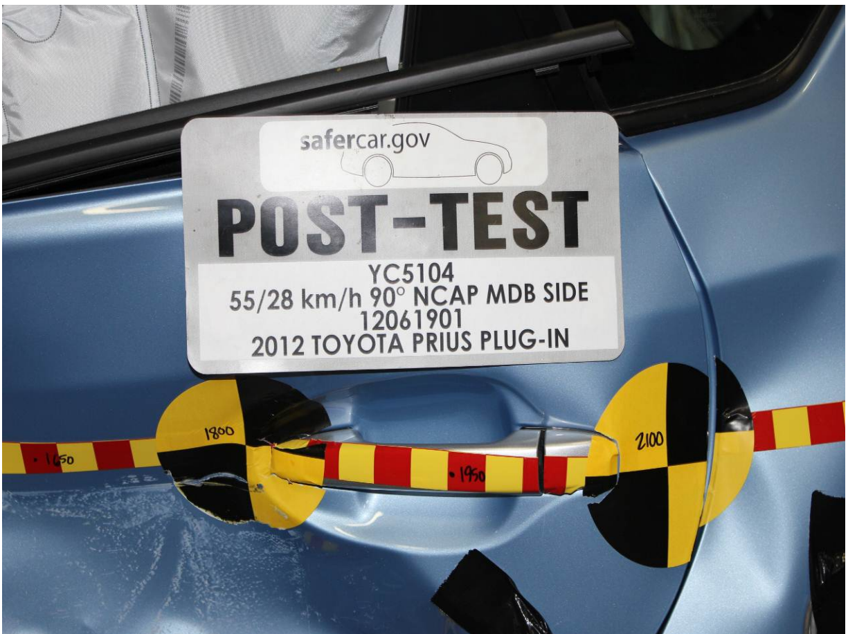
Post-Test Left Rear Door Latch Close-Up
