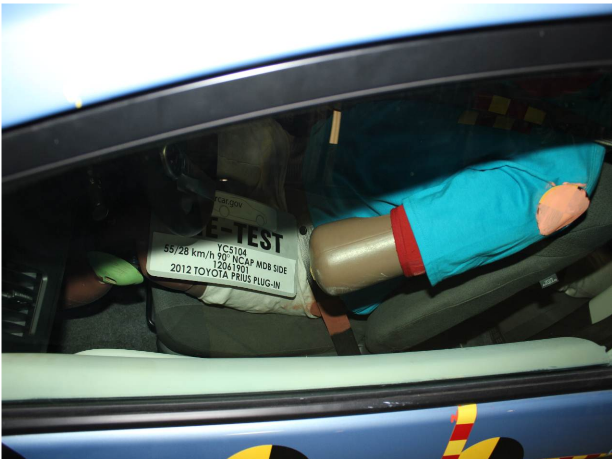
Pre-Test Driver Dummy and Door Clearance View
