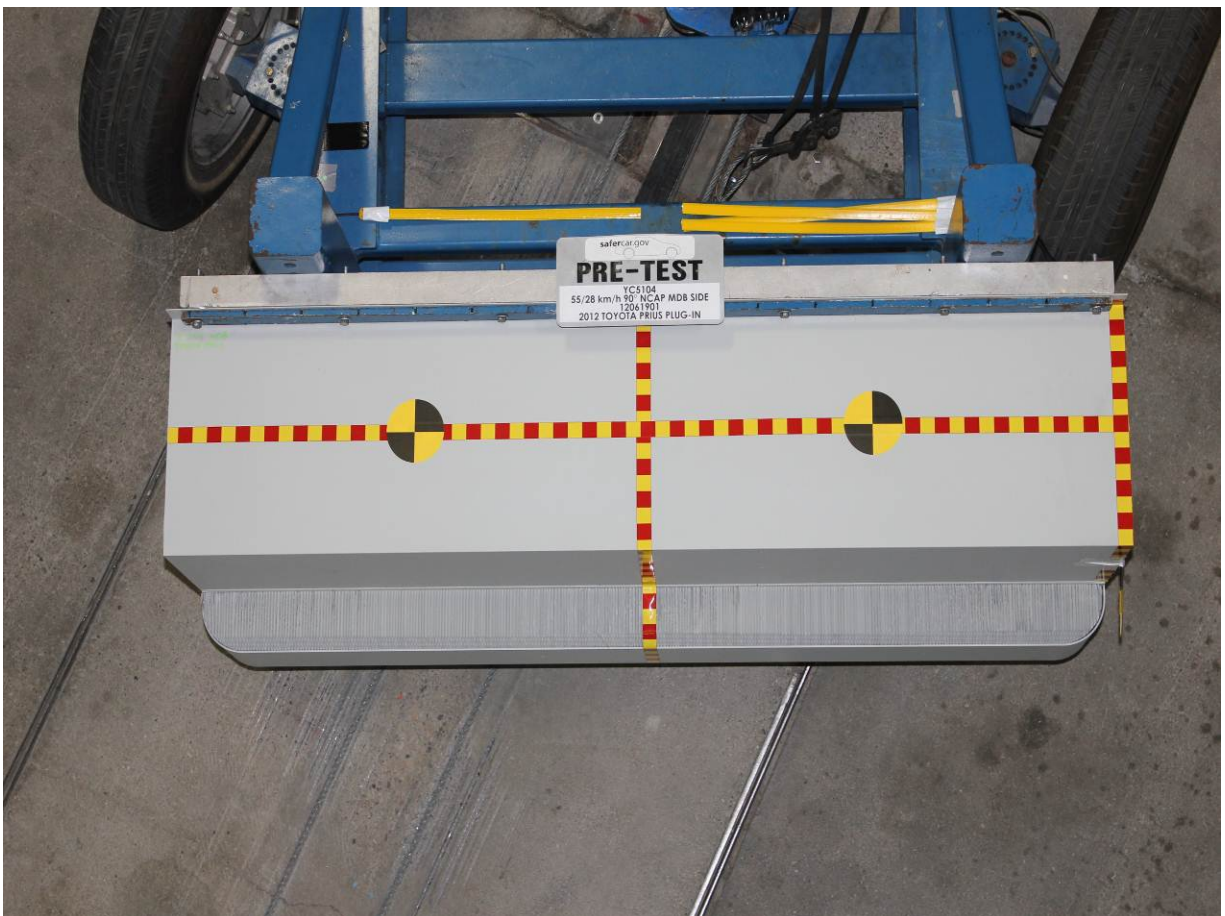
Pre-Test Top View of MDB Impactor Face
