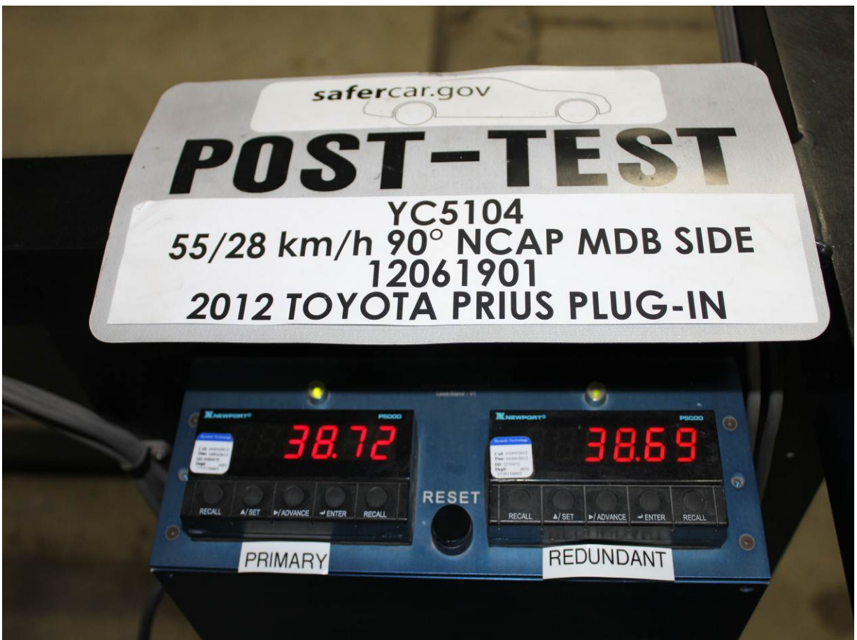
Post-Test Primary and Redundant Speed Trap Read-Out
