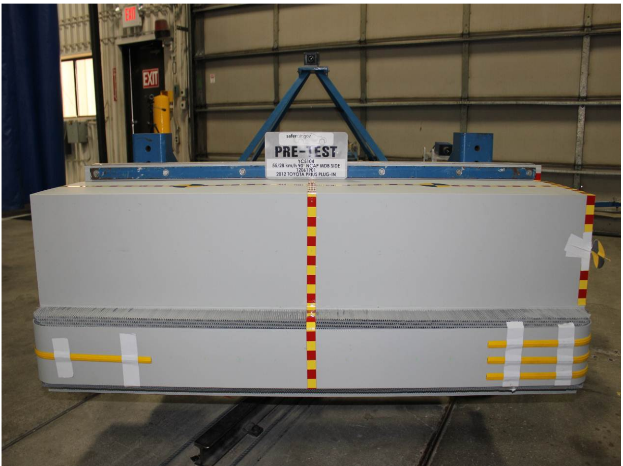
Pre-Test Front View of MDB Impactor Face
