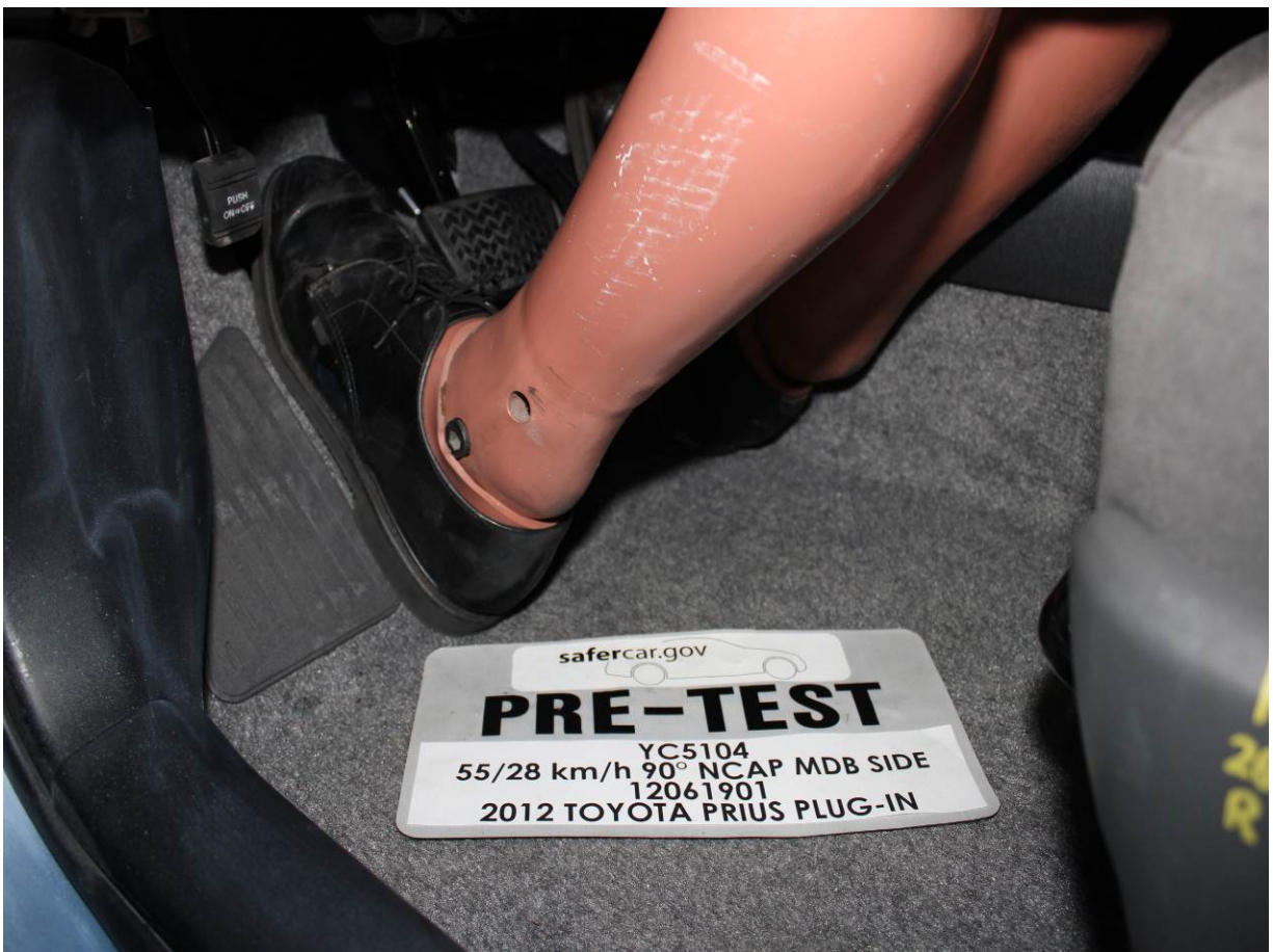
Pre-Test Placement of Driver Dummy's Feet
