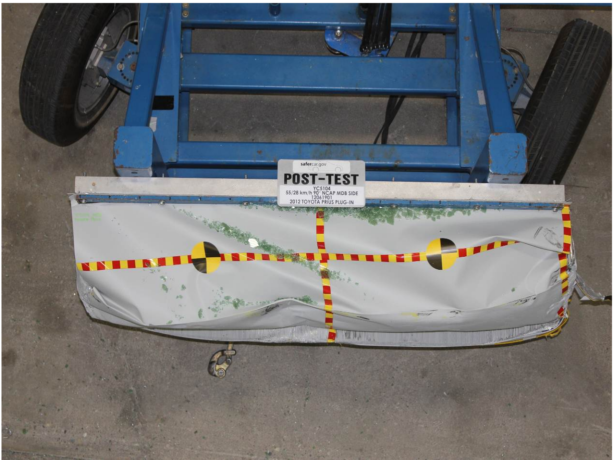
Post-Test Top View of MDB Impactor Face
