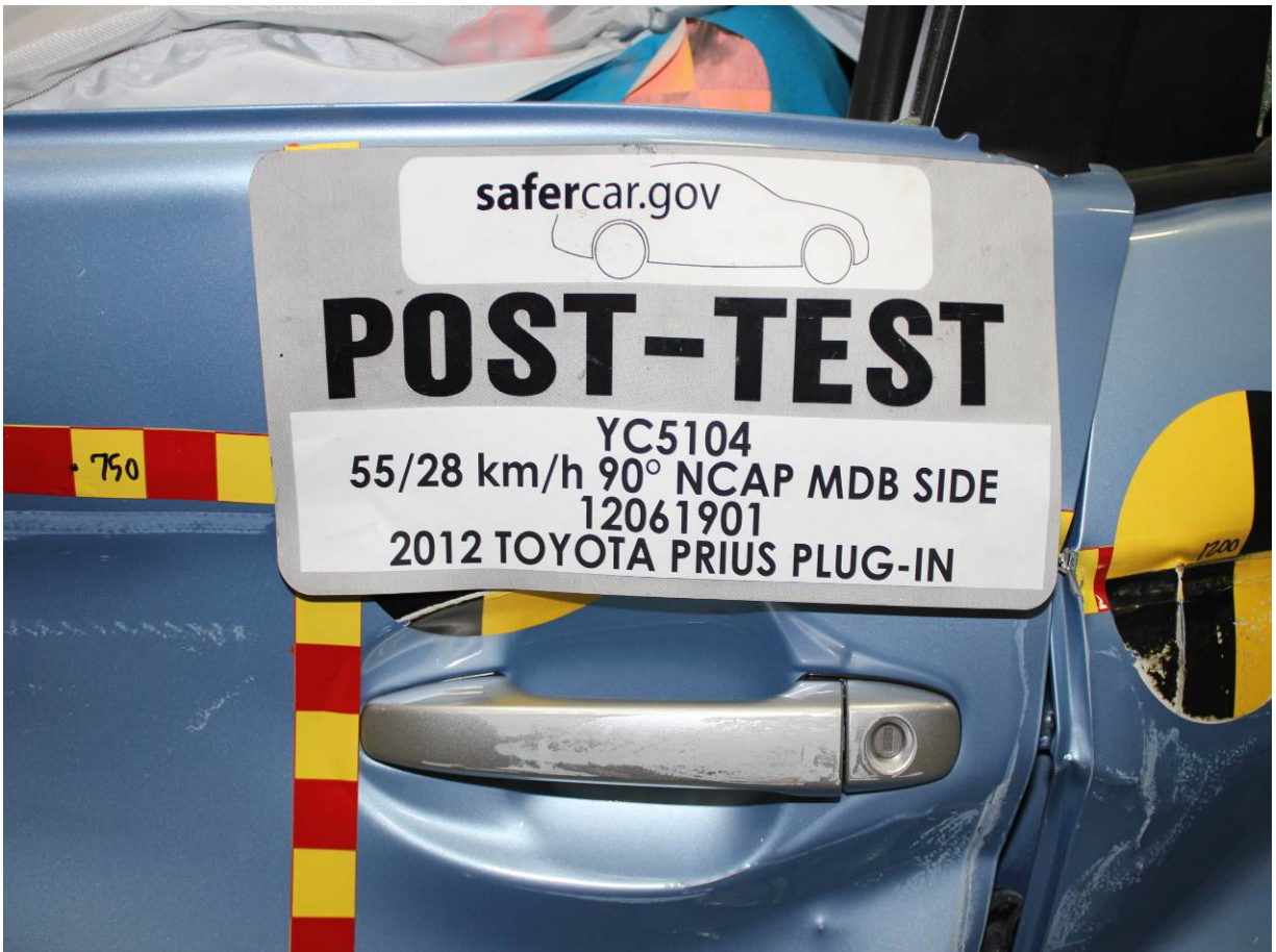
Post-Test Left Front Door Latch Close-Up
