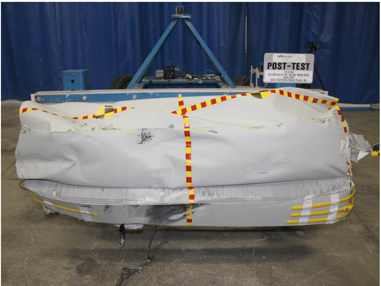
Post-Test Front View of MDB Impactor Face
