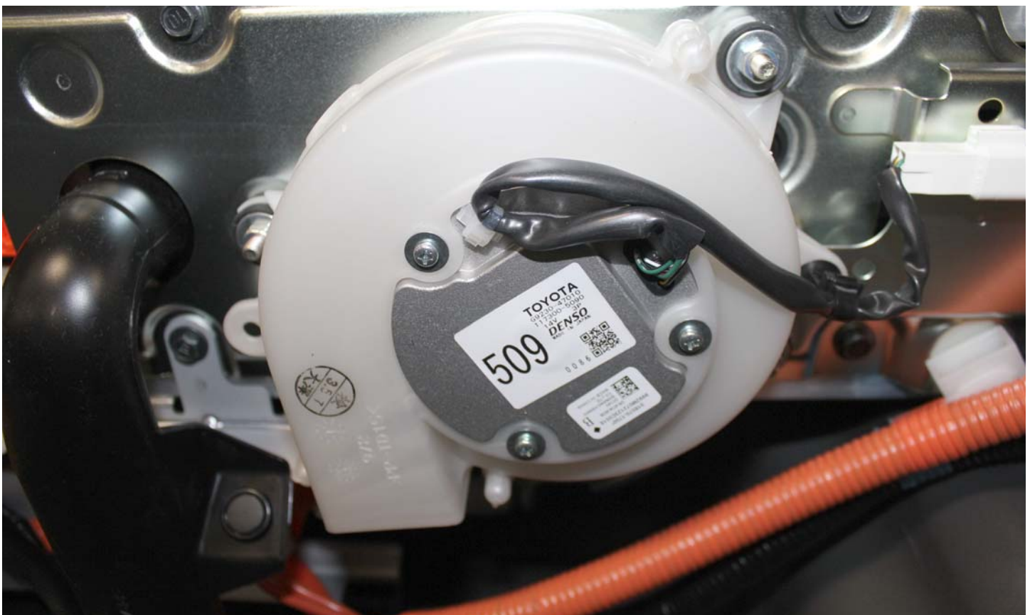
No. 019a Pre-Impact View Propulsion Battery Venting System(s)
