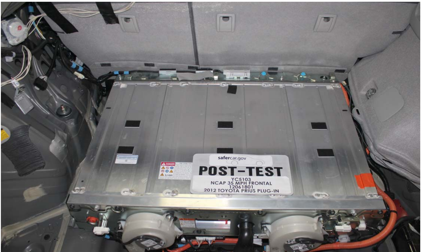
No. 010 Post-Impact Front View of Propulsion Battery
