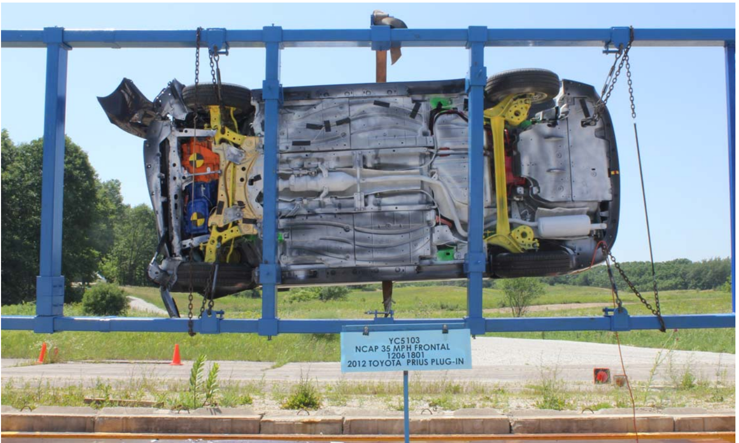
No. 030 FMVSS No. 305 Static Rollover at 270°
