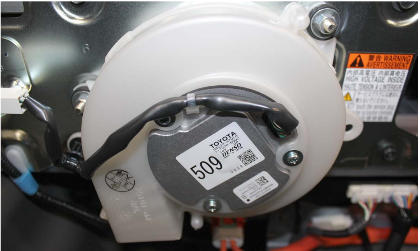
No. 019 Pre-Impact View Propulsion Battery Venting System(s)
