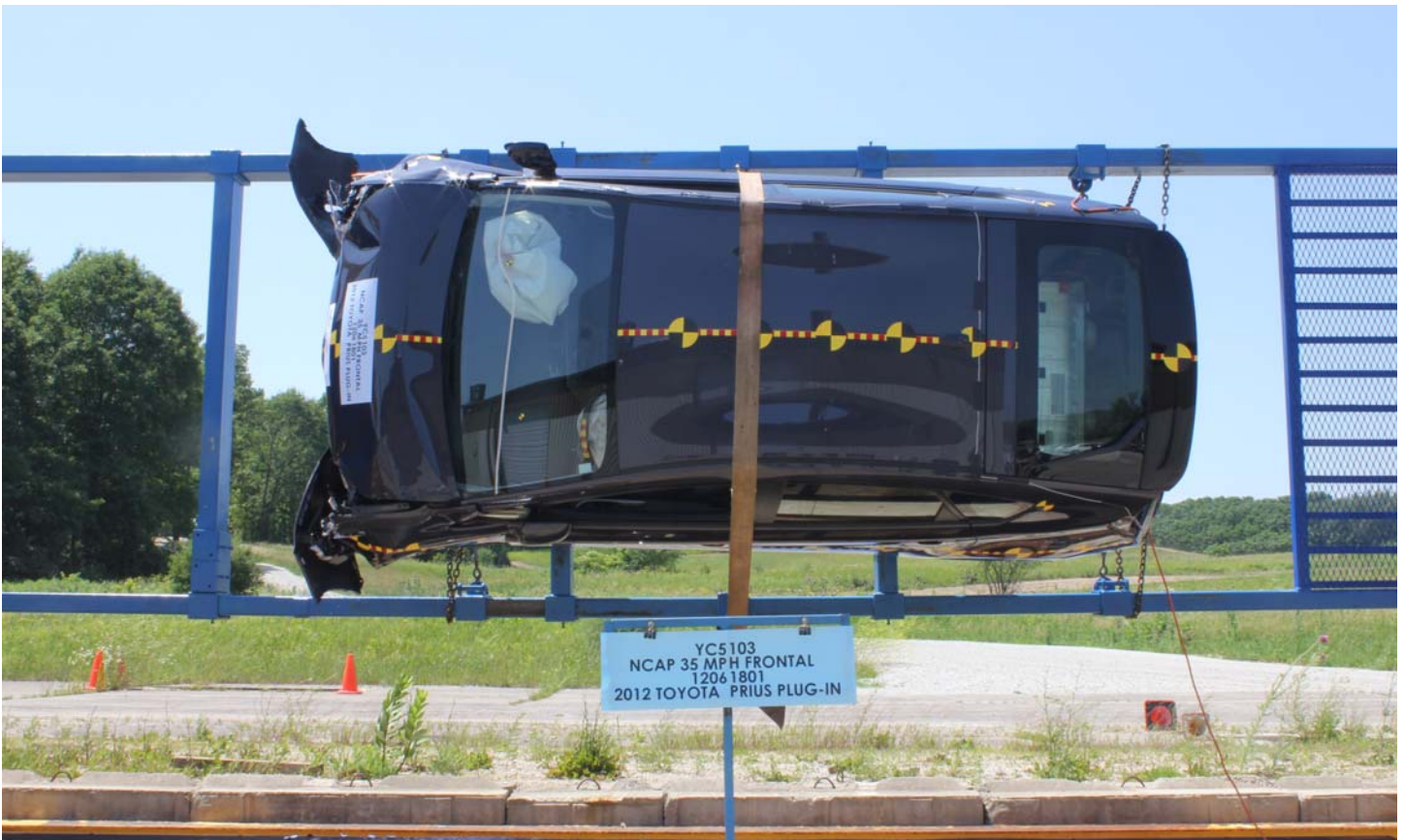
No. 028 FMVSS No. 305 Static Rollover at 90°
