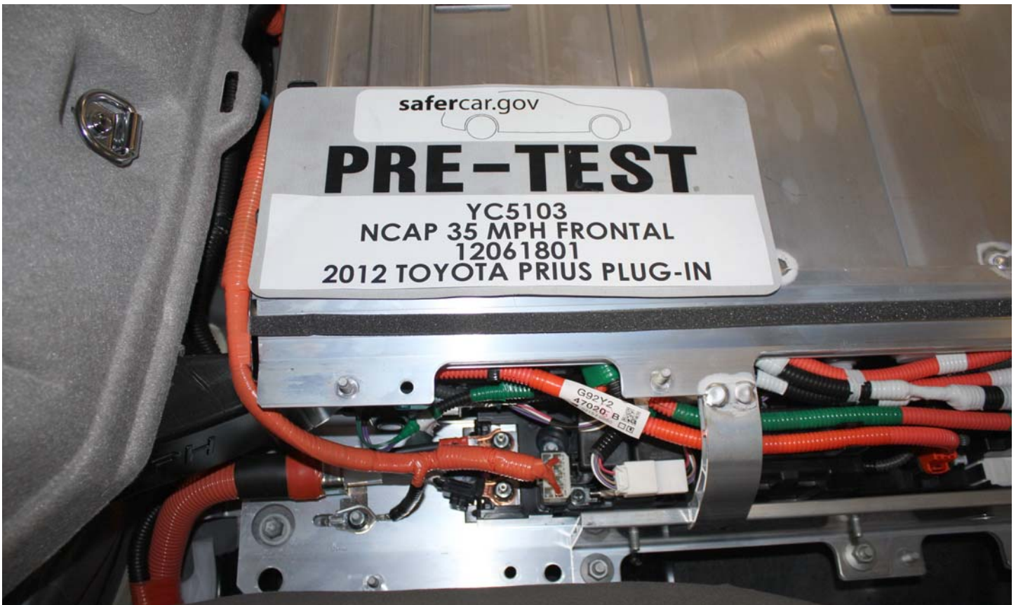
No. 018 Pre-Impact View of High Voltage Interconnect(s)
