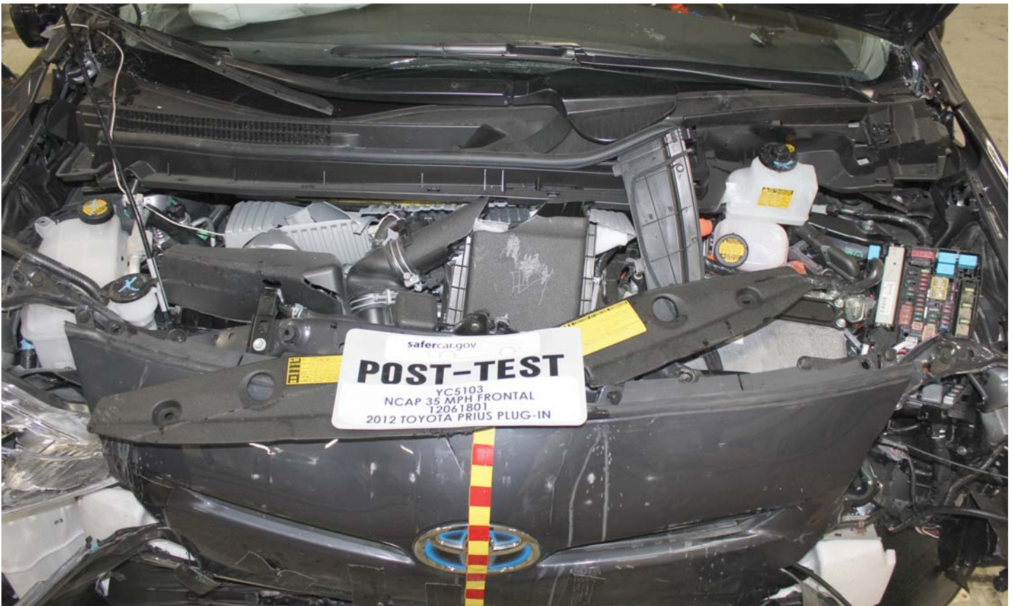
No. 017 Post-Impact View of Electric Propulsion Drive
