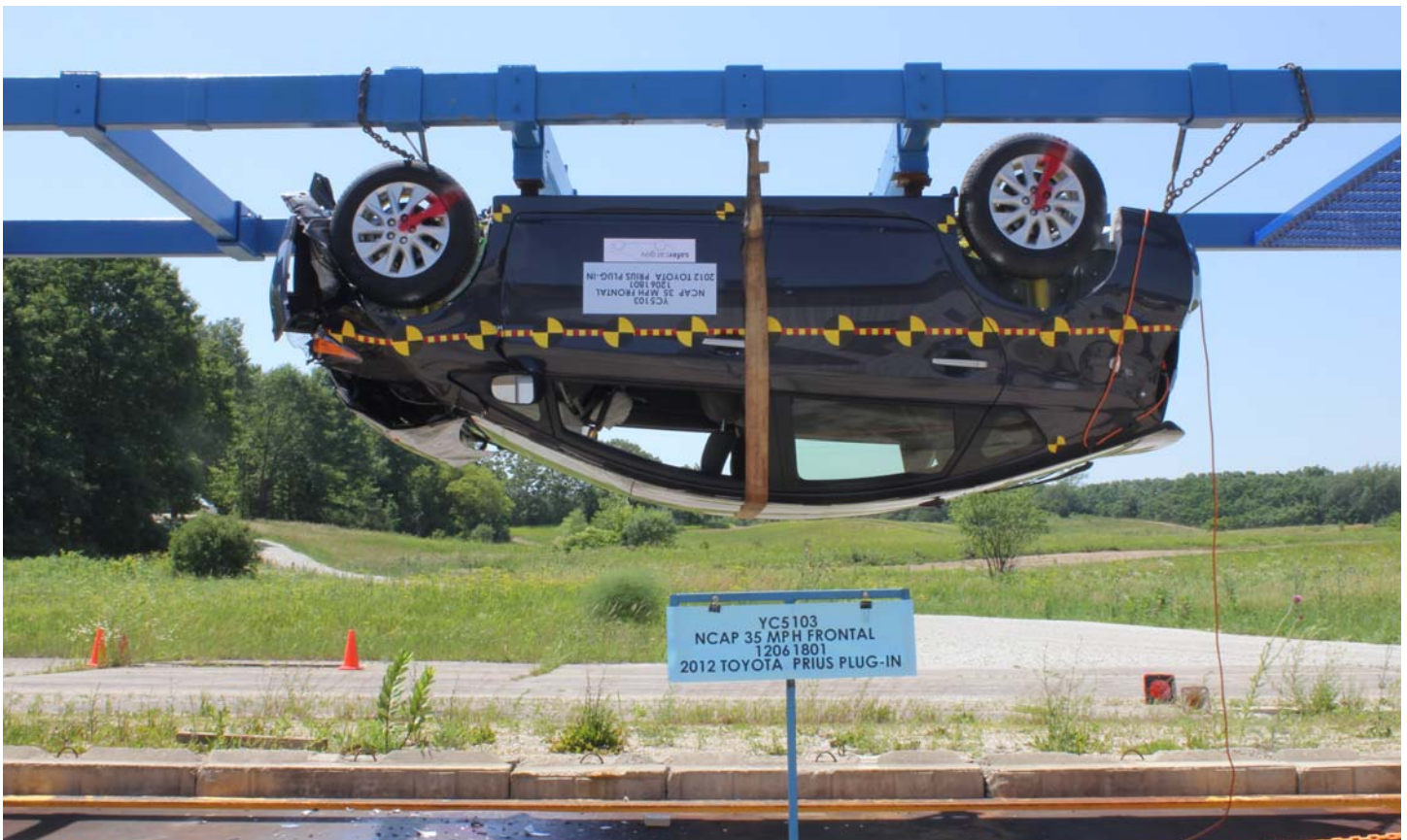
No. 029 FMVSS No. 305 Static Rollover at 180°
