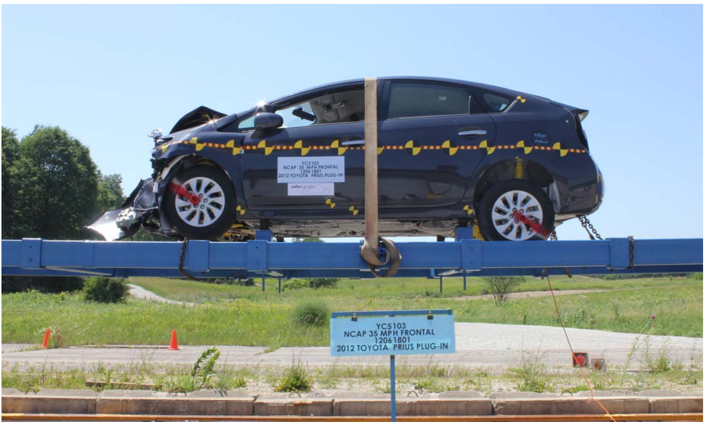
No. 031 FMVSS No. 305 Static Rollover at 360°
