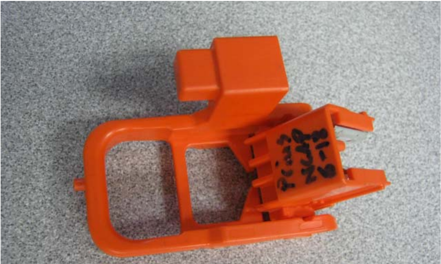
No. 007 Manual High Voltage Service Disconnect Removed
