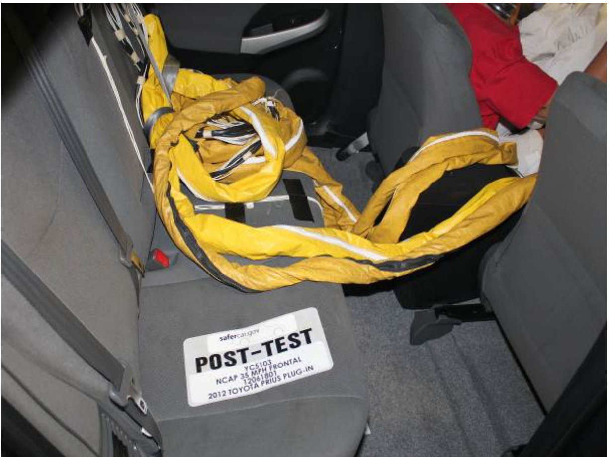
Post-Test Dummy Cable Routing
