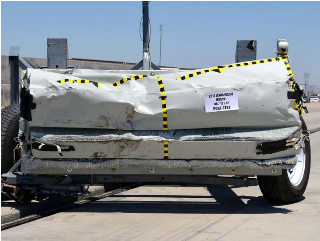
FIGURE 85. Post-Test Front View of MDB Impactor Face
