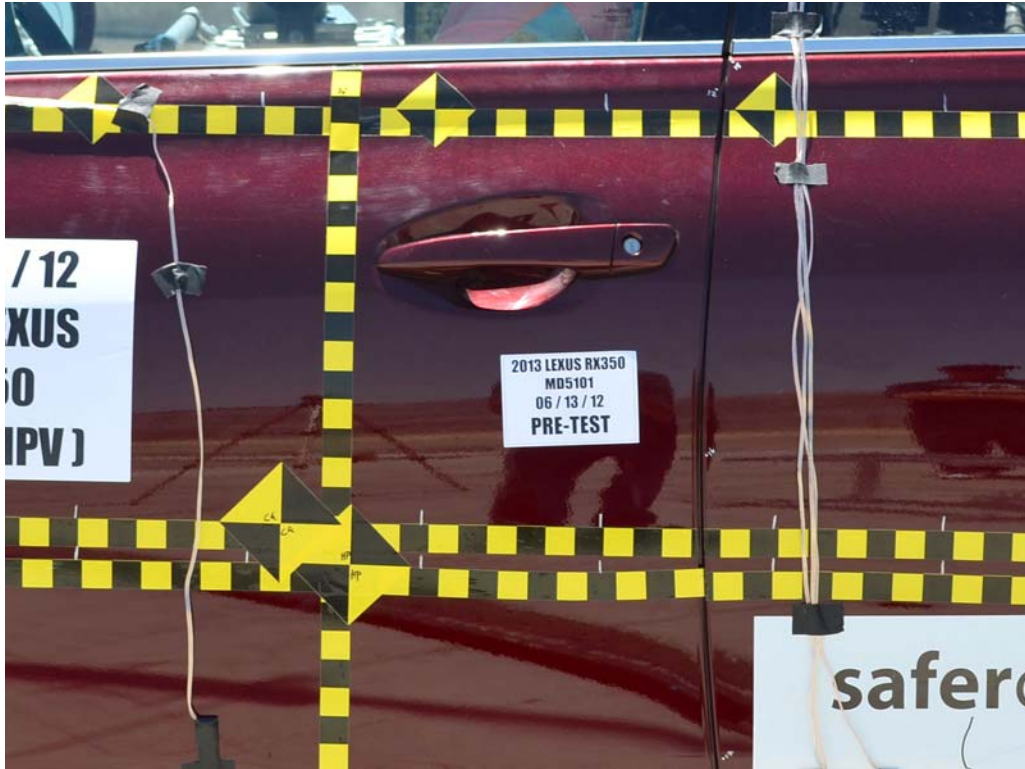
FIGURE 21. Pre-Test Left Front Door Latch Close-Up
