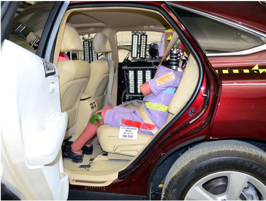
FIGURE 55. Pre-Test Left Side View of Rear Passenger Dummy Showing Belt, Chalking, and Contact Switches
