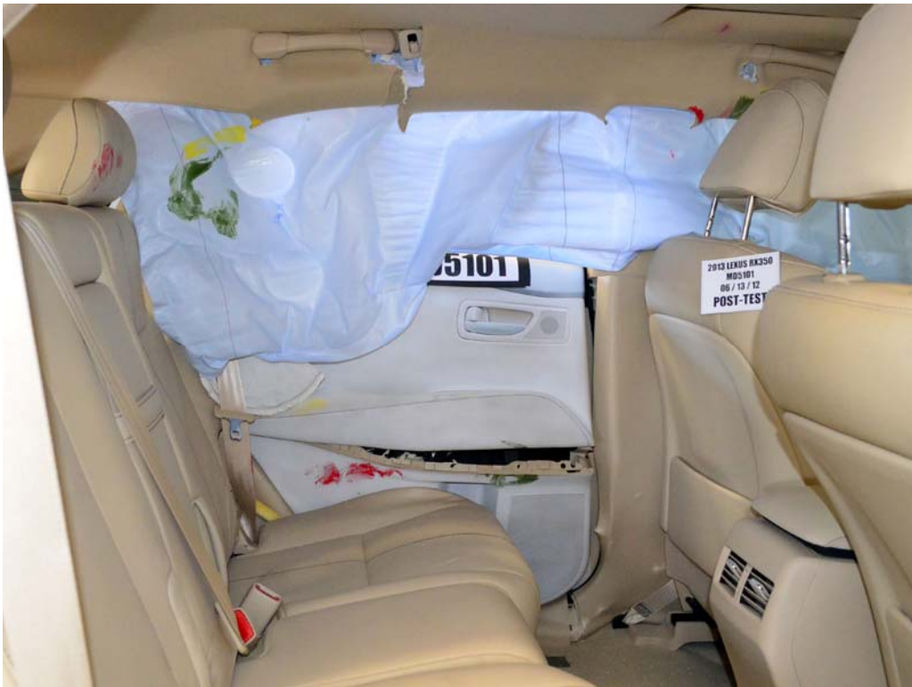
FIGURE 74. Post-Test Rear Passenger Inner Door Panel View
