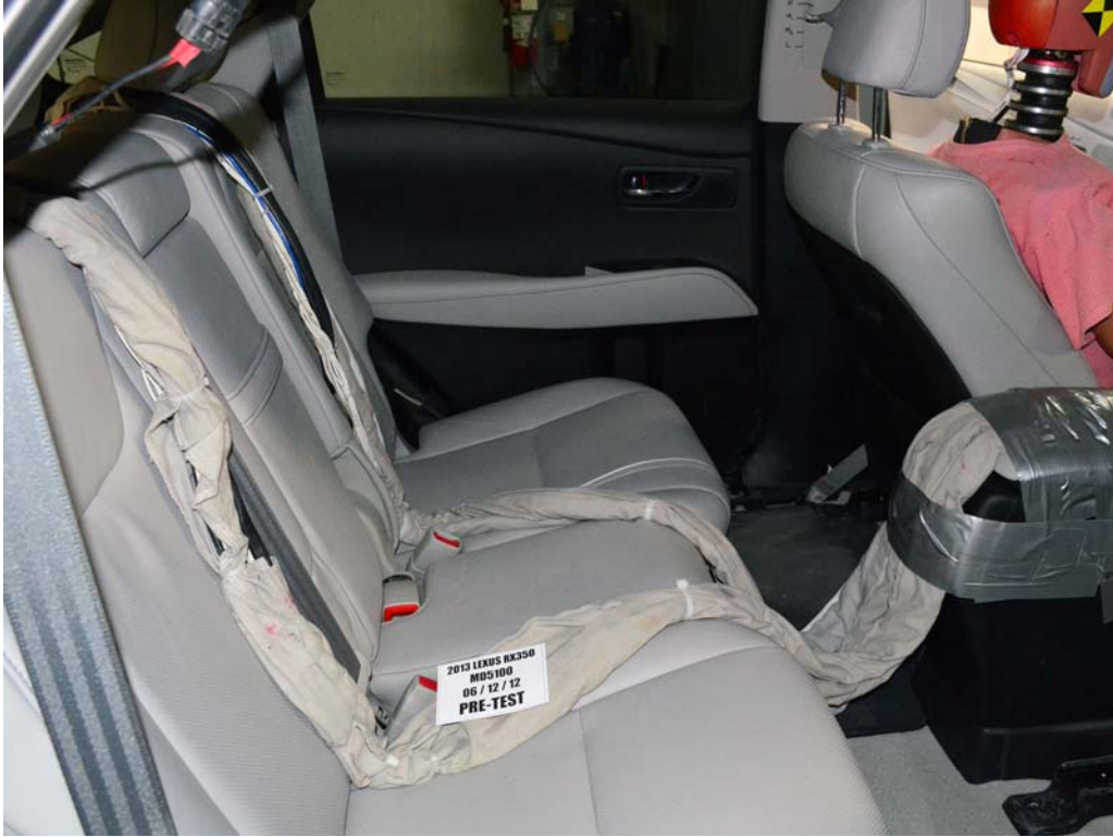
FIGURE 27. Pre-Test Dummy Cable Routing
