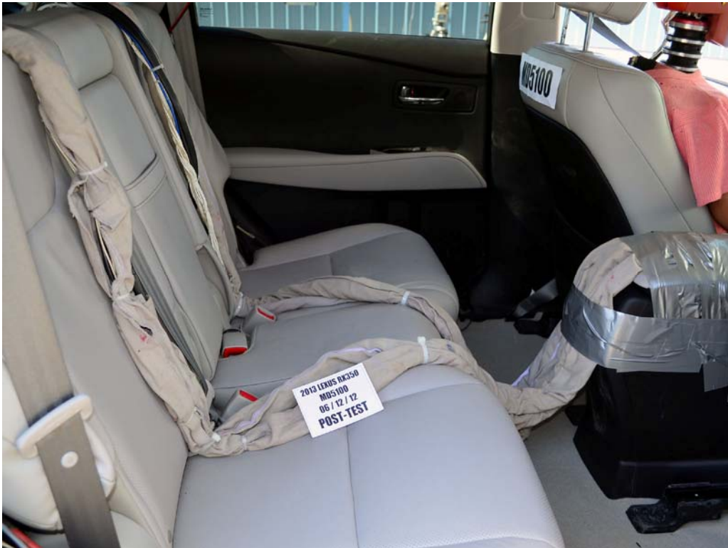
FIGURE 28. Post-Test Dummy Cable Routing
