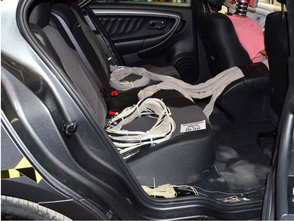
FIGURE 27. Pre-Test Dummy Cable Routing
