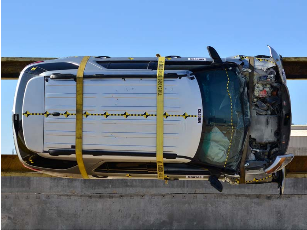
FIGURE 71. Vehicle at 90°on Static Rollover Device
