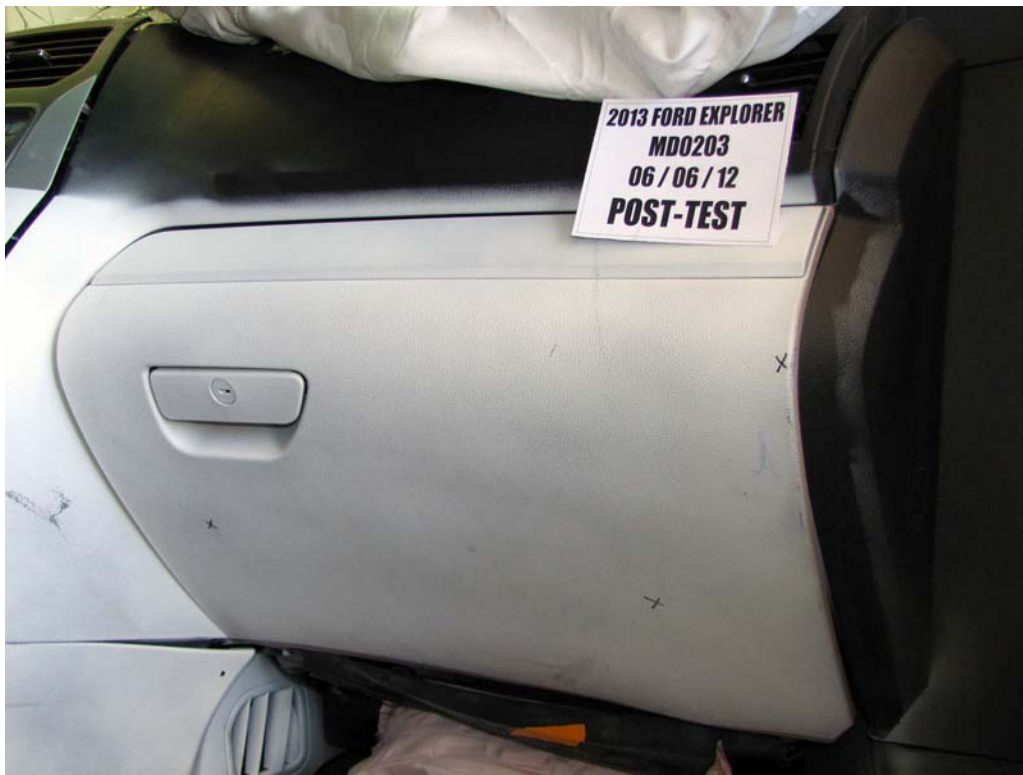
FIGURE 63. Post-Test Passenger's Side Knee Bolster
