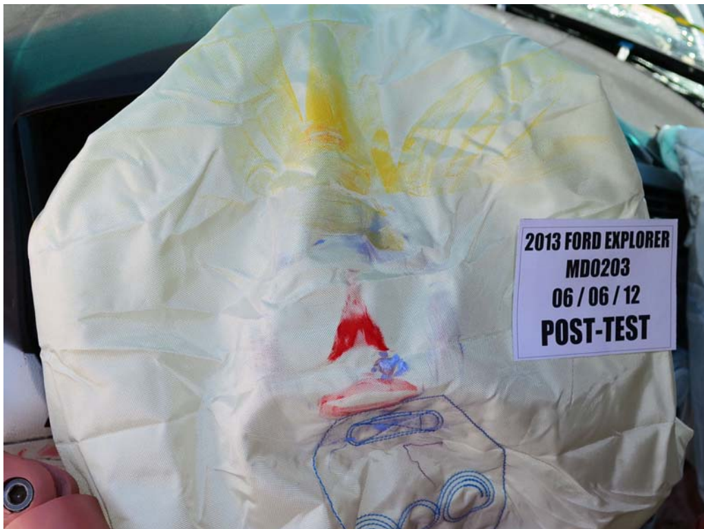
FIGURE 46. Post-Test Driver Dummy Contact With Airbag
