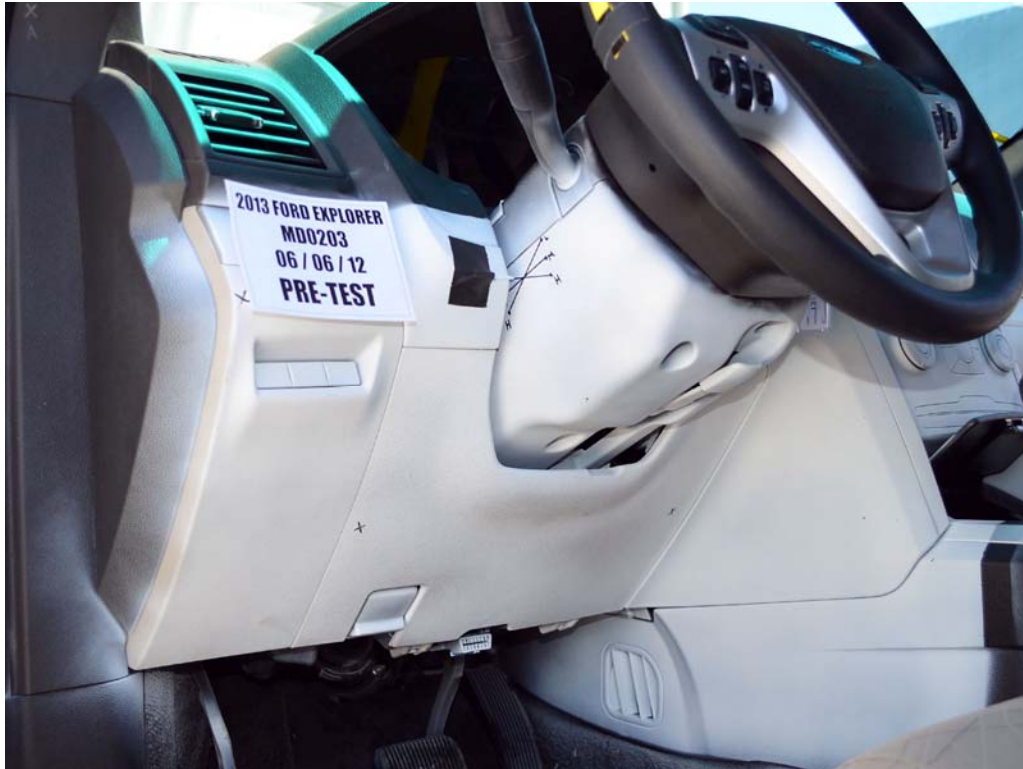
FIGURE 41. Pre-Test Driver's Side Knee Bolster
