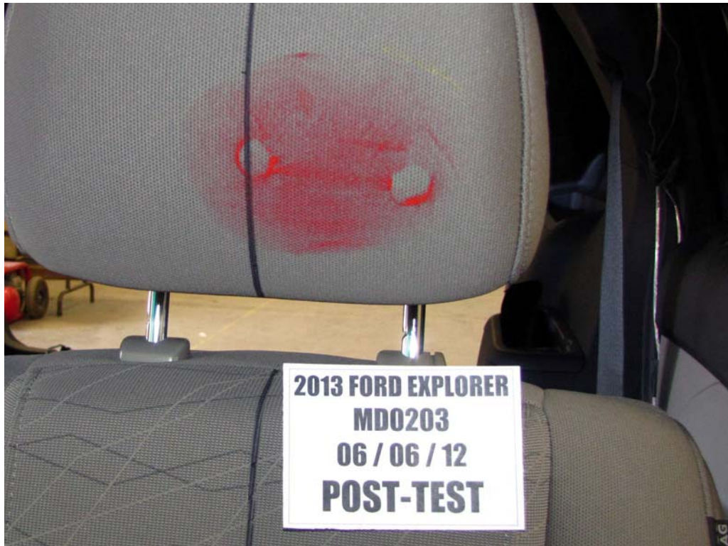
FIGURE 47. Post-Test Driver Dummy Contact With Headrest
