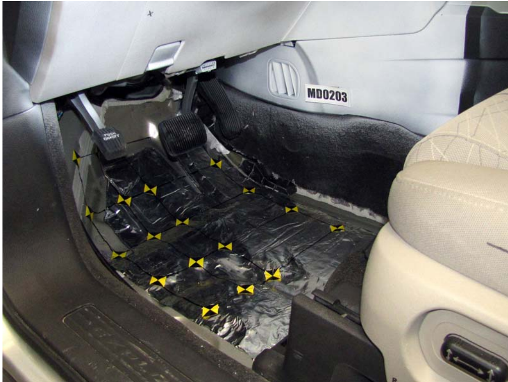
FIGURE 43. Pre-Test Driver's Side Floorpan
