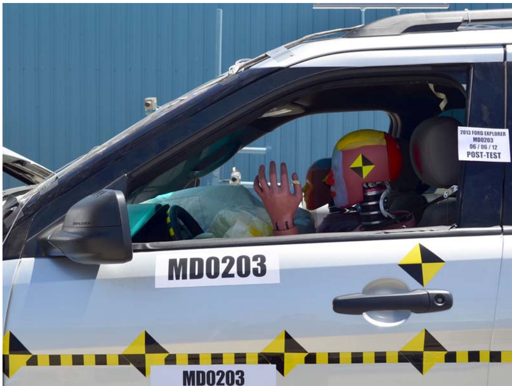
FIGURE 32. Post-Test Driver Dummy Window View
