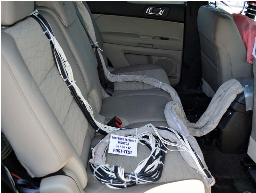
FIGURE 28. Post-Test Dummy Cable Routing
