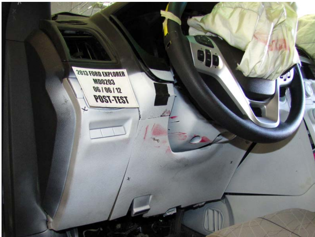
FIGURE 42. Post-Test Driver's Side Knee Bolster
