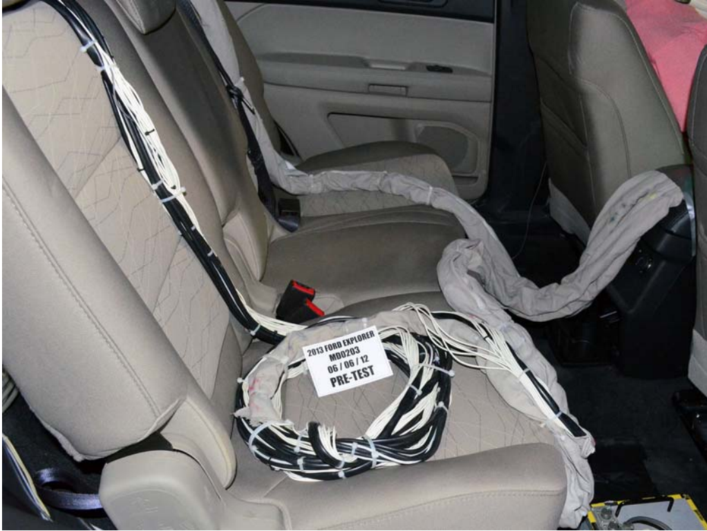
FIGURE 27. Pre-Test Dummy Cable Routing
