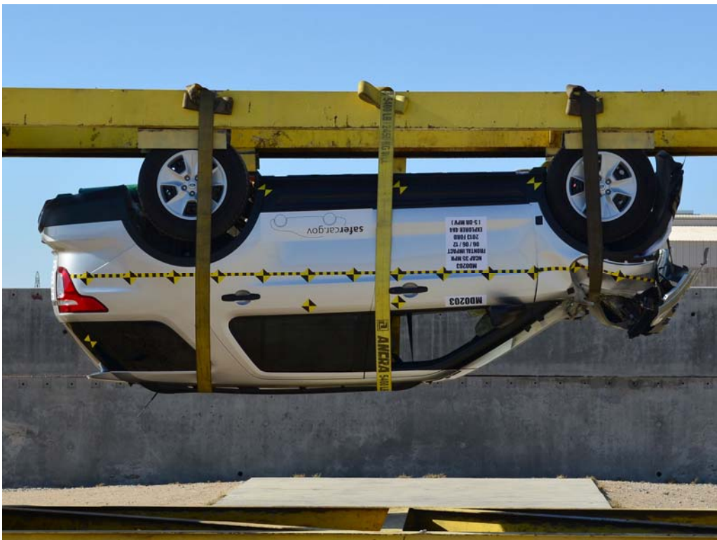
FIGURE 72. Vehicle at 180°on Static Rollover Device
