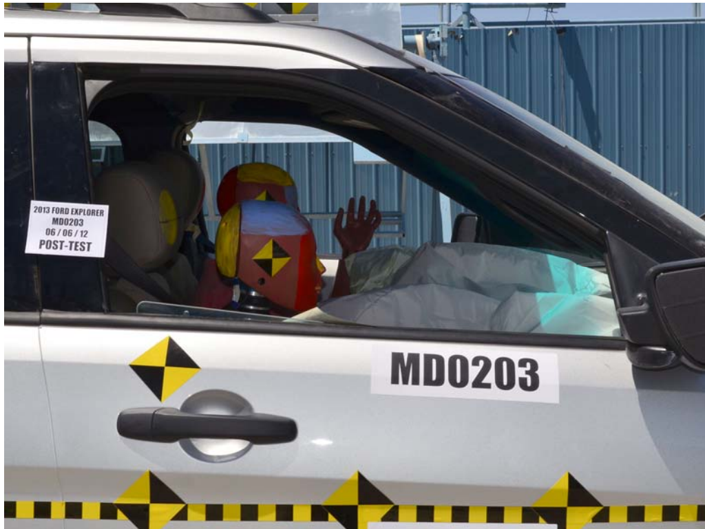
FIGURE 53. Post-Test Passenger Dummy Window View
