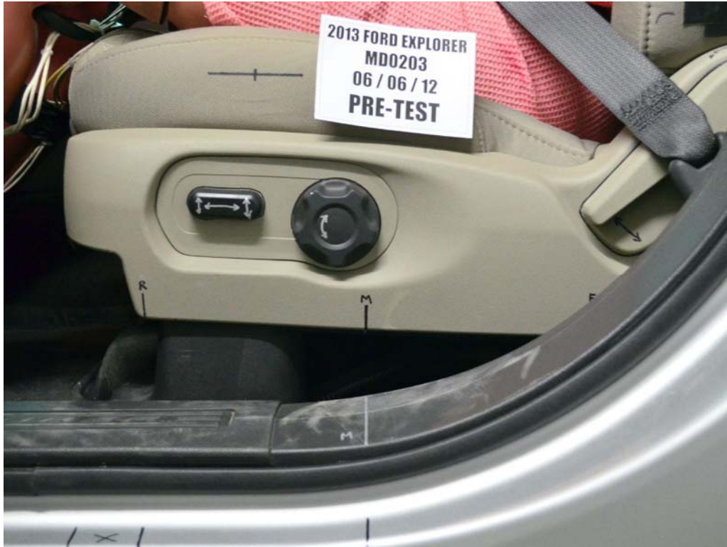
FIGURE 35. Pre-Test Driver's Seat Fore-Aft Markings
