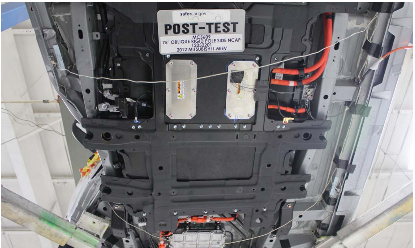
No. 015 Post-Impact View of Propulsion Battery Module(s)
