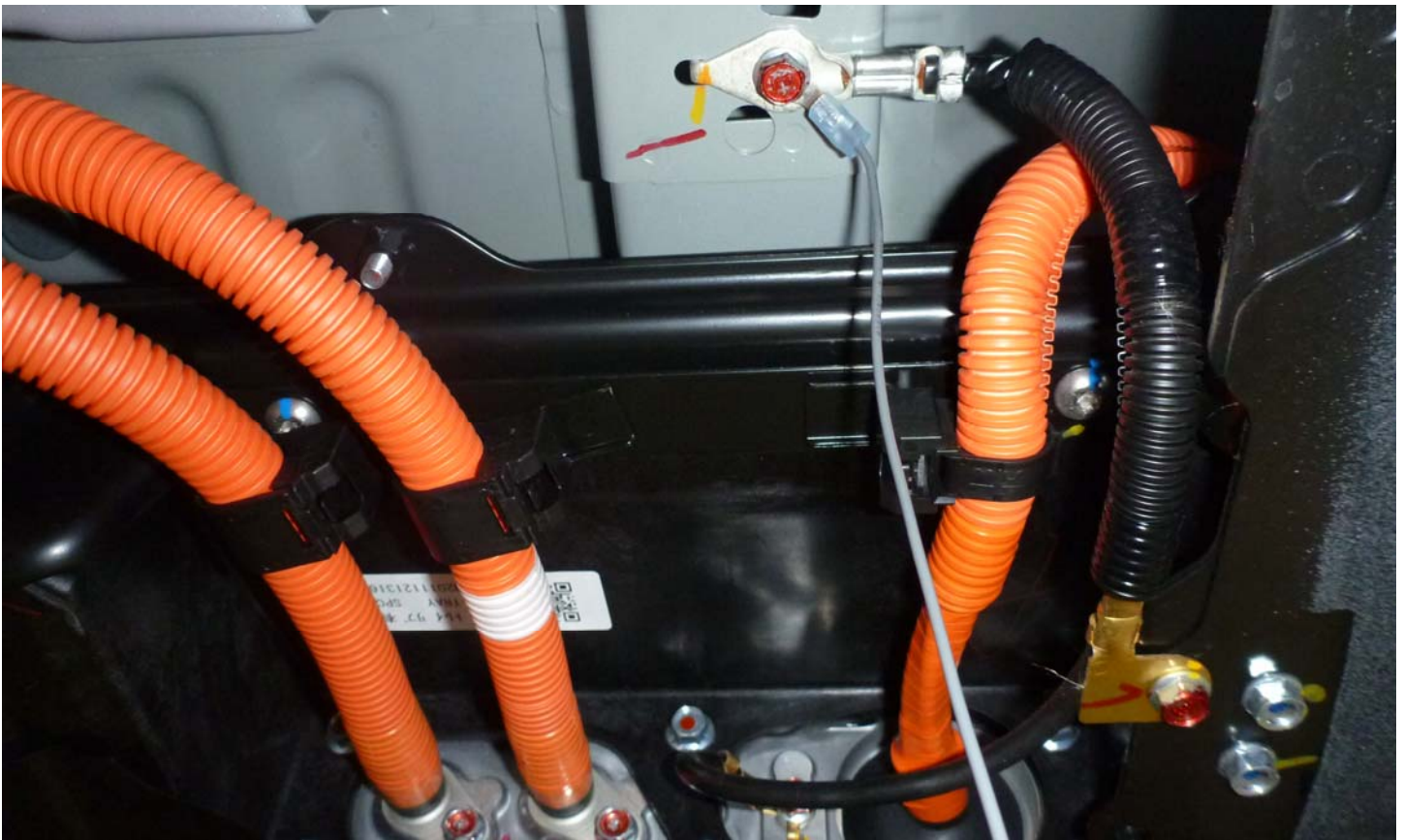
No. 021 Pre-Impact View of Ground Lead Attached
