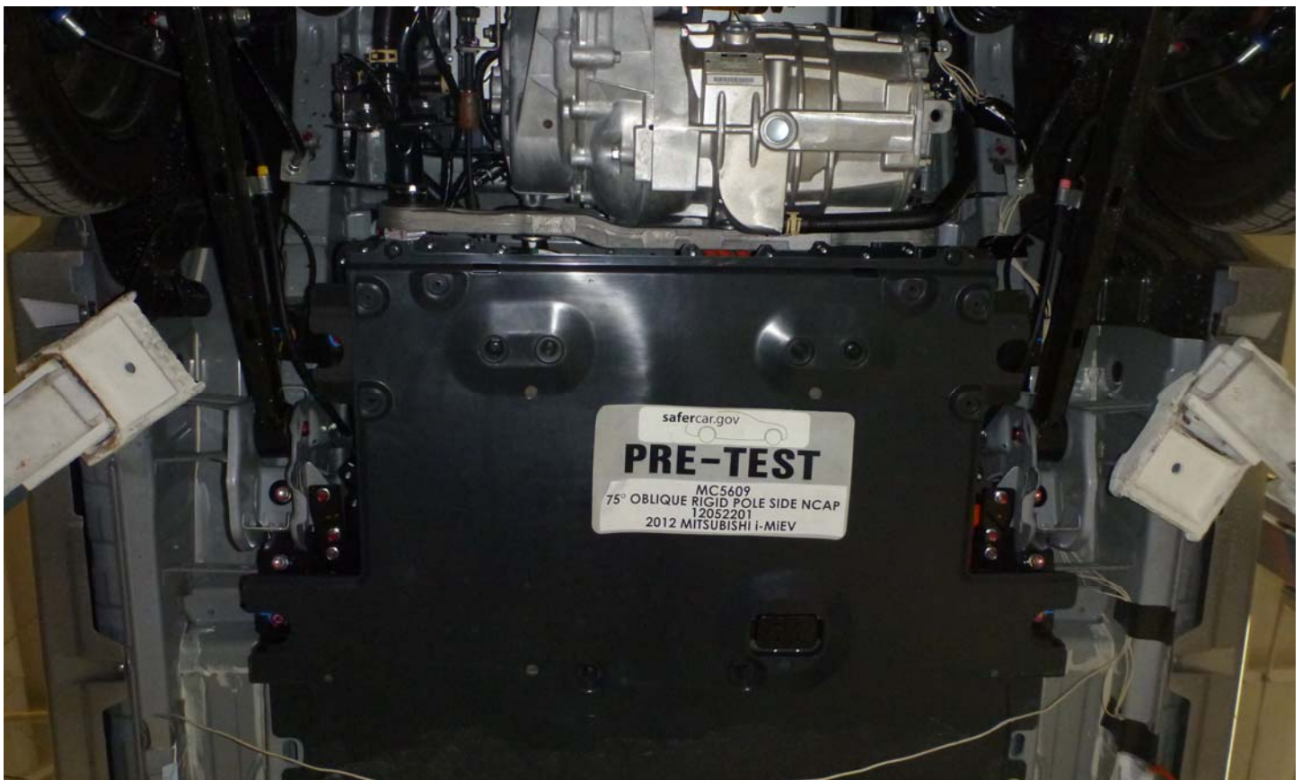
No. 012a Pre-Impact View of Battery Box(s) or Container(s) Which Holds Individual Battery Modules
