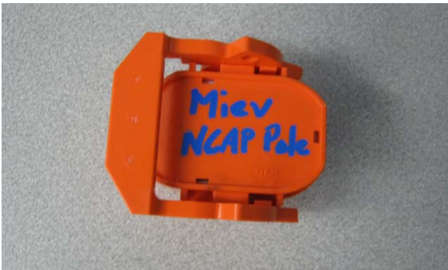
No. 008 Manual High Voltage Service Disconnect Removed
