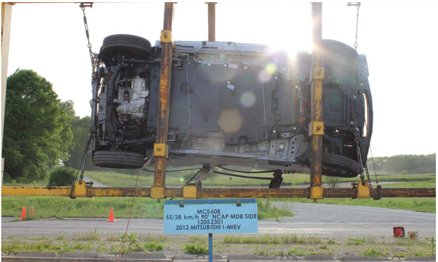
No. 030 FMVSS No. 305 Static Rollover at 270°
