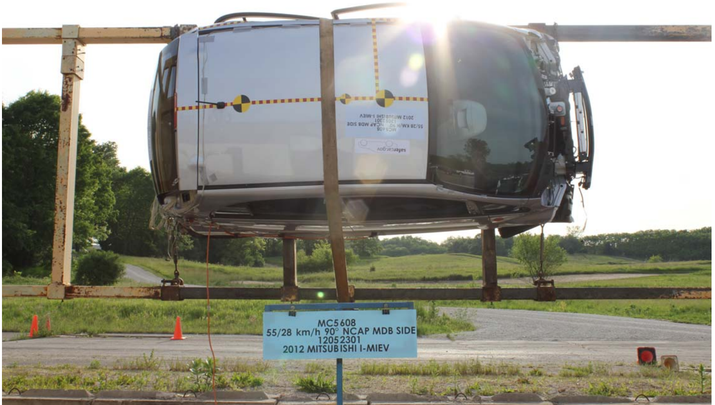
No. 028 FMVSS No. 305 Static Rollover at 90°
