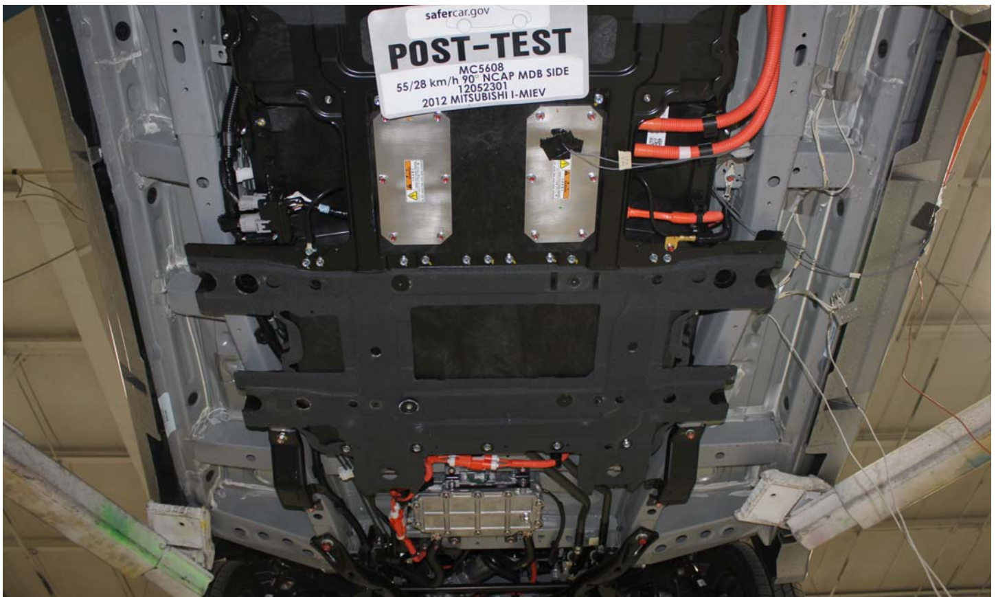
No. 010 Post-Impact Front View of Propulsion Battery
