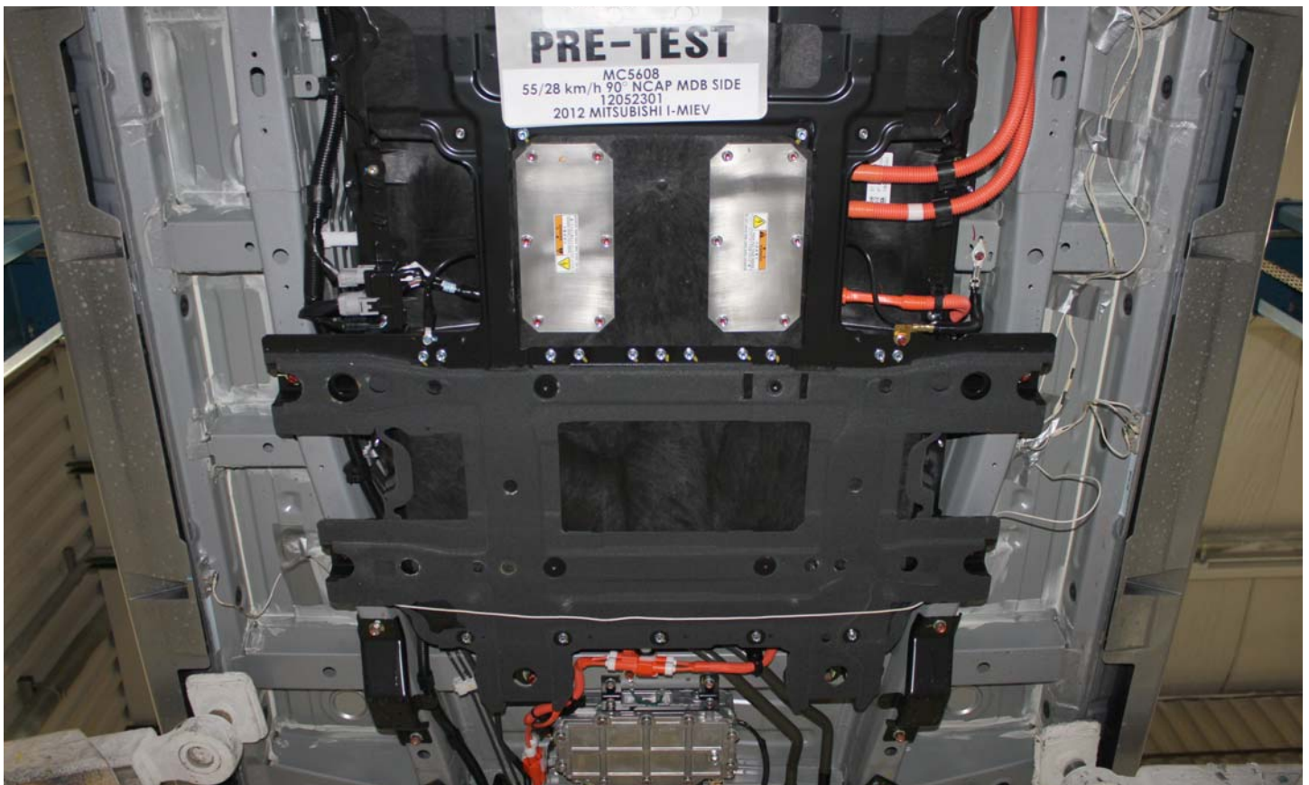
No. 014 Pre-Impact View of Propulsion Battery Module(s)
