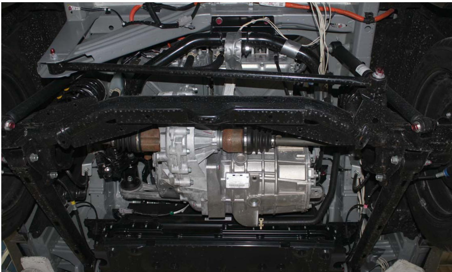
No. 016 Pre-Impact View of Electric Propulsion Drive
