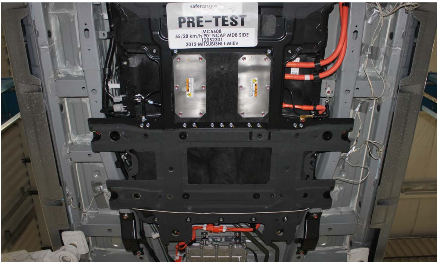
No. 009 Pre-Impact View of Propulsion Battery
