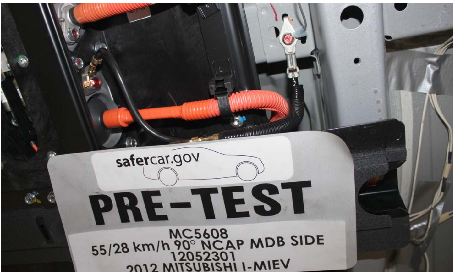
No. 021 Pre-Impact View of Ground Lead Attached
