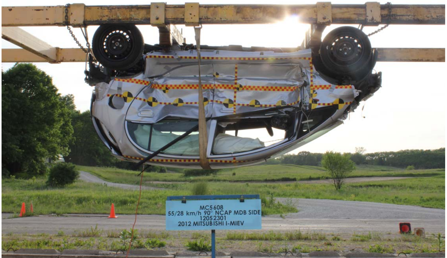
No. 029 FMVSS No. 305 Static Rollover at 180°
