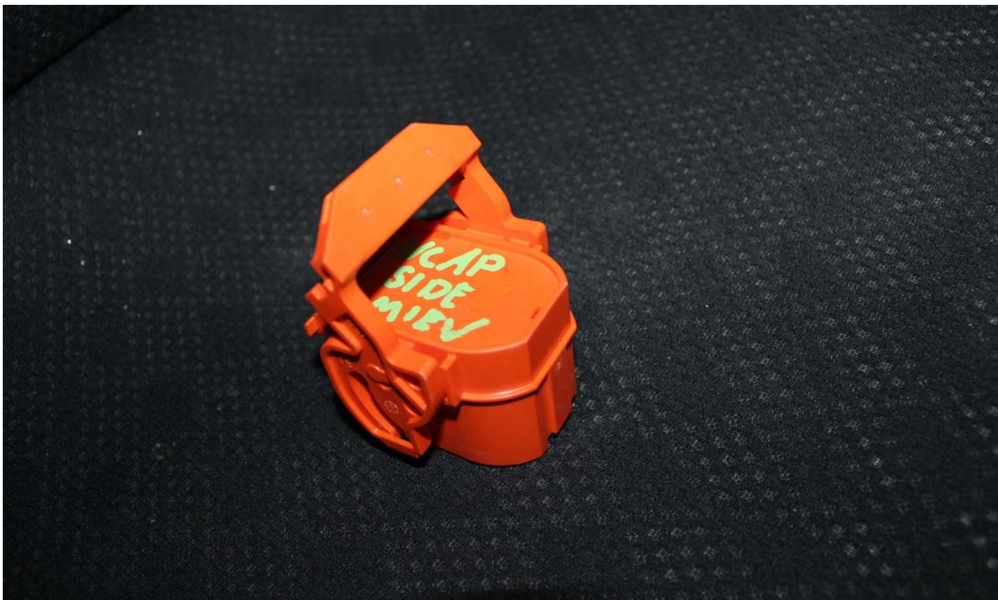
No. 007 Manual High Voltage Service Disconnect Removed
