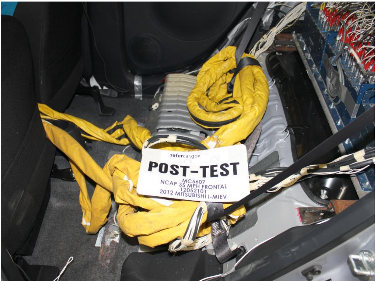
Post-Test Dummy Cable Routing
