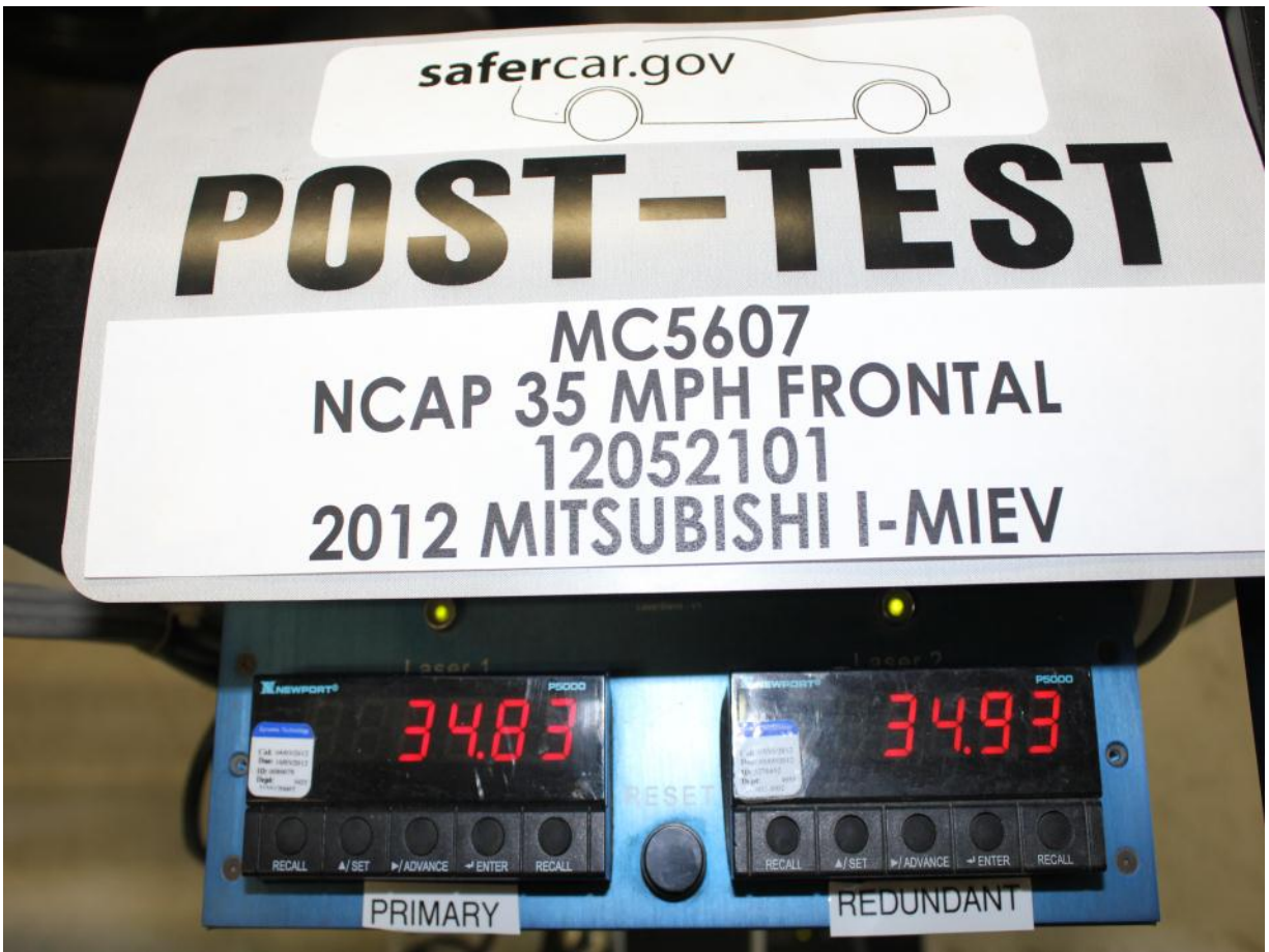
Post-Test Speed Trap Read-Out
