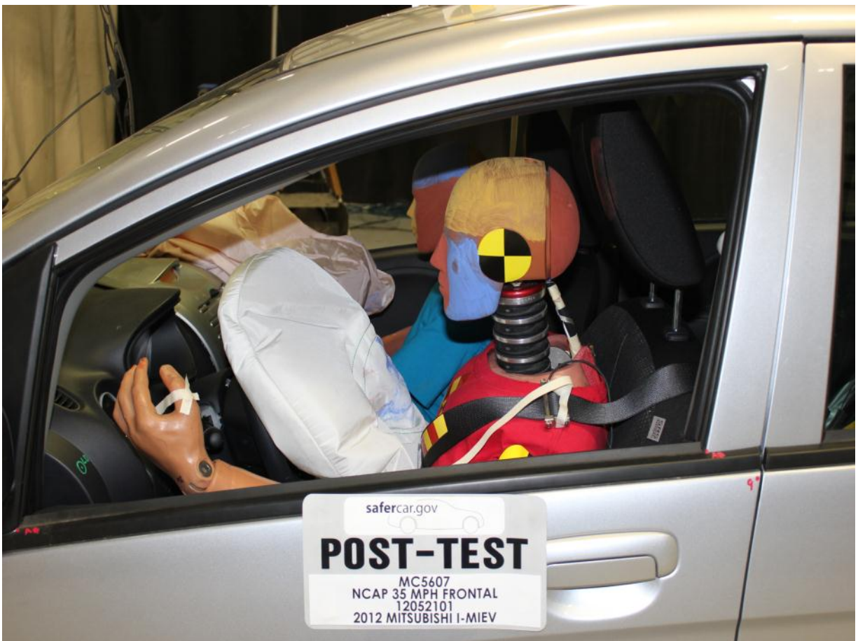
Post-Test Driver Dummy Window View
