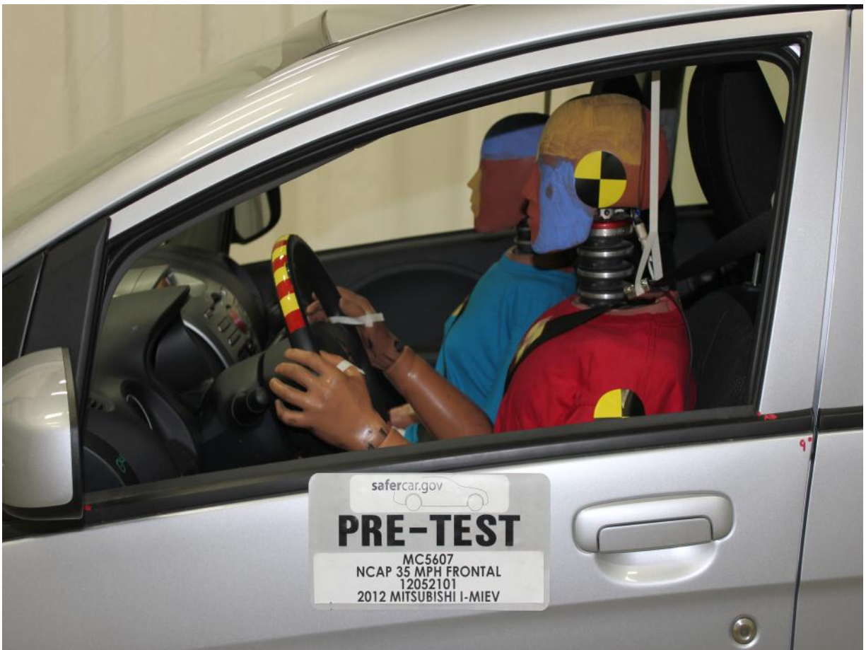
Pre-Test Driver Dummy Window View
