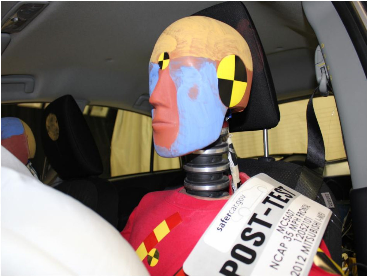
Post-Test Driver Dummy Face
