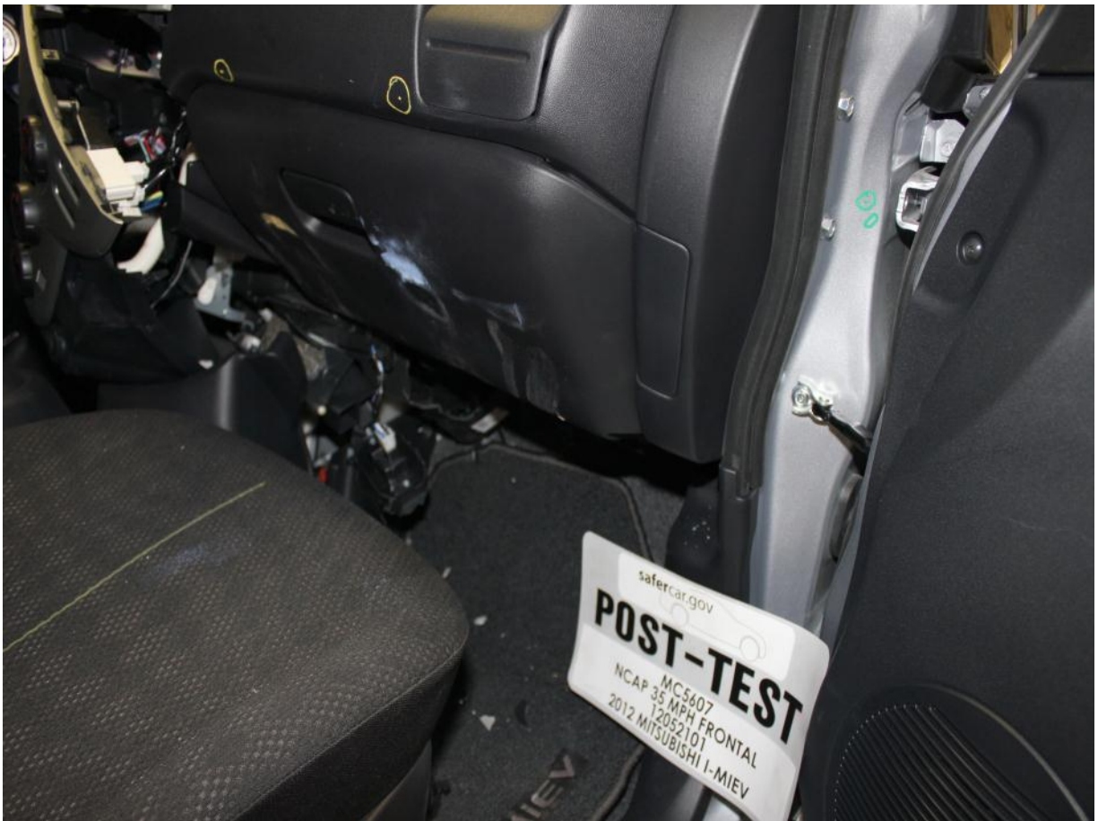
Post-Test Passenger's Side Knee Bolster (without dummy)
