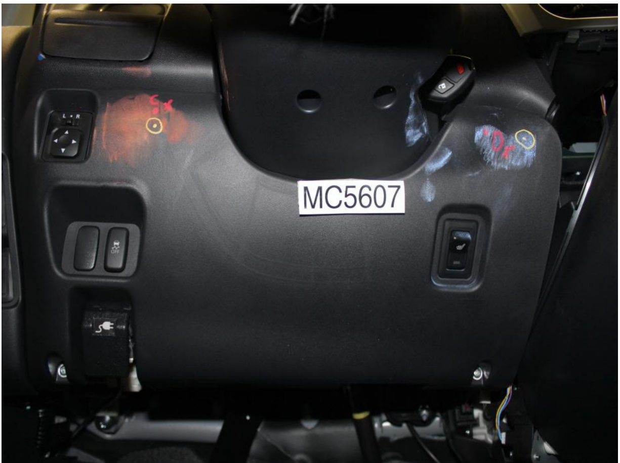
Post-Test Driver Dummy Contact with K nee Bolster
