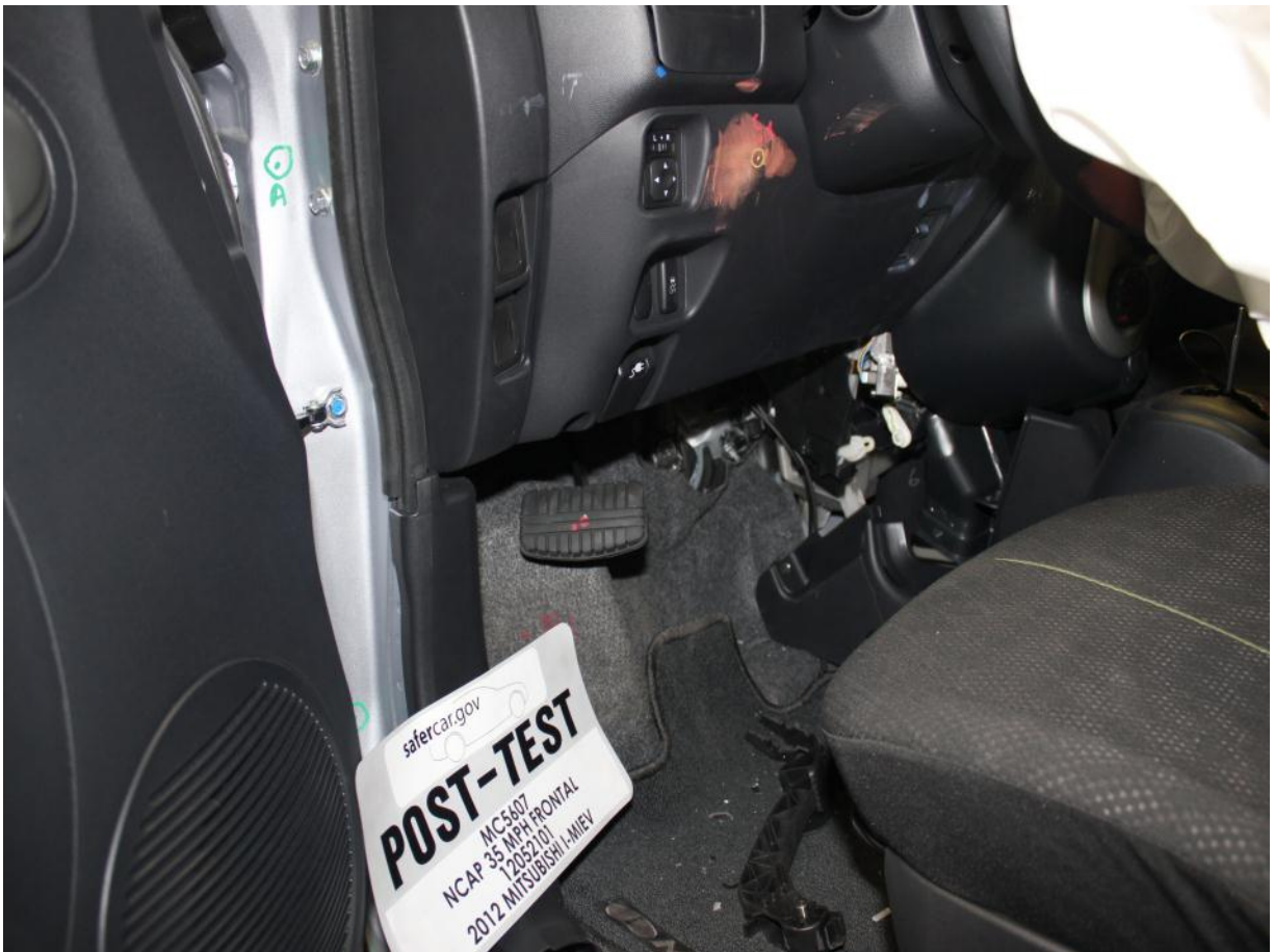
Post-Test Driver's Side Knee Bolster (without dummy)
