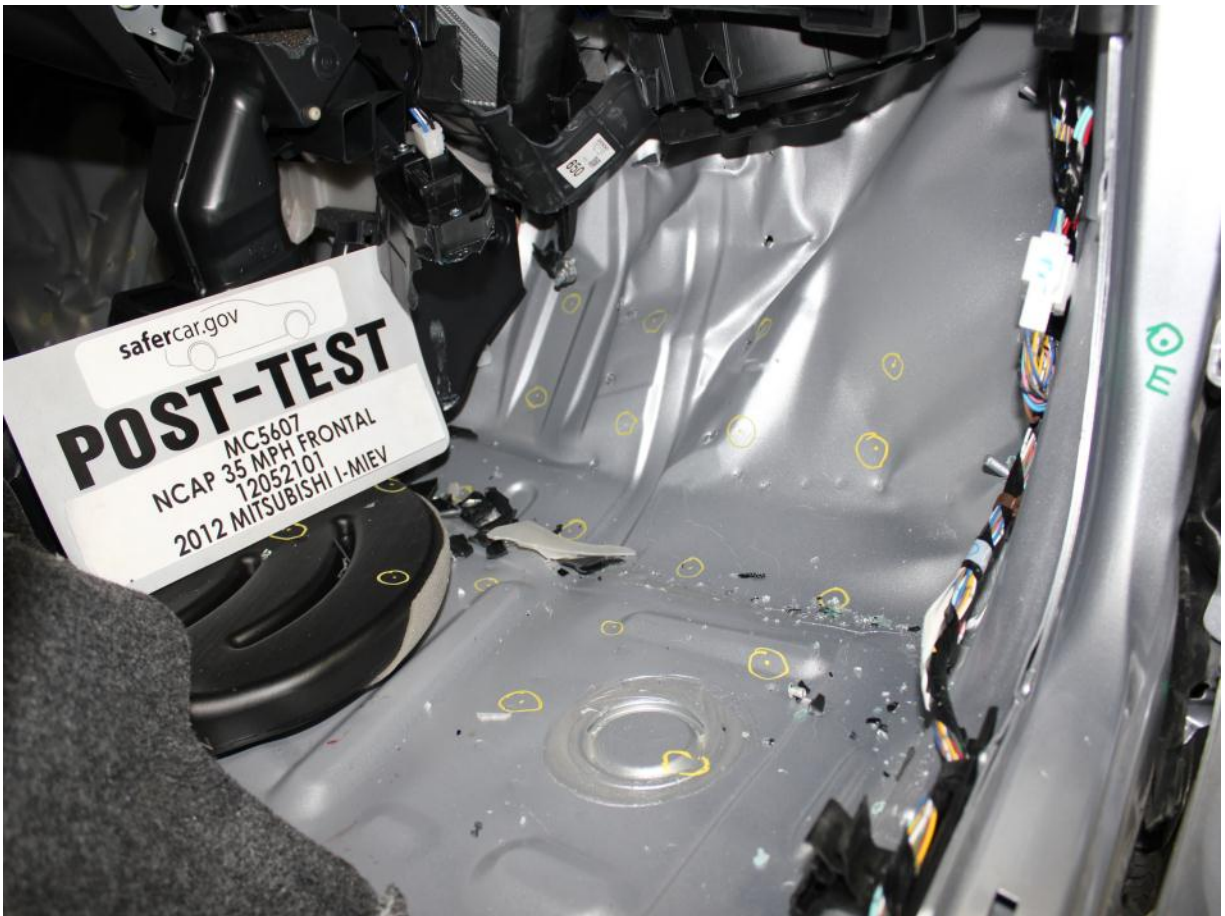
Post-Test Passenger's Side Floorpan
