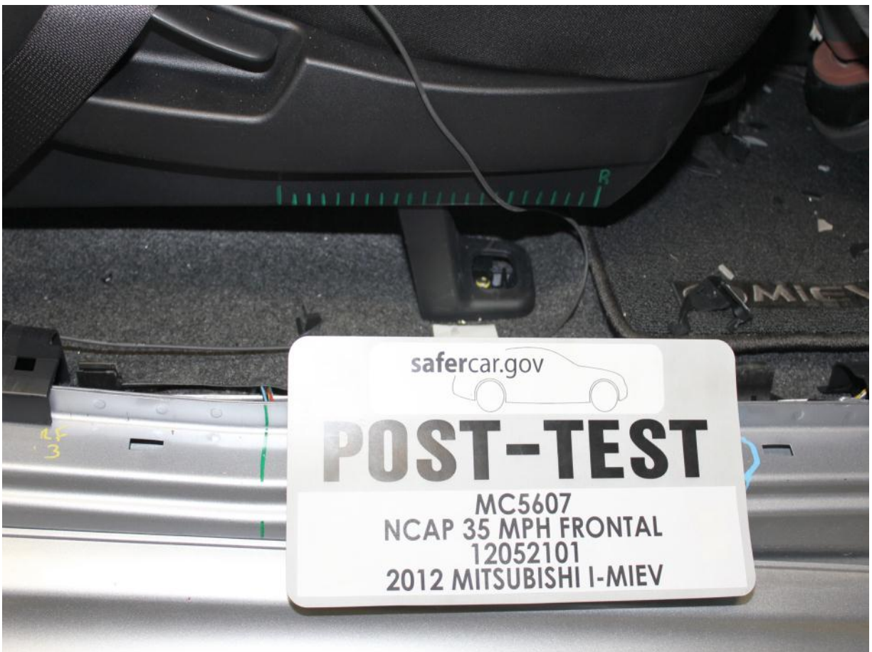
Post-Test Passenger's Seat Fore-Aft Markings
