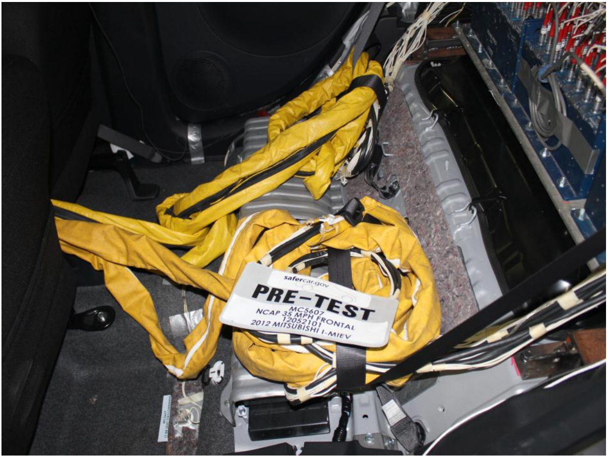
Pre-Test Dummy Cable Routing
