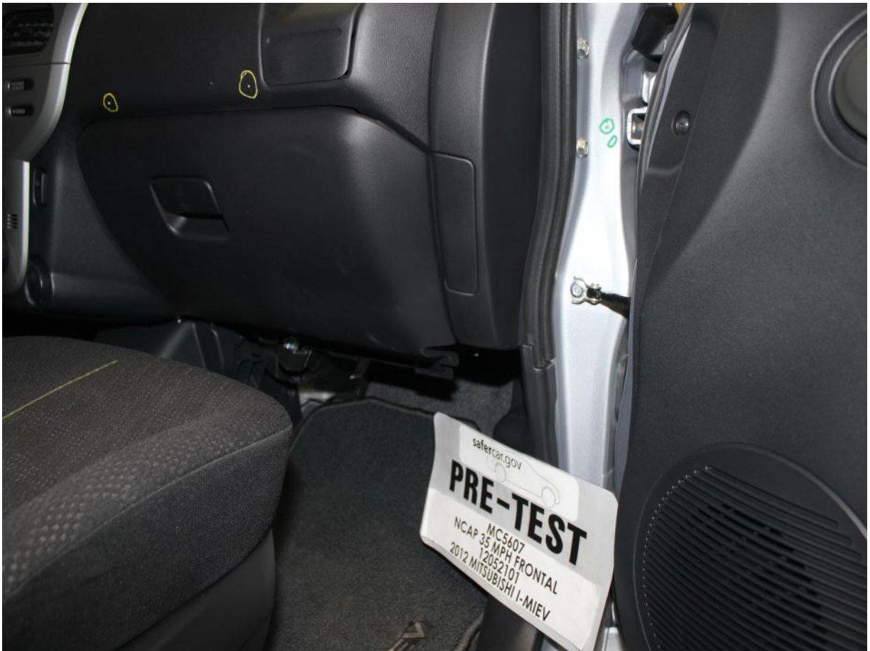
Pre-Test Passenger's Side Knee Bolster (without dummy)
