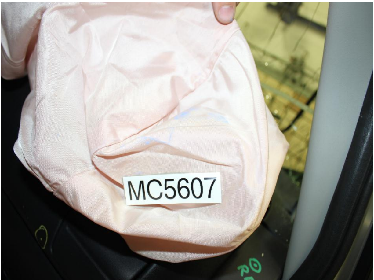
Post-Test Passenger Dummy Contact with Airbag
