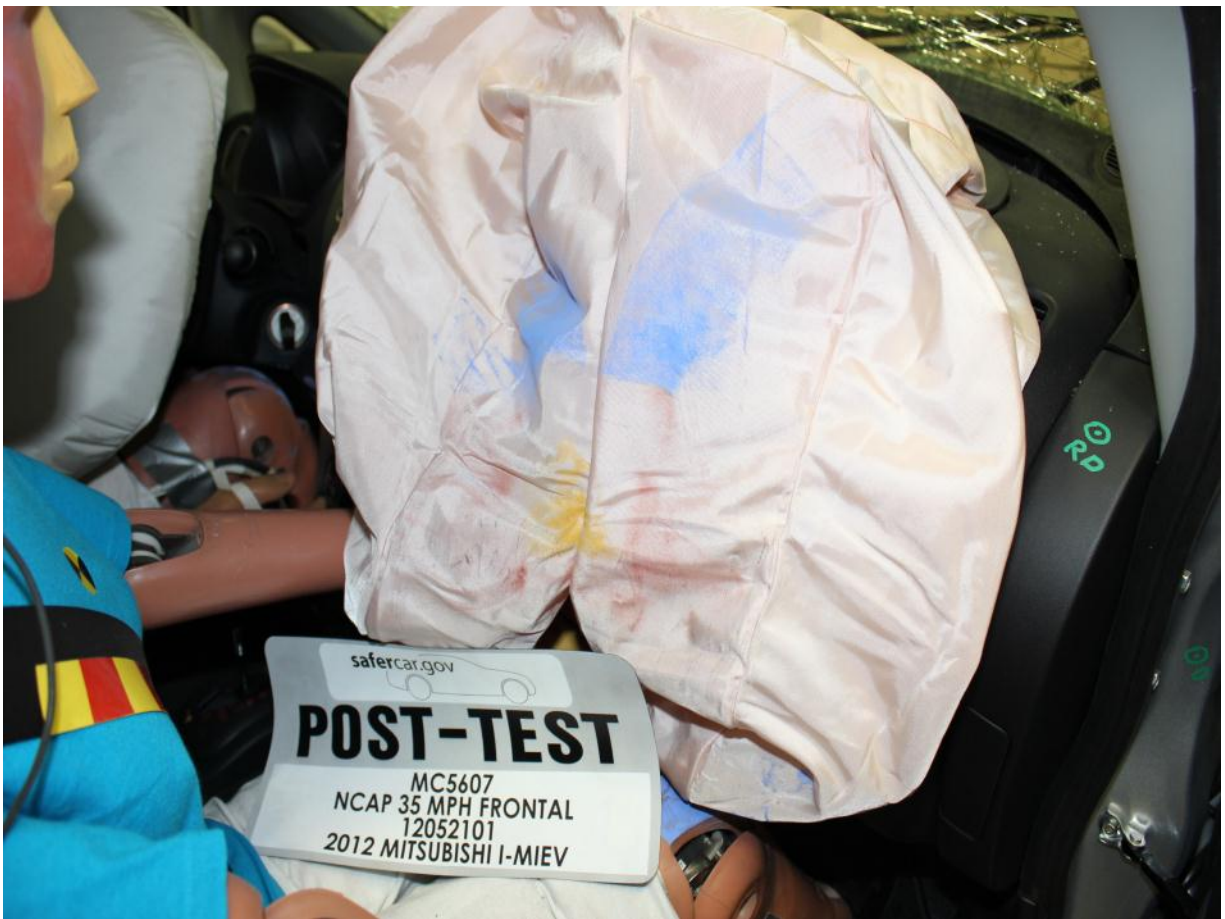
Post-Test Passenger Dummy Contact with Airbag
