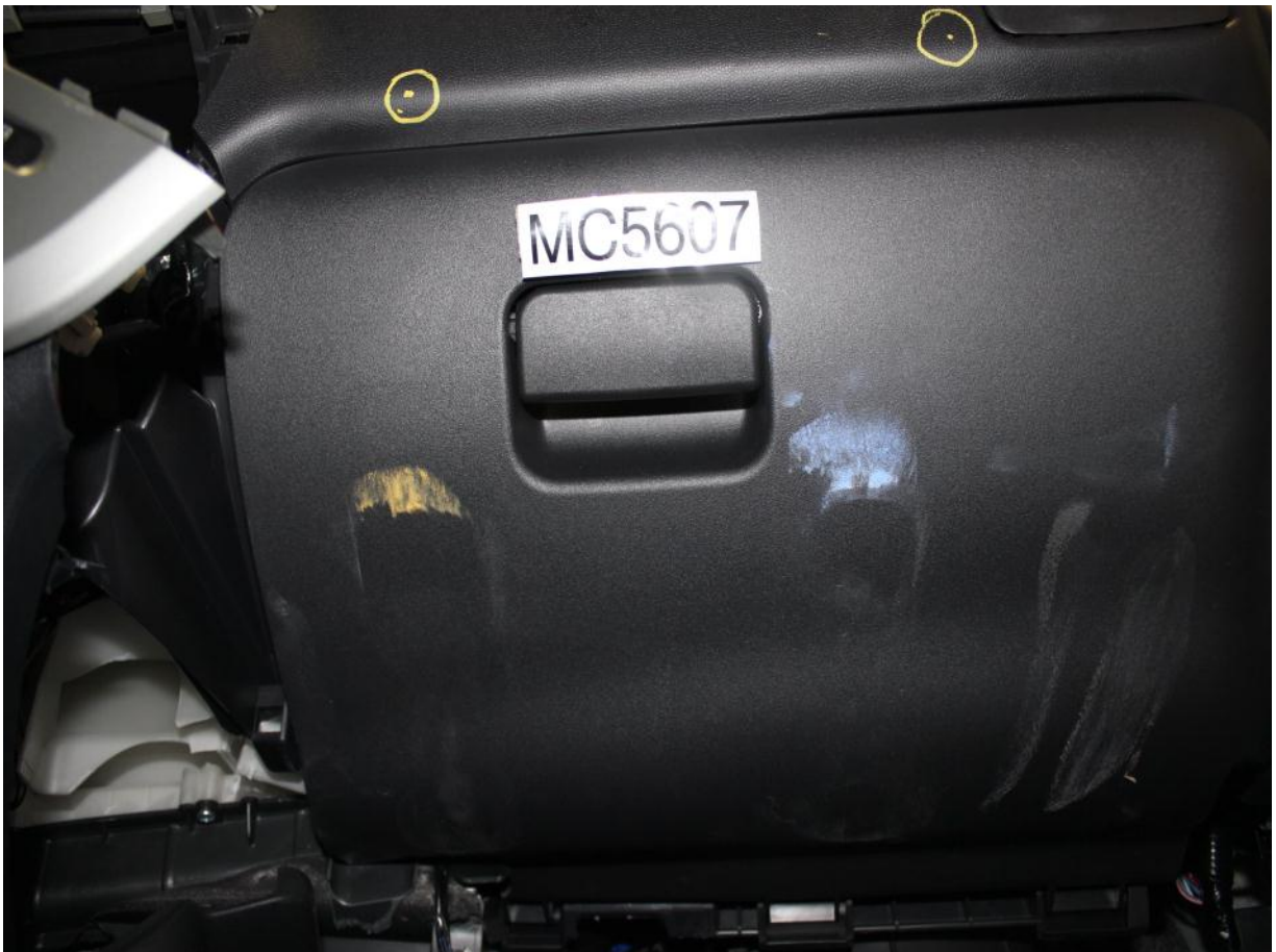
Post-Test Passenger Dummy Contact with Glove Box
