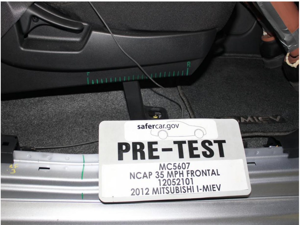
Pre-Test Passenger's Seat Fore-Aft Markings
