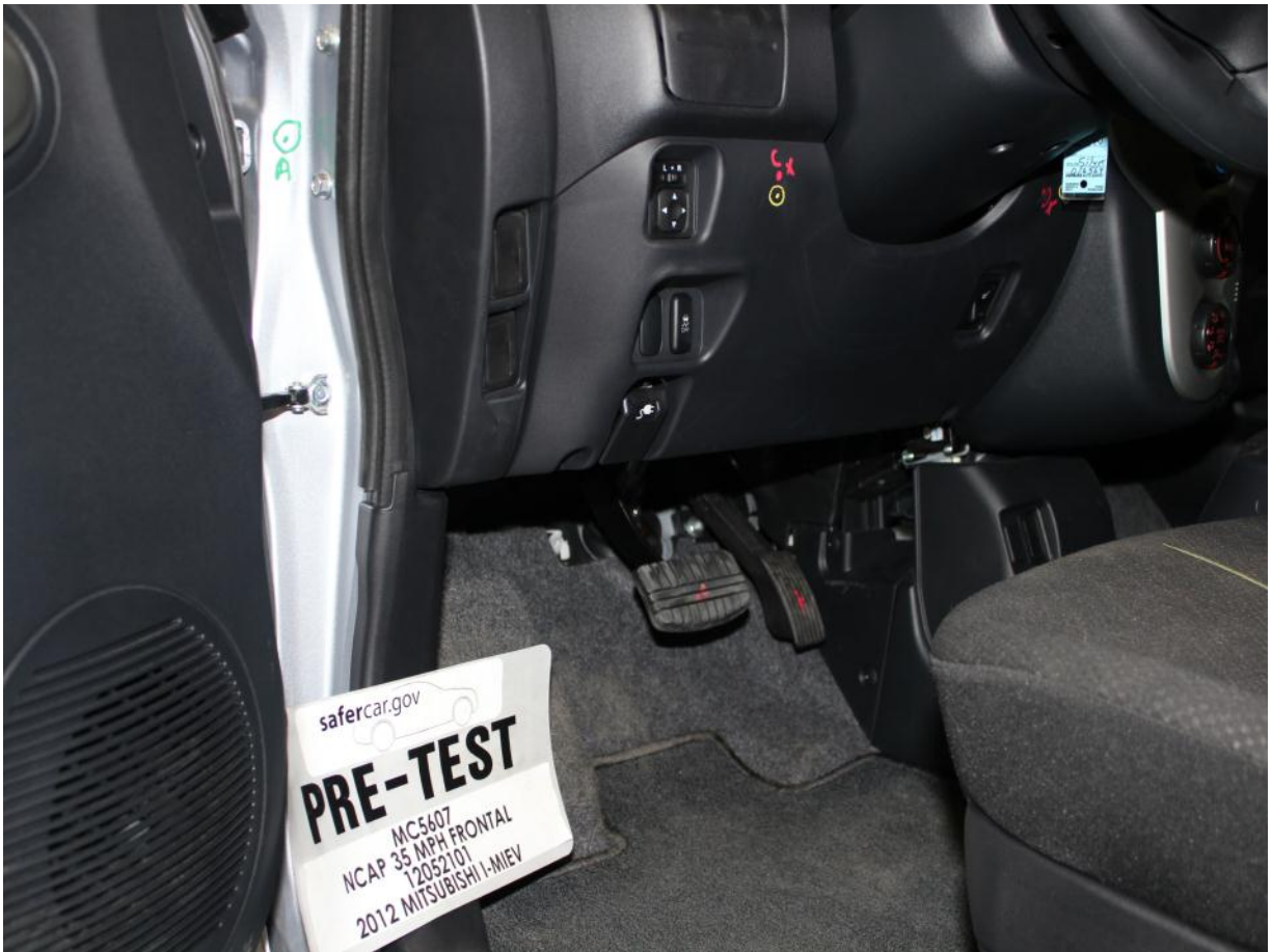
Pre-Test Driver's Side Knee Bolster (without dummy)
