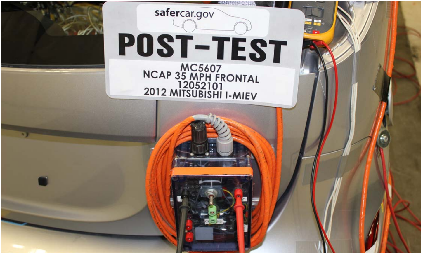
No. 025 Post-Impact View of Installed Impact Interface Port
