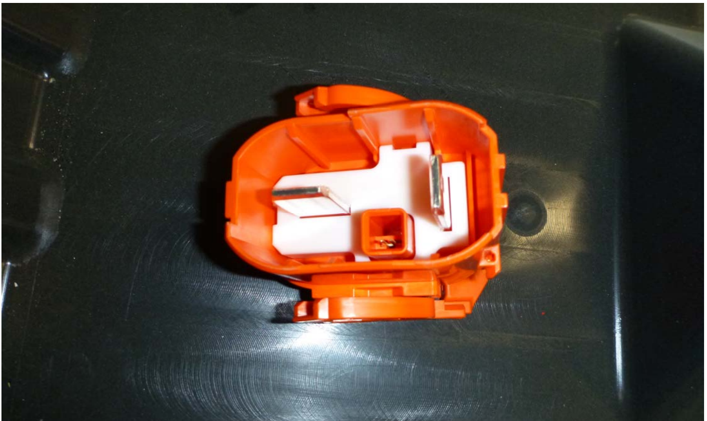
No. 007a Manual High Voltage Service Disconnect Removed
