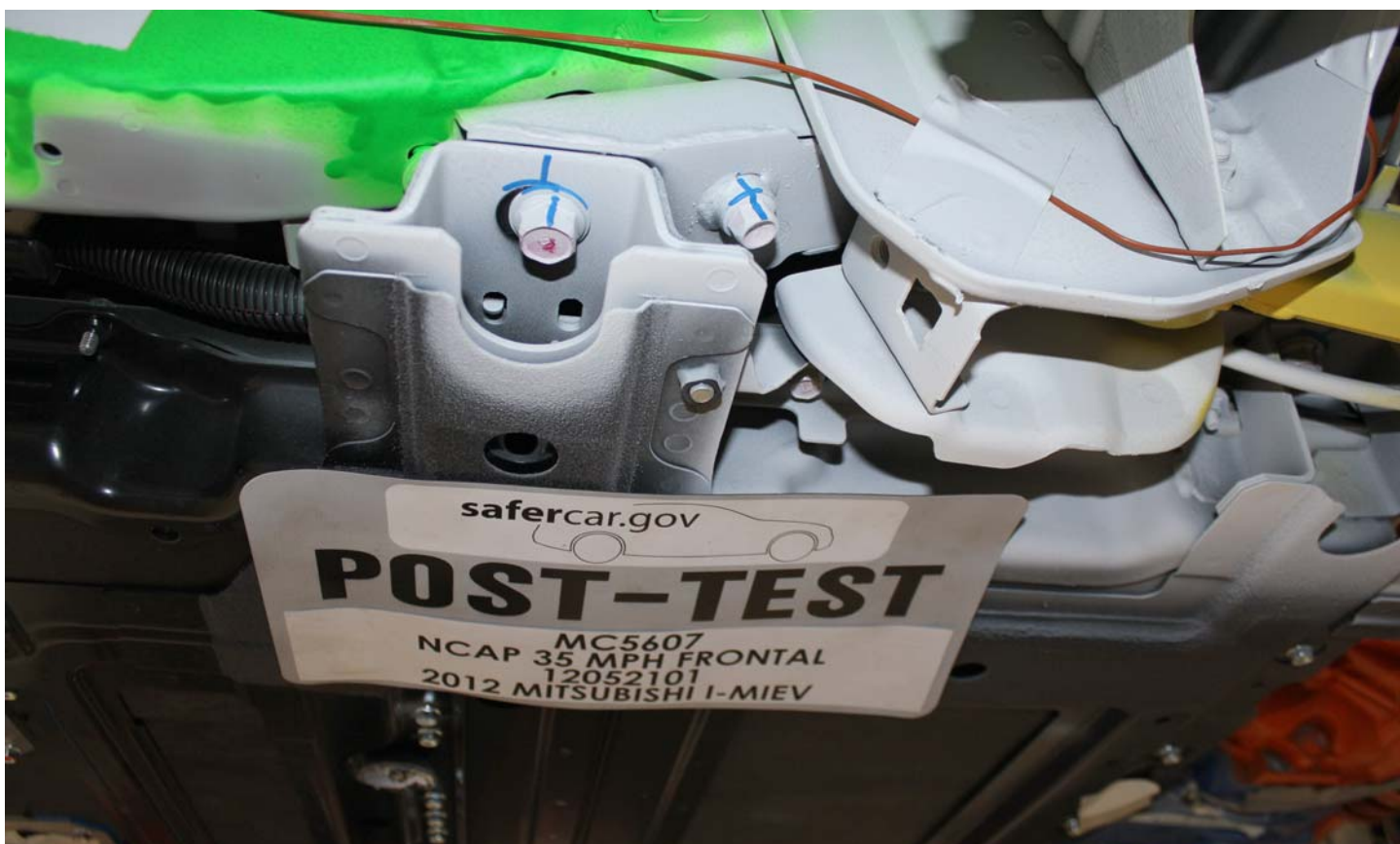
No. 036 Post-Impact View of Battery Module Movement or Retention Loss
