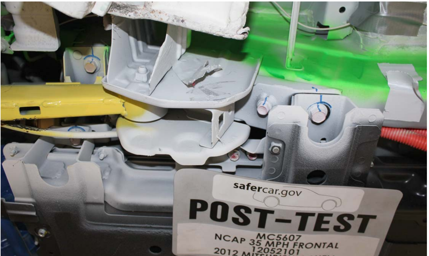
No. 036a Post-Impact View of Battery Module Movement or Retention Loss
