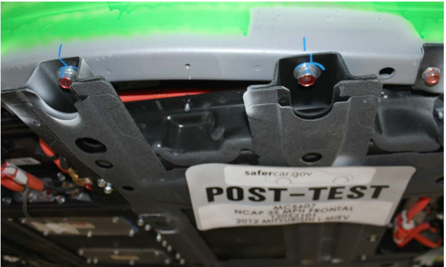
No. 036c Post-Impact View of Battery Module Movement or Retention Loss
