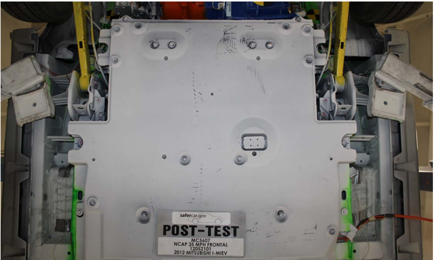
No. 013a Post-Impact View of Battery Box(s) or Container(s) Which Holds Individual Battery Modules
