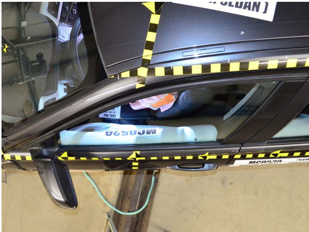
FIGURE 40. Pre-Test Driver Dummy and Door Clearance
