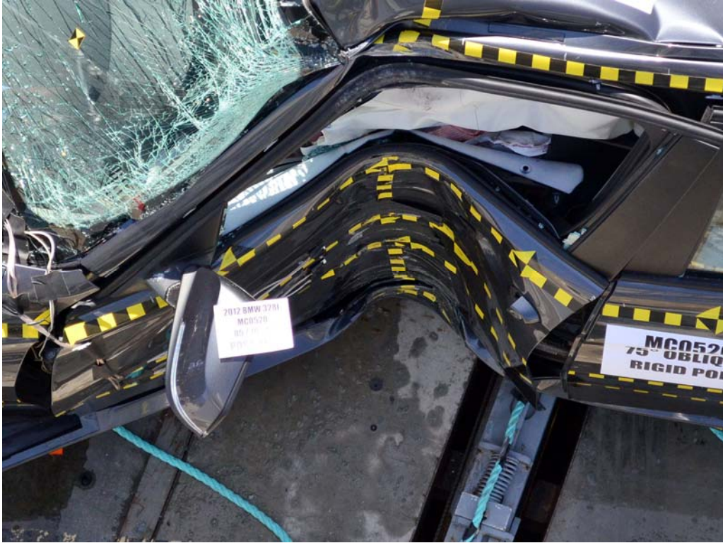
FIGURE 41. Post-Test Driver Dummy and Door Clearance
