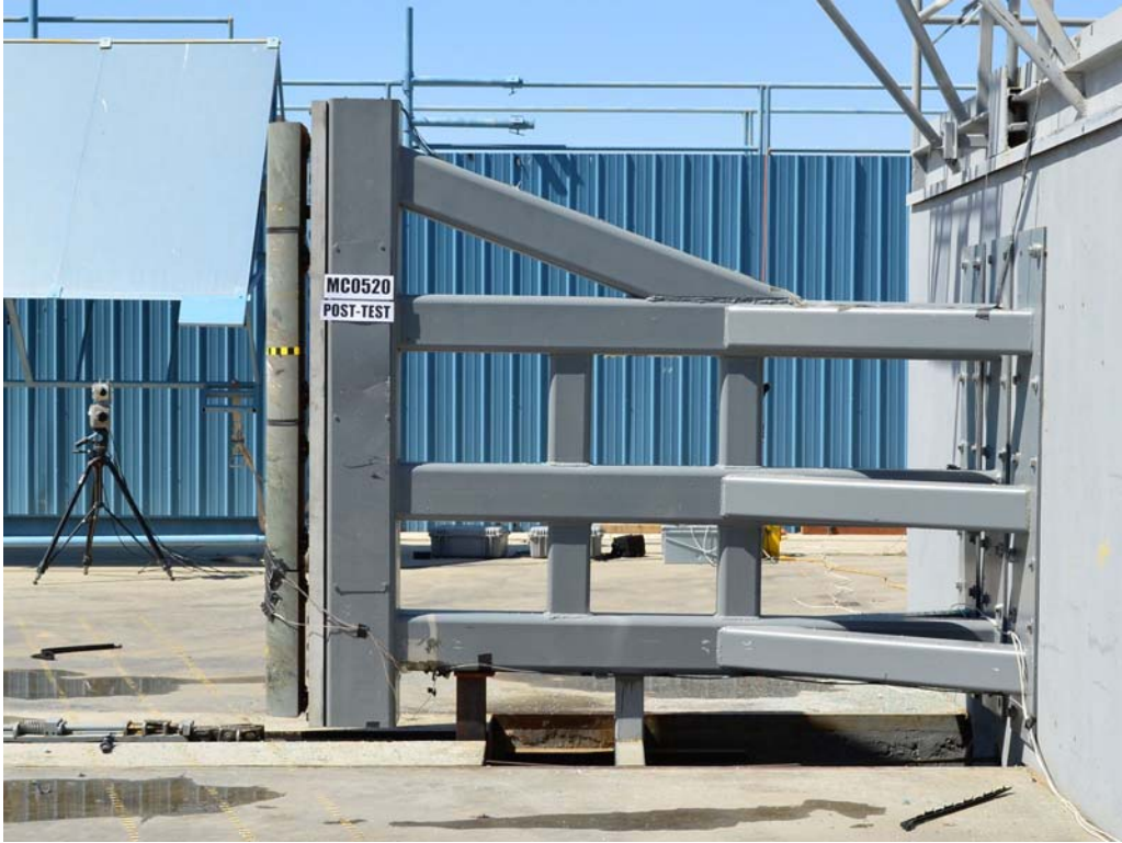
FIGURE 59. Post-Test Pole Barrier Side View
