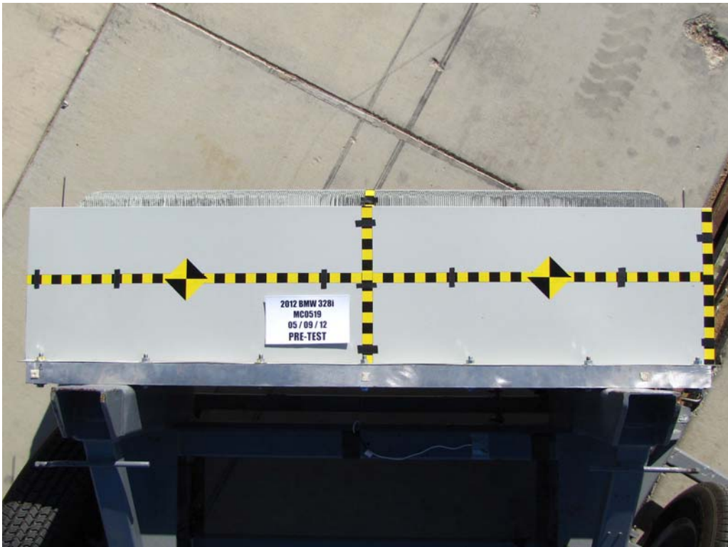
FIGURE 84. Pre-Test Top View of MDB Impactor Face
