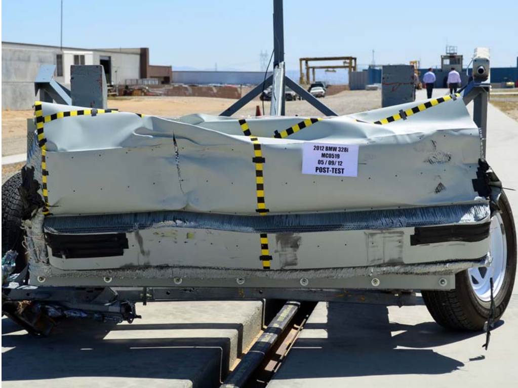
FIGURE 83. Post-Test Front View of MDB Impactor Face
