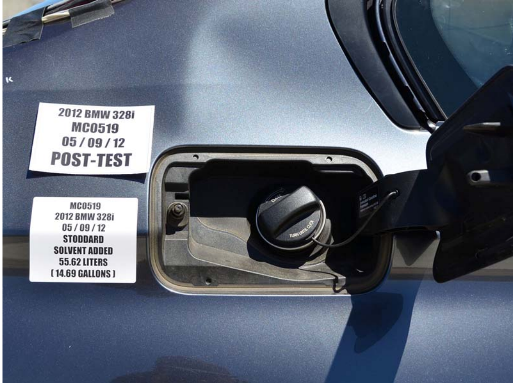
FIGURE 81. Post-Test View of Fuel Filler Neck
