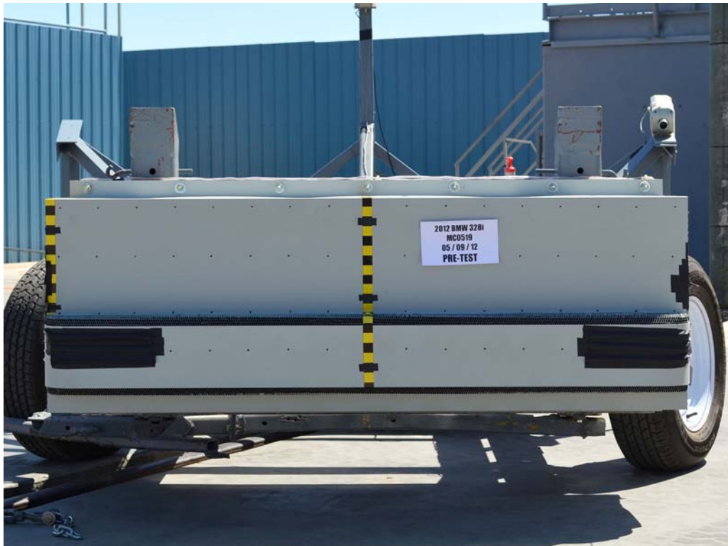
FIGURE 82. Pre-Test Front View of MDB Impactor Face
