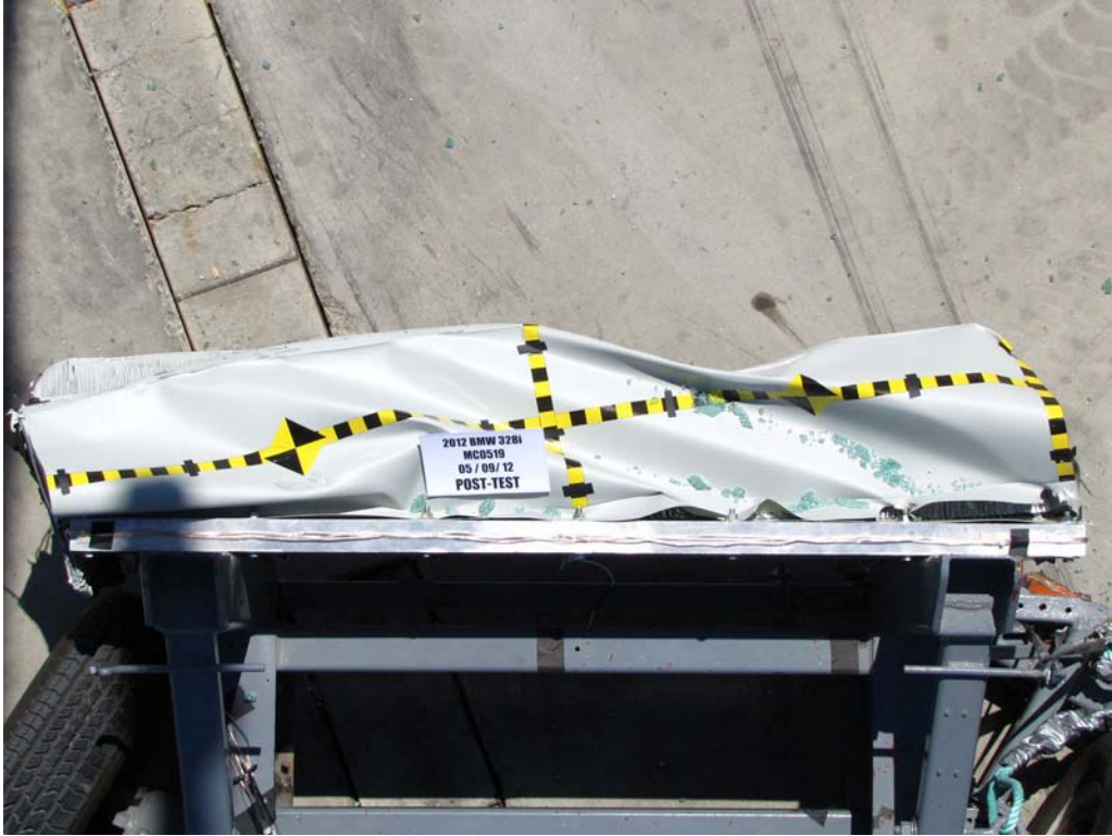
FIGURE 85. Post-Test Top View of MDB Impactor Face
