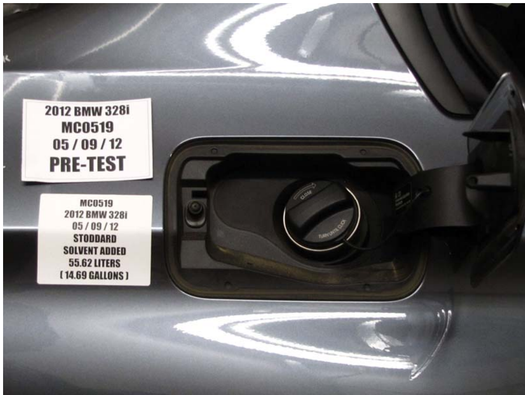
FIGURE 80. Pre-Test View of Fuel Filler Neck
