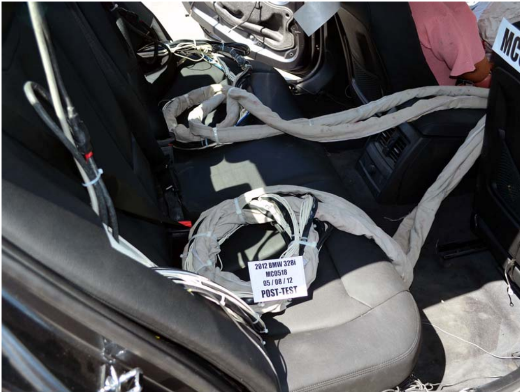
FIGURE 28. Post-Test Dummy Cable Routing
