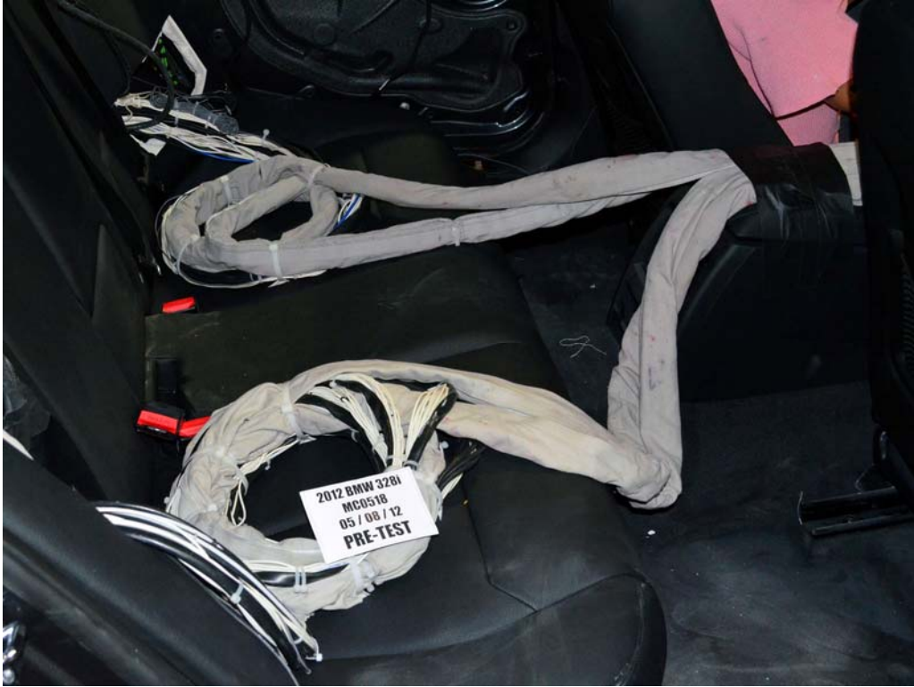
FIGURE 27. Pre-Test Dummy Cable Routing
