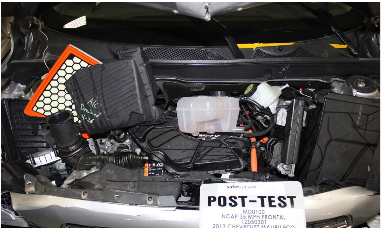
No. 017 Post-Impact View of Electric Propulsion Drive
