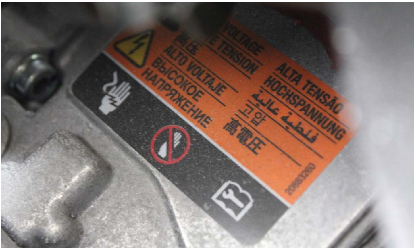
No. 005b Other Vehicle Label(s) Related to Electrical Propulsion System
