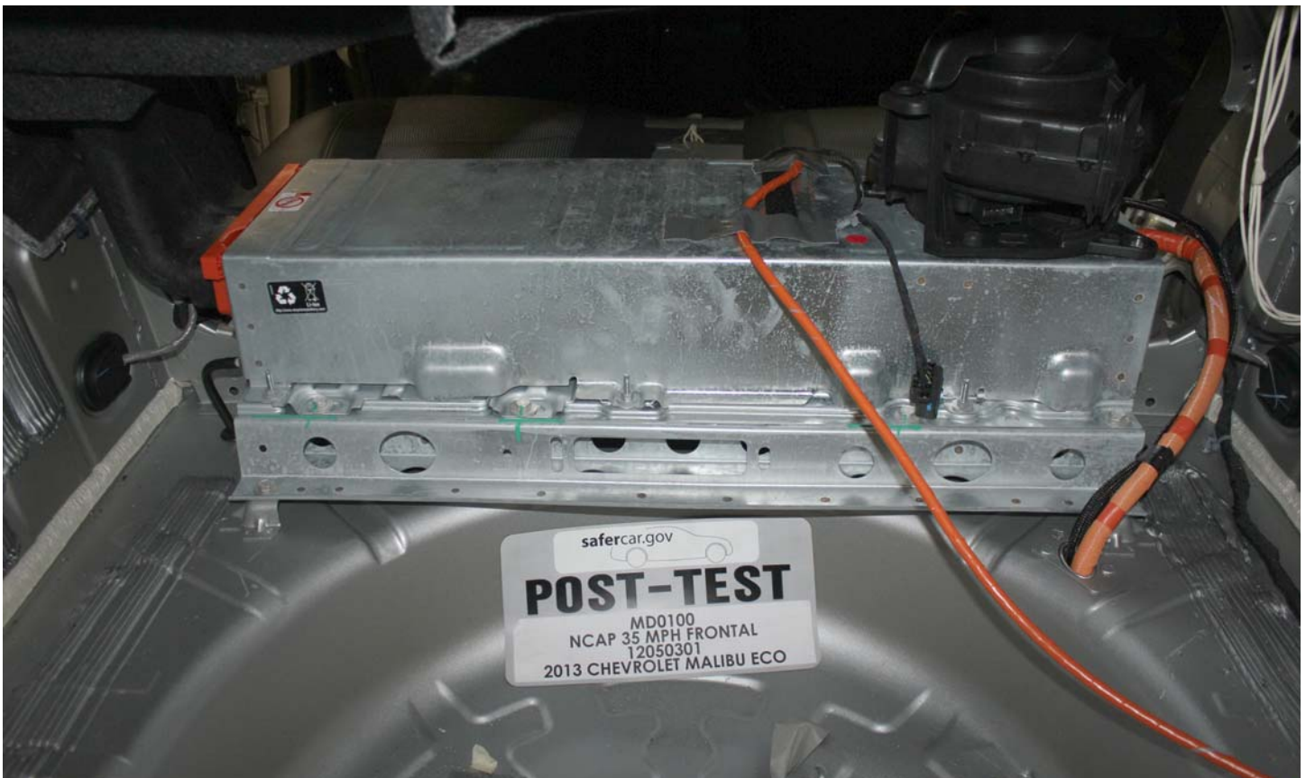
No. 011 Post-Impact Rear View of Propulsion Battery
