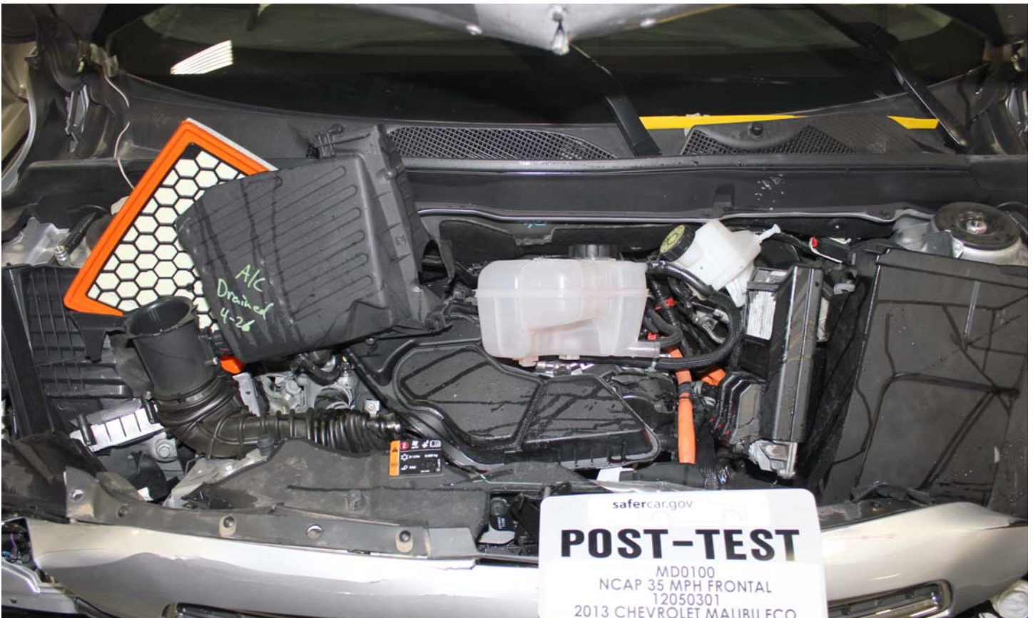
No. 008 Manual High Voltage Service Disconnect Removed
