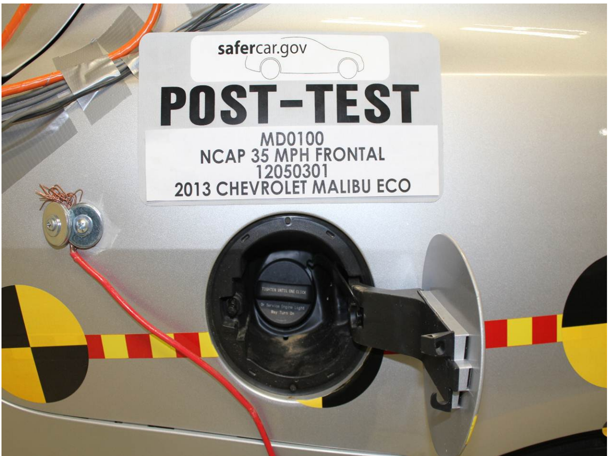
Post-Test Fuel Filler Cap View
