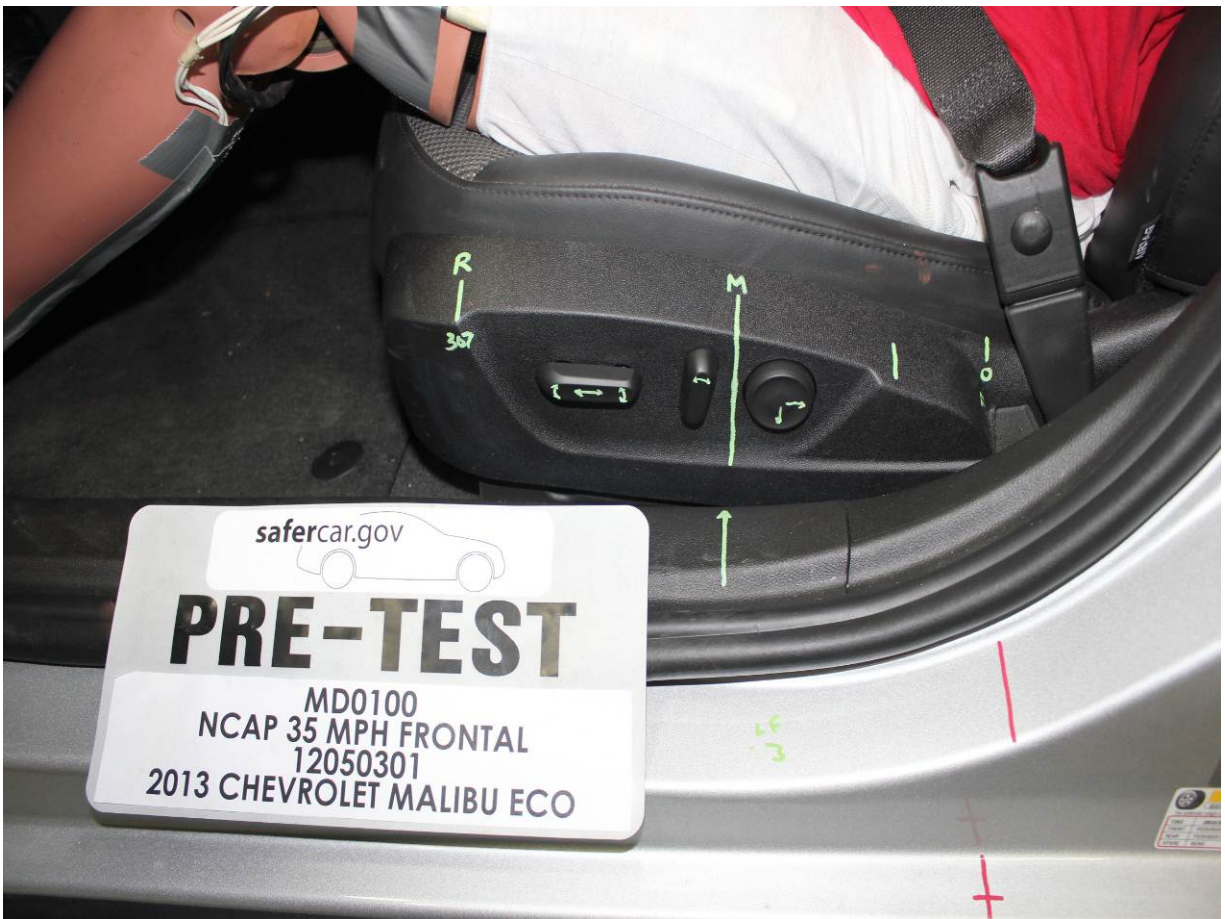
Pre-Test Driver's Seat Fore-Aft Markings
