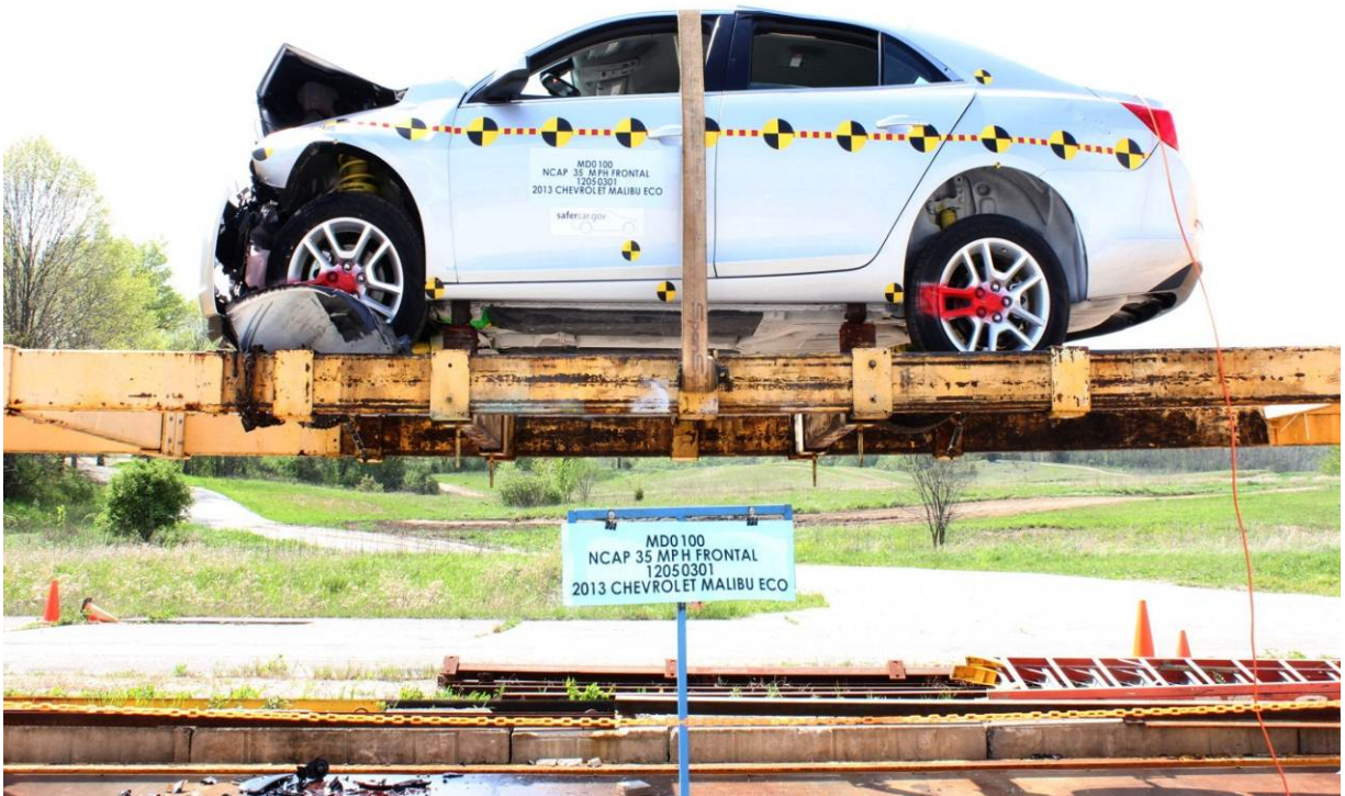
Vehicle at 360 Degrees on Static Rollover Device
