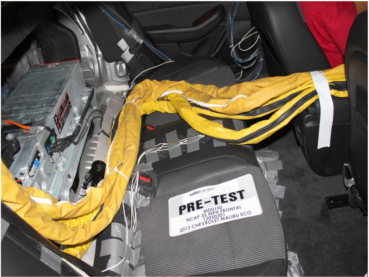
Pre-Test Dummy Cable Routing
