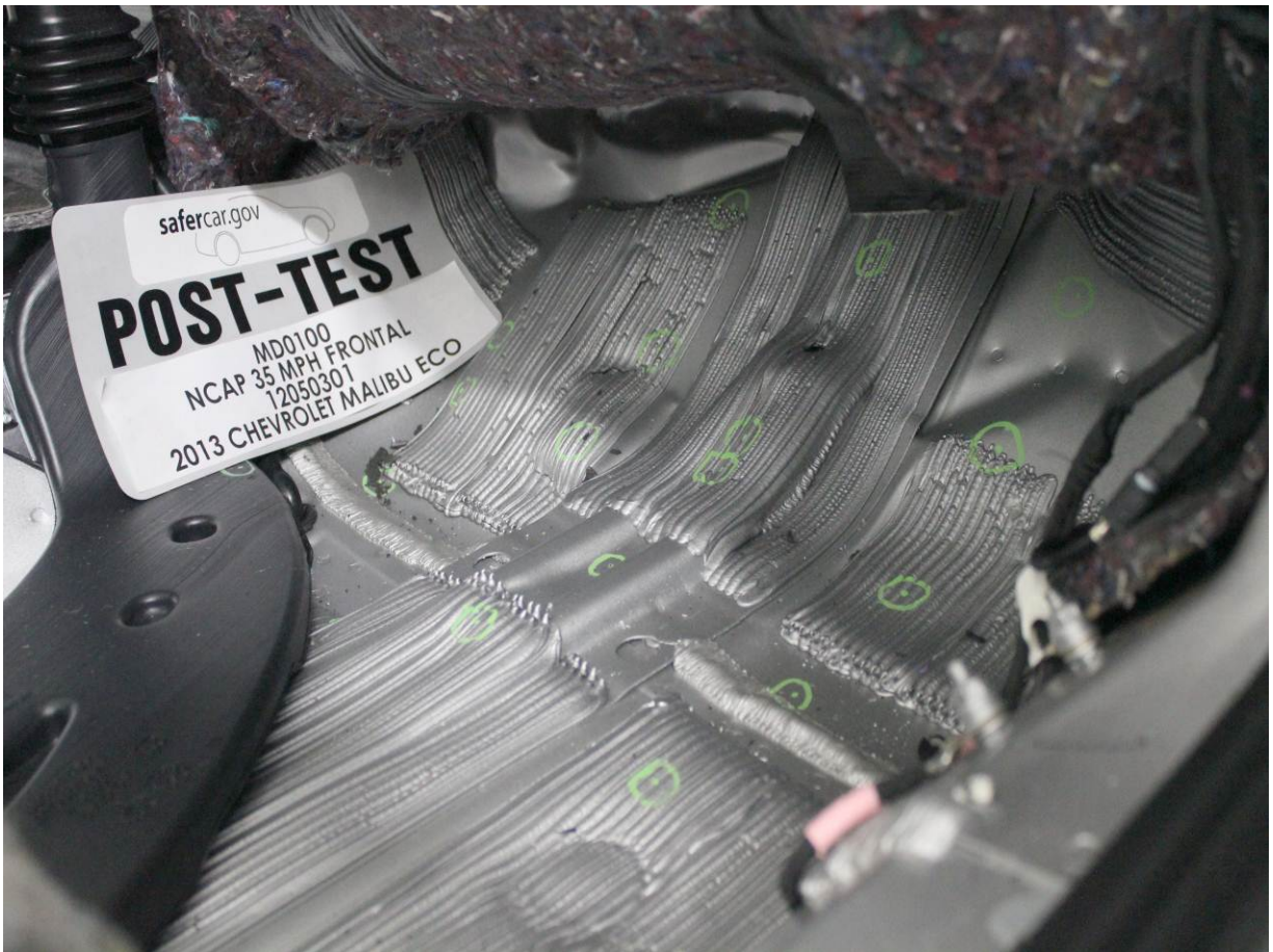
Post-Test Passenger's Side Floorpan
