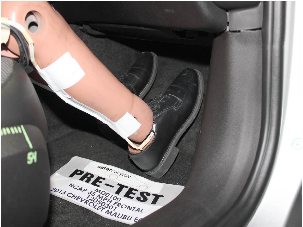
Pre-Test Passenger Dummy Feet
