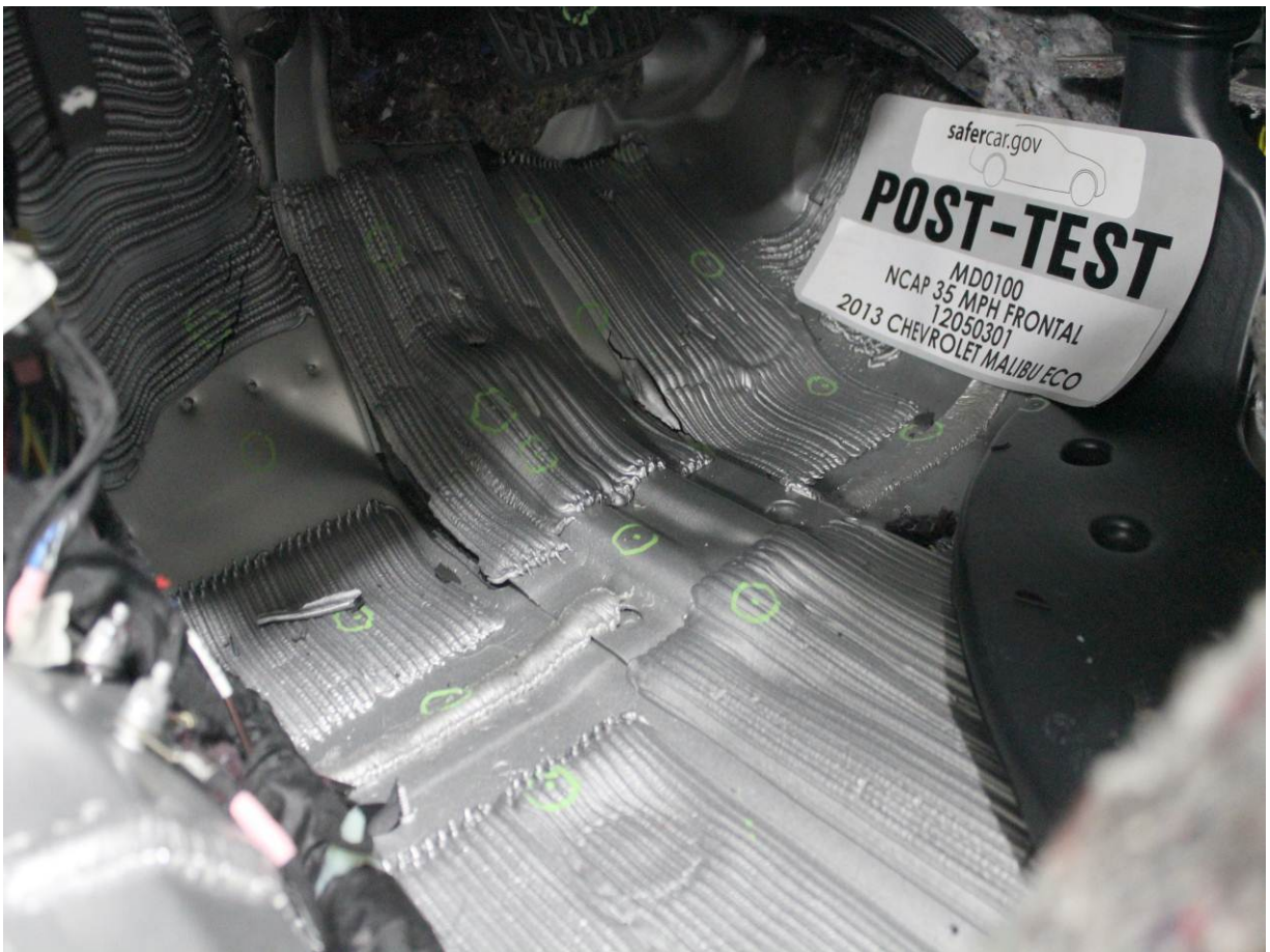
Post-Test Driver's Side Floorpan
