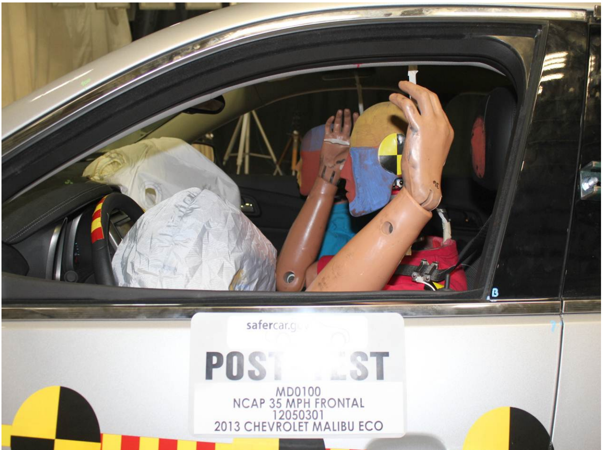
Post-Test Driver Dummy Window View
