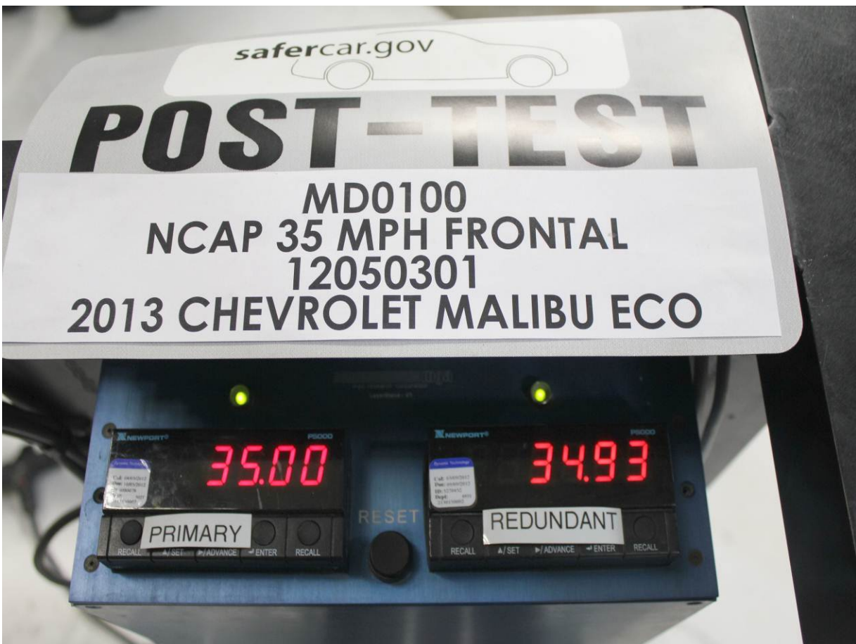
Post-Test Speed Trap Read-Out
