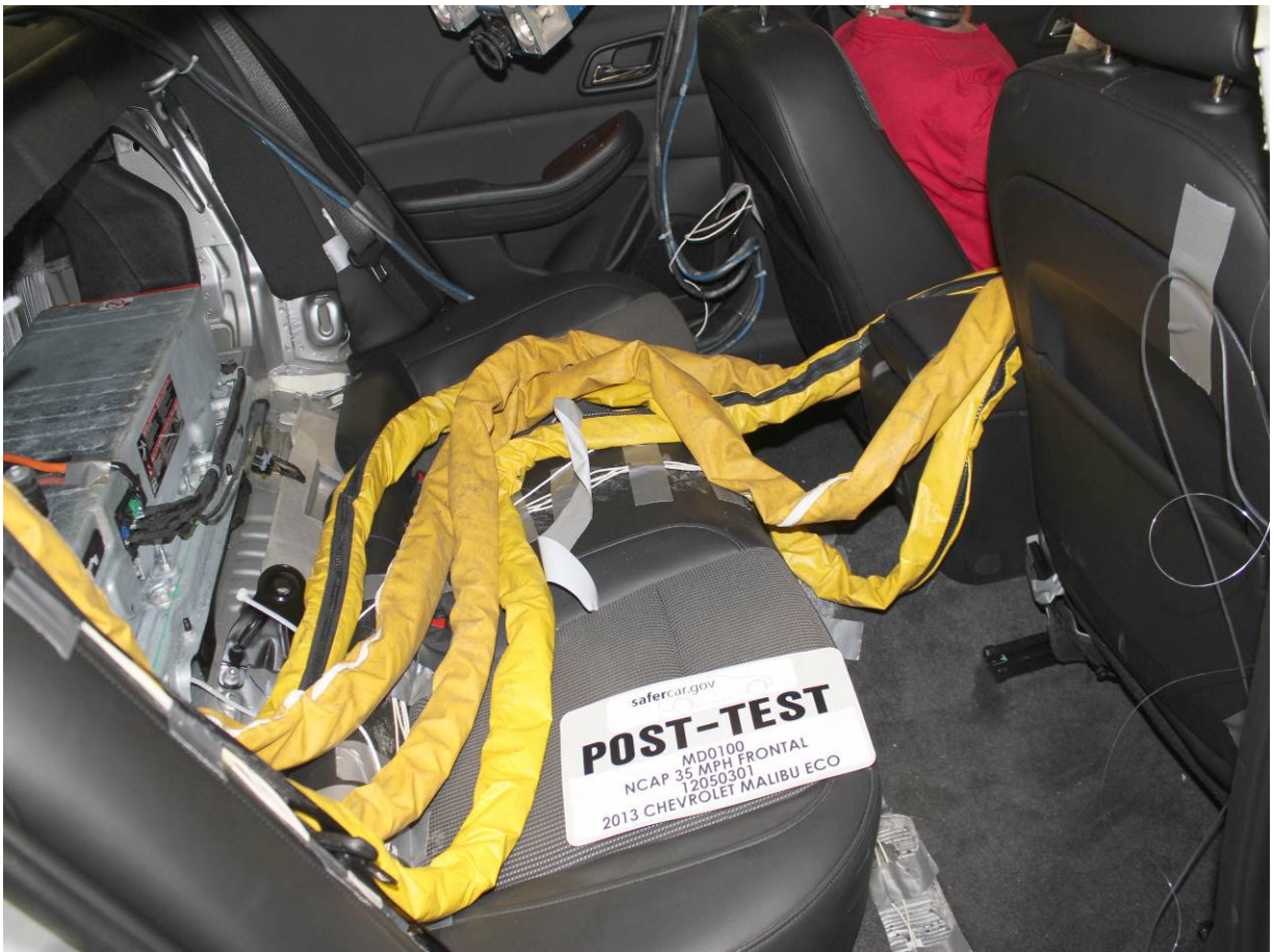
Post-Test Dummy Cable Routing
