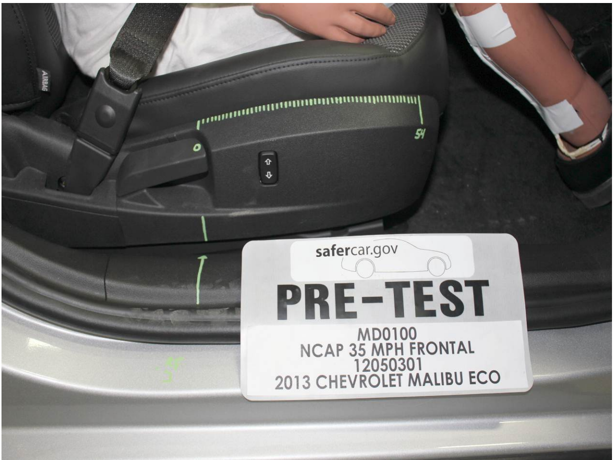
Pre-Test Passenger's Seat Fore-Aft Markings
