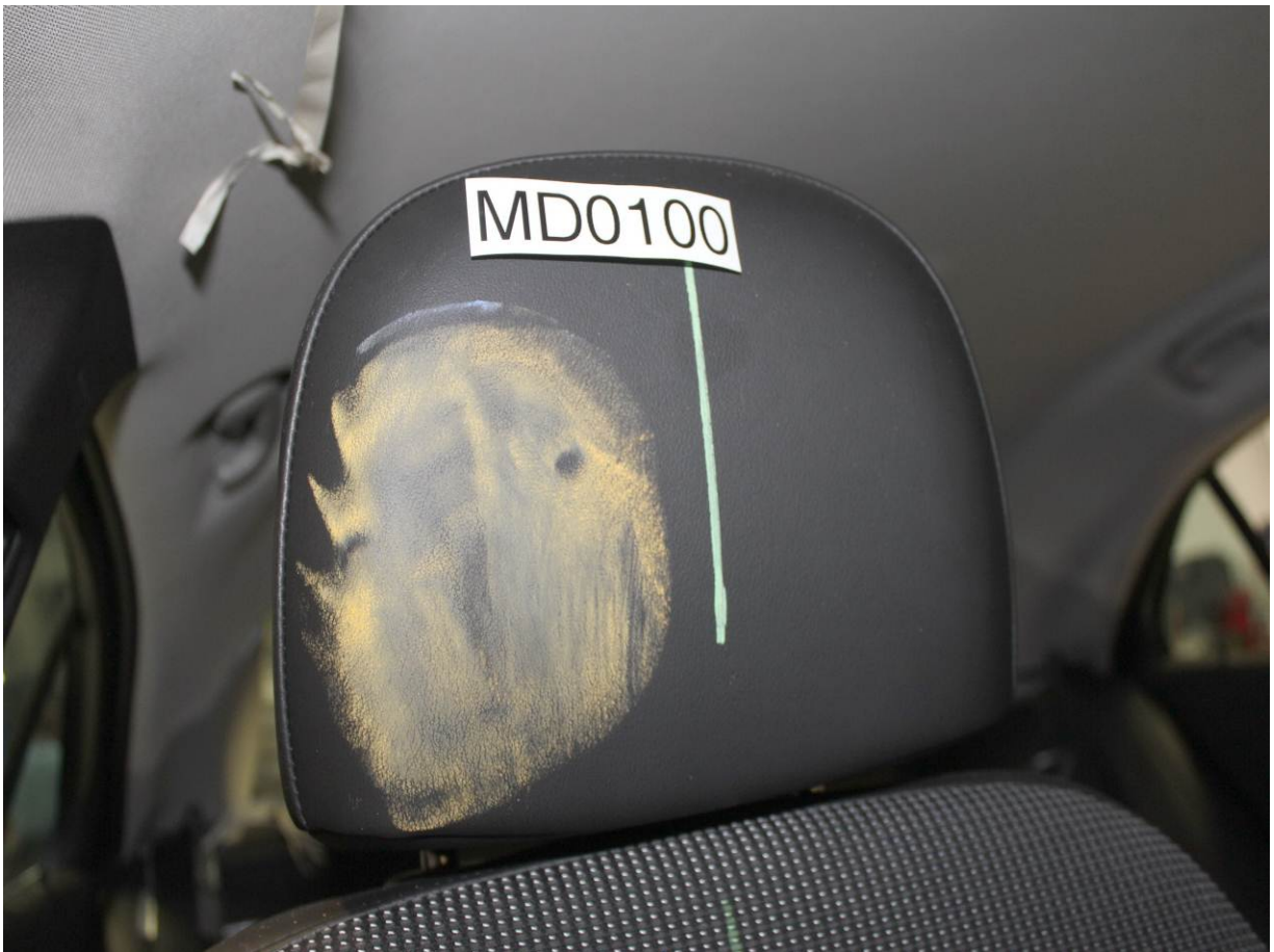
Post-Test Passenger Dummy Contact with Headrest
