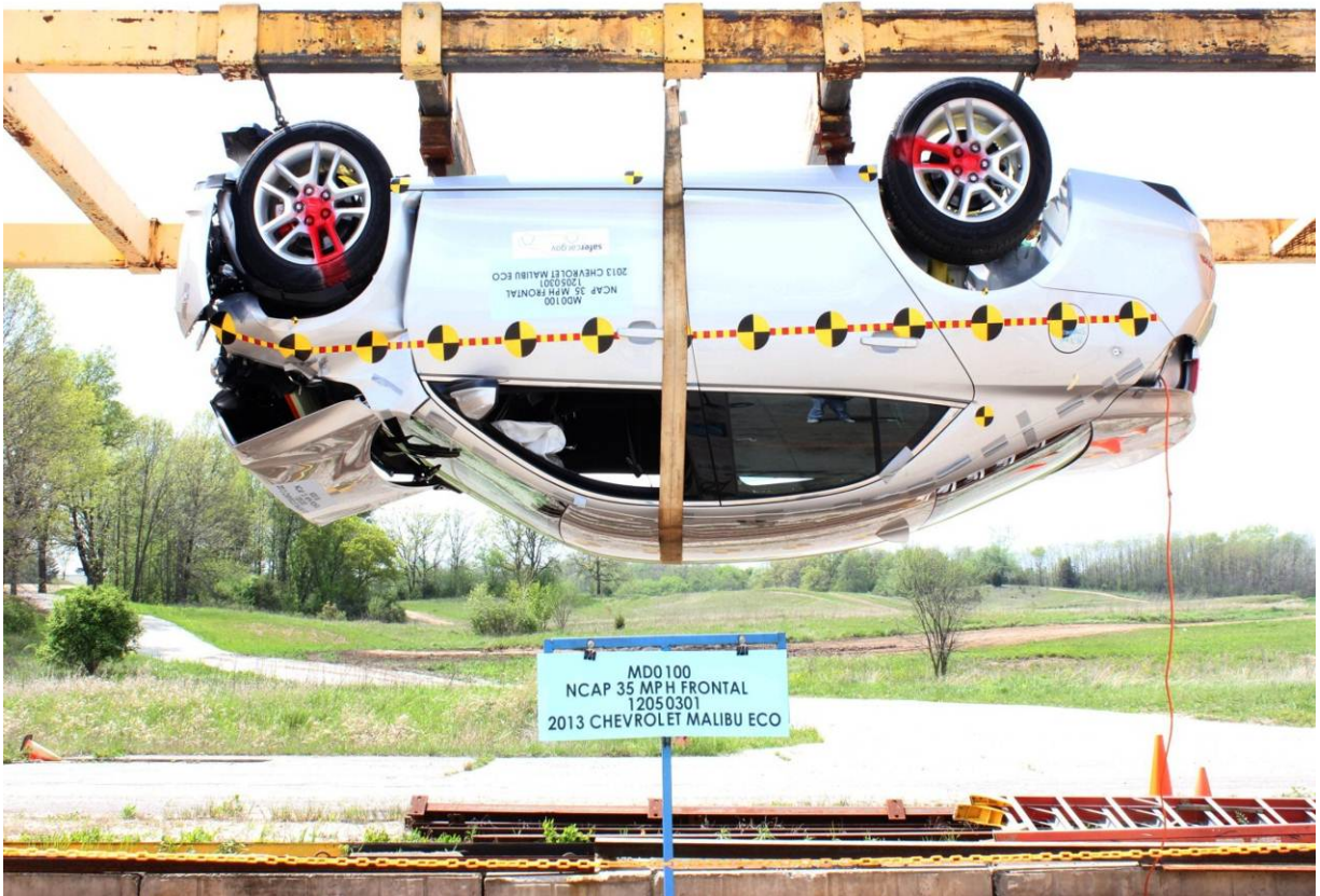
Vehicle at 180 Degrees on Static Rollover Device
