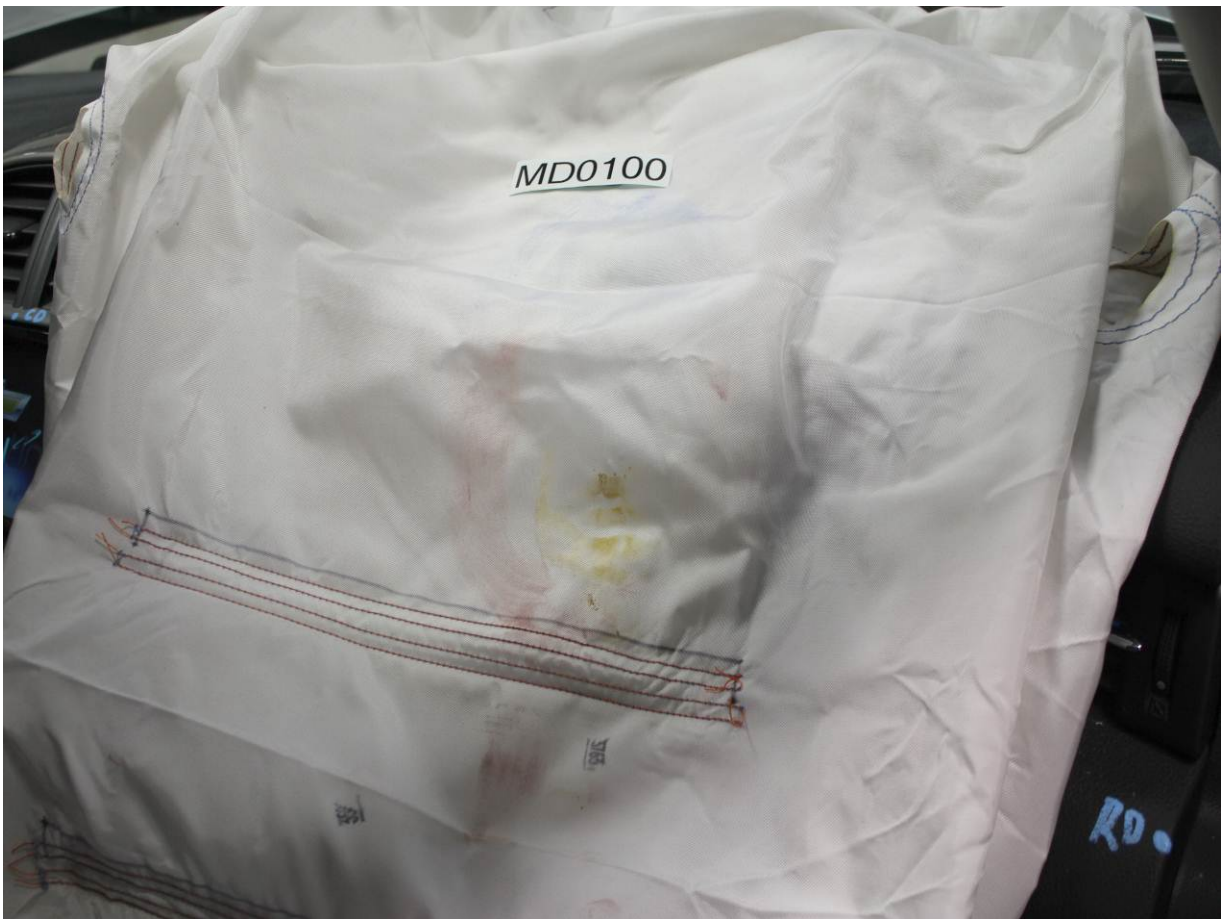
Post-Test Passenger Dummy Contact with Airbag
