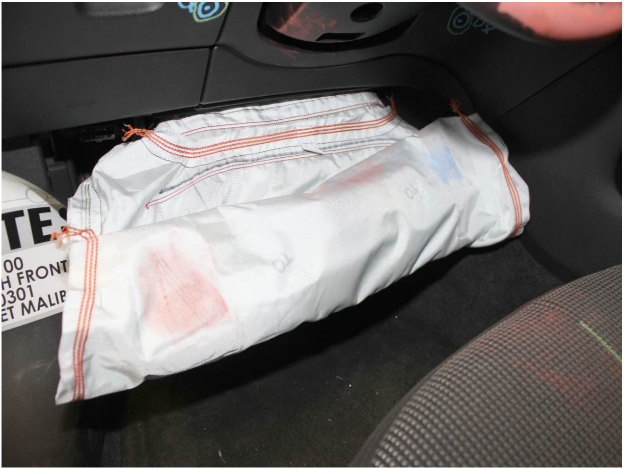
Post-Test Driver Dummy Contact with Knee Airbag
