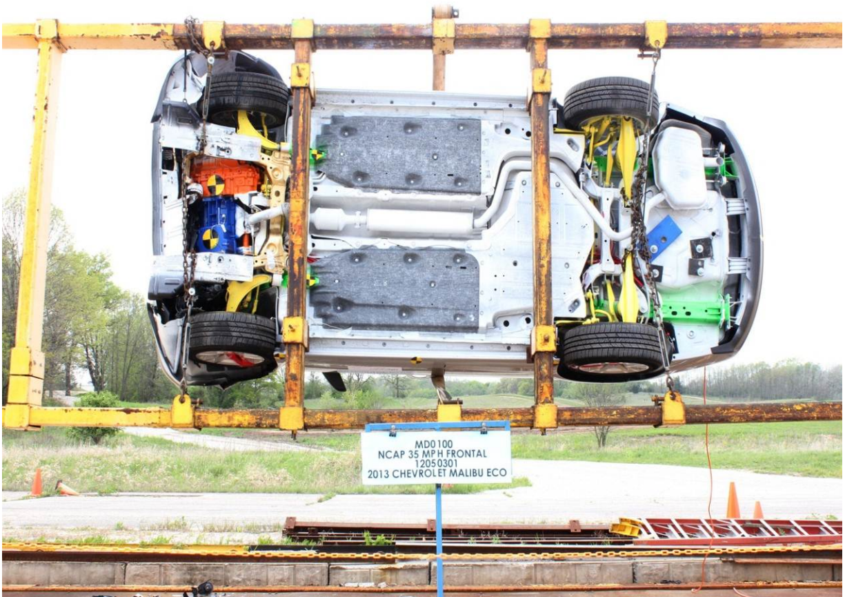
Vehicle at 90 Degrees on Static Rollover Device
