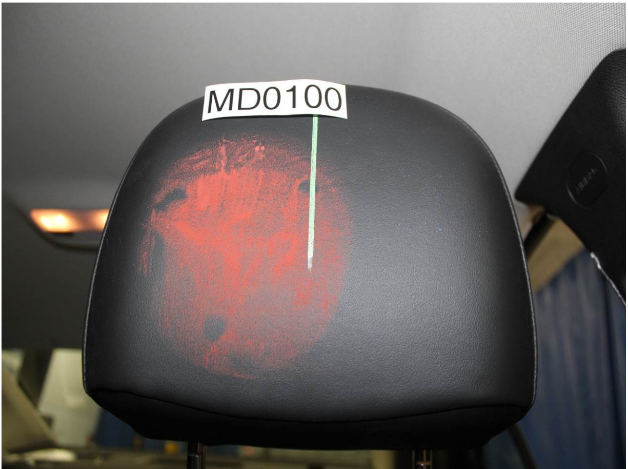
Post-Test Driver Dummy Contact with Headrest
