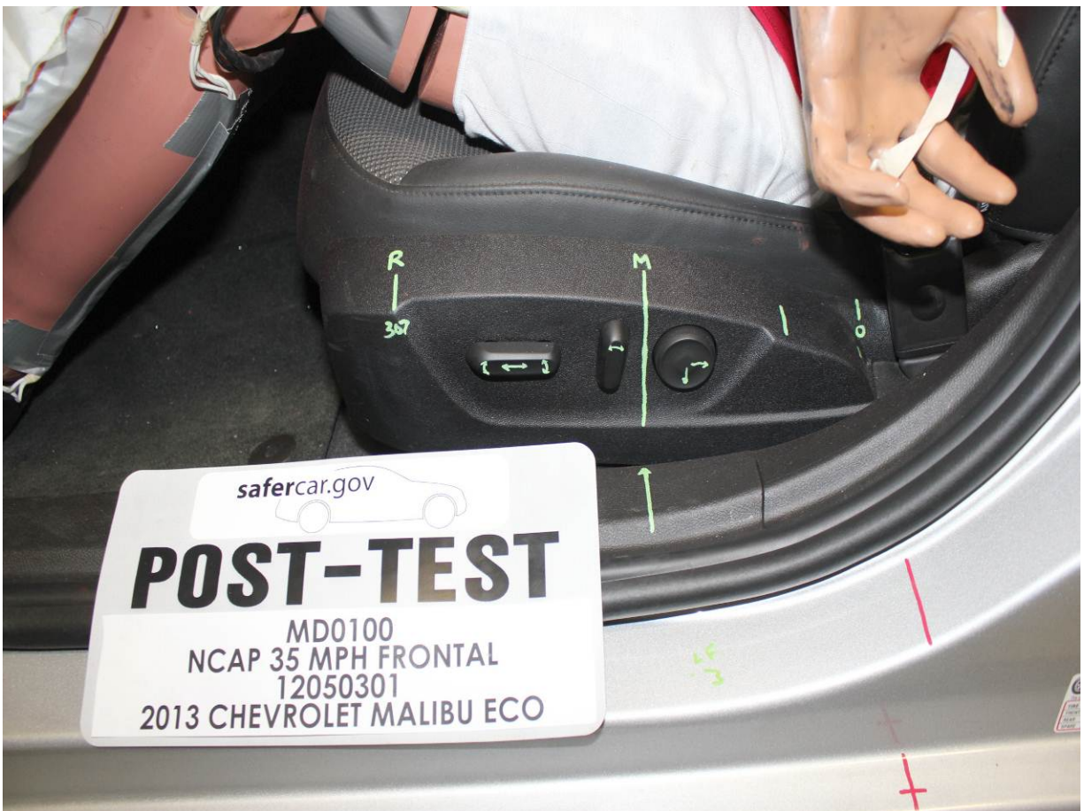
Post-Test Driver's Seat Fore-Aft Markings
