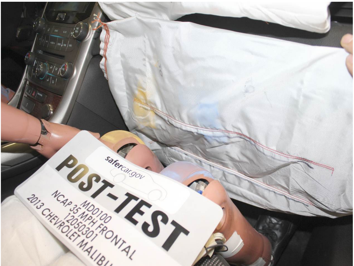
Post-Test Passenger Dummy Contact with Knee Airbag
