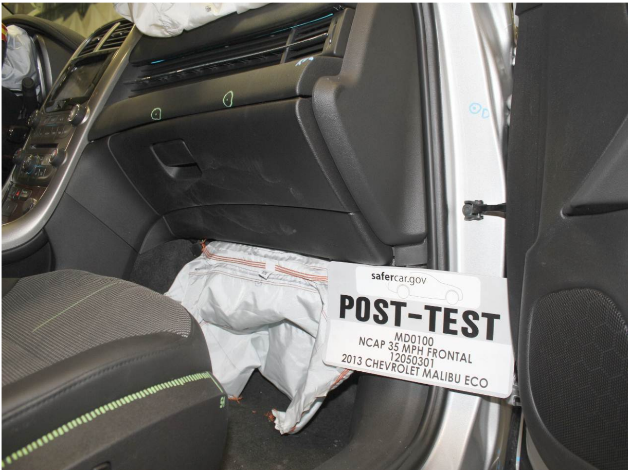
Post-Test Passenger's Side Knee Bolster (without dummy)
