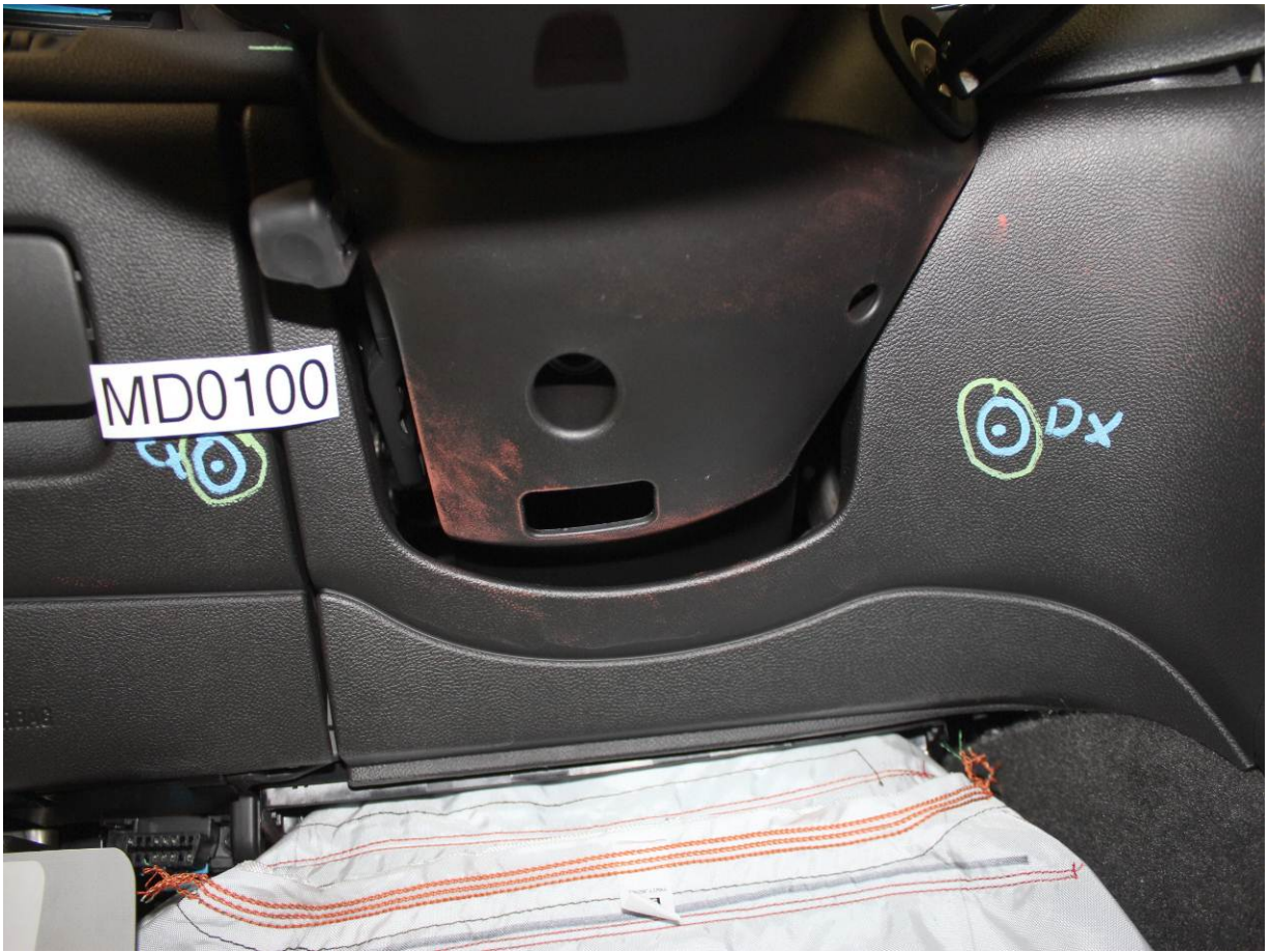
Post-Test Driver's Side Knee Bolster (without dummy)
