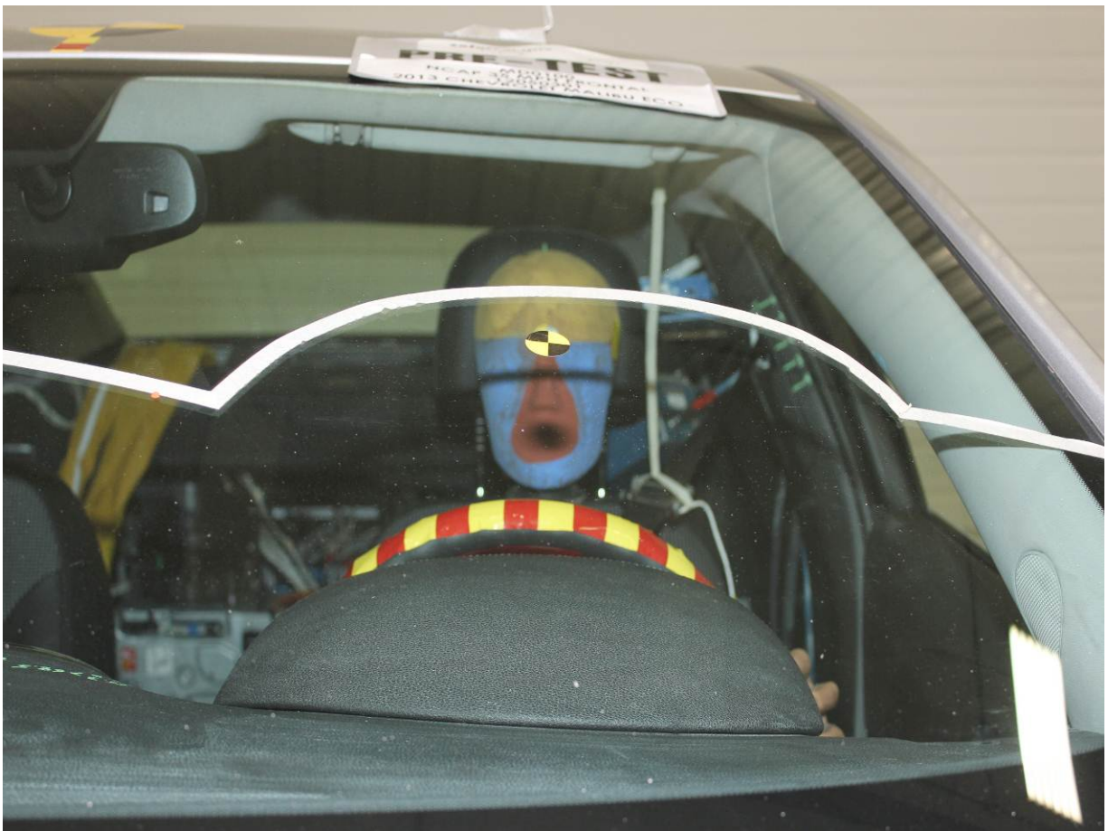
Pre-Test Driver Dummy Front View
