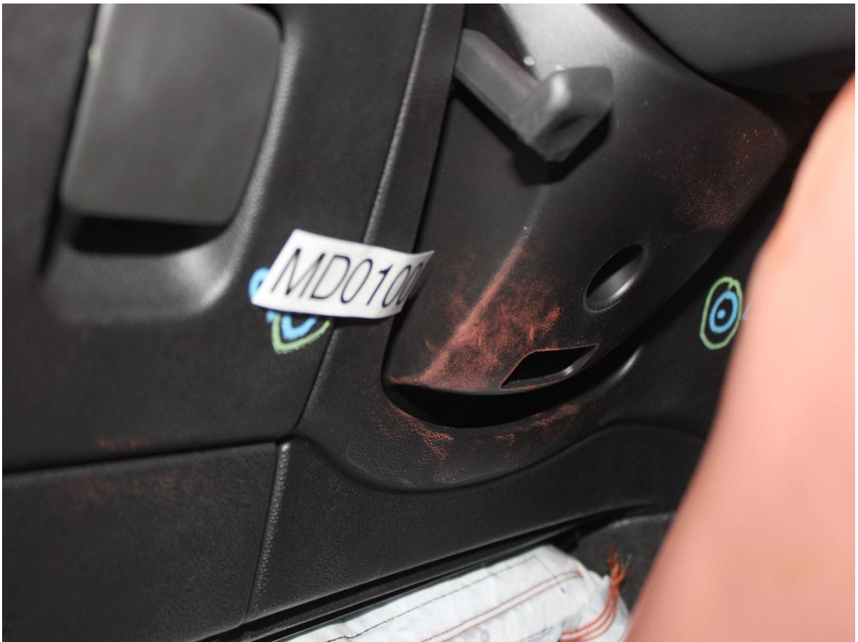
Post-Test Driver Dummy Contact with Steering Column
