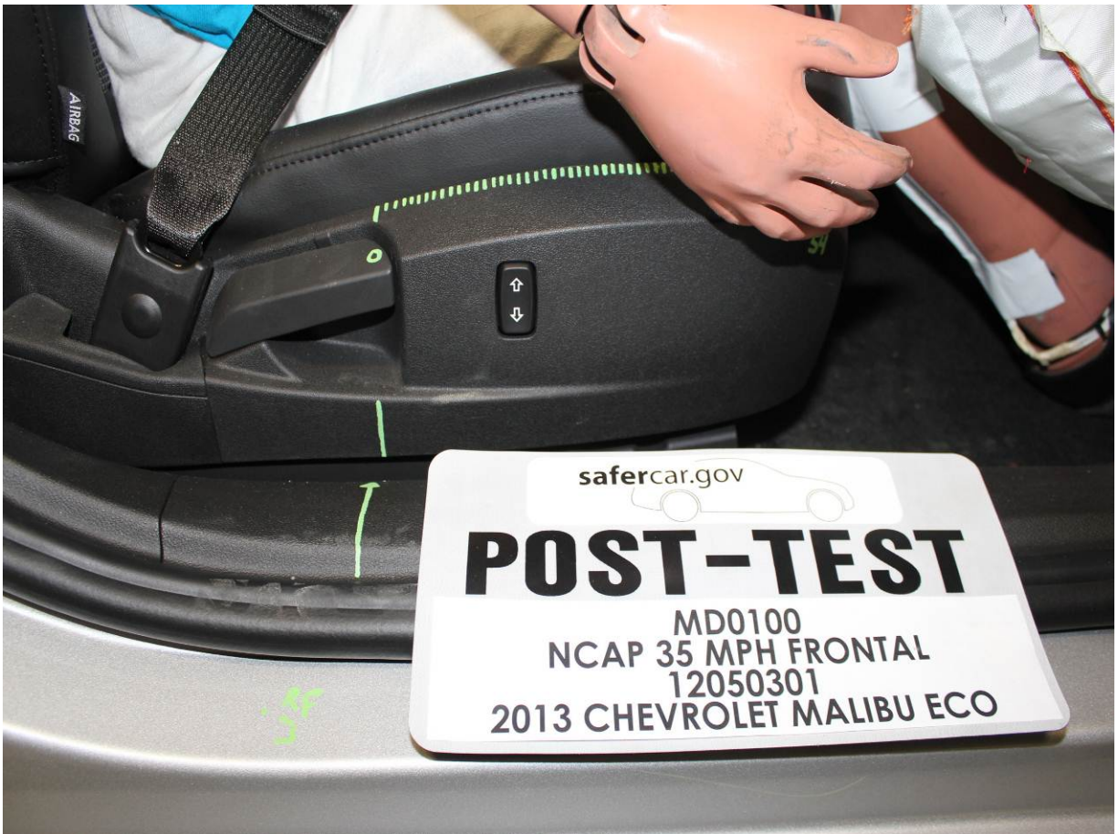
Post-Test Passenger's Seat Fore-Aft Markings
