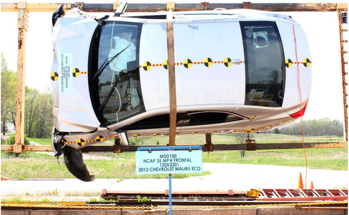
Vehicle at 270 Degrees on Static Rollover Device
