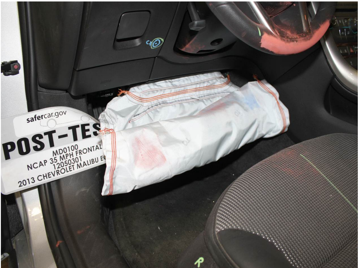
Post-Test Driver's Side Knee Bolster (without dummy)
