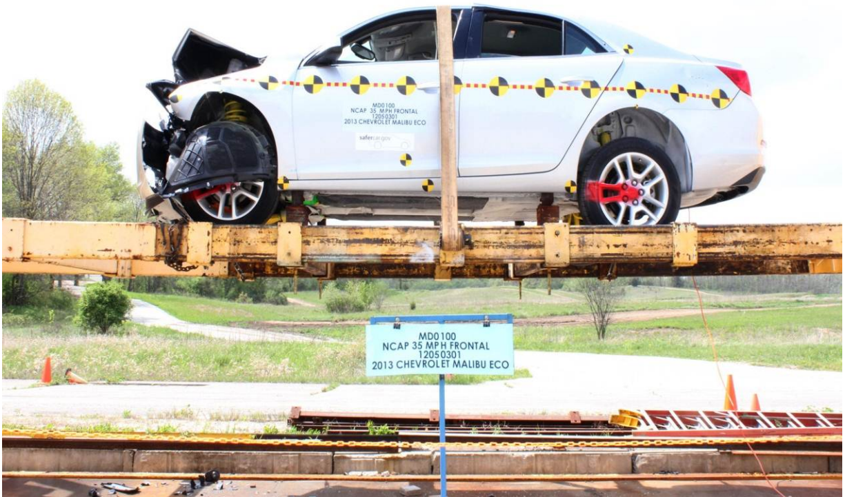
Vehicle at 0 Degrees on Static Rollover Device
