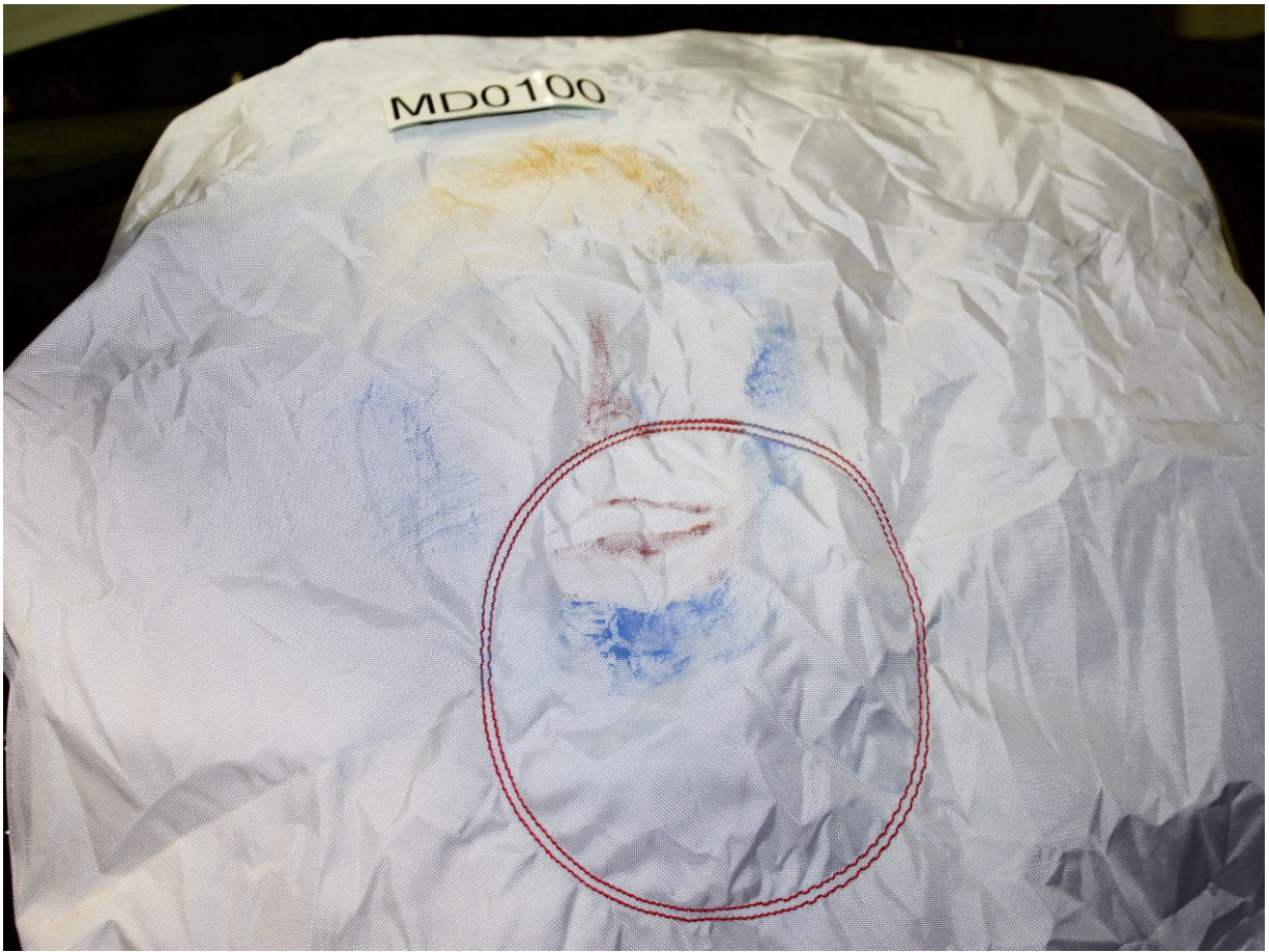
Post-Test Driver Dummy Contact with Airbag
