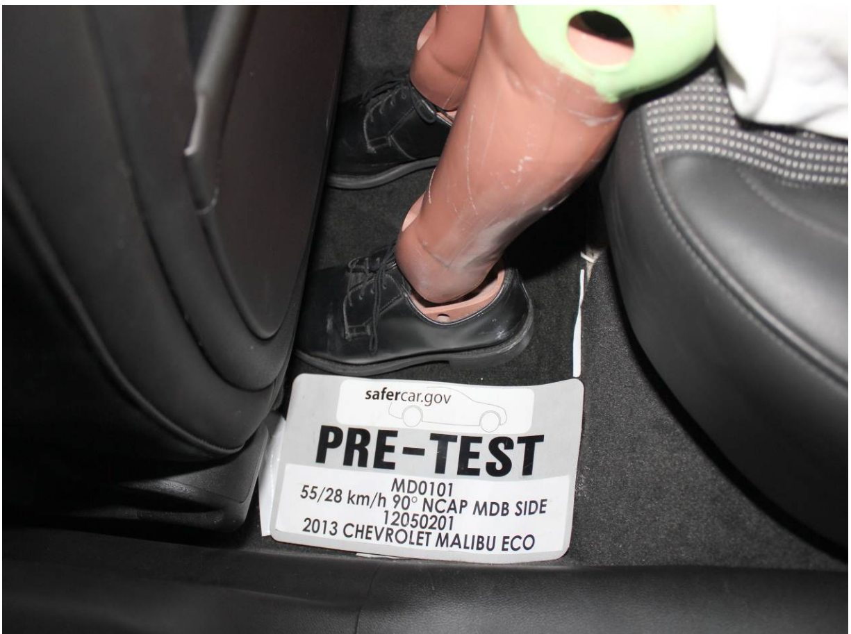
Pre-Test Placement of Rear Passenger Dummy's Feet
