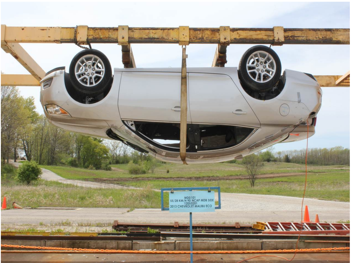
FMVSS No. 301 Static Rollover 180 Degrees
