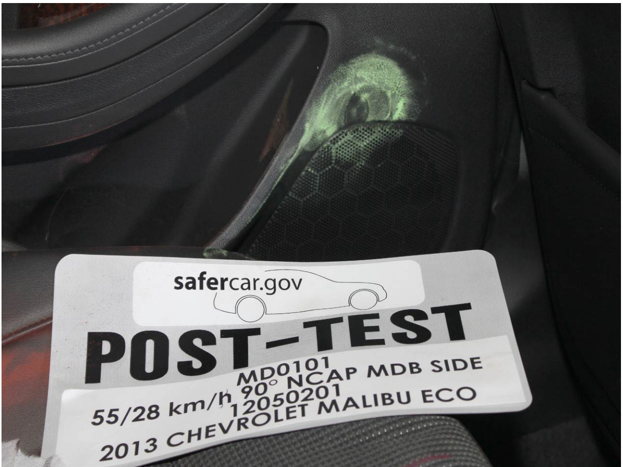
Post-Test Driver Rear Passenger Knee Contact with Vehicle Interior View
