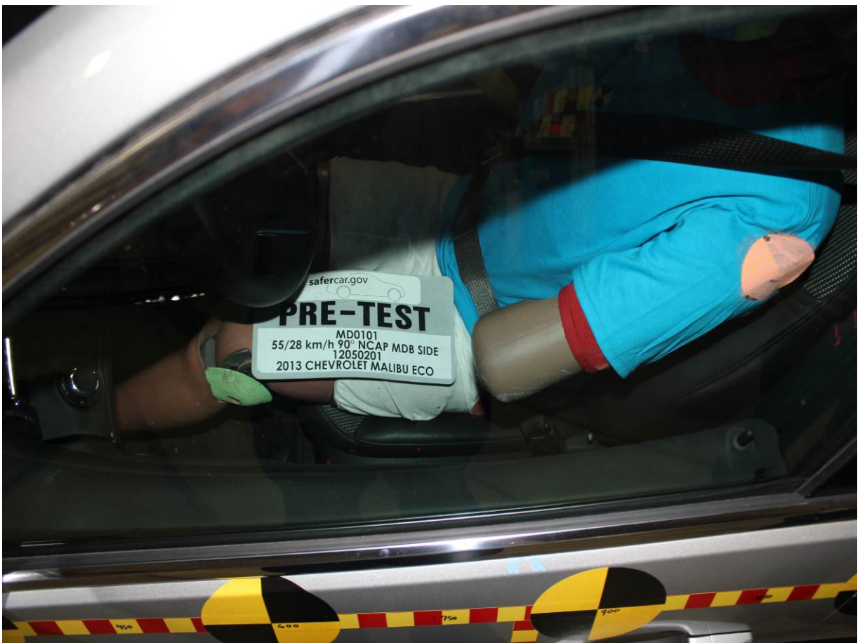
Pre-Test Driver Dummy and Door Clearance View
