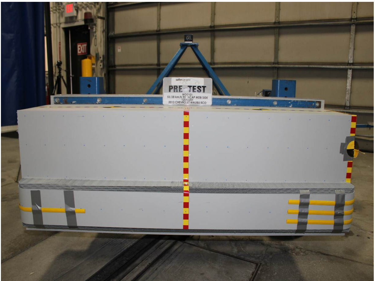
Pre-Test Front View of MDB Impactor Face
