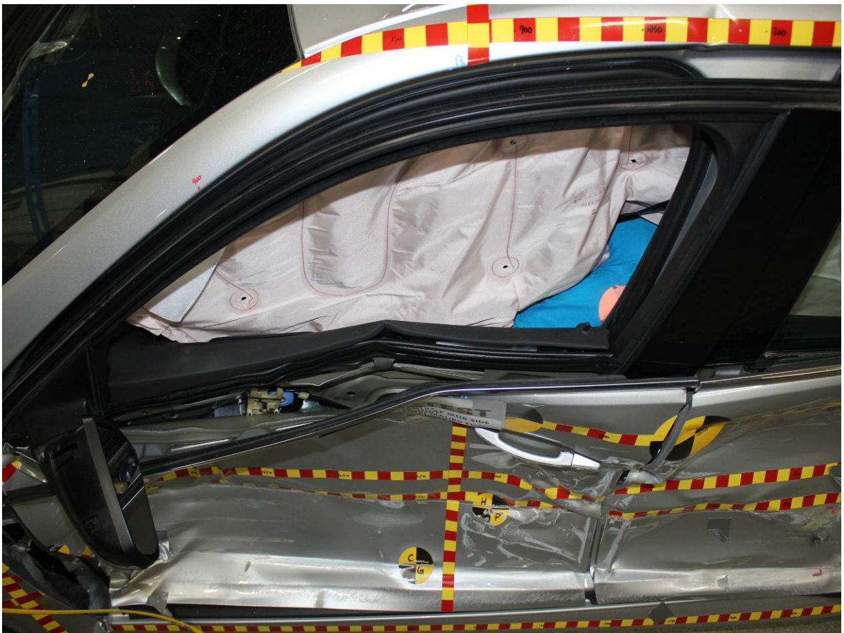
Post-Test Driver Dummy and Door Clearance View
