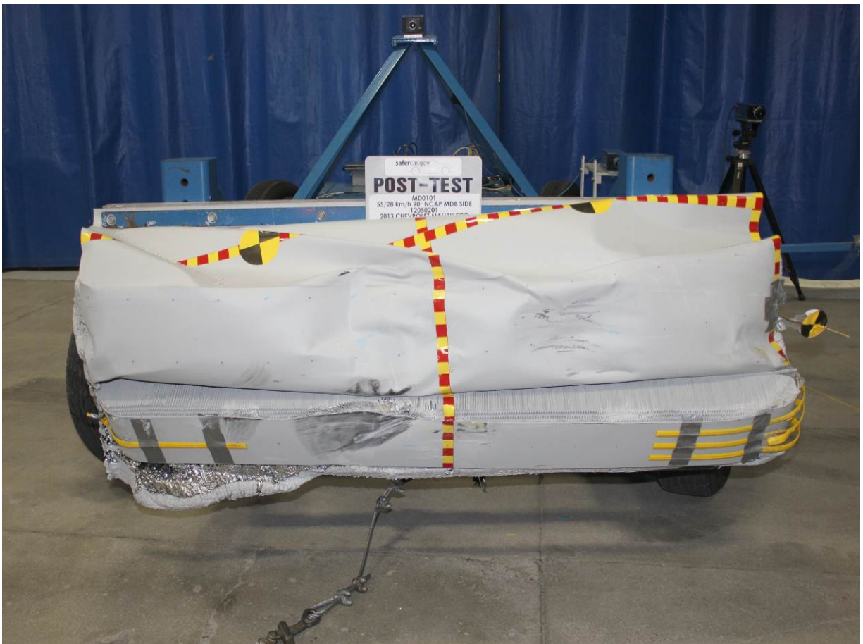
Post-Test Front View of MDB Impactor Face
