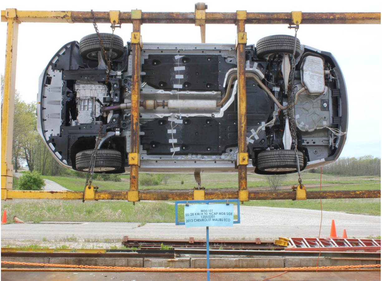
FMVSS No. 301 Static Rollover 90 Degrees
