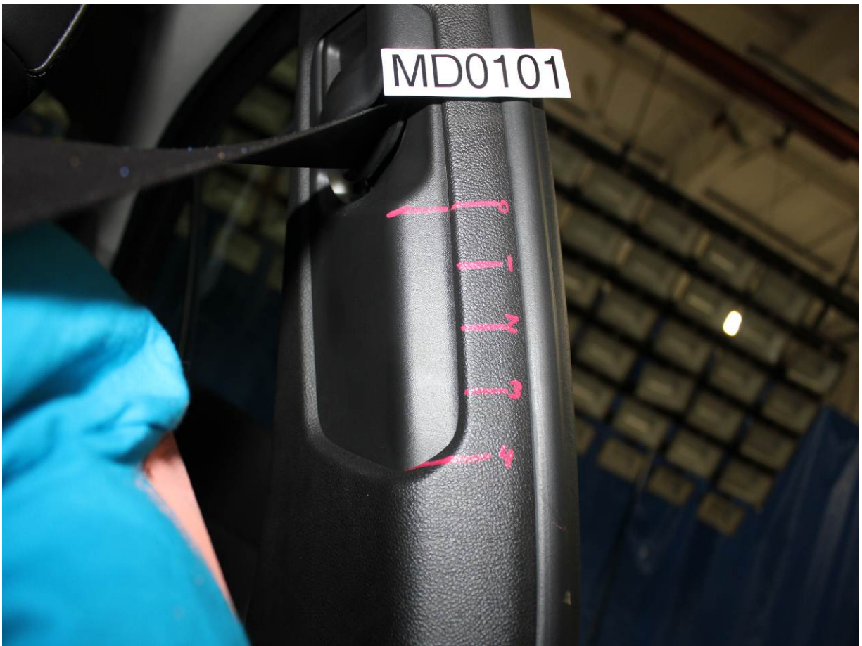
Pre-Test View of Belt Anchorage for Driver Dummy
