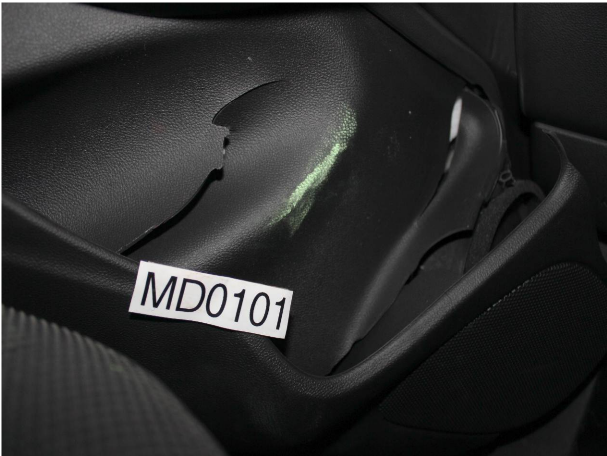
Post-Test Driver Dummy Knee Contact with Vehicle Interior View
