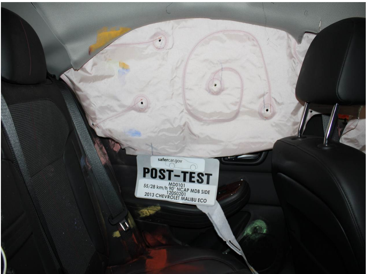
Post-Test Rear Passenger Inner Door Panel View
