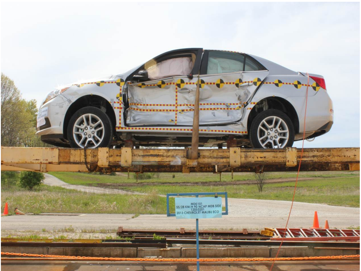
FMVSS No. 301 Static Rollover 360 Degrees
