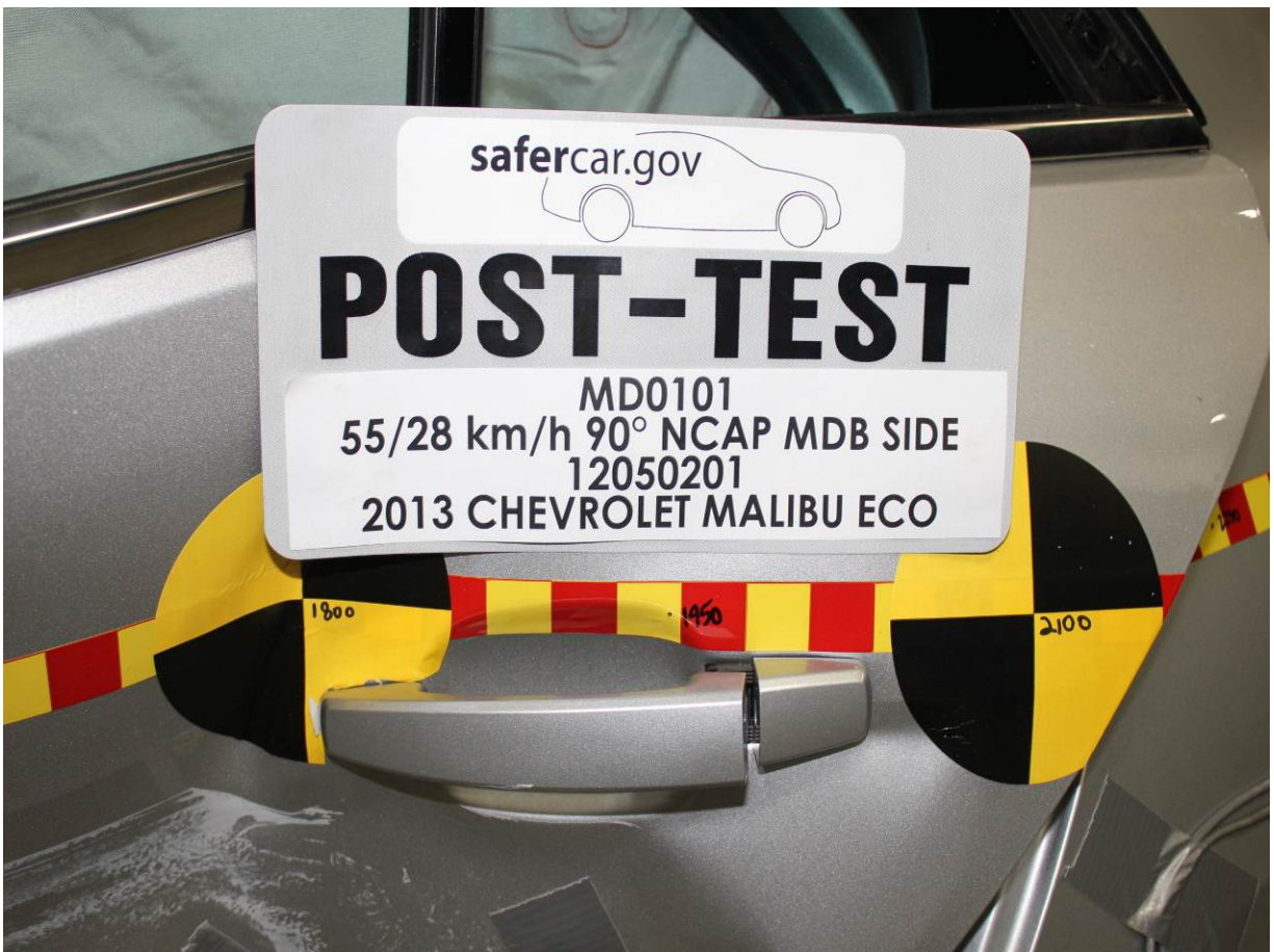
Post-Test Left Rear Door Latch Close-Up
