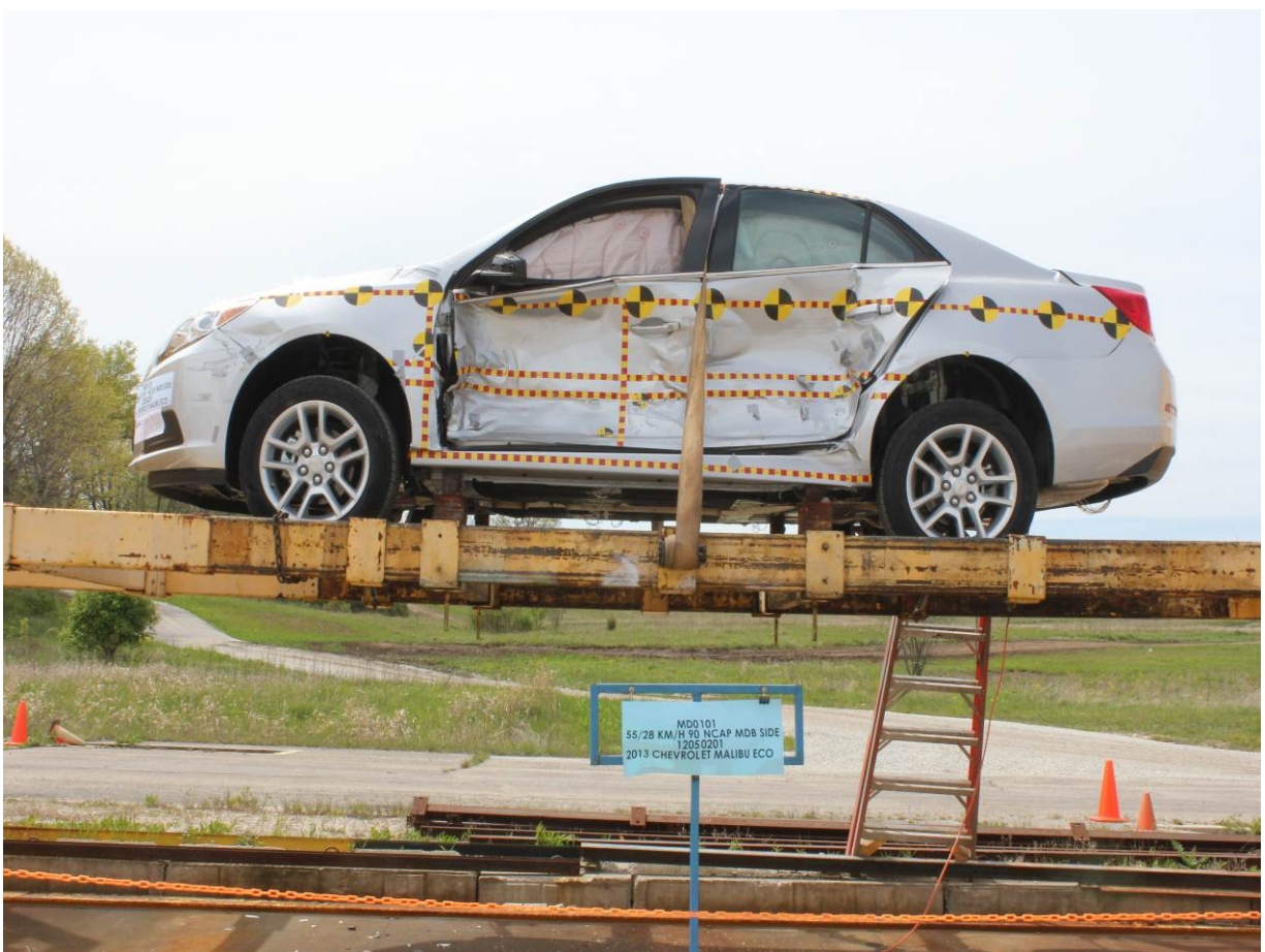
FMVSS No. 301 Static Rollover 0 Degrees
