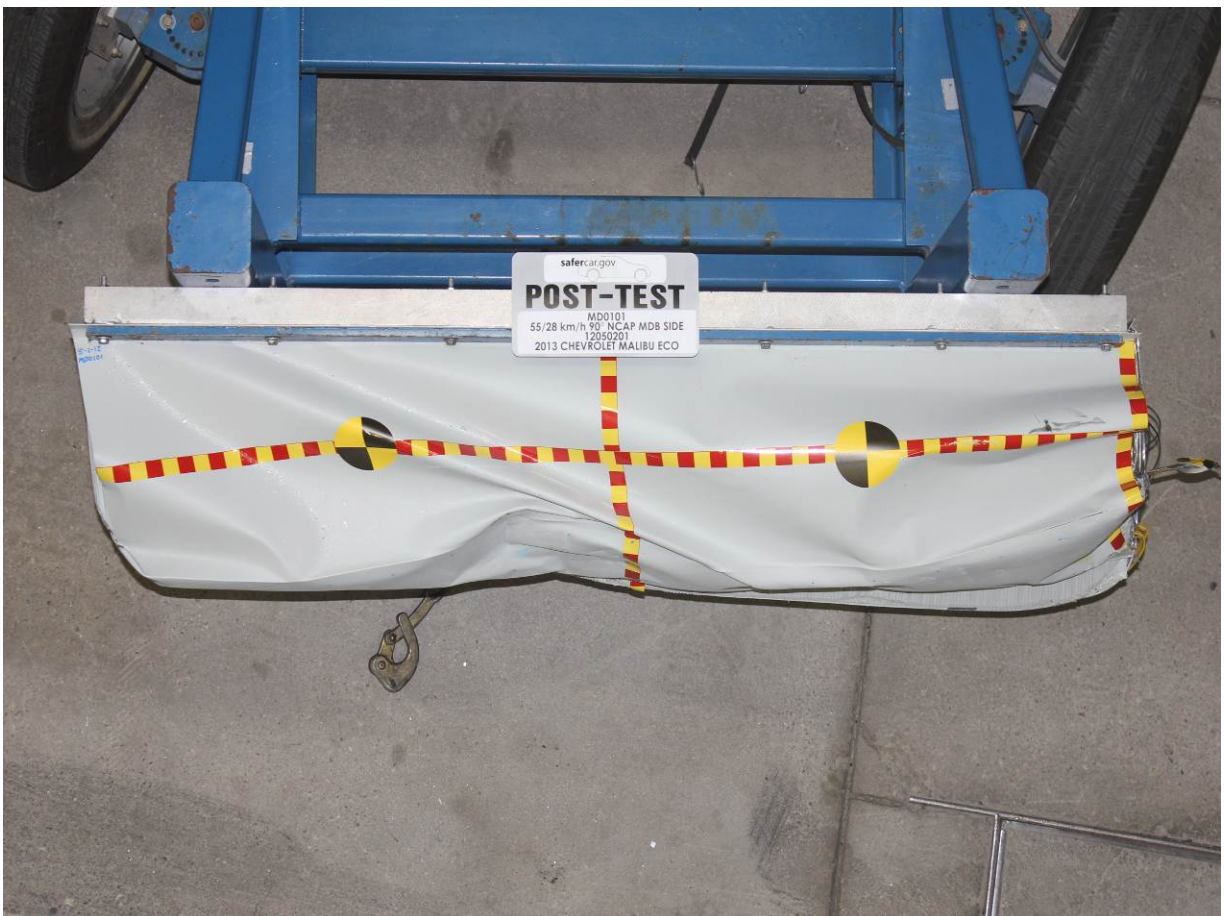
Post-Test Top View of MDB Impactor Face
