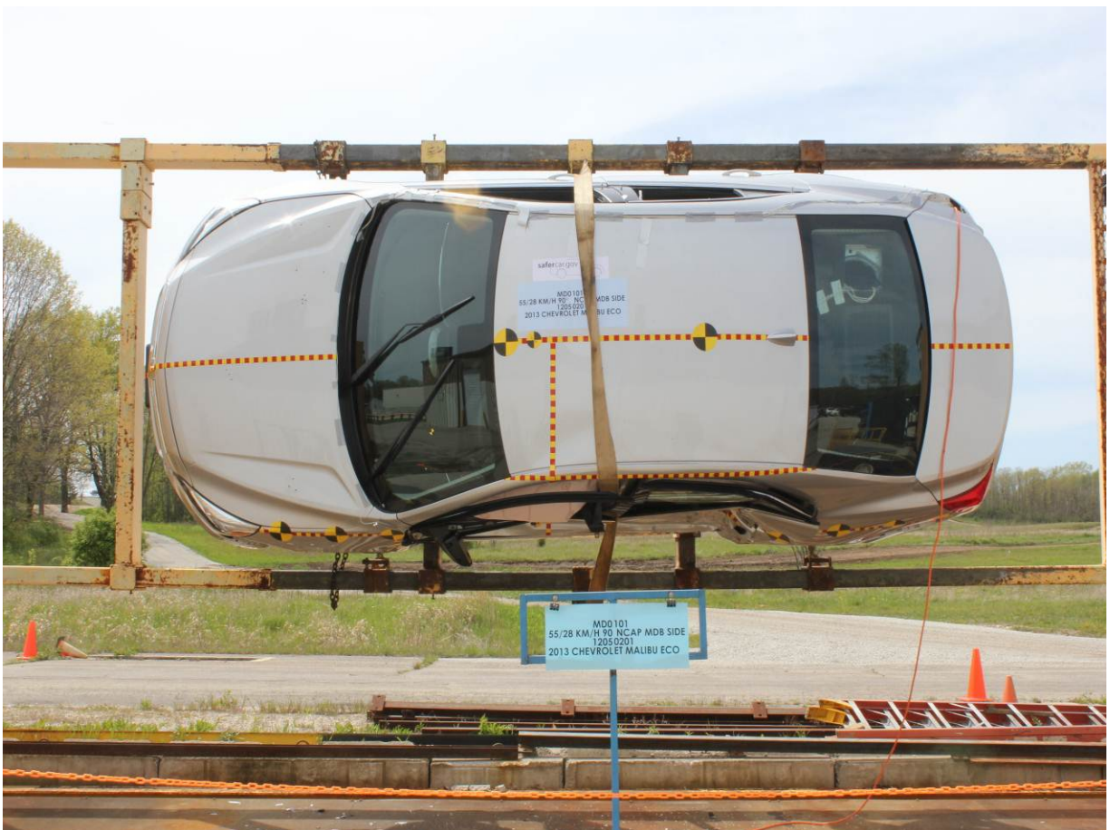
FMVSS No. 301 Static Rollover 270 Degrees
