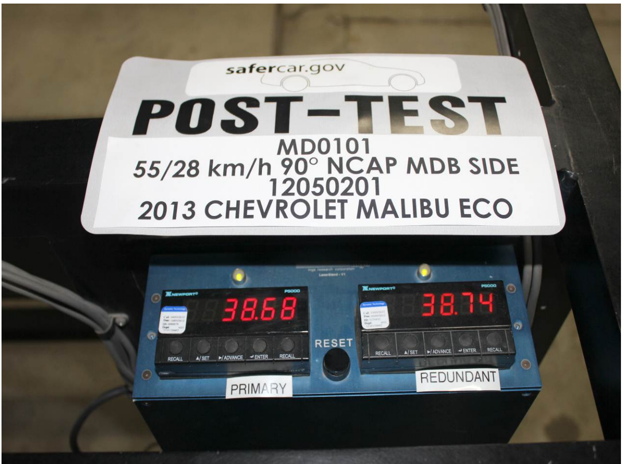
Post-Test Primary and Redundant Speed Trap Read-Out
