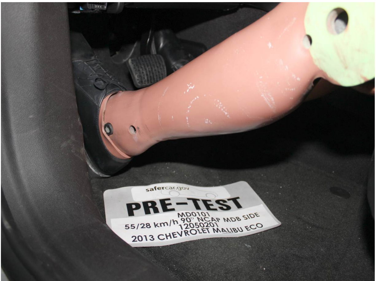
Pre-Test Placement of Driver Dummy's Feet
