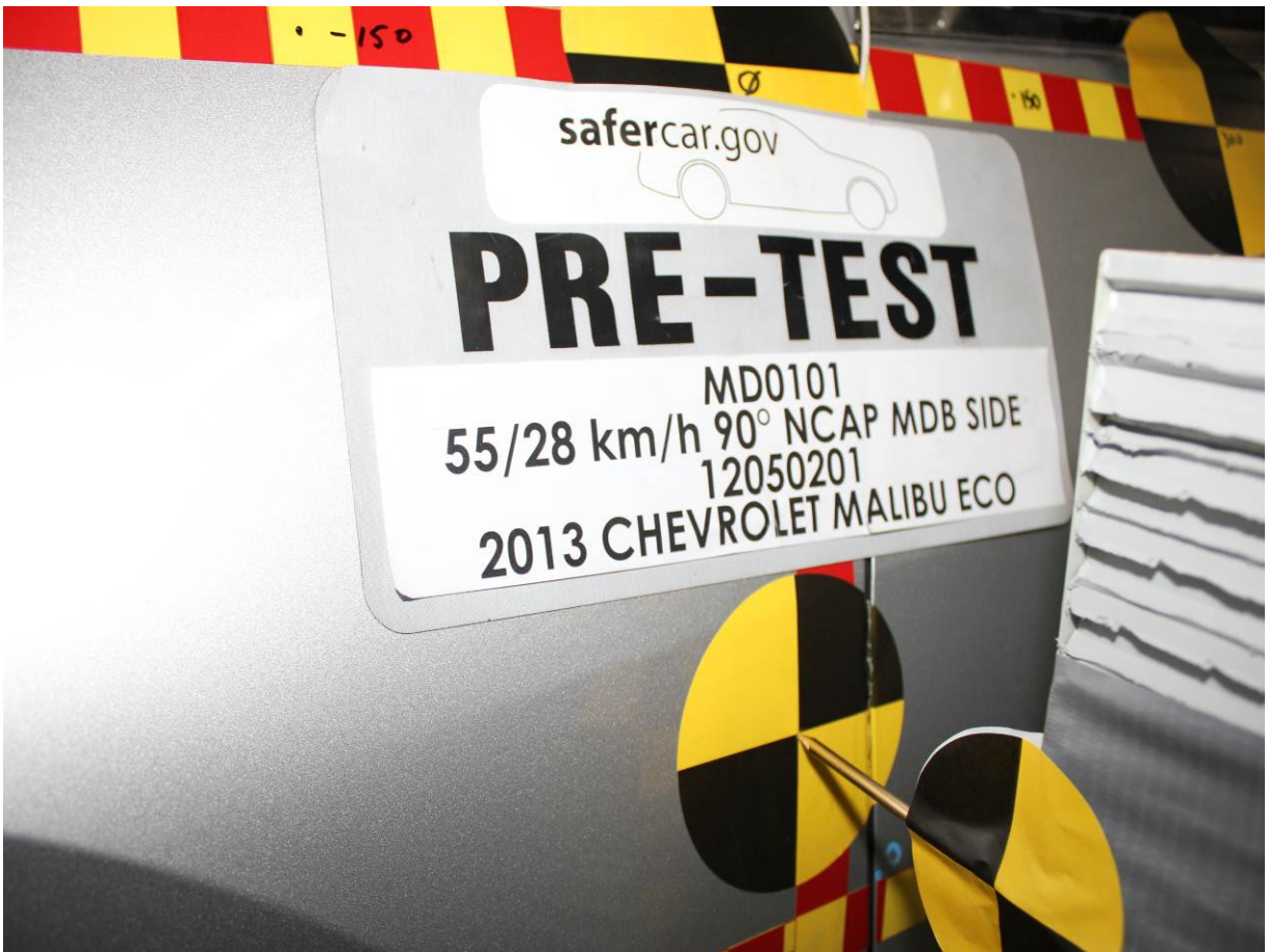
Pre-Test Close-Up View of Impact Point Target
