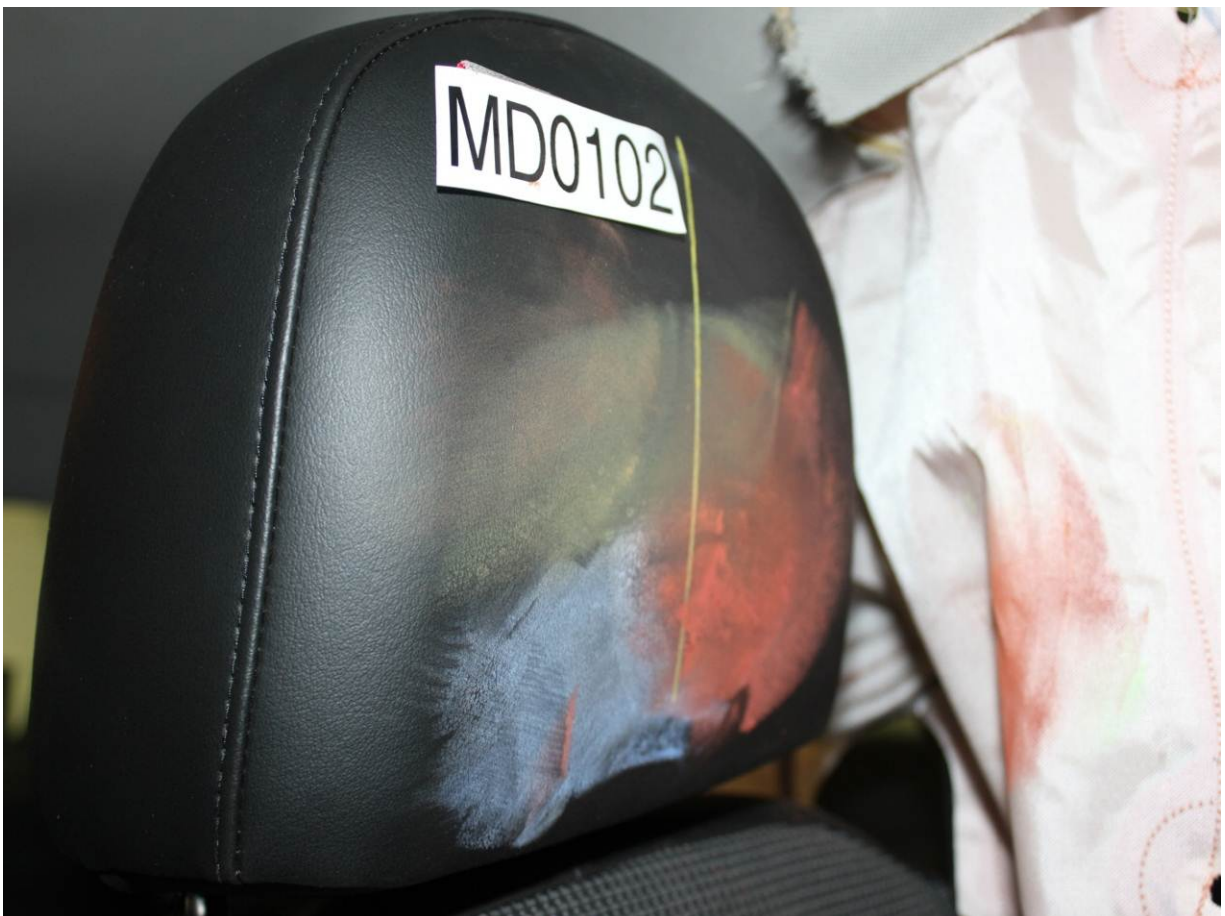
Post-Test Dummy Close-Up Head Contact with Vehicle Interior View
