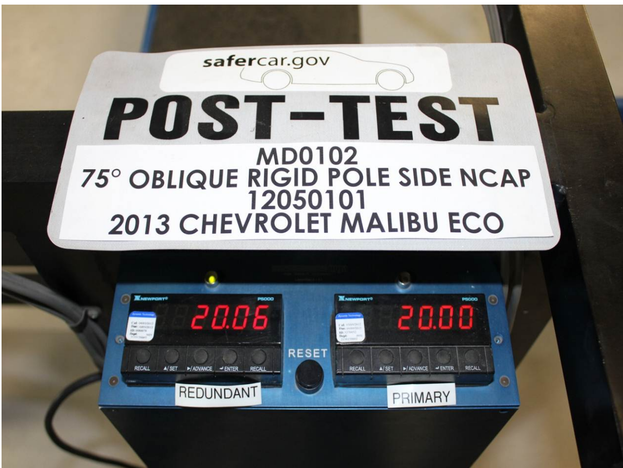
Post-Test Primary and Redundant Speed Trap Read-Out
