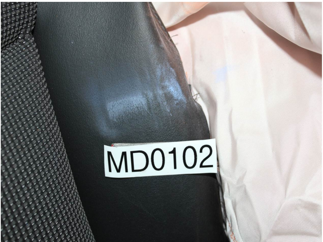
Post-Test Dummy Close-Up Torso Contact with Vehicle Interior View
