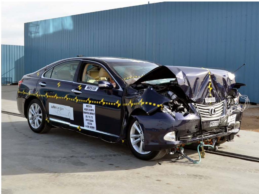
FIGURE 4. Post-Test Left Front ¾ View of NCAP Frontal Impact Test
