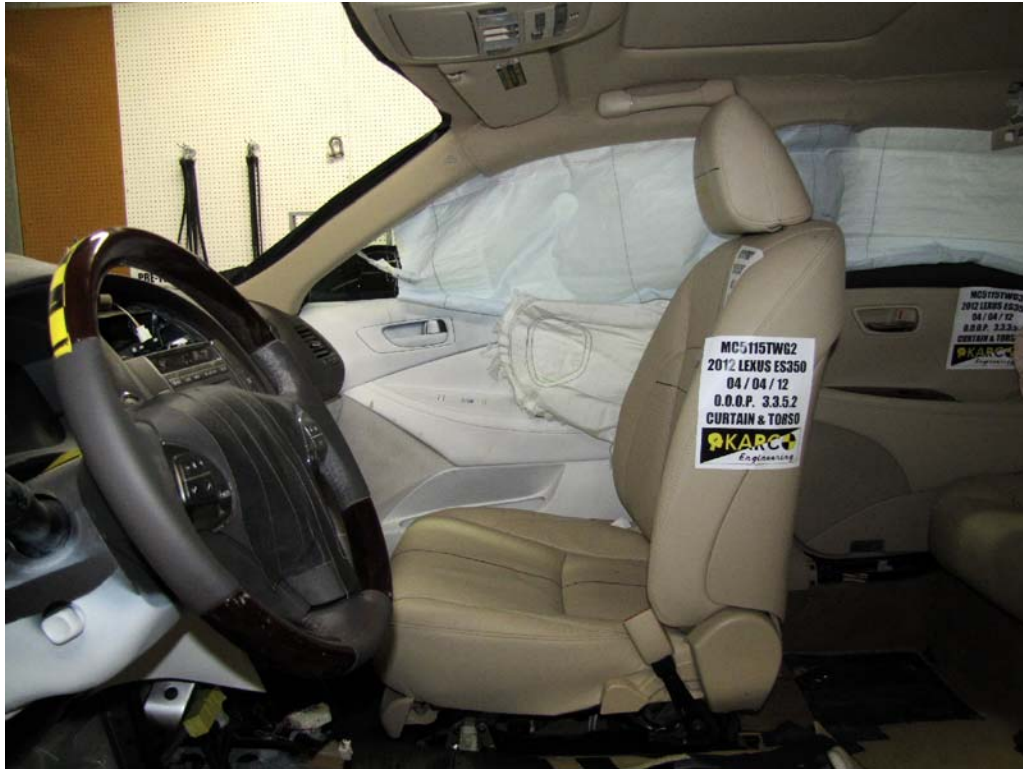
FIGURE 13. Post-Test Airbags, Left Side View
