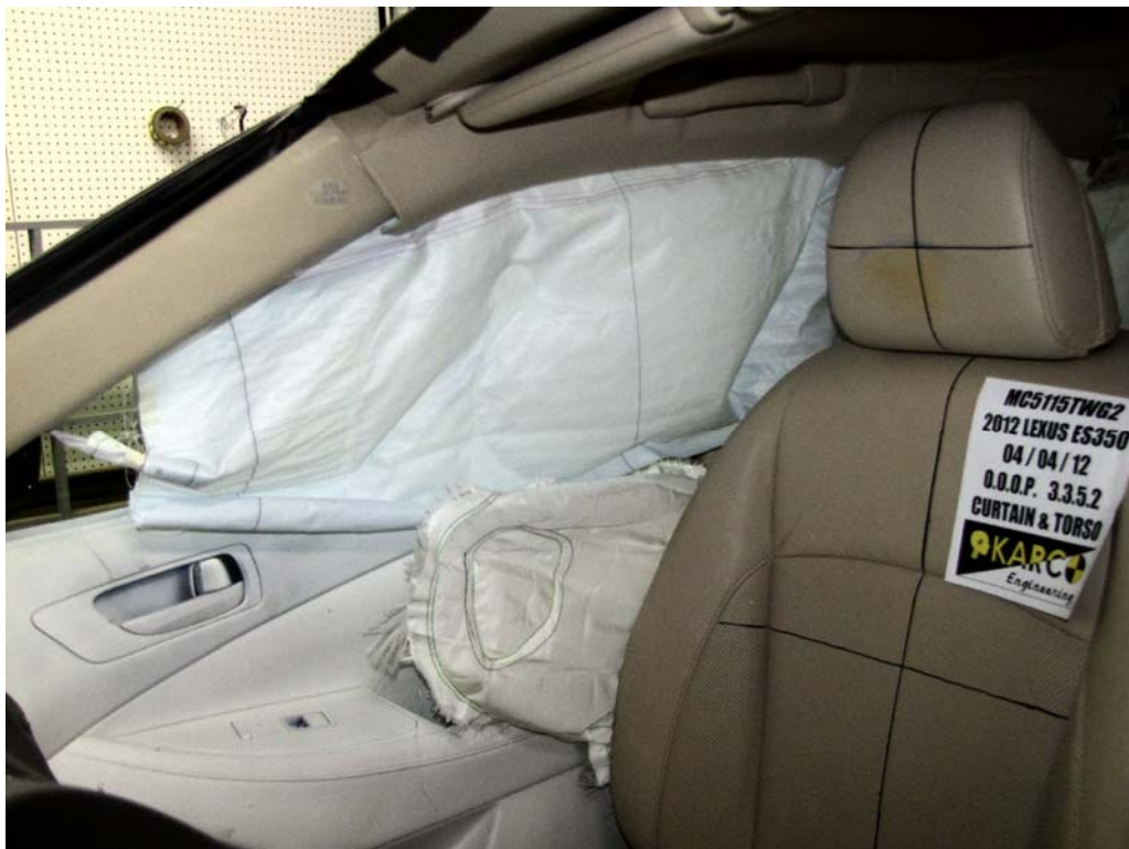
FIGURE 14. Post-Test Airbags, Left Front \frac{3}{4} View
