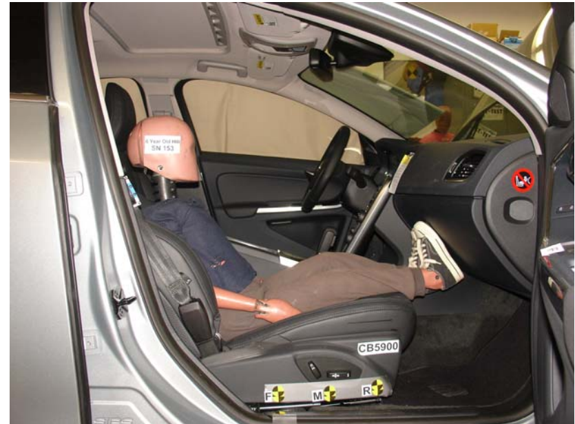
6-Year-Old Unbelted, Forward Seat Track, Position 2
