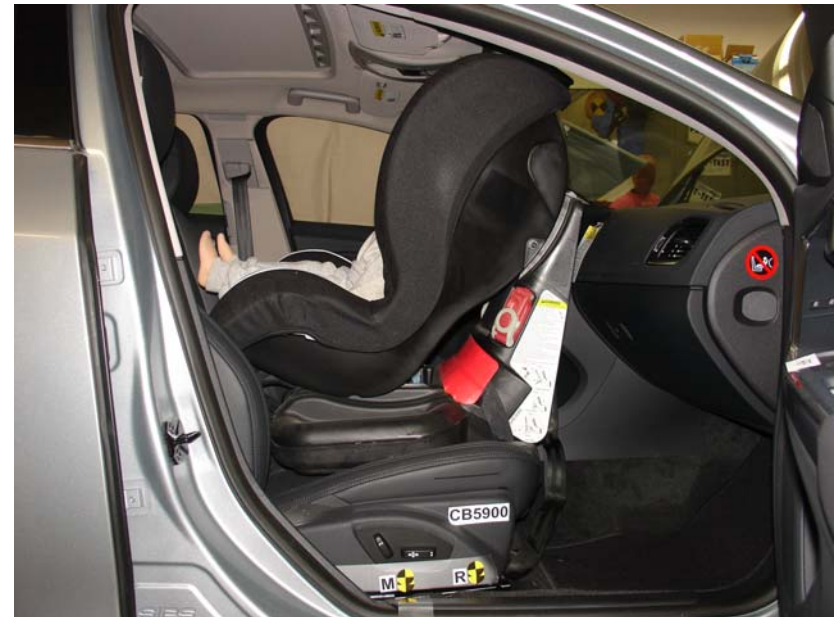
Graco Toddler Safeseat Step 2 Rear Facing Unbelted, Middle Seat Track
