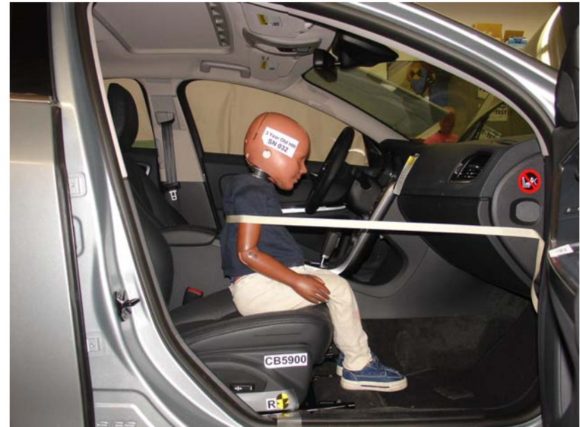
3-Year-Old Unbelted, Rearward Seat Track, Position 4
