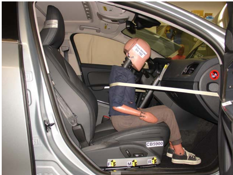
6-Year-Old Unbelted, Forward Seat Track, Position 3
