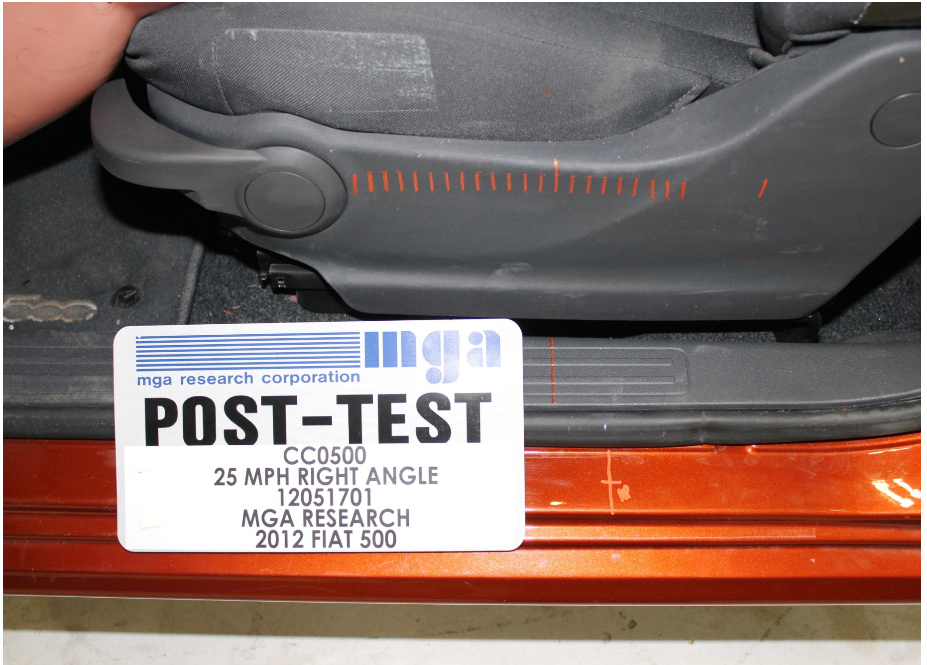
Post-Test Driver Dummy Seat Position
