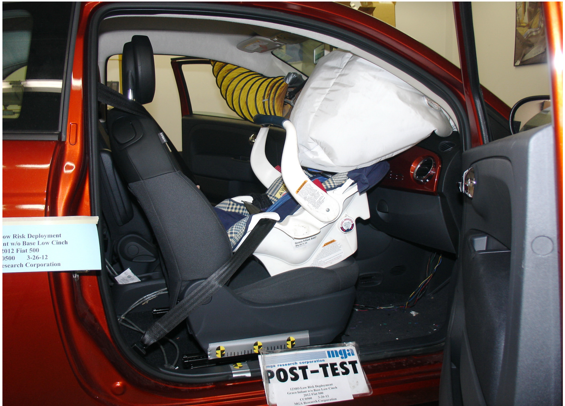
Post-Test 12 Mo Pass. Dummy Right Side View (Graco Infant Low Cinch)
