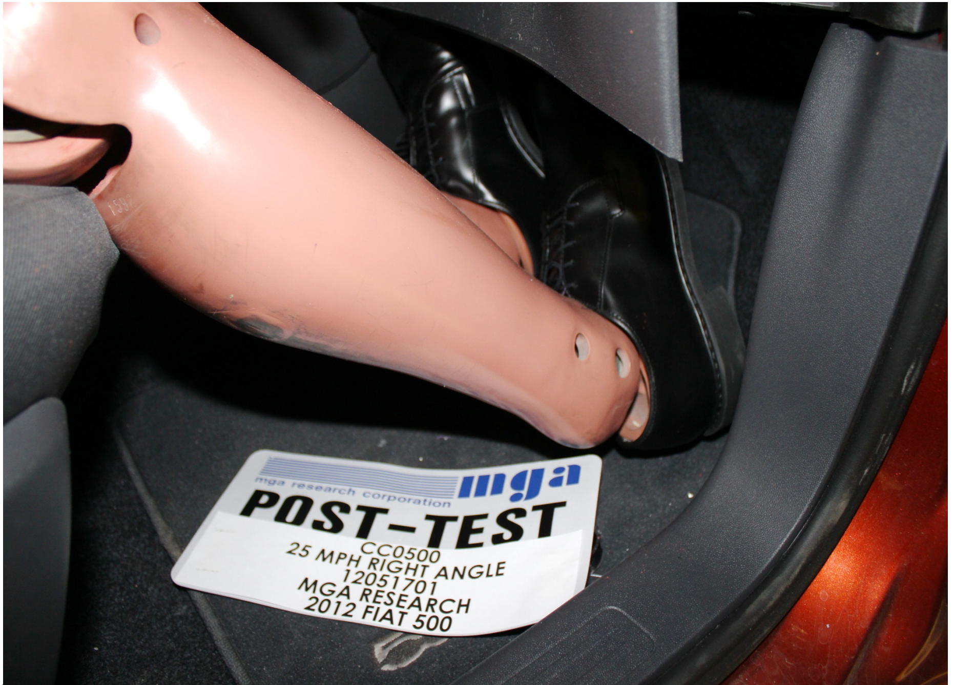
Post-Test Passenger Dummy Feet Position
