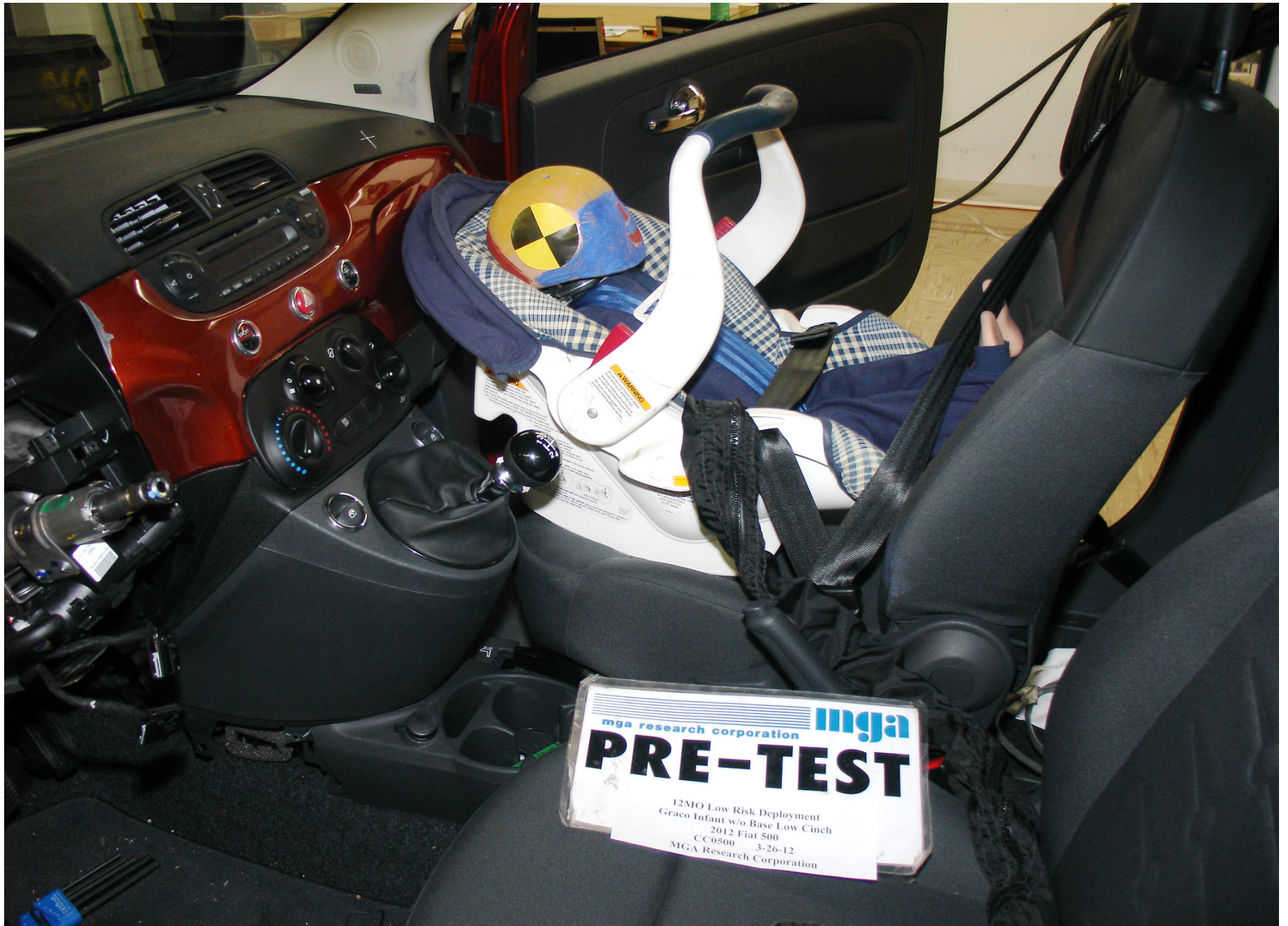
Pre-Test 12 Mo Pass. Dummy Left Side View (Graco Infant Low Cinch)
