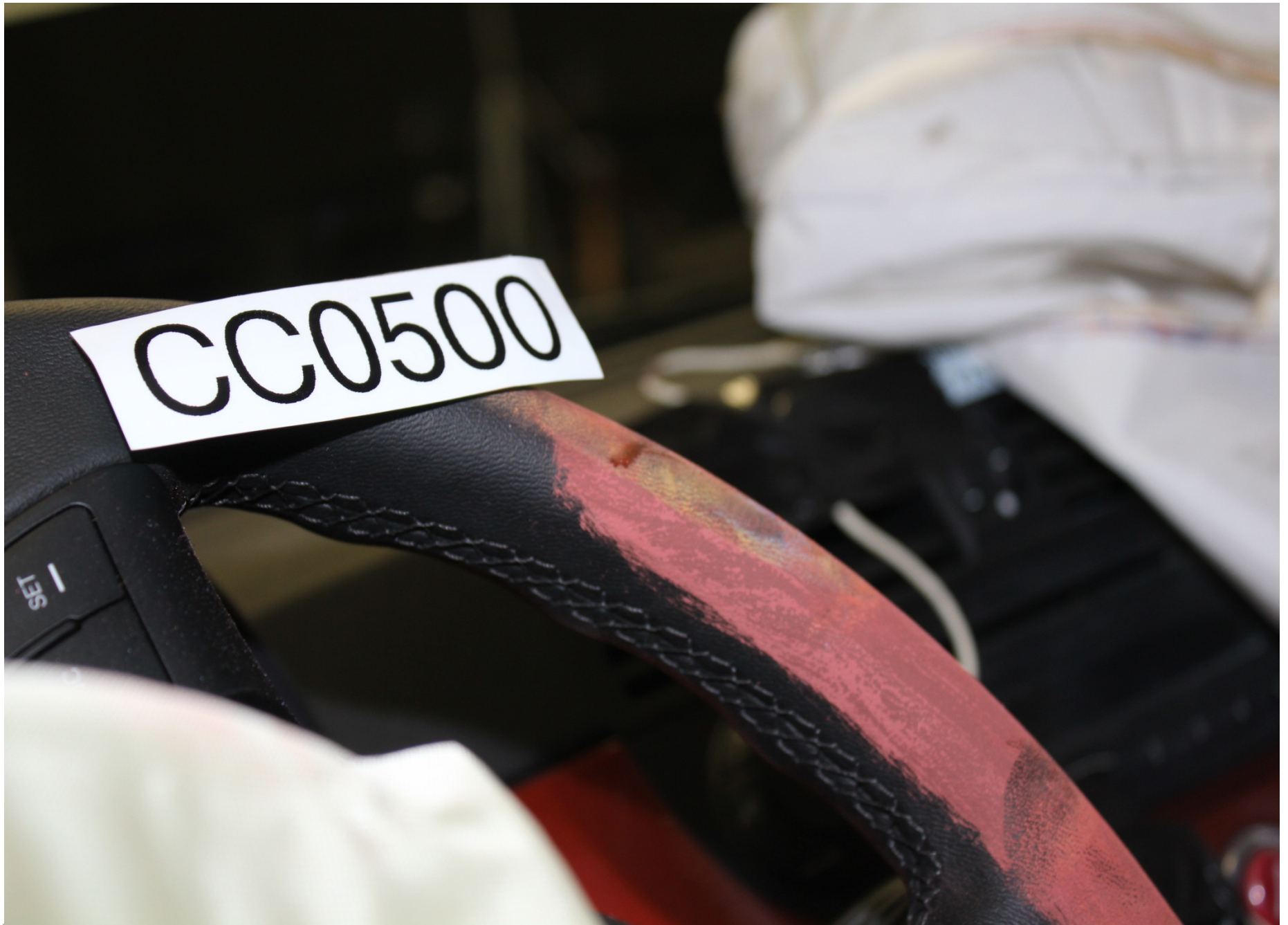
Post-Test Driver Dummy Head Contact (steering wheel)
