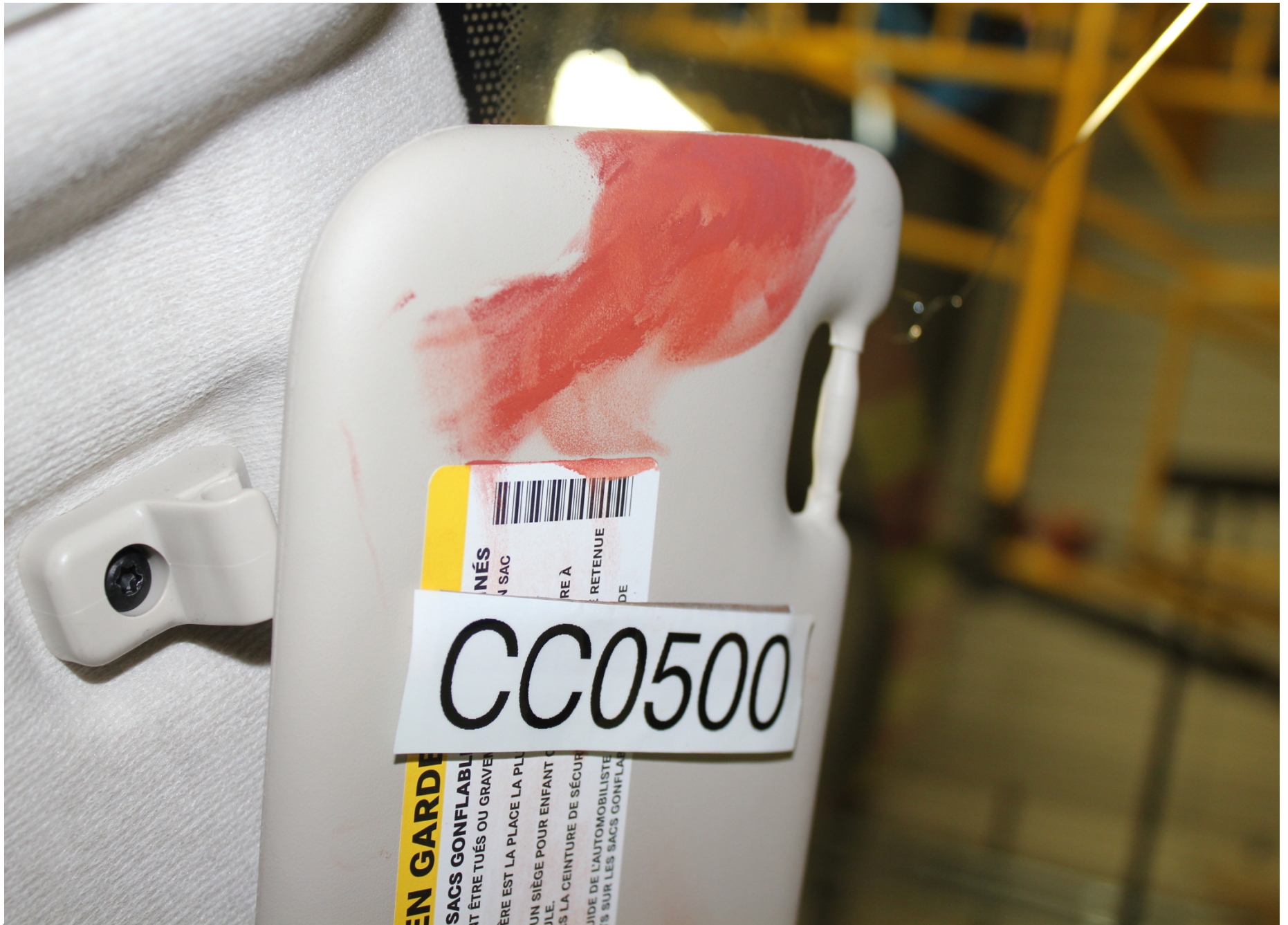
Post-Test Driver Dummy Head Contact (visor)
