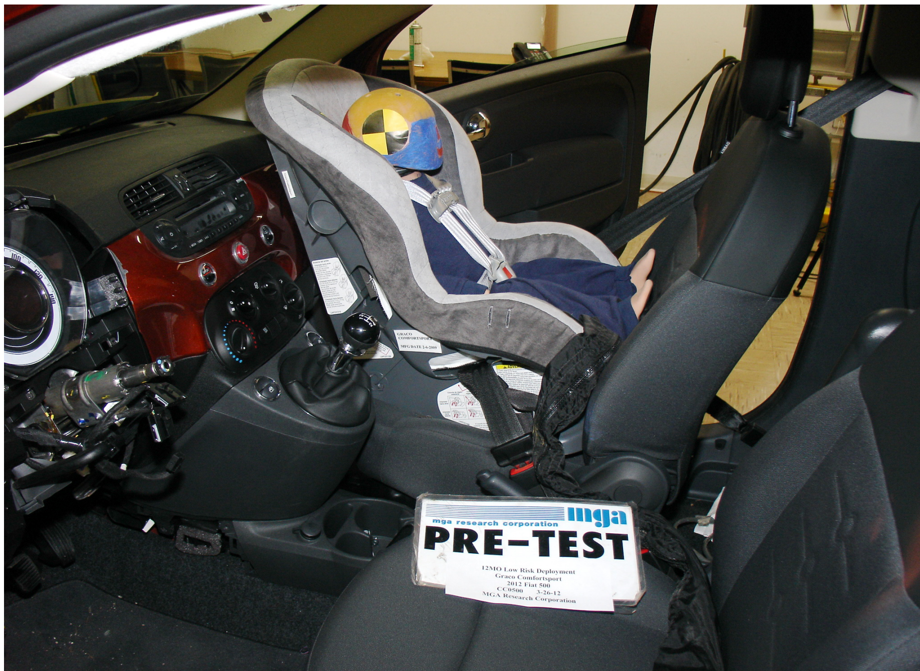
Pre-Test 12 Mo Pass. Dummy Left Side View (Graco Comfortsport Low Cinch)
