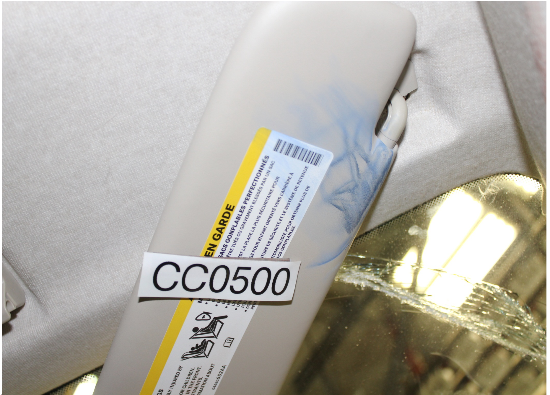
Post-Test Passenger Dummy Head Contact (visor)
