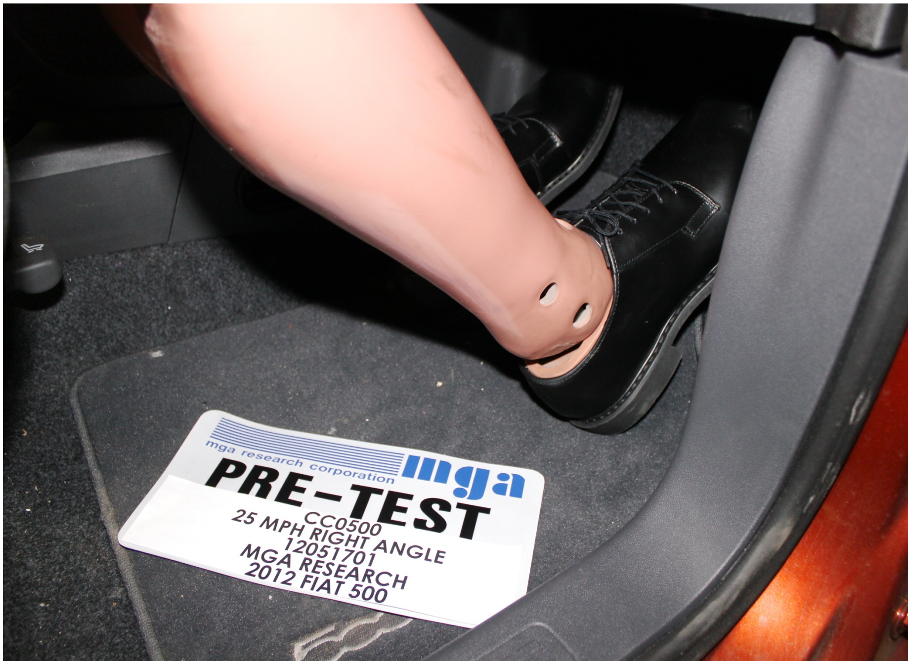
Pre-Test Passenger Dummy Feet Position
