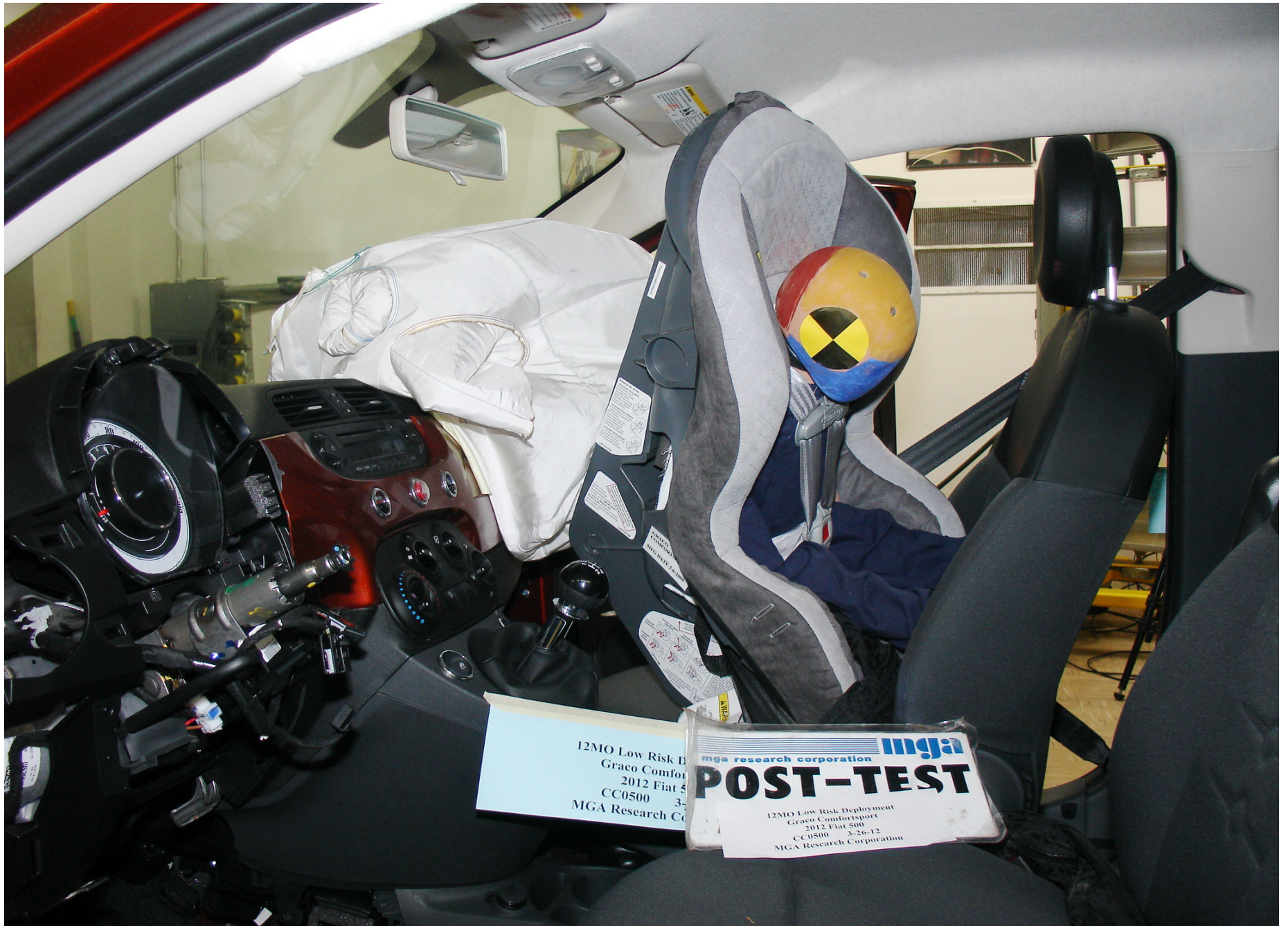
Post-Test 12 Mo Pass. Dummy Left Side View (Graco Comfortsport Low Cinch)
