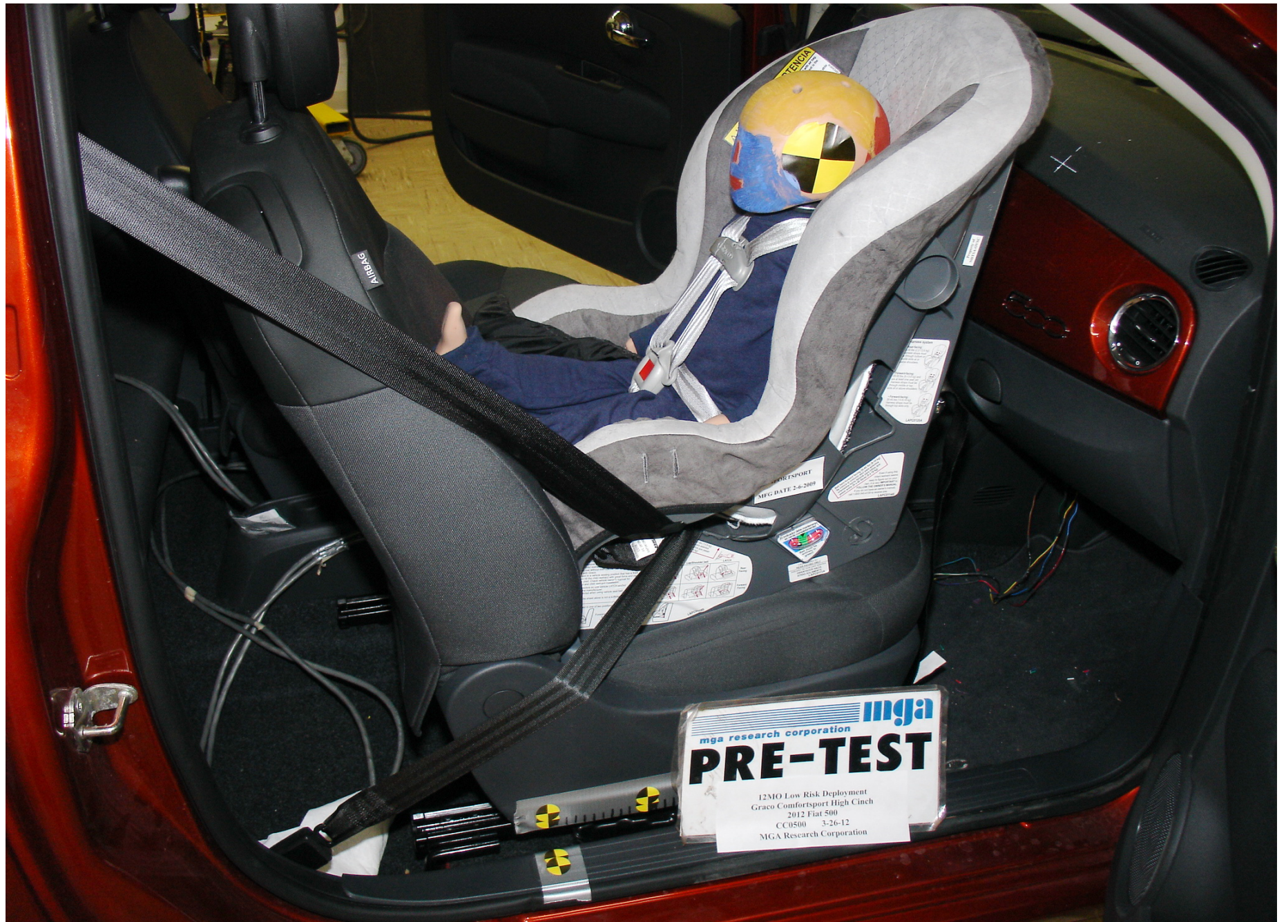
Pre-Test 12 Mo Pass. Dummy Right Side View (Graco Comfortsport High Cinch)
