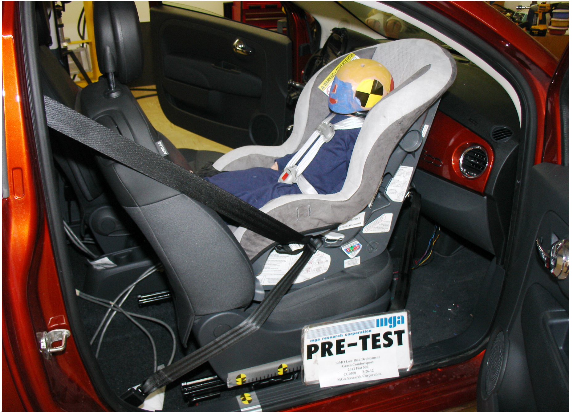
Pre-Test 12 Mo Pass. Dummy Right Side View (Graco Comfortsport Low Cinch)
