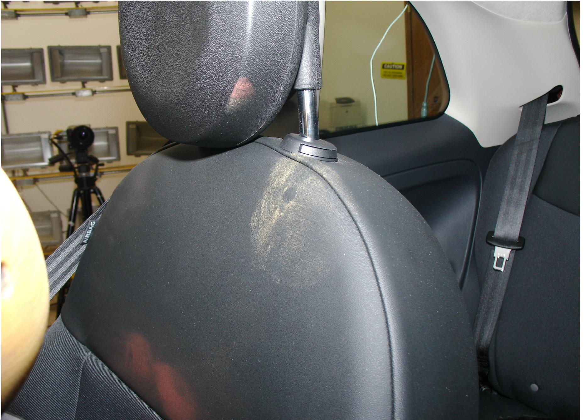
Post-Test 12 Mo Pass. Dummy Head Contact (seatback)
