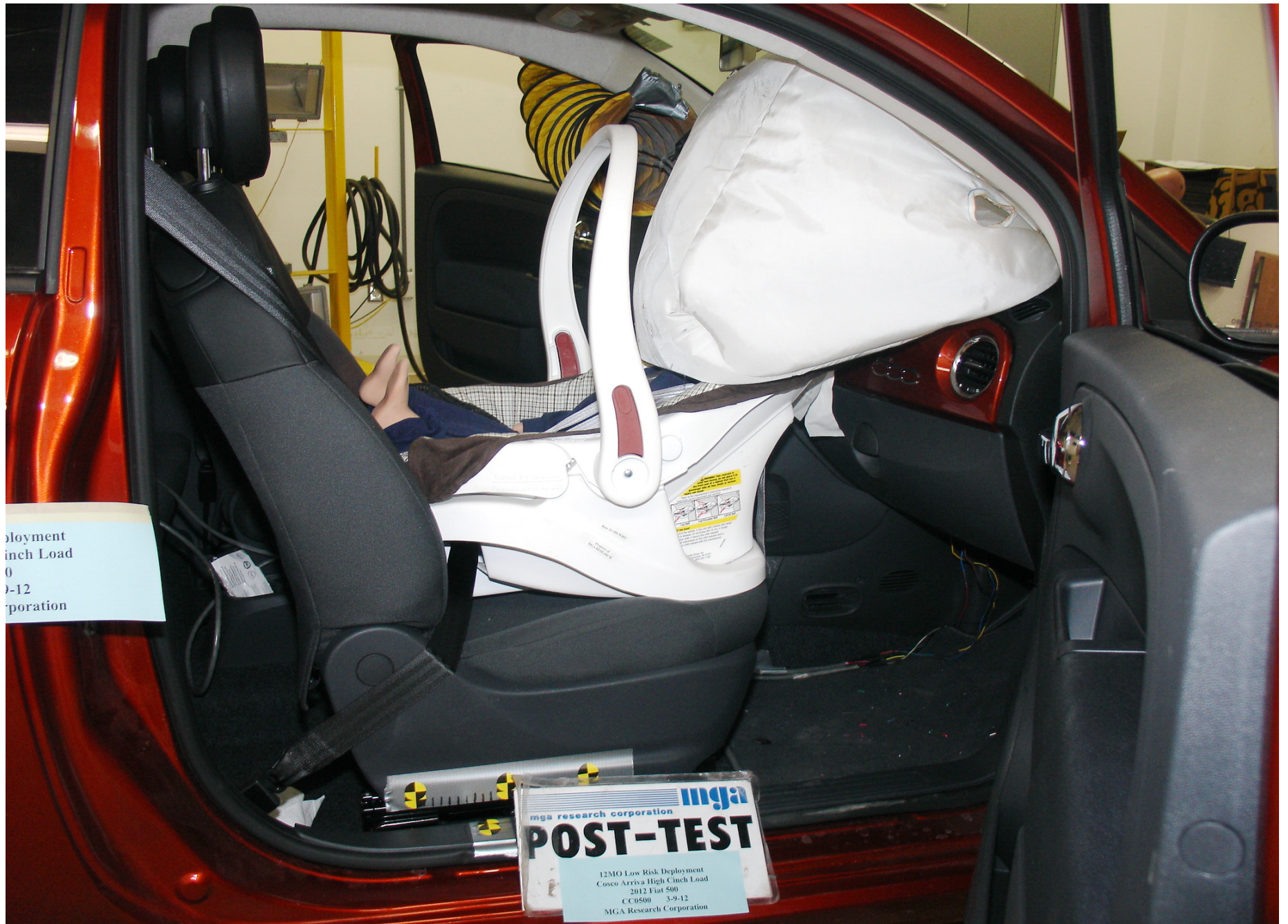
Post-Test 12 Mo Pass. Dummy Right Side View (Cosco Arriva High Cinch)
