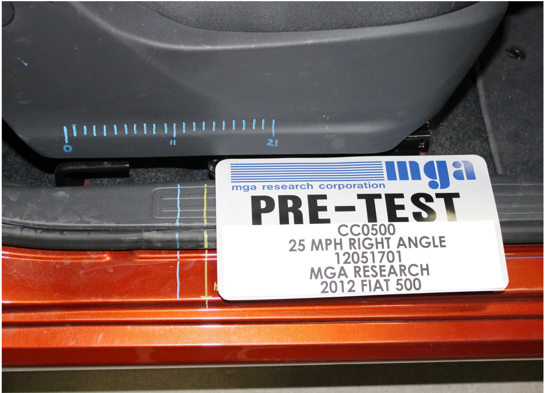
Pre-Test Passenger Dummy Seat Position
