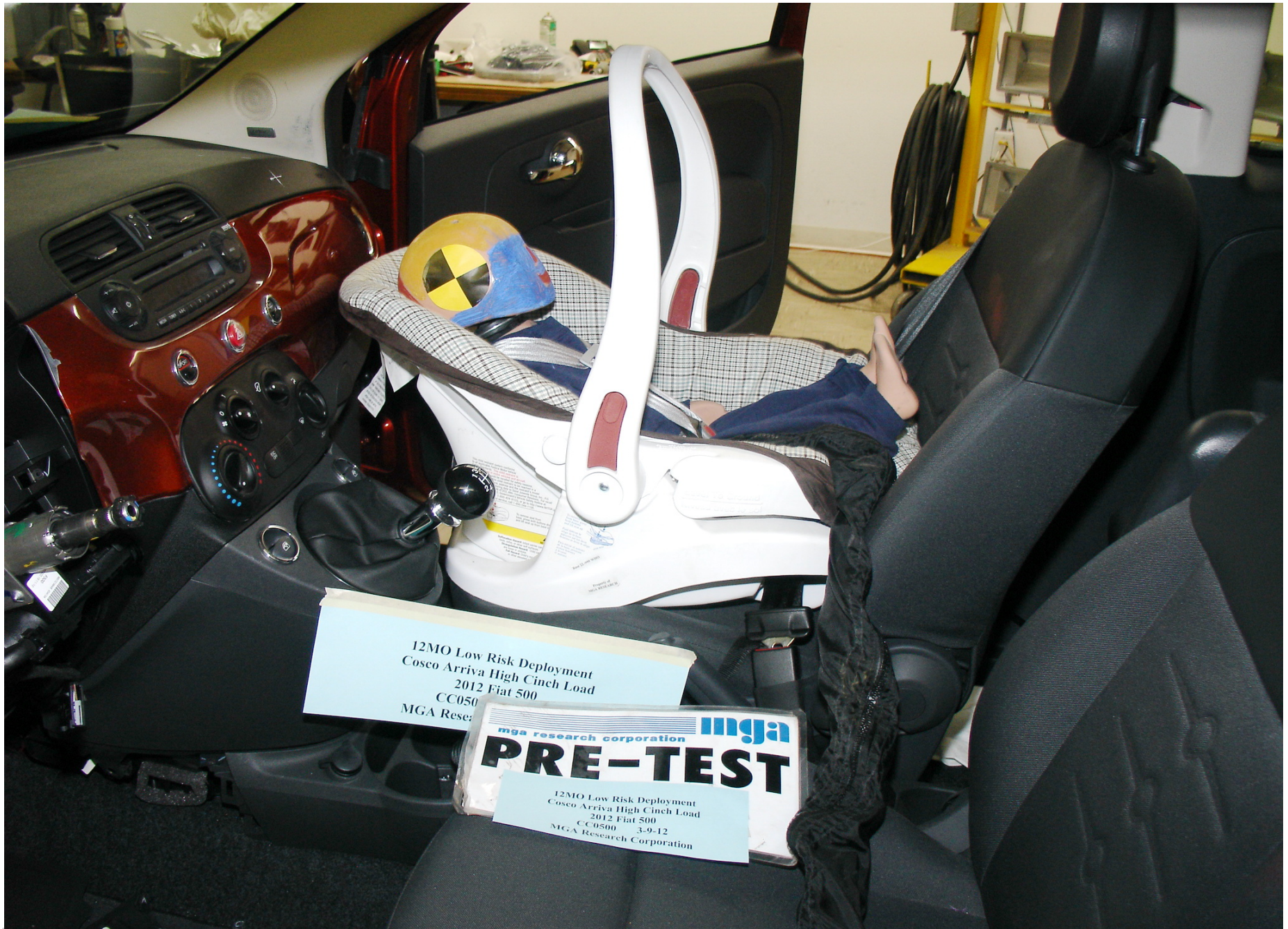
Pre-Test 12 Mo Pass. Dummy Right Side View (Cosco Arriva High Cinch)
