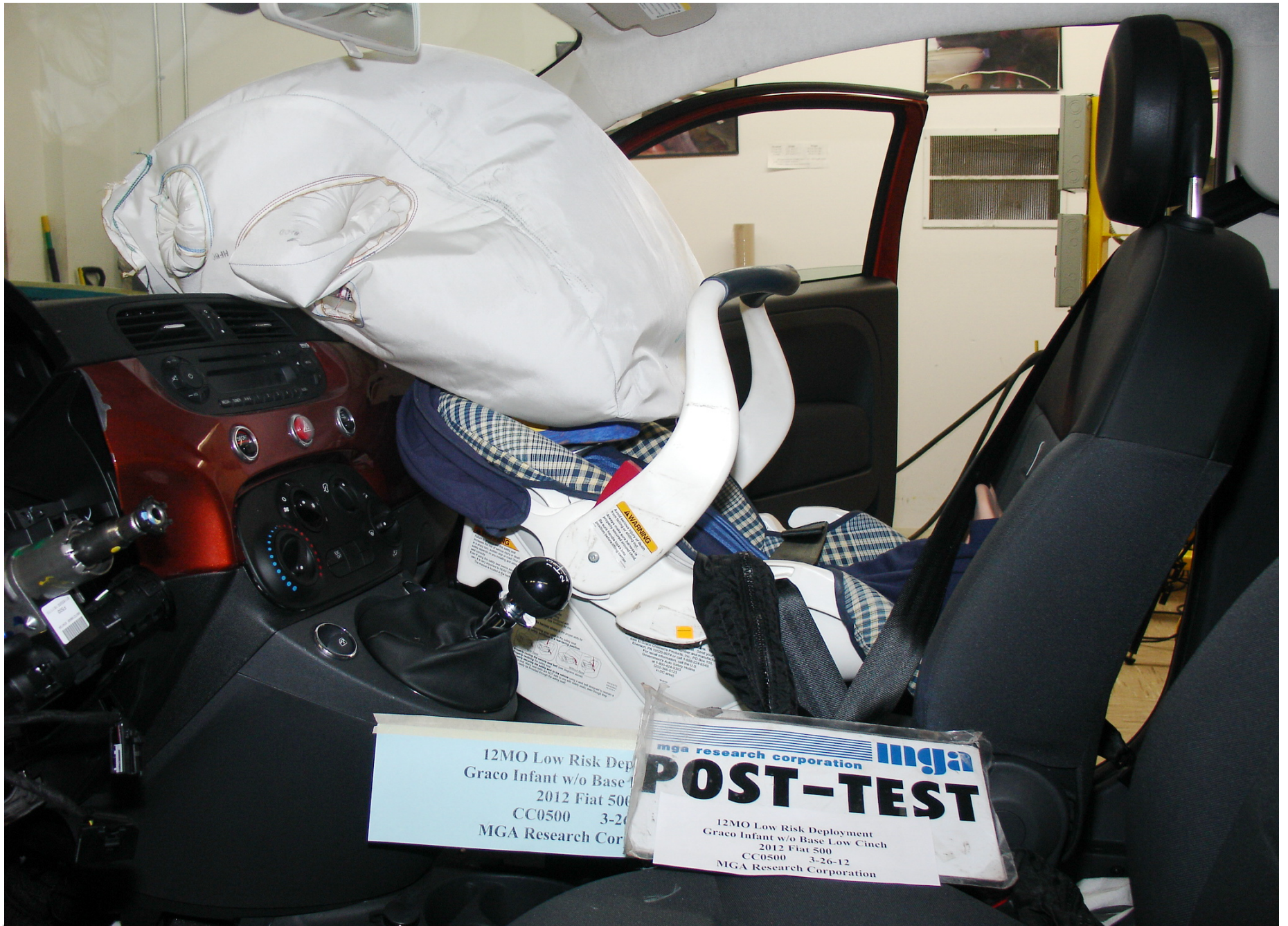
Post-Test 12 Mo Pass. Dummy Left Side View (Graco Infant Low Cinch)
