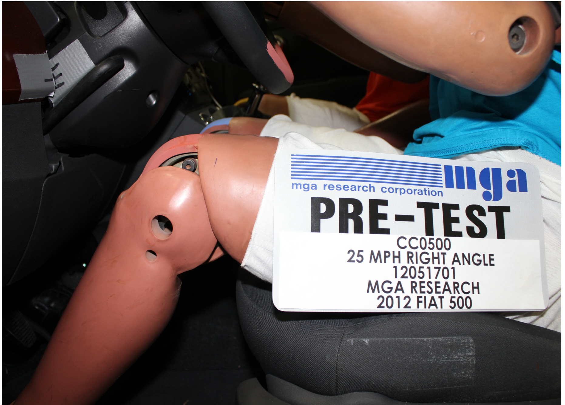
Pre-Test Driver Side Knee Bolster View
