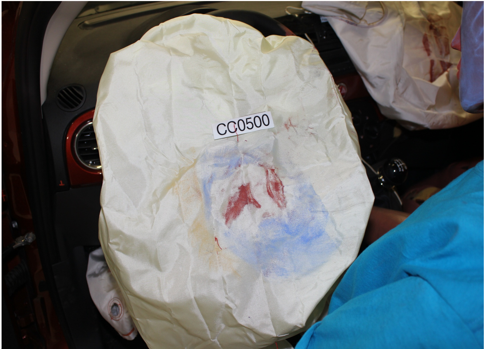
Post-Test Driver Dummy Airbag Contact
