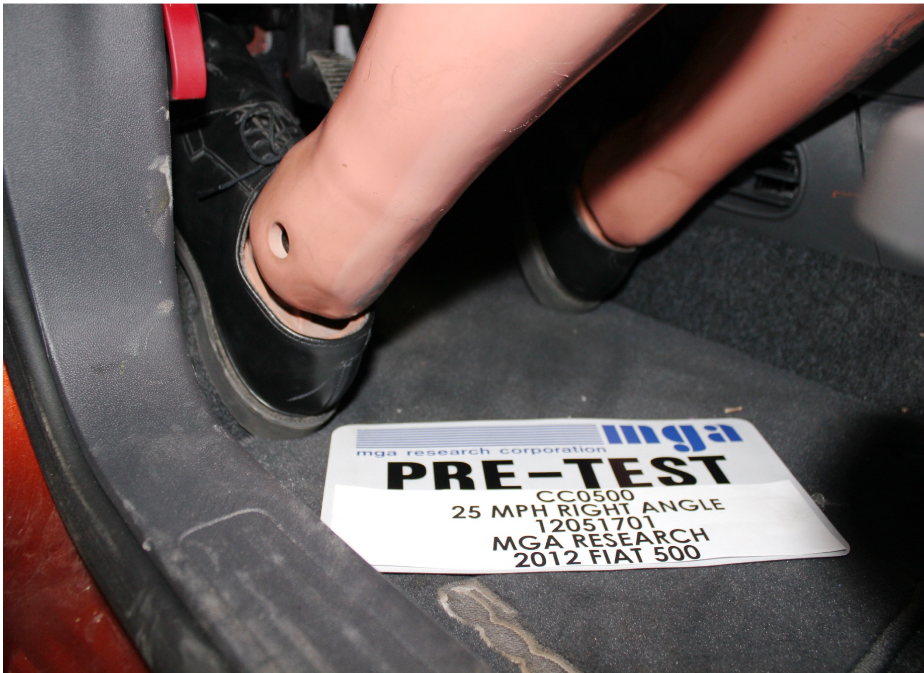
Pre-Test Driver Dummy Feet Position
