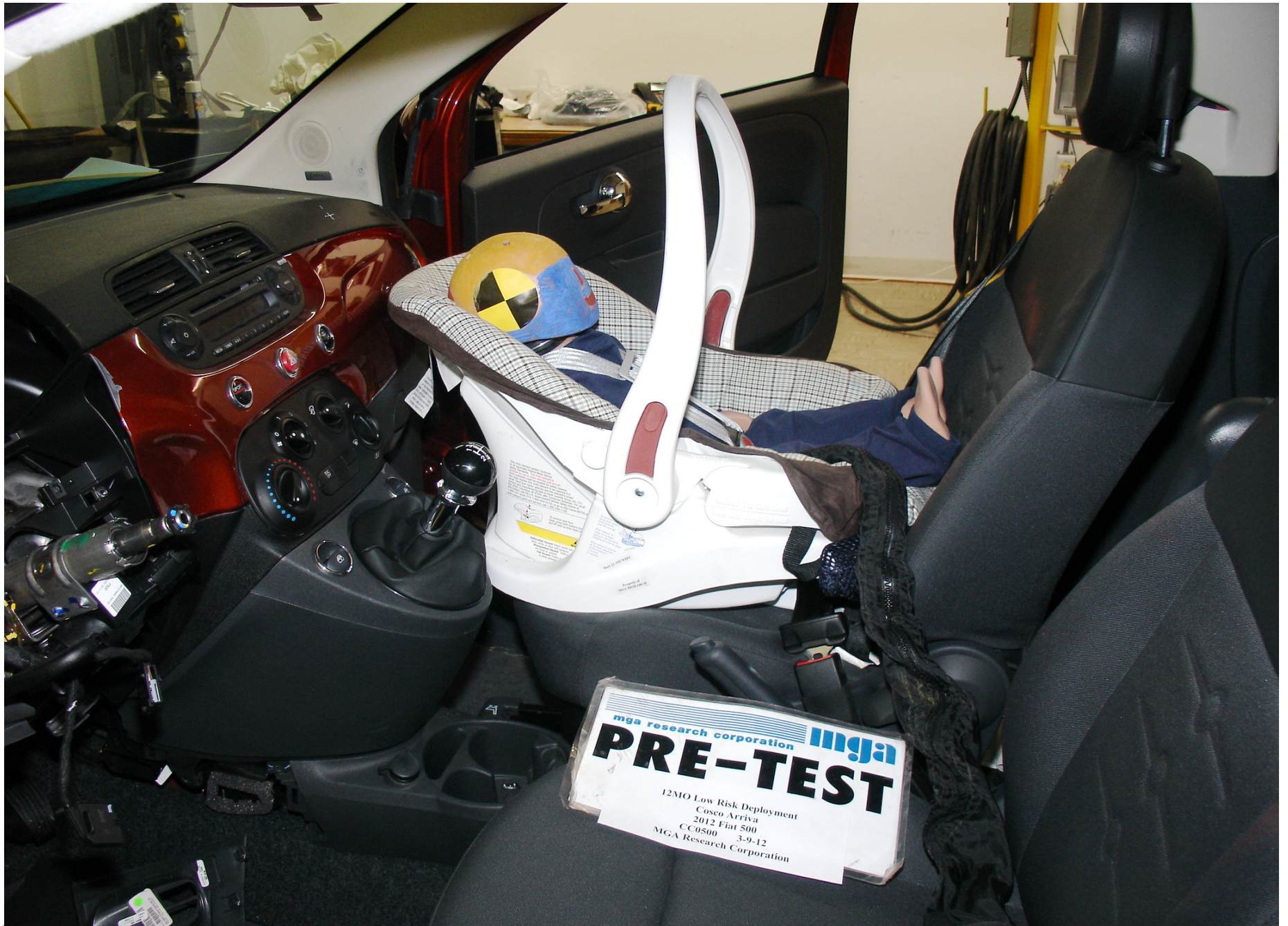
Pre-Test 12 Mo Pass. Dummy Left Side View (Cosco Arriva Low Cinch)
