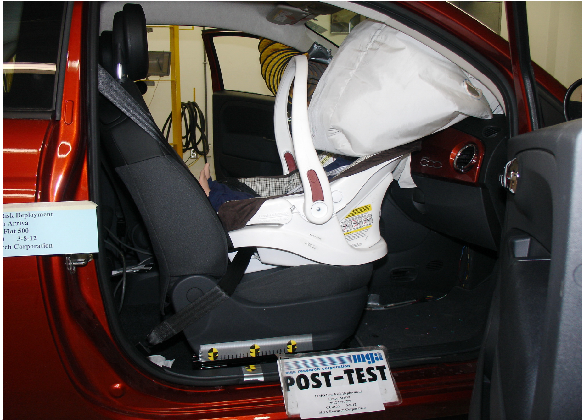
Post-Test 12 Mo Pass. Dummy Right Side View (Cosco Arriva Low Cinch)
