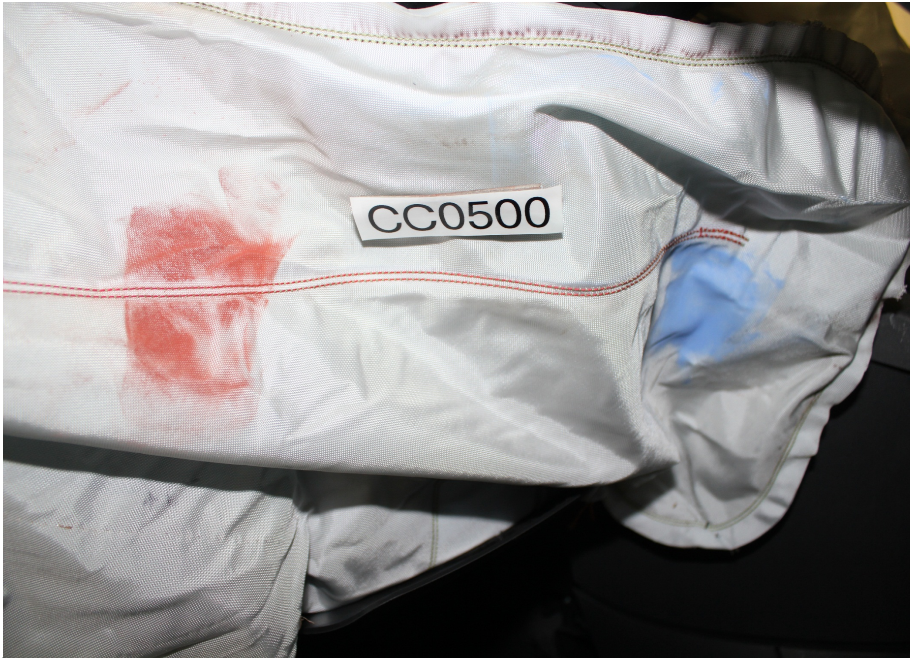
Post-Test Driver Dummy Knee Contact
