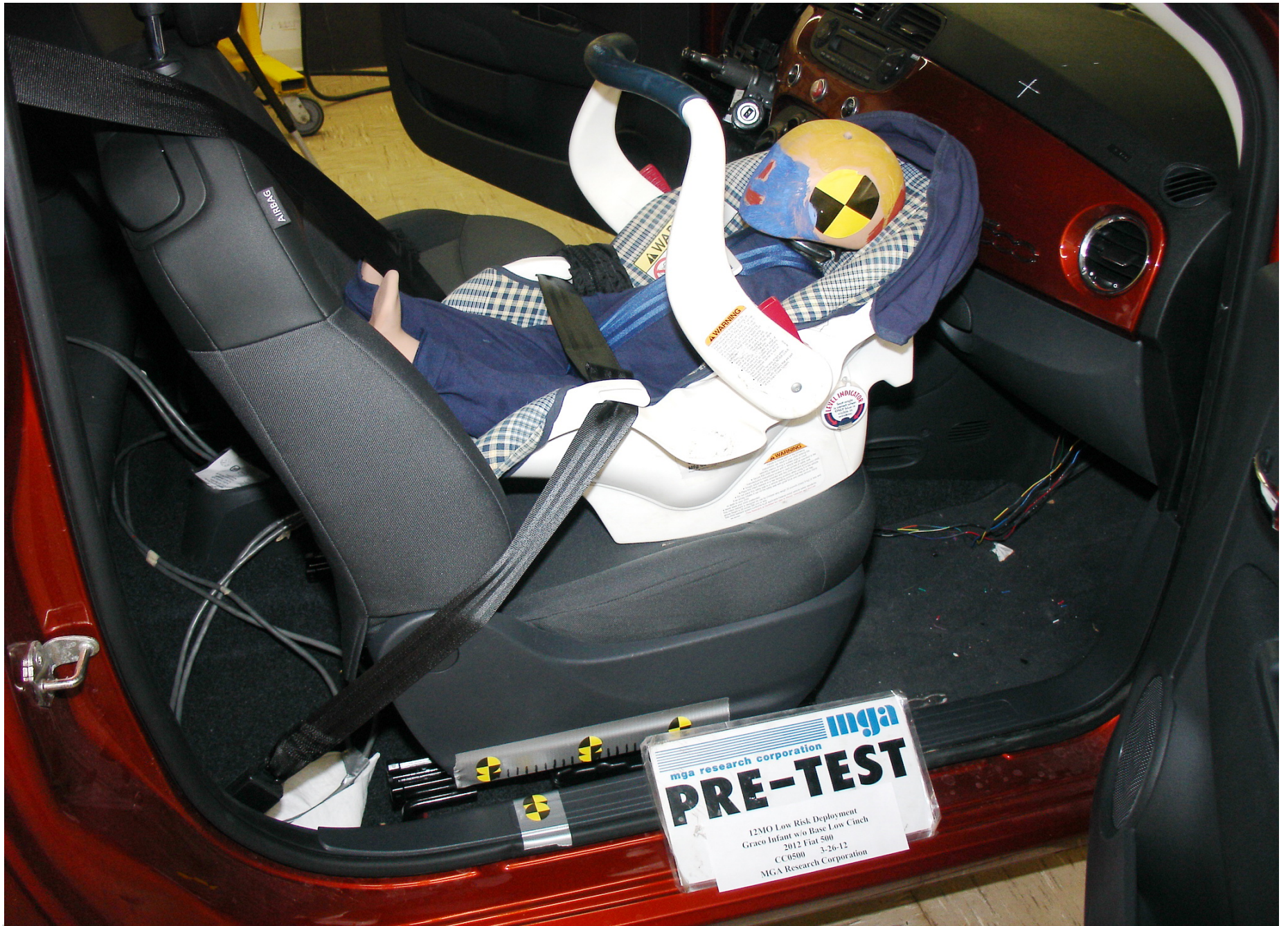
Pre-Test 12 Mo Pass. Dummy Right Side View (Graco Infant Low Cinch)
