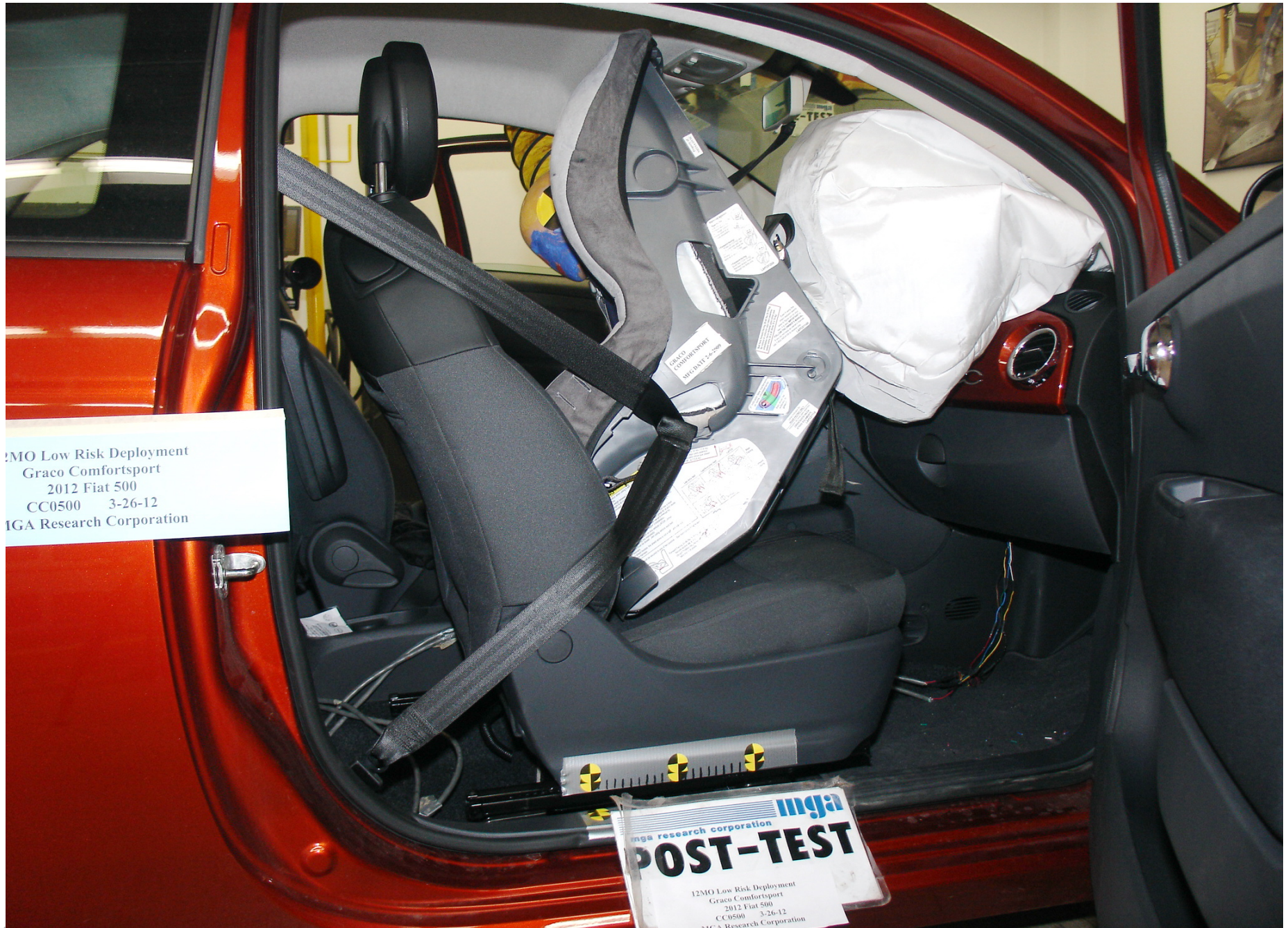
Post-Test 12 Mo Pass. Dummy Right Side View (Graco Comfortsport Low Cinch)
