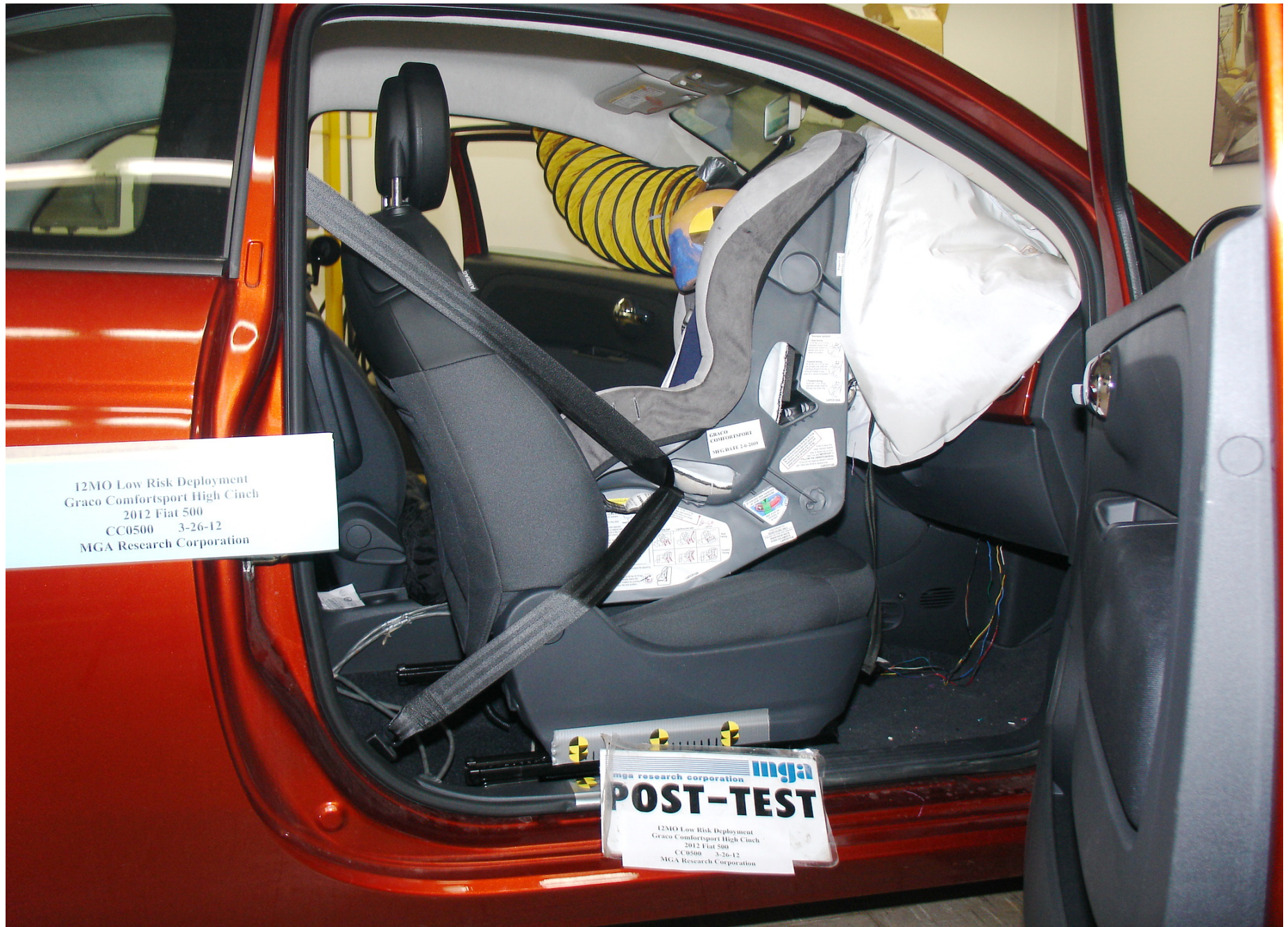
Post-Test 12 Mo Pass. Dummy Right Side View (Graco Comfortsport High Cinch)
