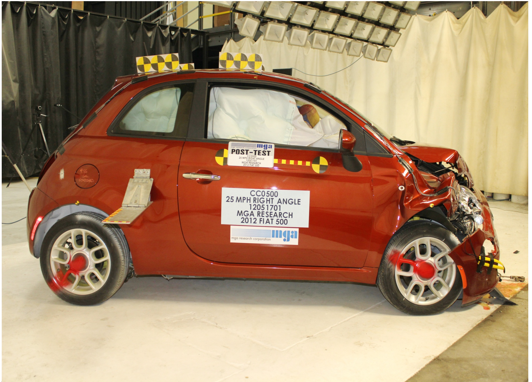
Post-Test Right Side View of Test Vehicle
