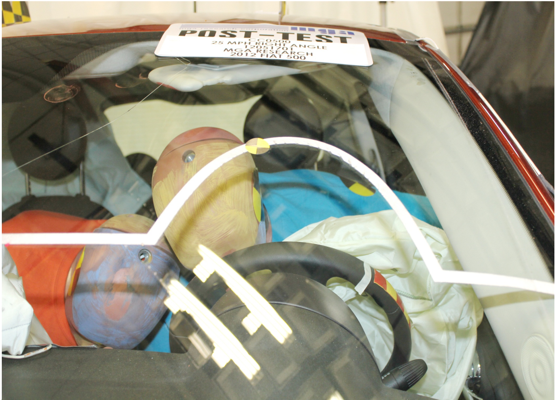
Post-Test Driver Dummy Front View (head position)
