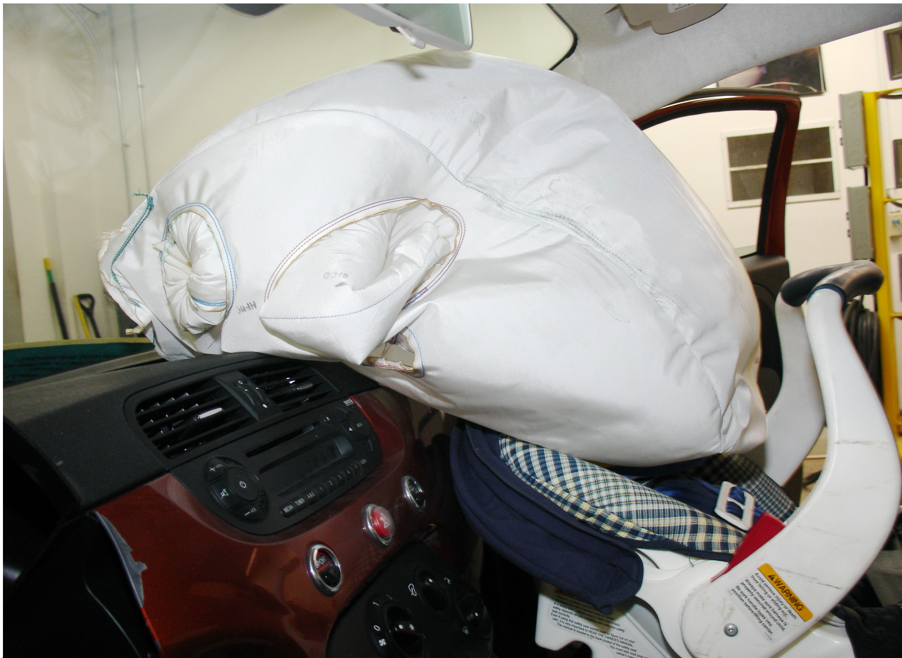
Post-Test 12 Mo Pass. Dummy Airbag Left Side View
