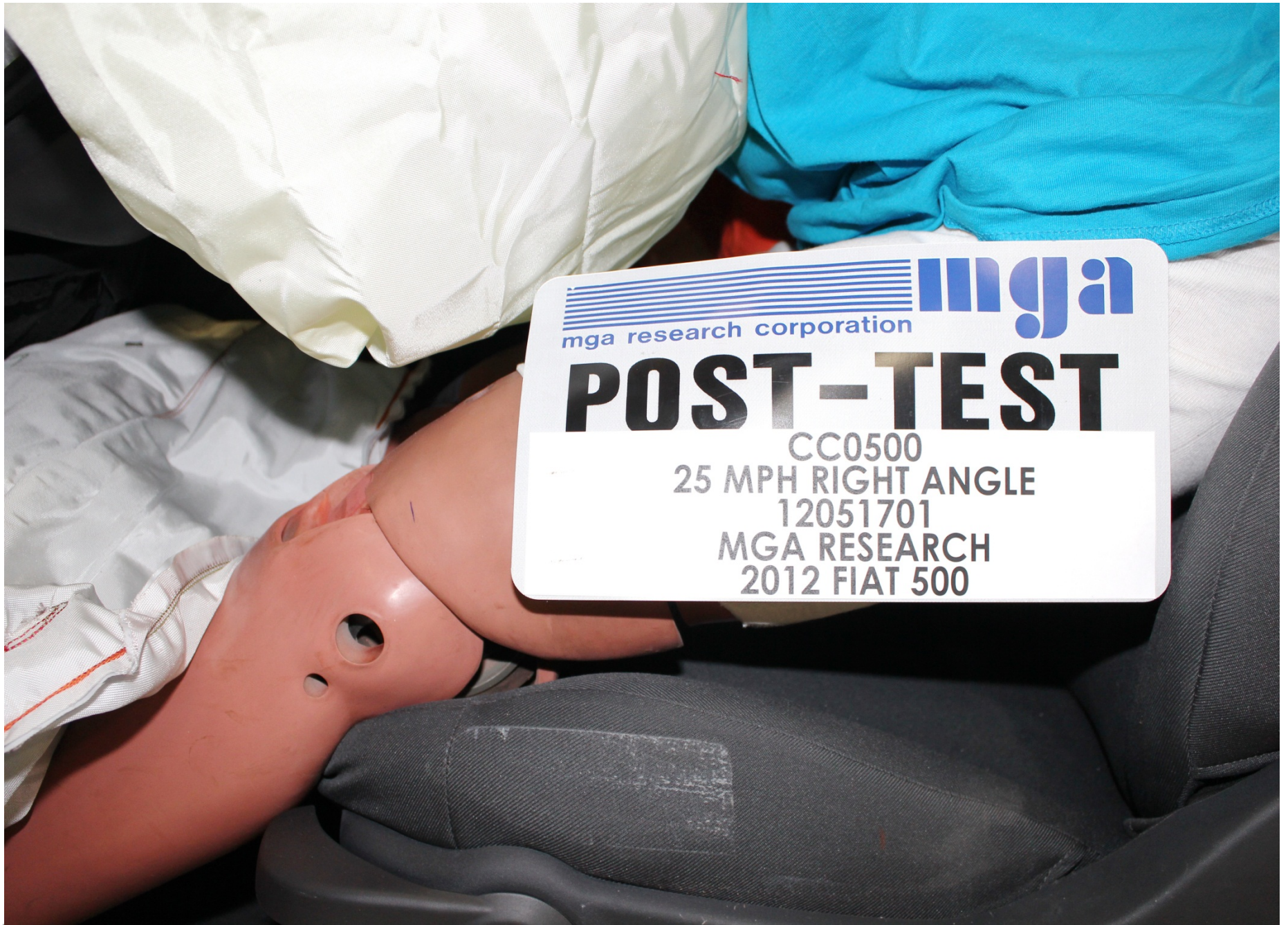
Post-Test Driver Side Knee Bolster View
