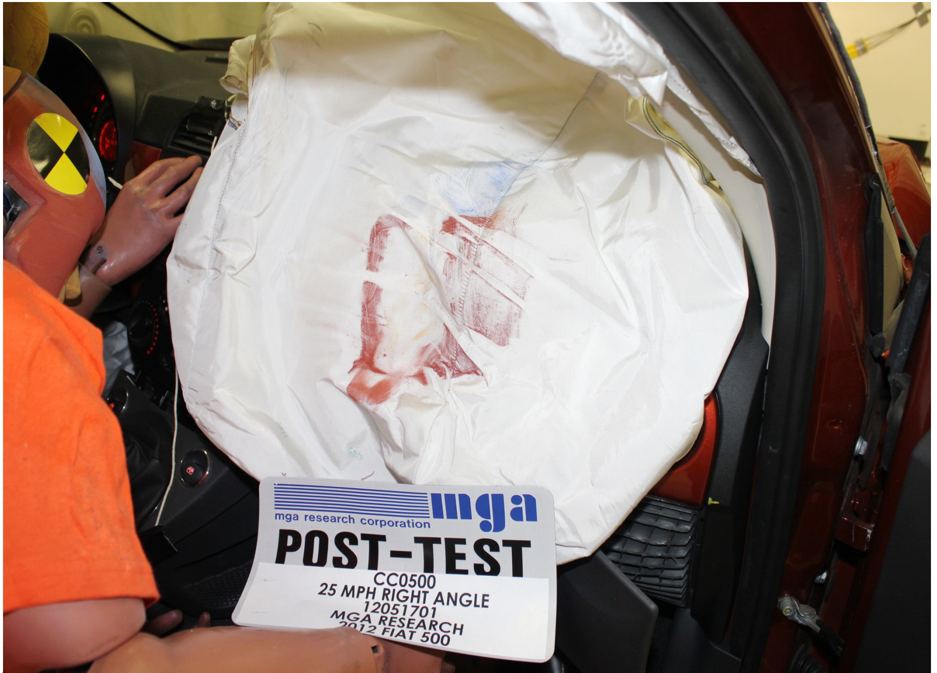
Post-Test Passenger Dummy Airbag Contact
