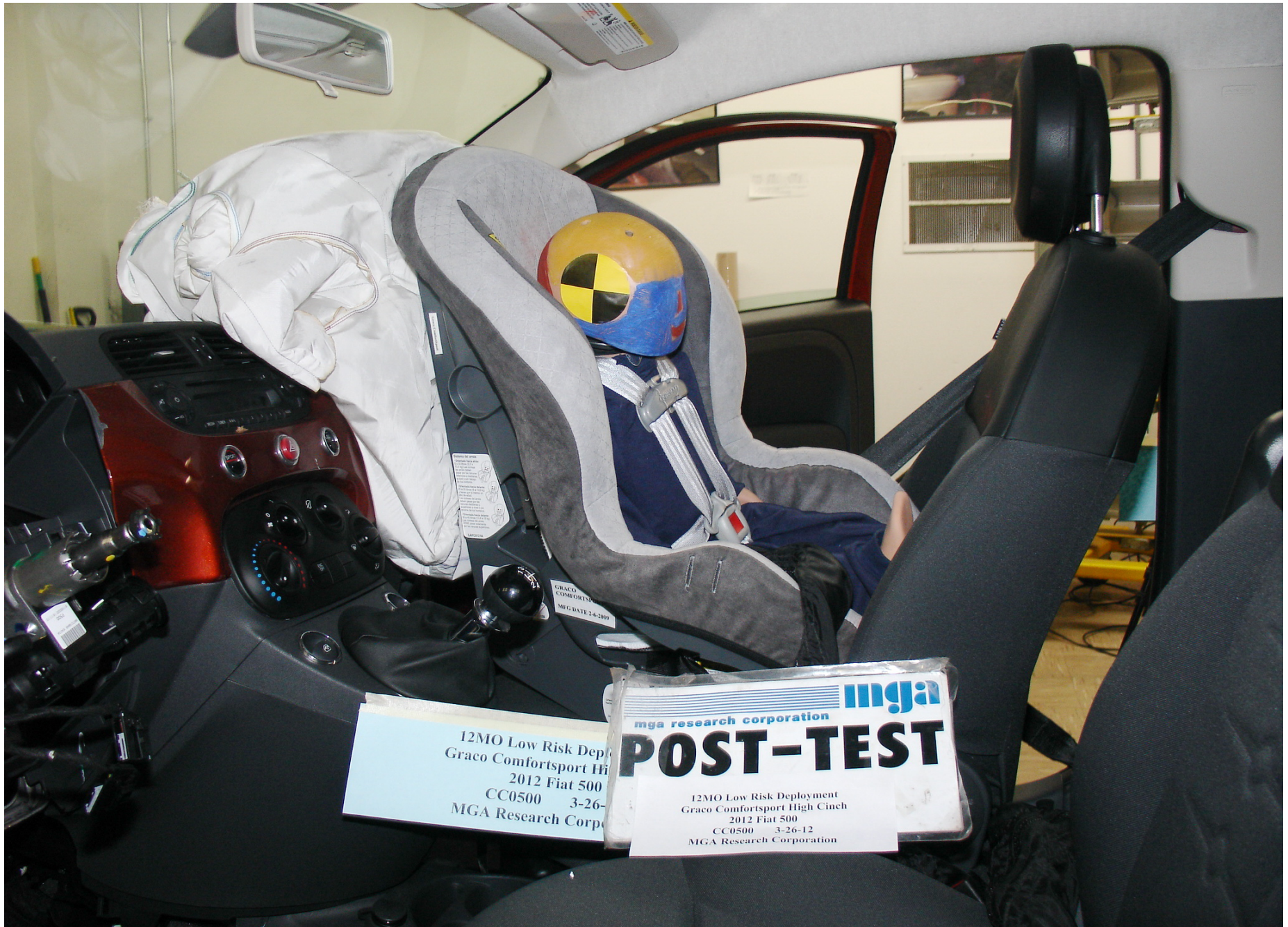
Post-Test 12 Mo Pass. Dummy Left Side View (Graco Comfortsport High Cinch)
