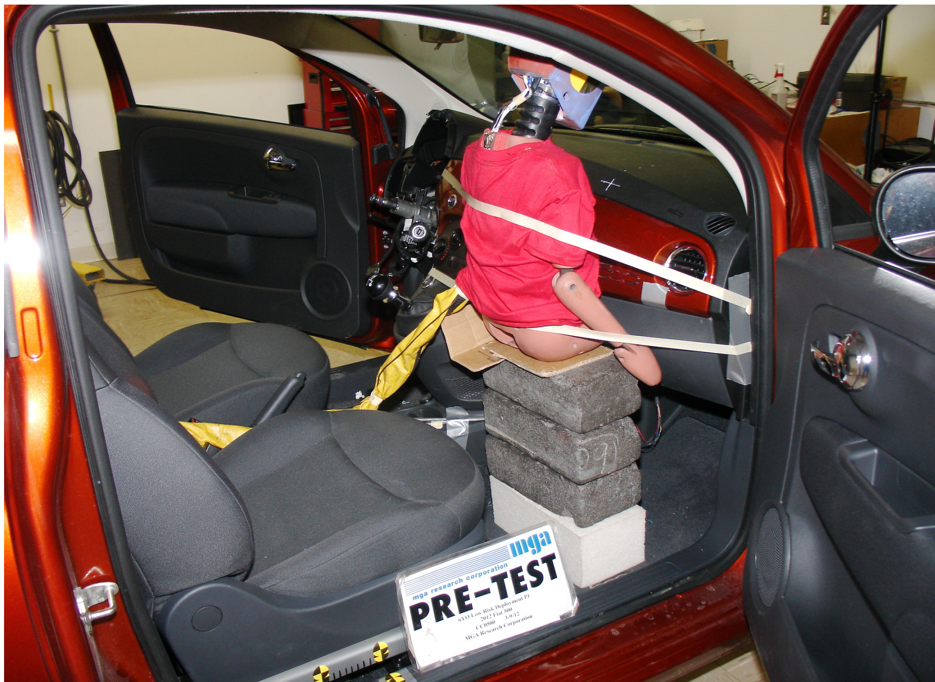
Pre-Test 6YO P1 Passenger Dummy Right Side View
