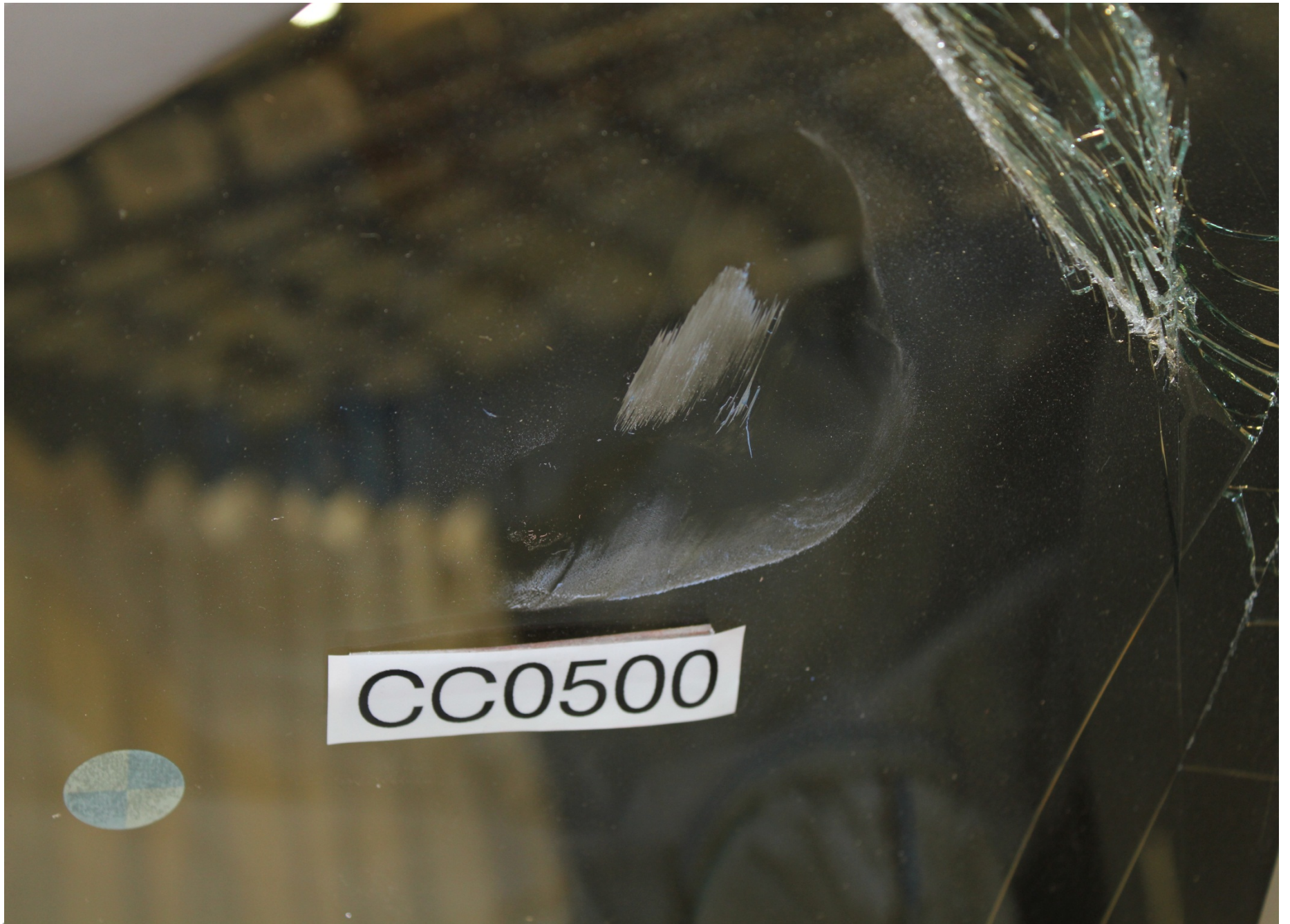
Post-Test Passenger Dummy Head Contact (windshield)
