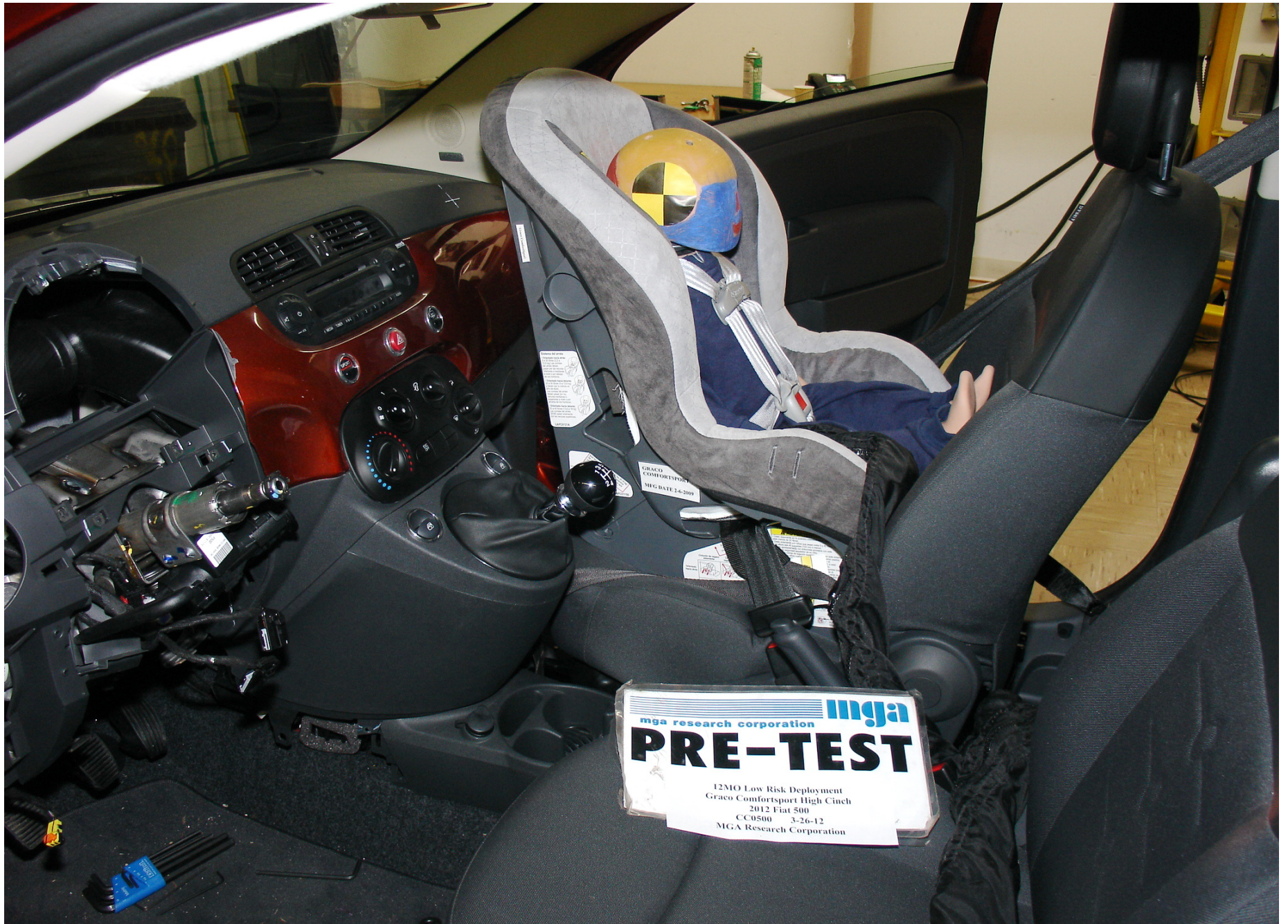
Pre-Test 12 Mo Pass. Dummy Left Side View (Graco Comfortsport High Cinch)
