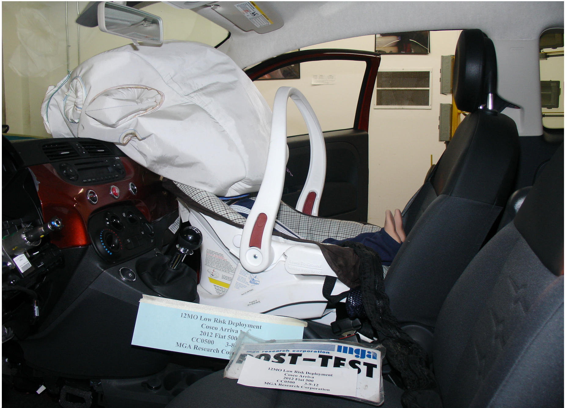
Post-Test 12 Mo Pass. Dummy Left Side View (Cosco Arriva Low Cinch)
