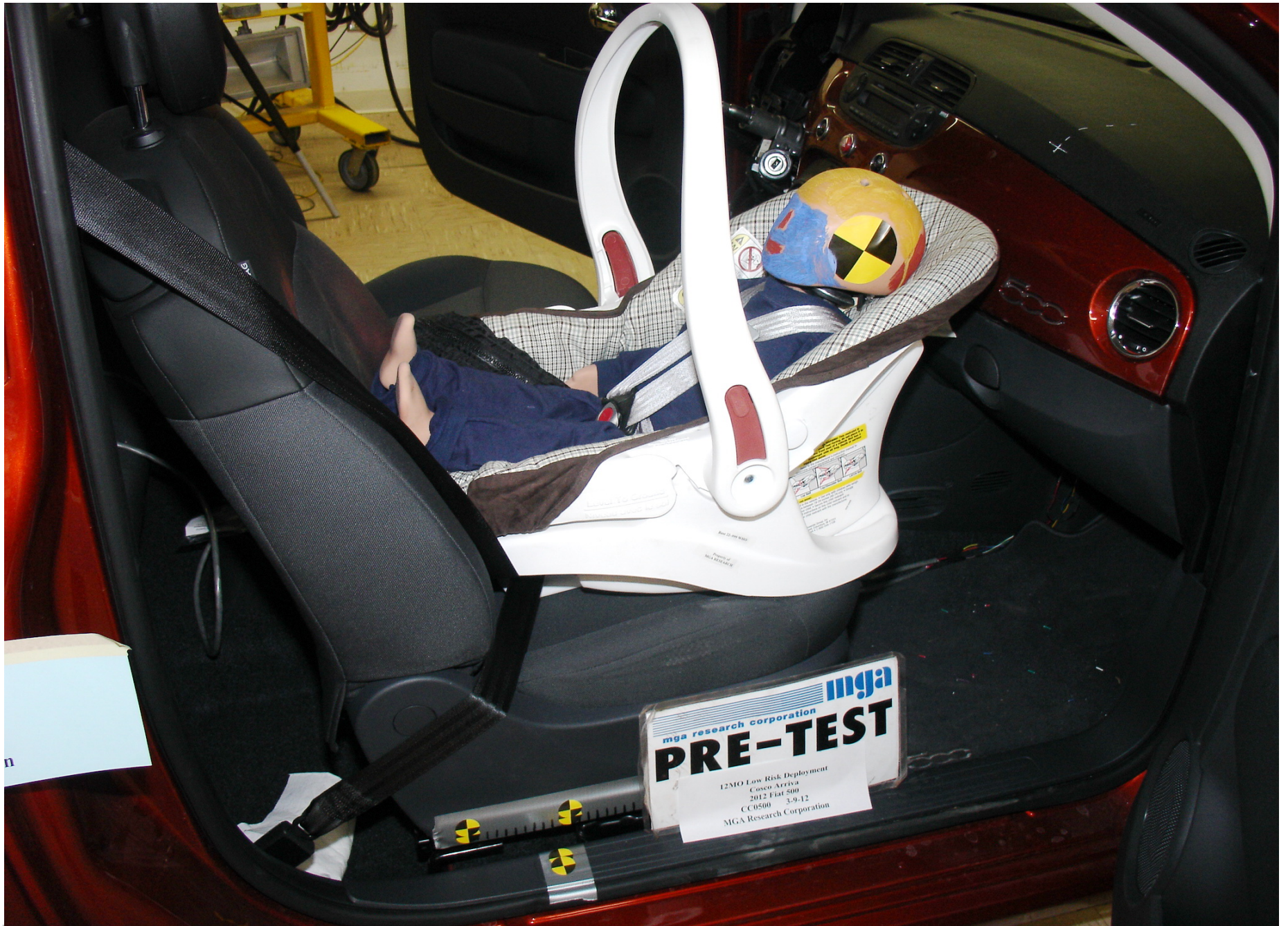
Pre-Test 12 Mo Pass. Dummy Right Side View (Cosco Arriva Low Cinch)
