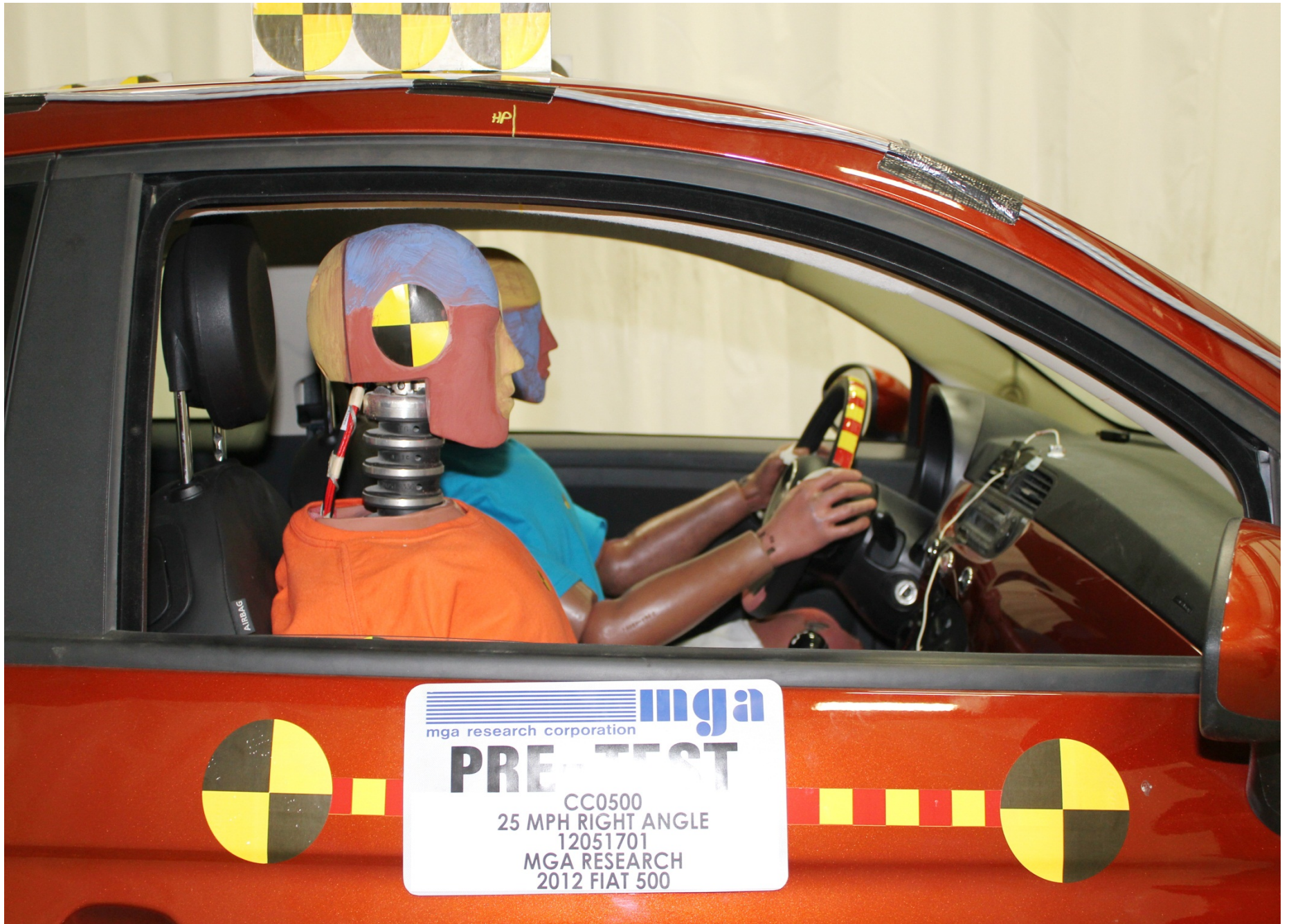
Pre-Test Passenger Dummy Position Right Side View
