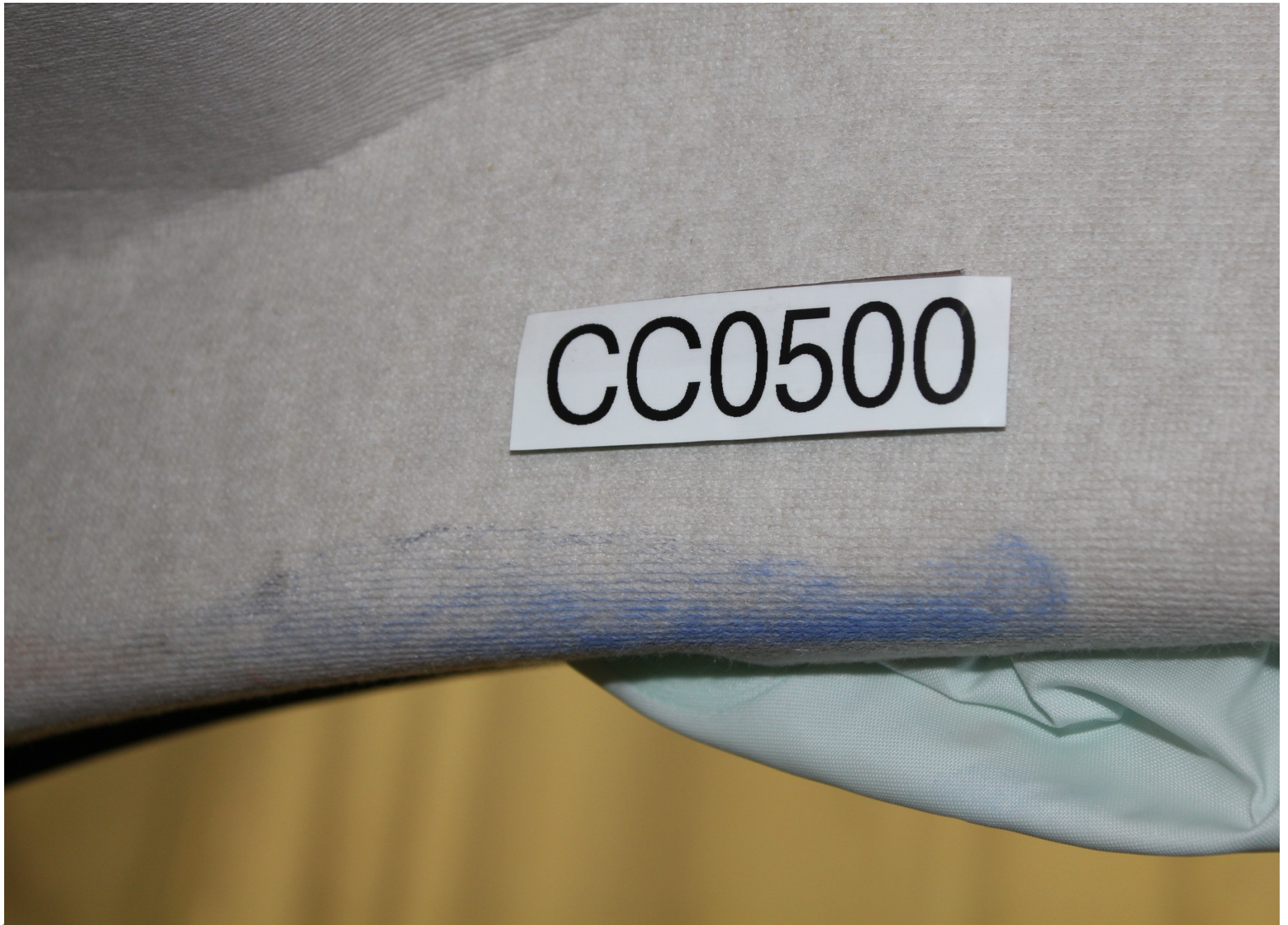
Post-Test Passenger Dummy Head Contact (headliner)
