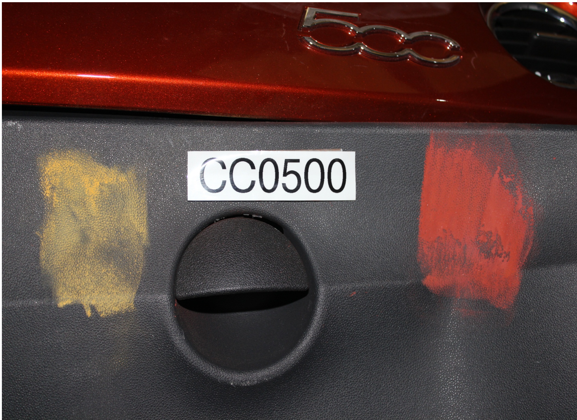
Post-Test Passenger Dummy Knee Contact
