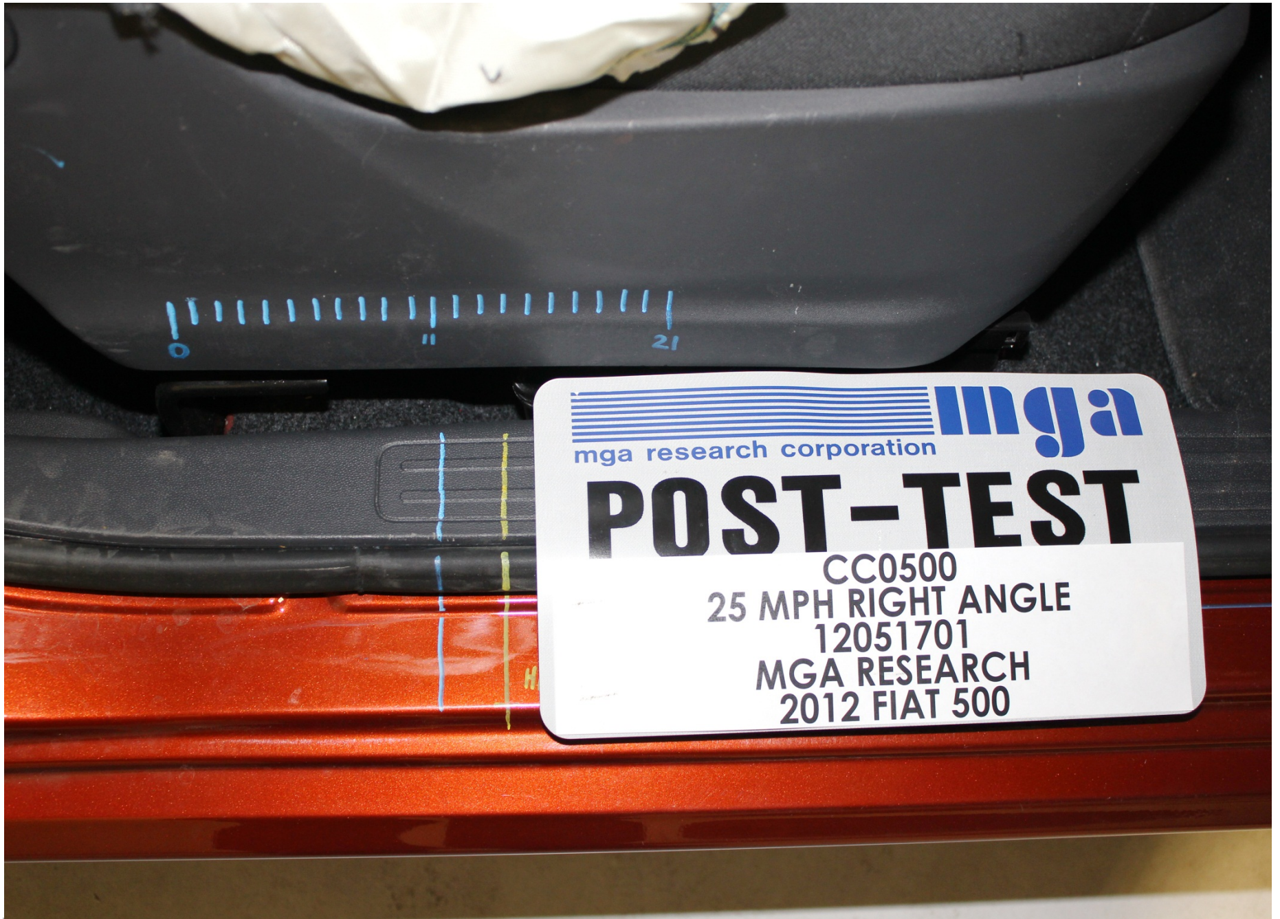
Post-Test Passenger Dummy Seat Position
