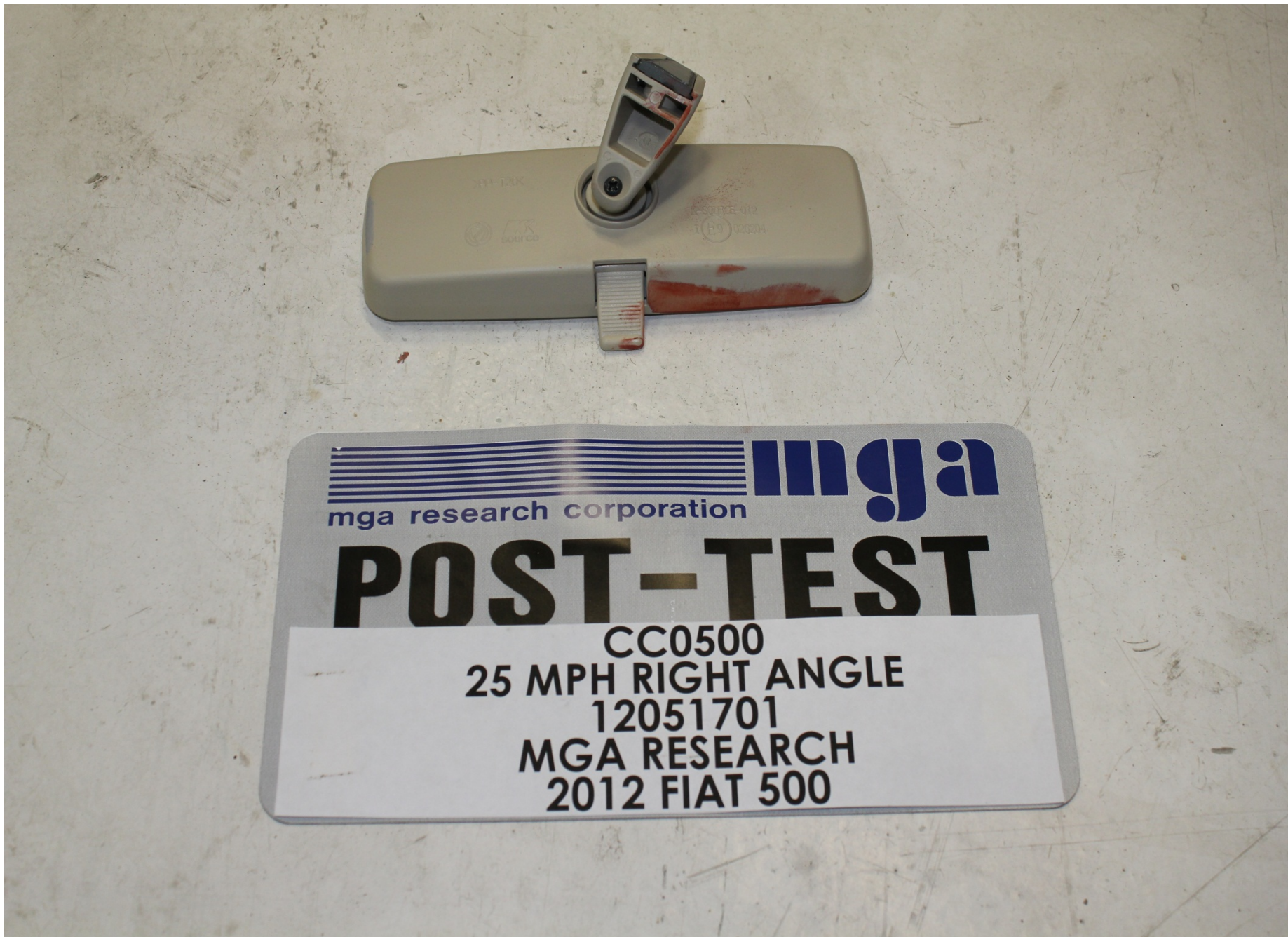
Post-Test Driver Dummy Head Contact (rearview mirror)
