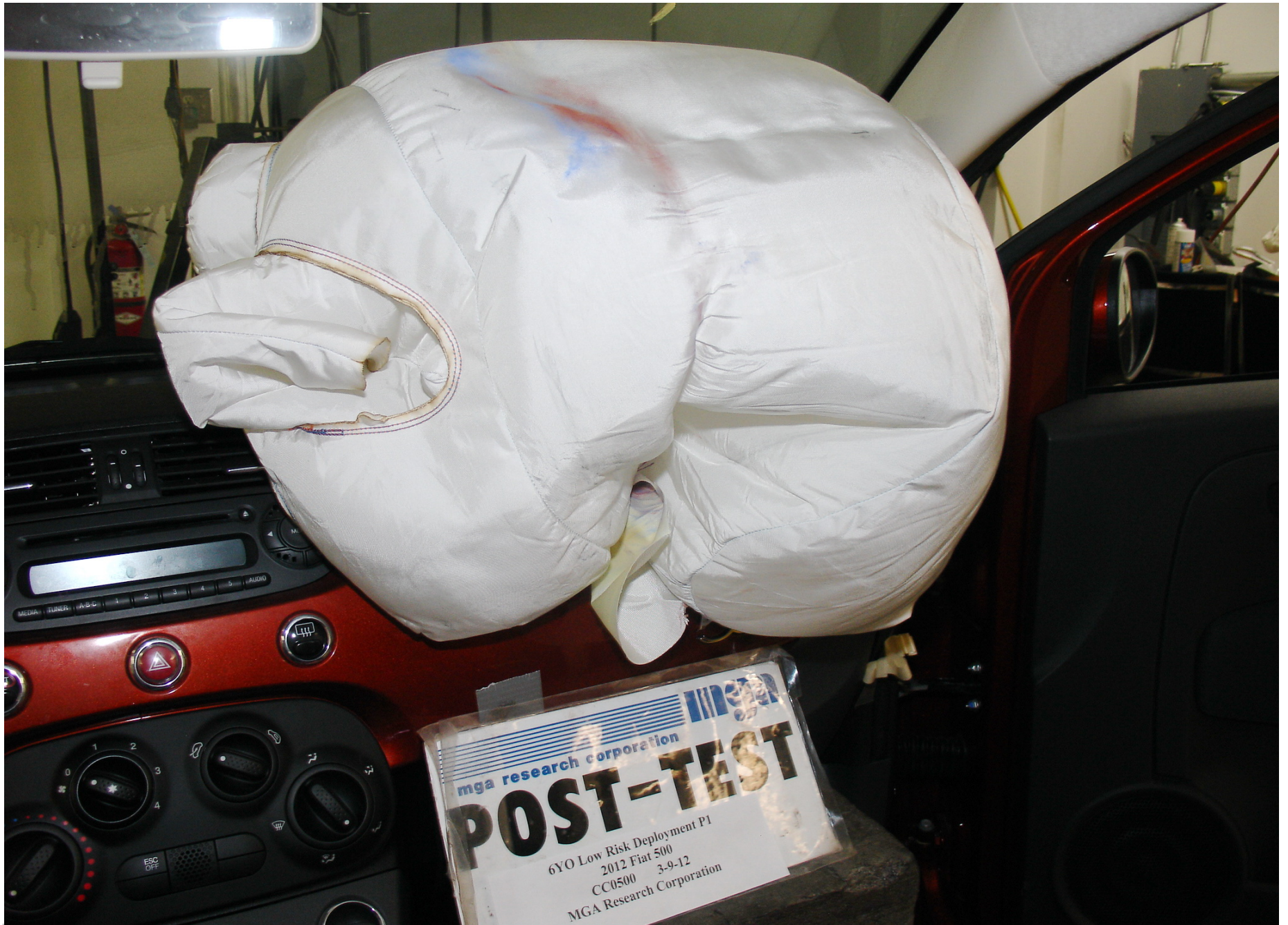
Post-Test 6YO P1 Passenger Dummy Airbag Left Side View
