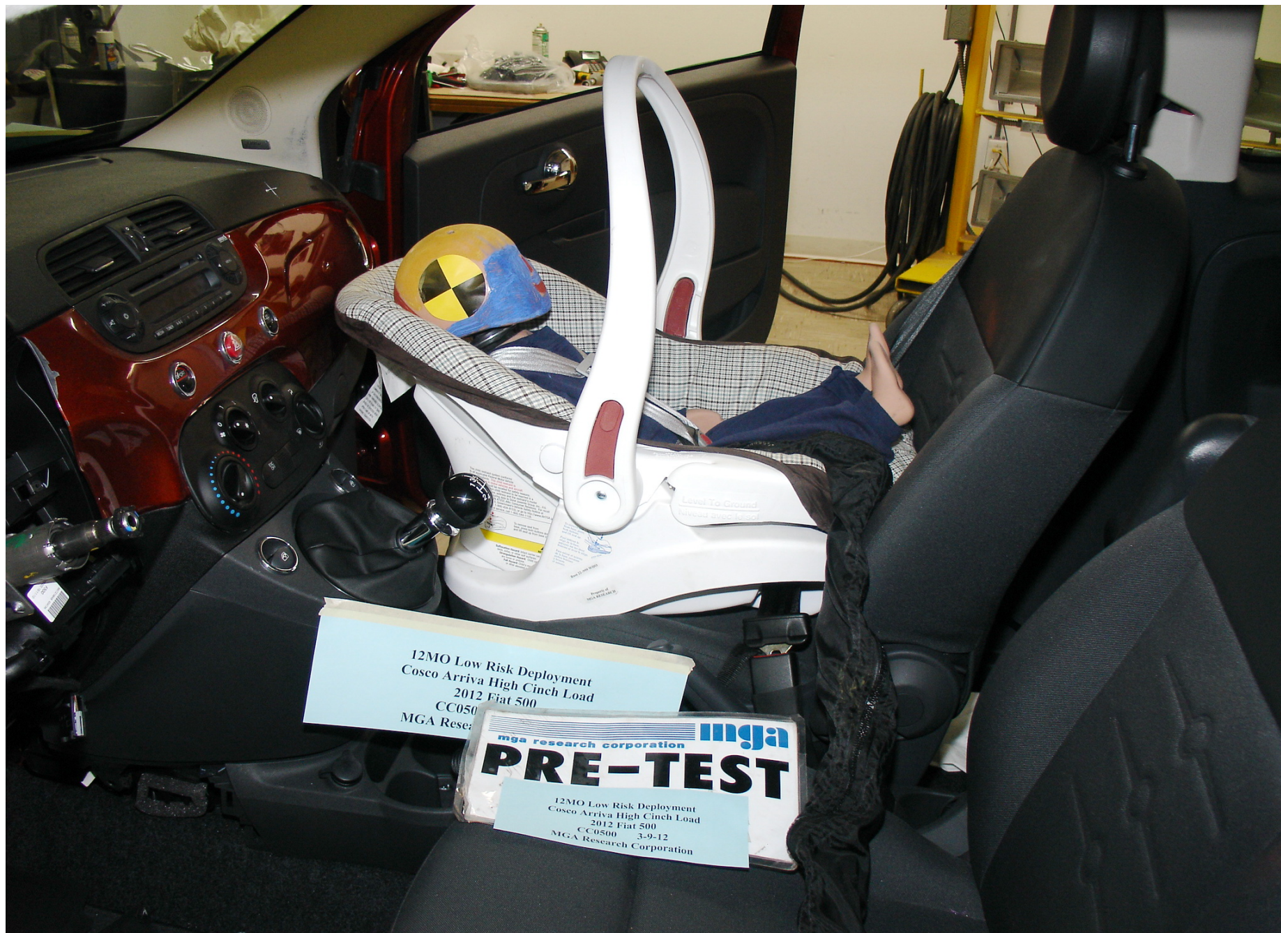
Pre-Test 12 Mo Pass. Dummy Left Side View (Cosco Arriva High Cinch)
