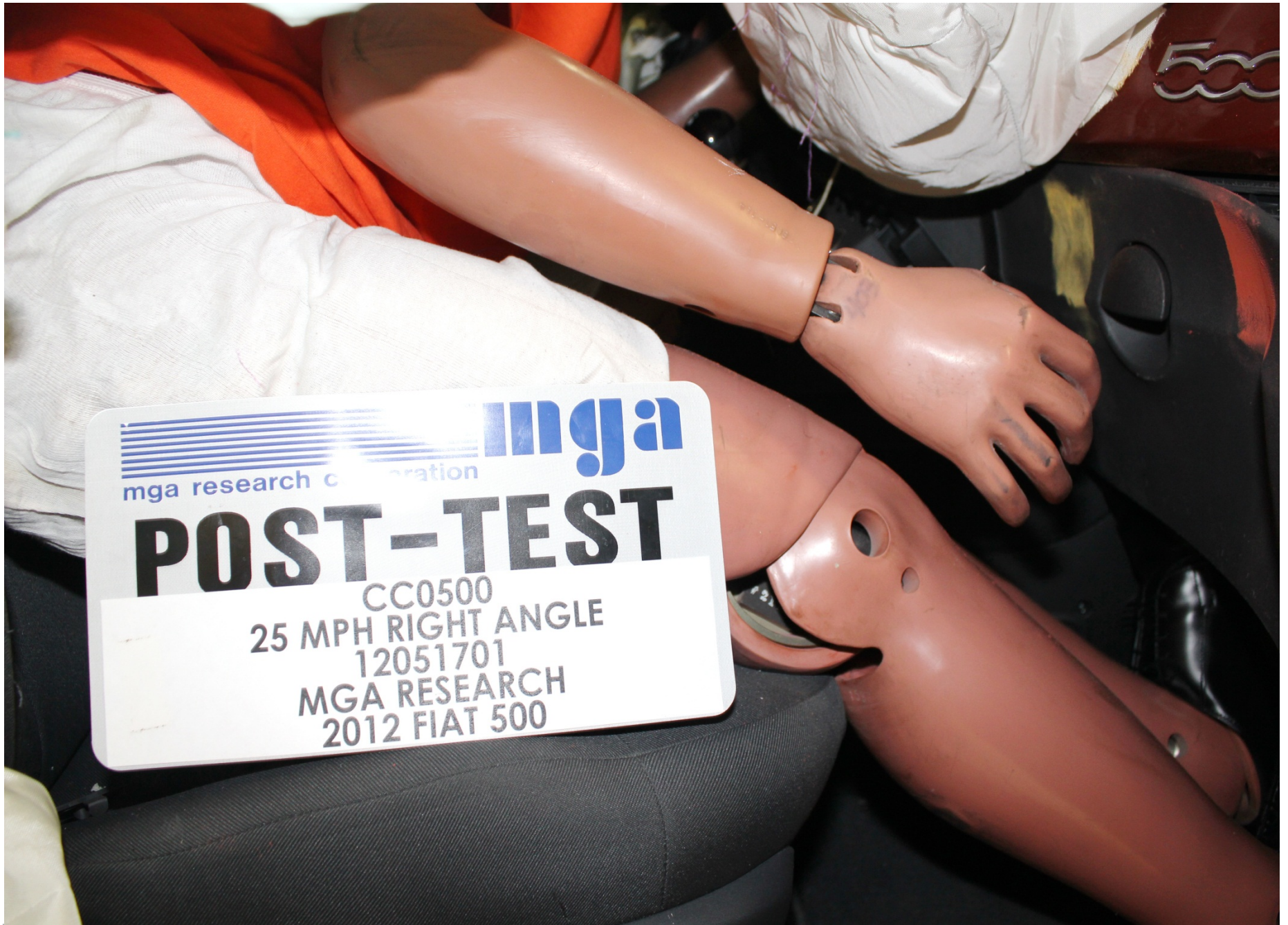
Post-Test Passenger Side Knee Bolster View
