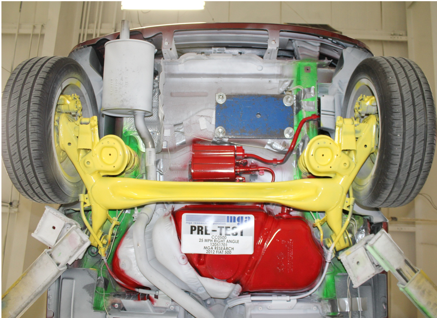
Pre-Test Rear Underbody View
