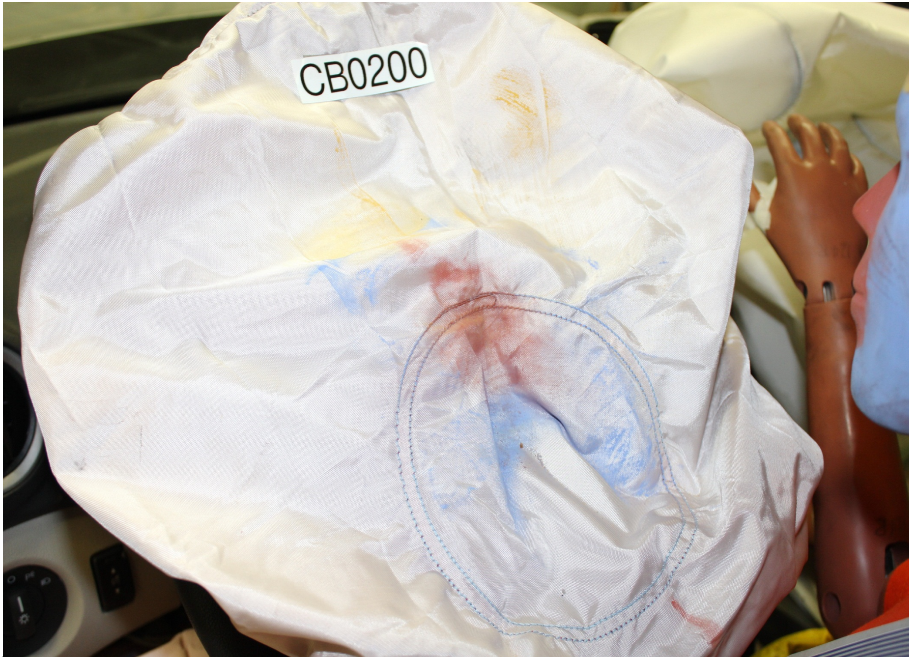
Post-Test Driver Dummy Airbag Contact
