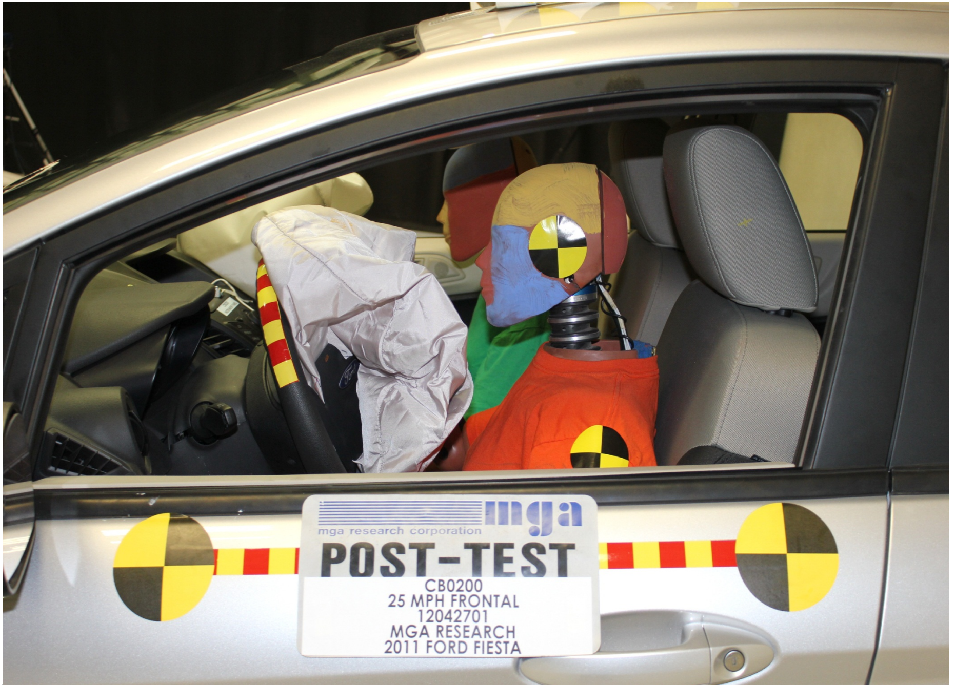
Post-Test Driver Dummy Position Left Side View
