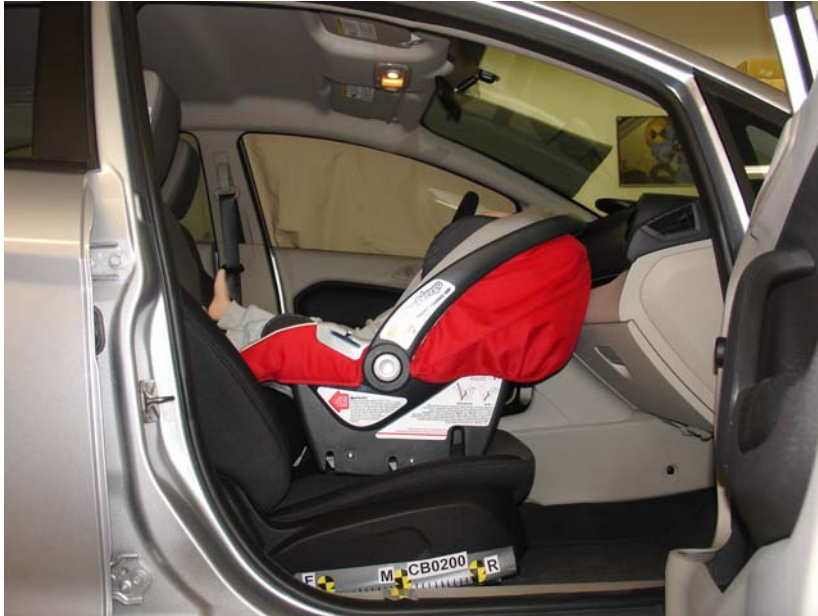
Peg Perego Viaggio WOut Base, Unbelted, Rear Facing, Forward Seat Track
