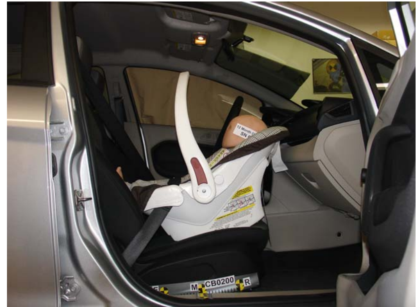
Cosco Arriva WOut Base, Belted, Rear Facing, Middle Seat Track
