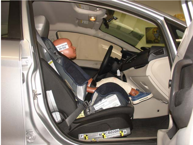
3-Year-Old Forward Facing Cosco High Back Booster Belted, Forward Seat Track
