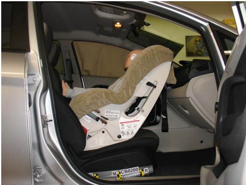
Britax Roundabout Rear Facing Unbelted, Middle Seat Track
