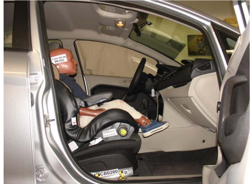
3-Year-Old Forward Facing Evenflo Generations Crs Cinched With Harness, Rearward Seat Track
