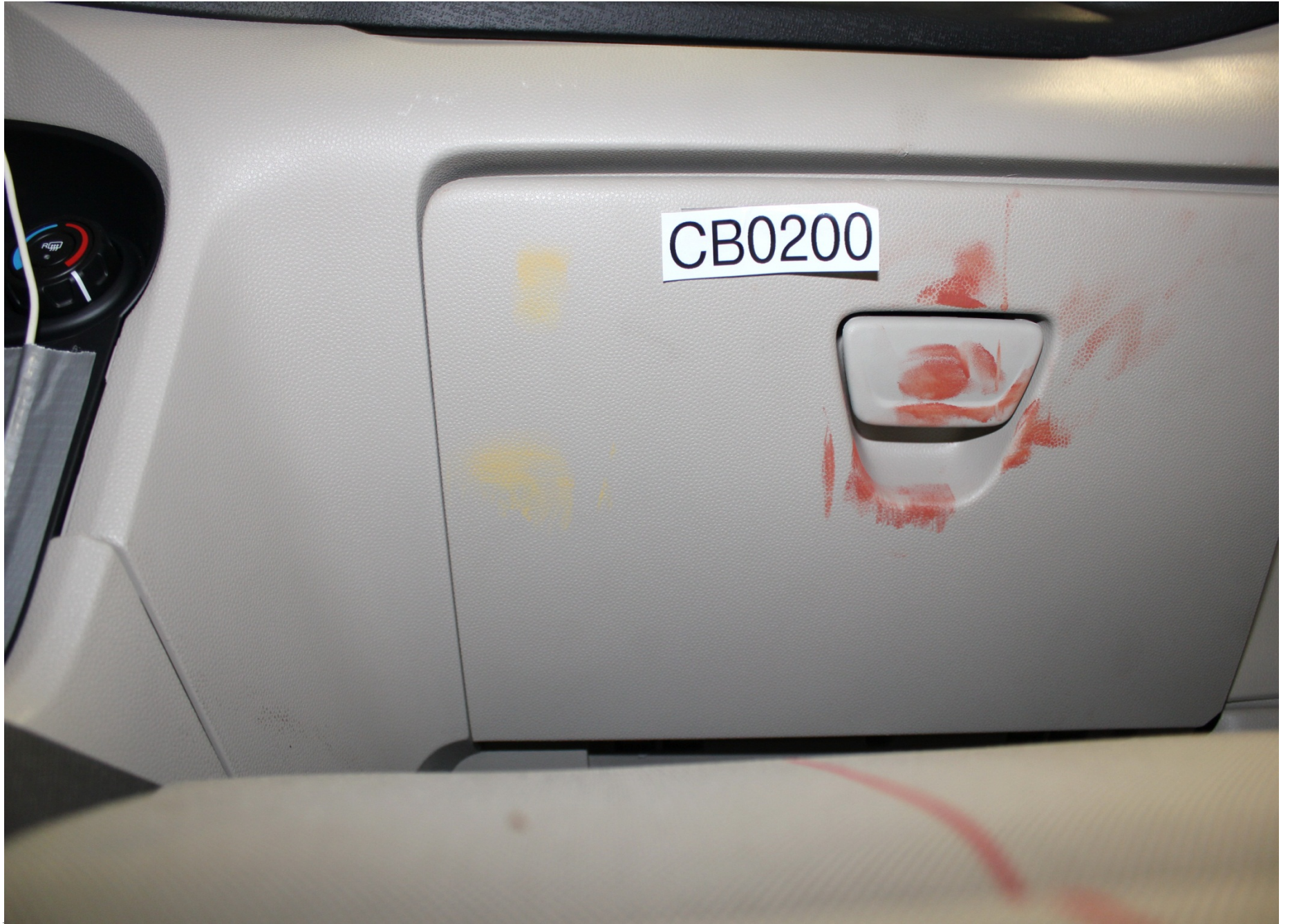
Post-Test Passenger Dummy Knee Contact
