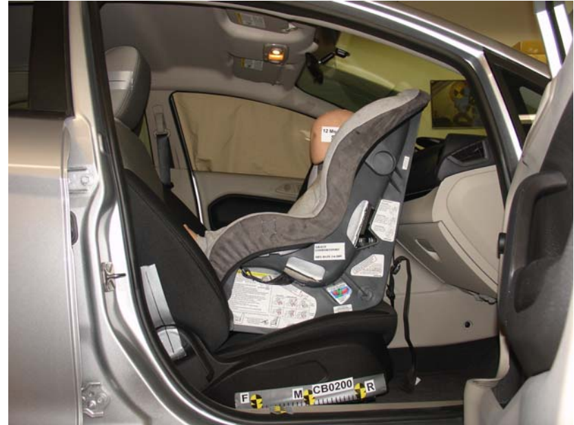
Graco Comfortsport Rear Facing Unbelted, Forward Seat Track
