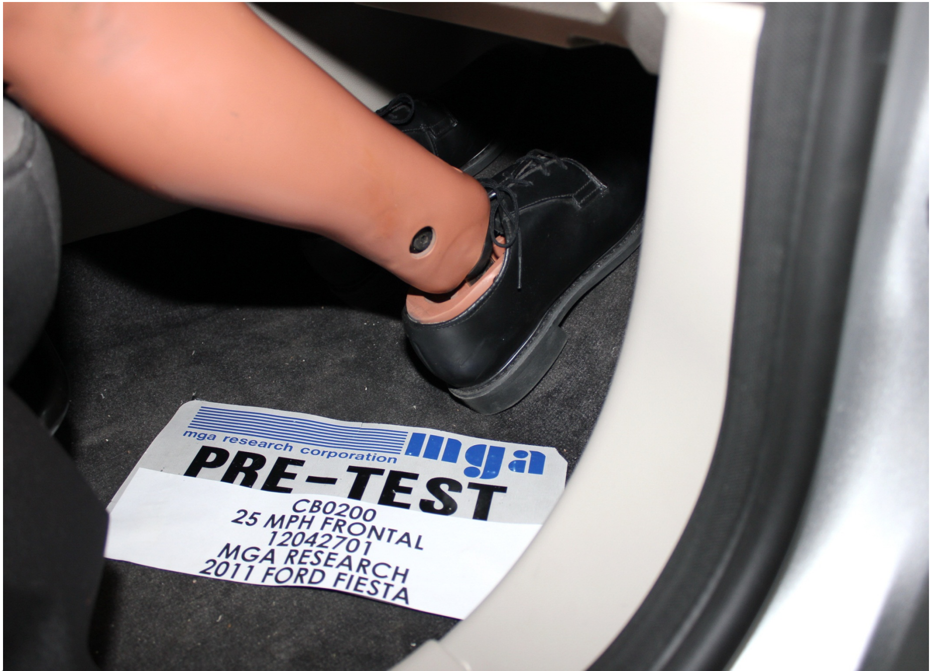
Pre-Test Passenger Dummy Feet Position
