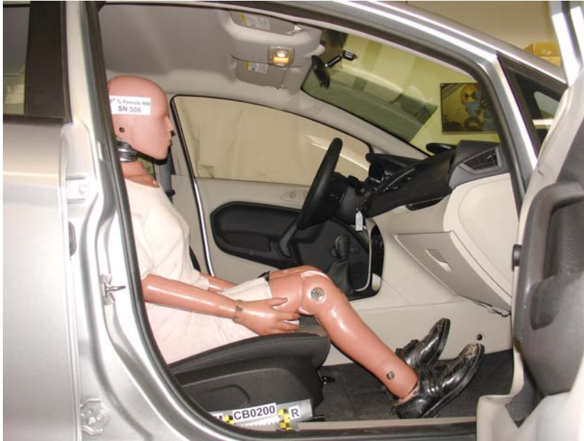
Unbelted 5th Percentile Female Dummy Reactivation, Rearward Seat Track
