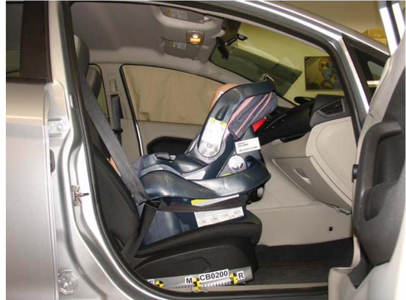
Graco Snugride WBase, Belted, Rear Facing, Middle Seat Track
