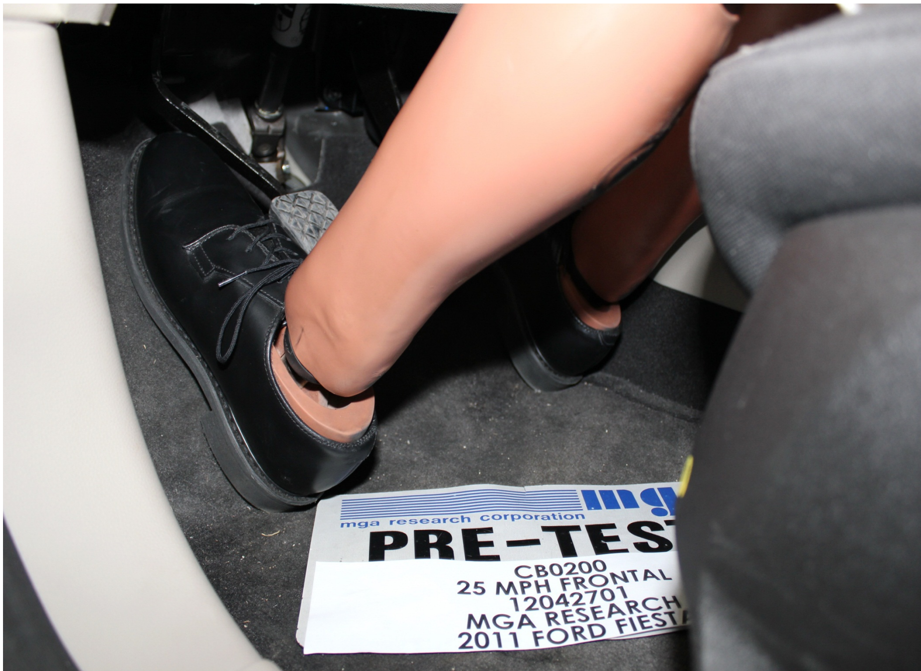
Pre-Test Driver Dummy Feet Position
