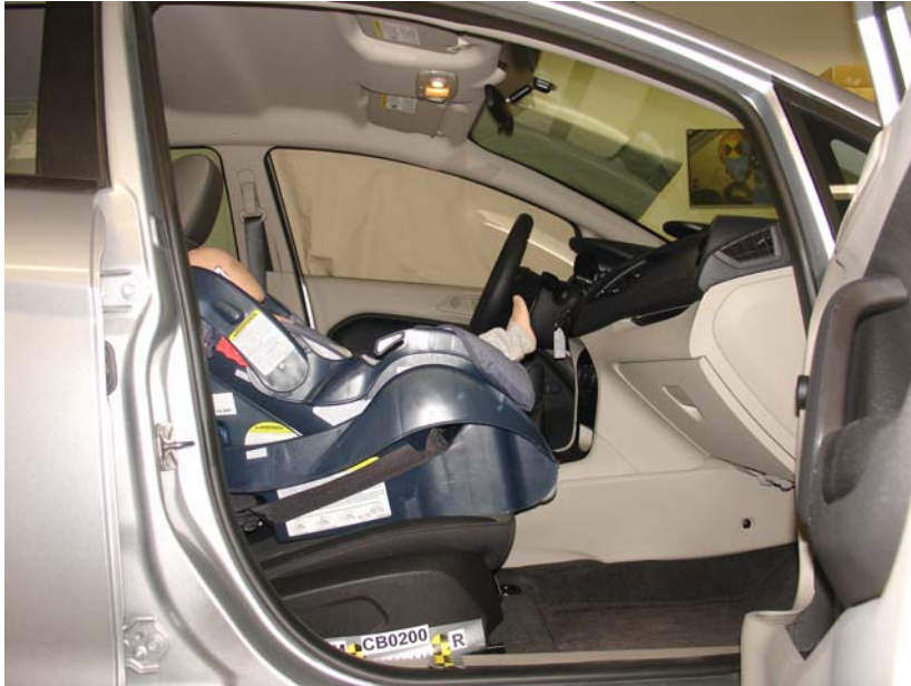
Graco Snugride WBase, Unbelted, Forward Facing, Rearward Seat Track
