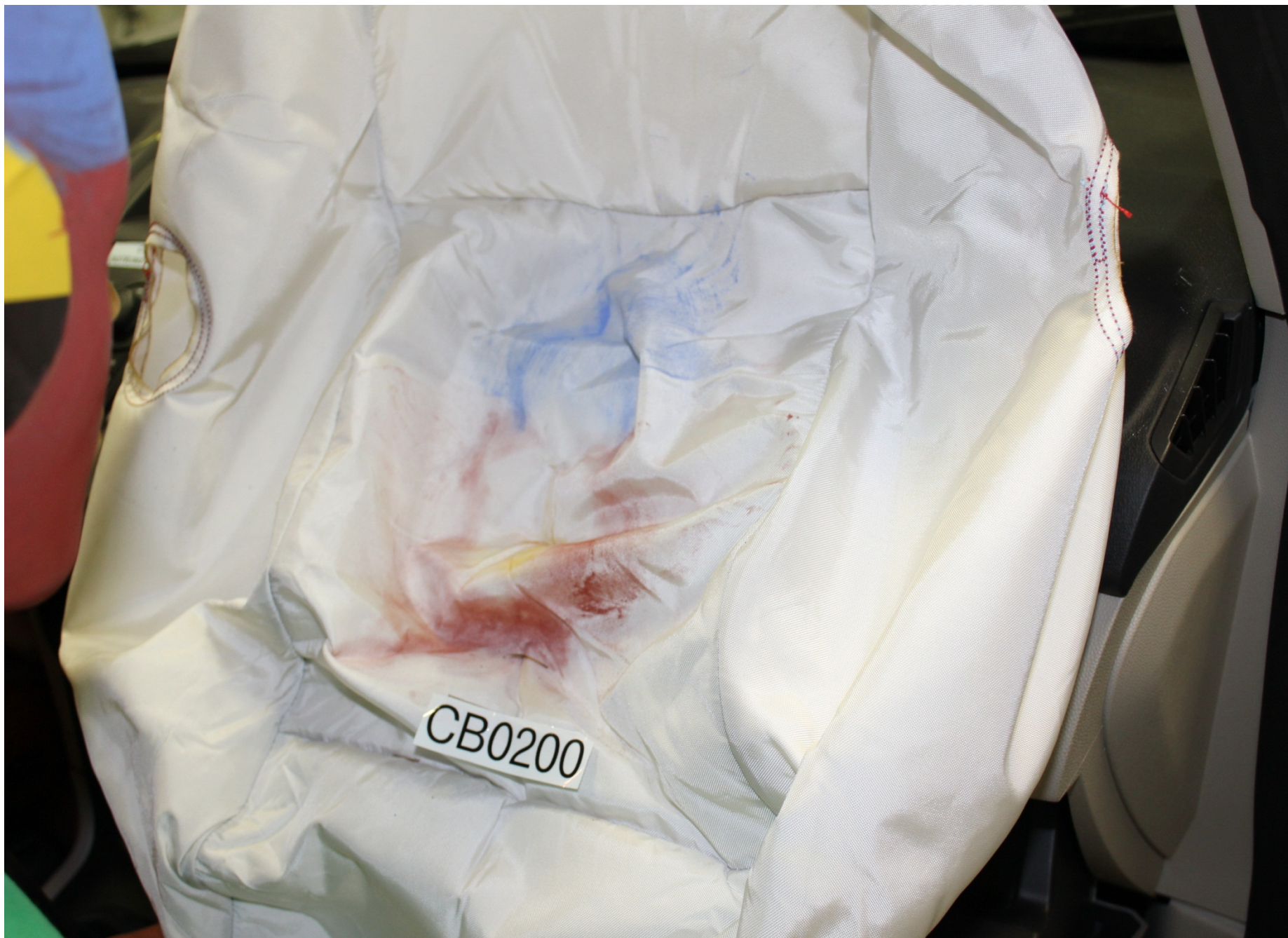
Post-Test Passenger Dummy Airbag Contact
