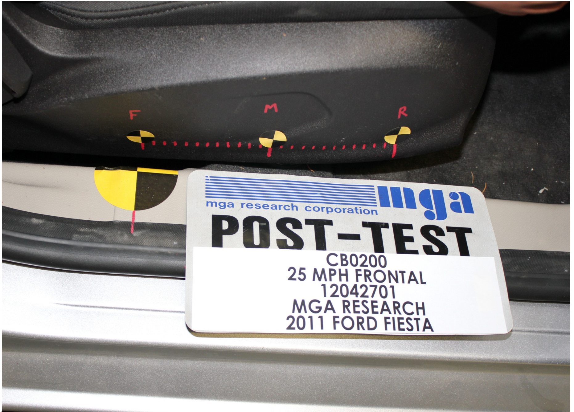
Post-Test Passenger Dummy Seat Position
