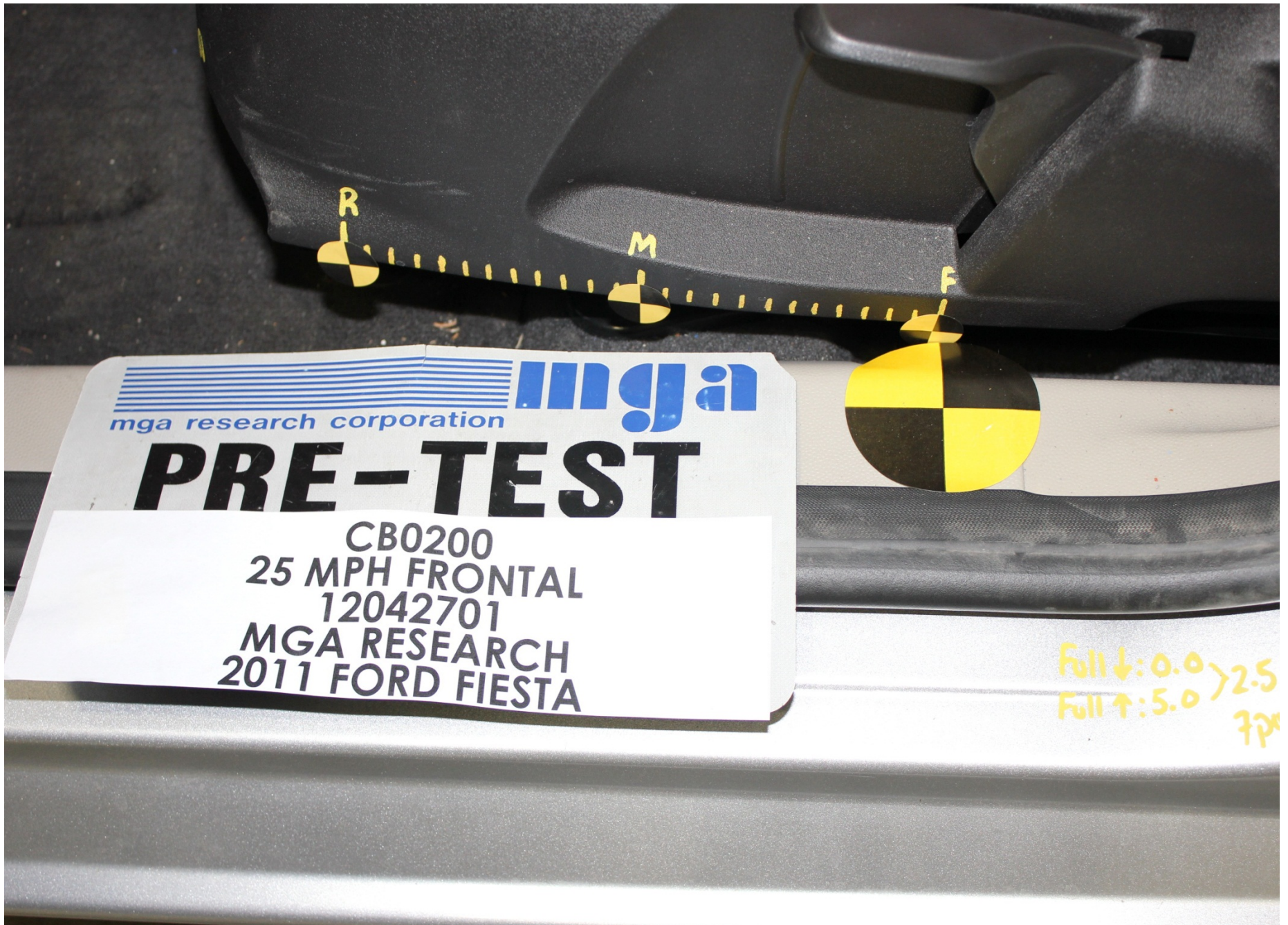
Pre-Test Driver Dummy Seat Position
