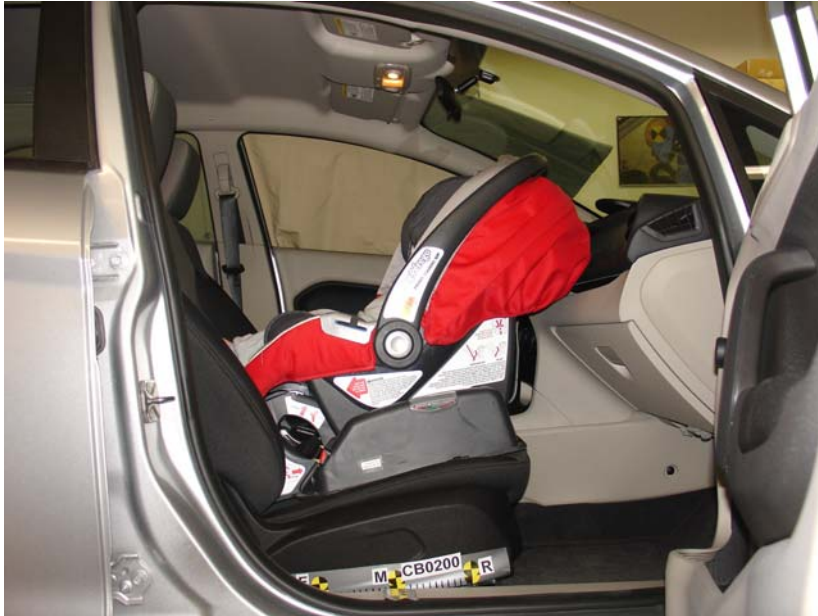
Peg Perego Viaggio WBase, Unbelted, Rear Facing, Middle Seat Track
