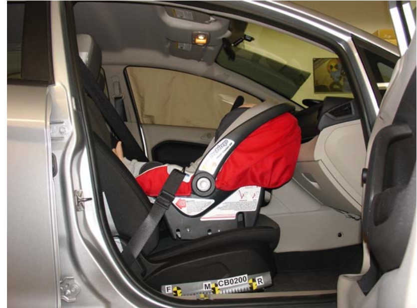
Peg Perego Viaggio WOut Base, Belted, Rear Facing, Forward Seat Track
