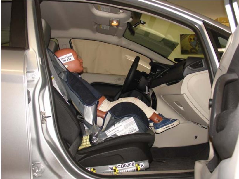
3-Year-Old Forward Facing Cosco High Back Booster Cinched With Harness, Middle Seat Track
