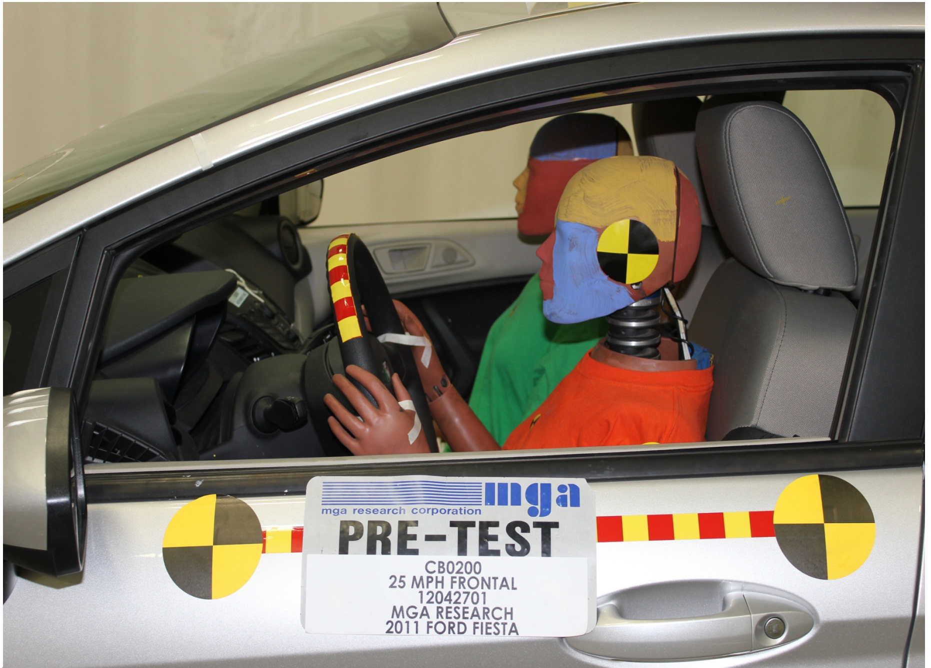
Pre-Test Driver Dummy Position Left Side View
