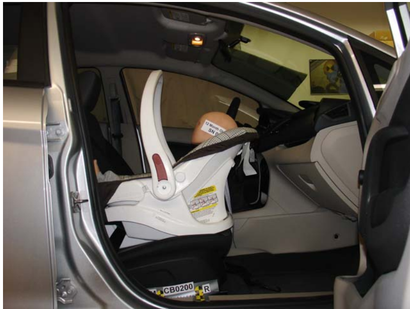
Cosco Arriva WBase, Belted, Rear Facing, Rearward Seat Track
