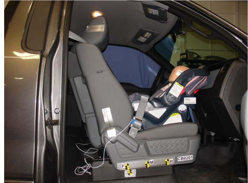
Graco Snugride WOut Base, Belted, Rear Facing, Forward Seat Track
