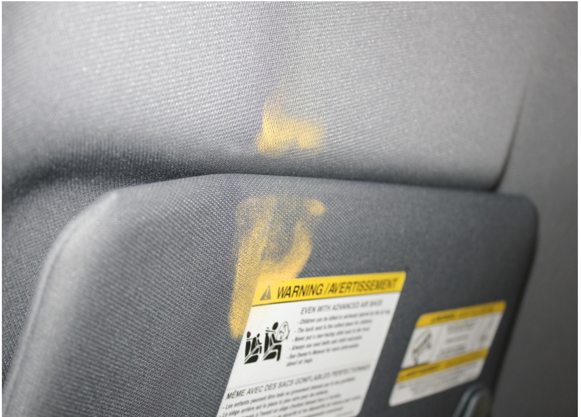
Post-Test Driver Dummy Head Contact (headliner/visor)
