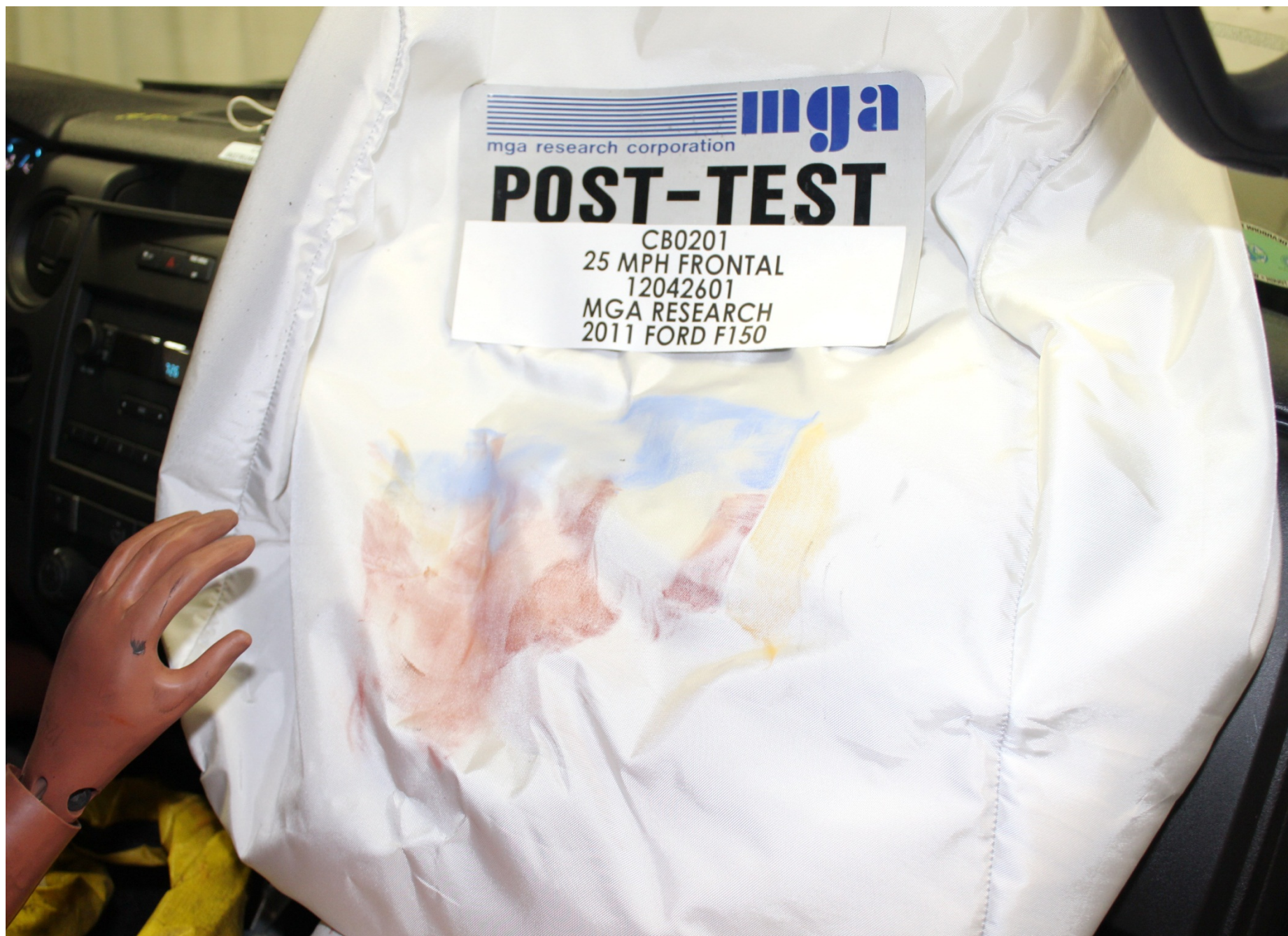
Post-Test Passenger Dummy Airbag Contact
