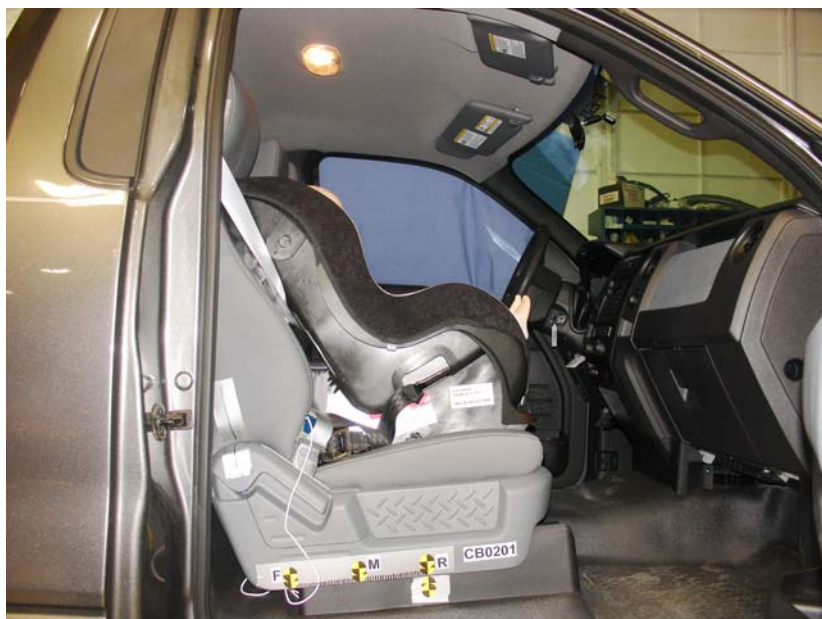
Evenflo Tribute Forward Facing Belted, Rearward Seat Track
