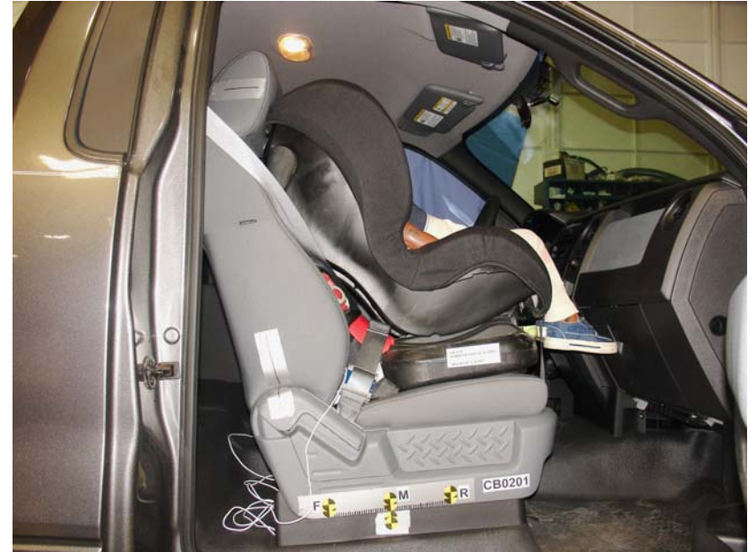
3-Year-Old Forward Facing Graco Toddler Safeseat Step 2 Belted, Middle Seat Track
