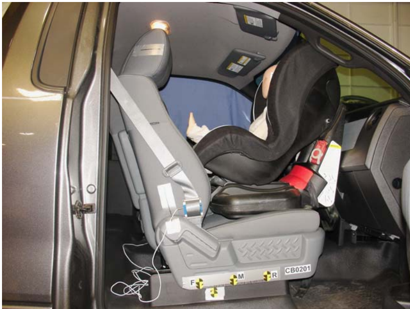
Graco Toddler Safeseat Step 2 Rear Facing Unbelted, Forward Seat Track
