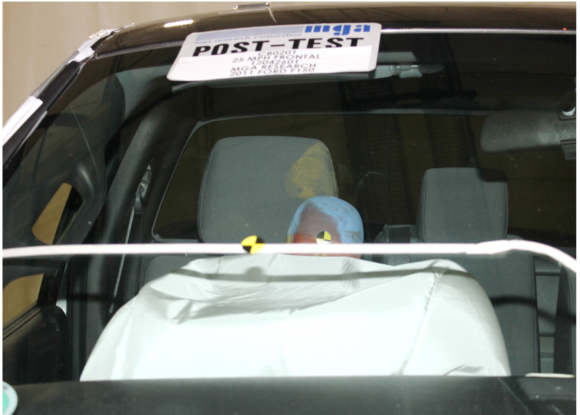
Post-Test Passenger Dummy Front View (head position)
