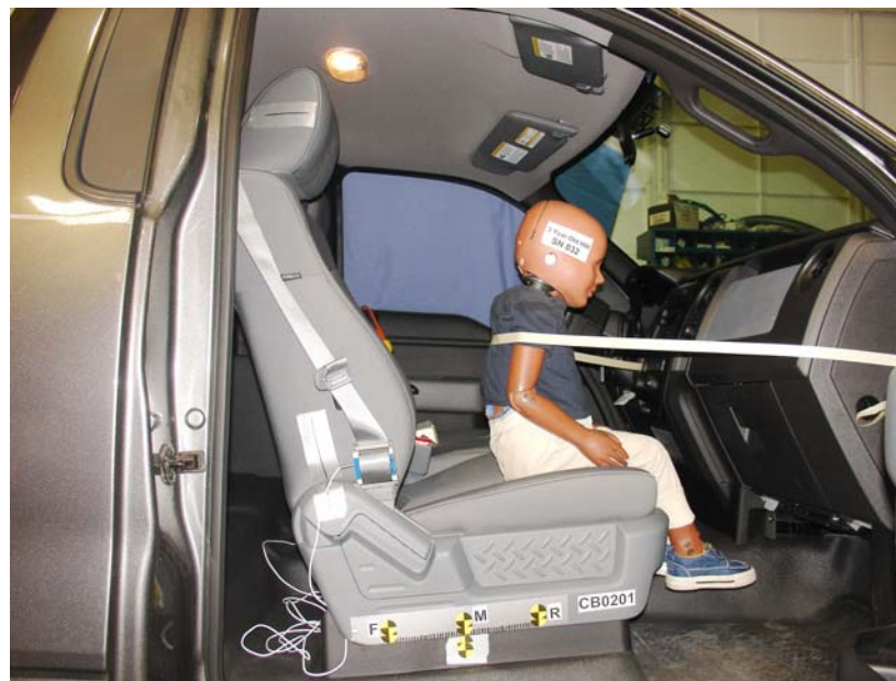
3-Year-Old Unbelted, Middle Seat Track, Position 4
