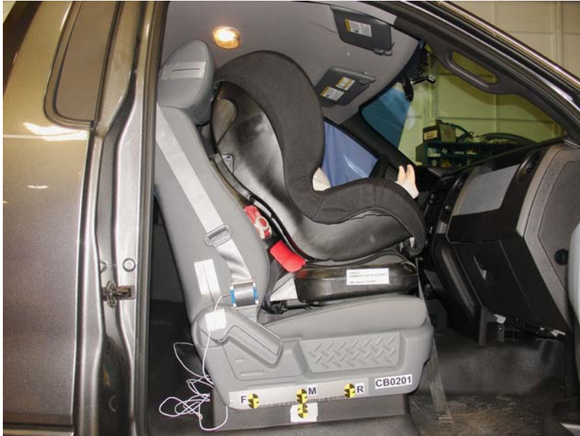
Graco Toddler Safeseat Step 2 Forward Facing Unbelted, Middle Seat Track
