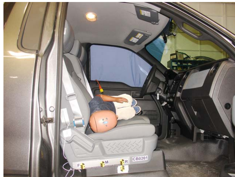
3-Year-Old Unbelted, Rearward Seat Track, Position 8
