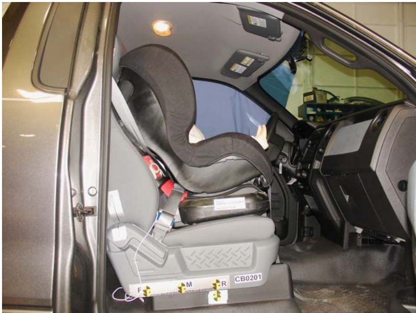
Graco Toddler Safeseat Step 2 Forward Facing Belted, Rearward Seat Track
