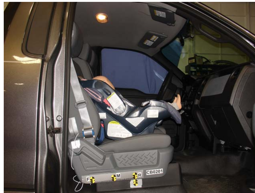
Graco Snugride WOut Base, Unbelted, Forward Facing, Rearward Seat Track
