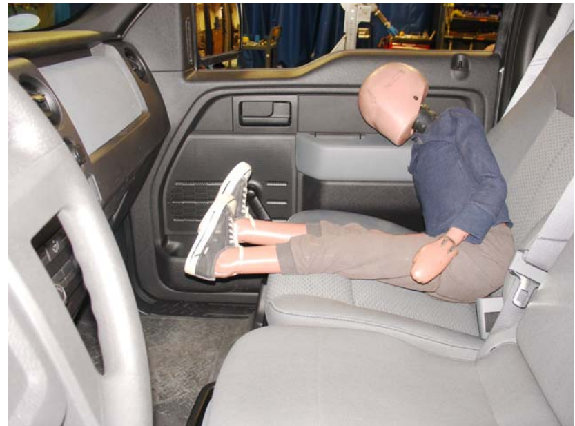
6-Year-Old Unbelted, Rearward Seat Track, Position 4
