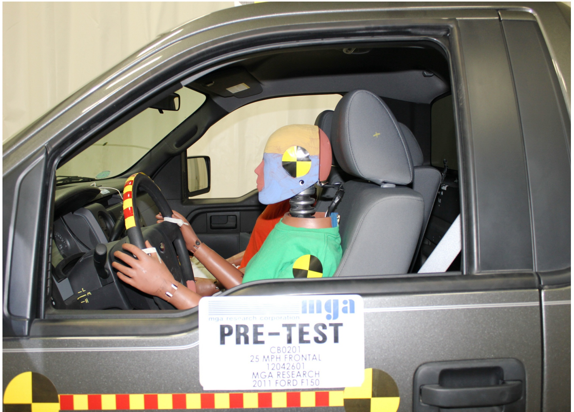
Pre-Test Driver Dummy Position Left Side View
