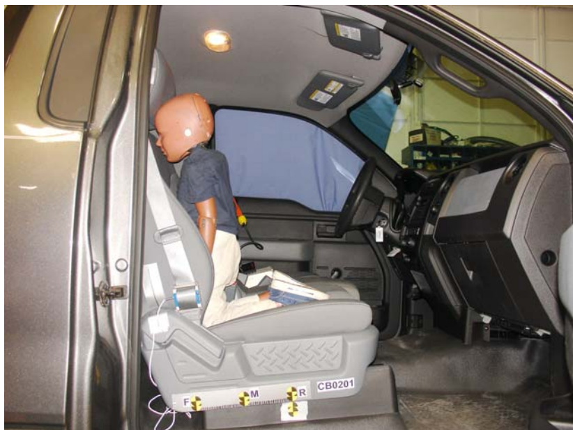
3-Year-Old Unbelted, Rearward Seat Track, Position 7
