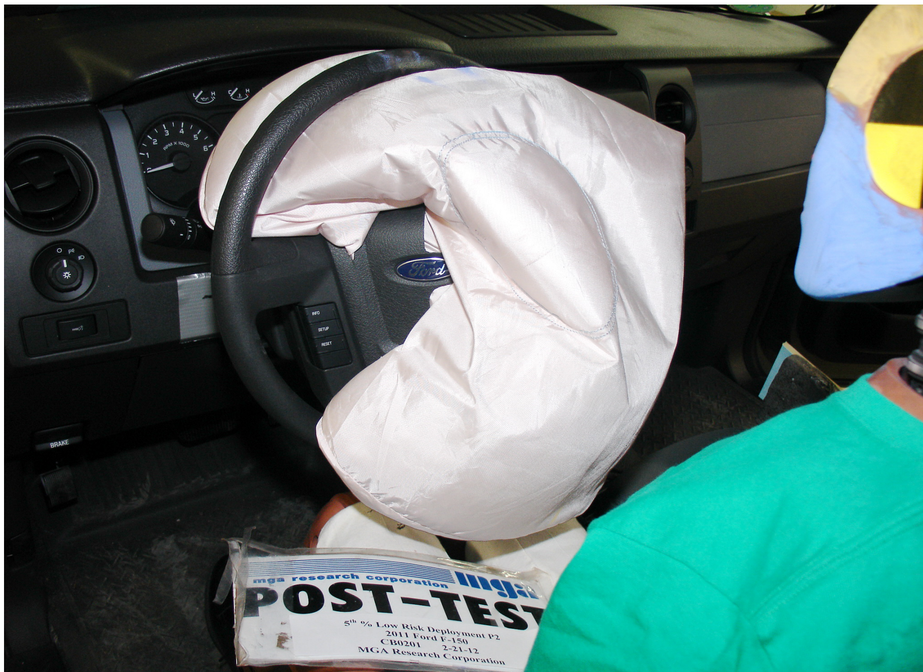
Post-Test 5th Fem. P2 Driver Dummy Airbag Left Side View
