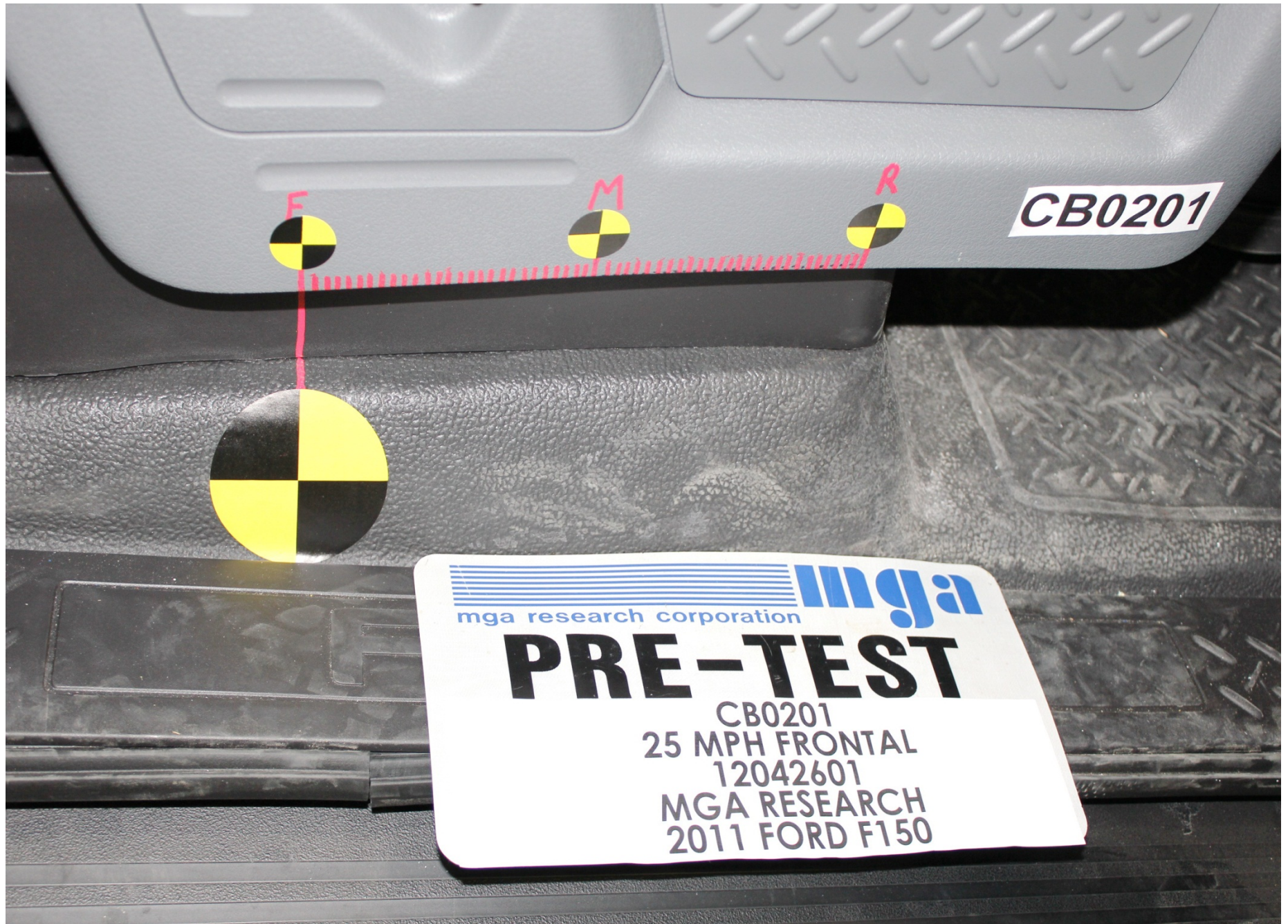
Pre-Test Passenger Dummy Seat Position
