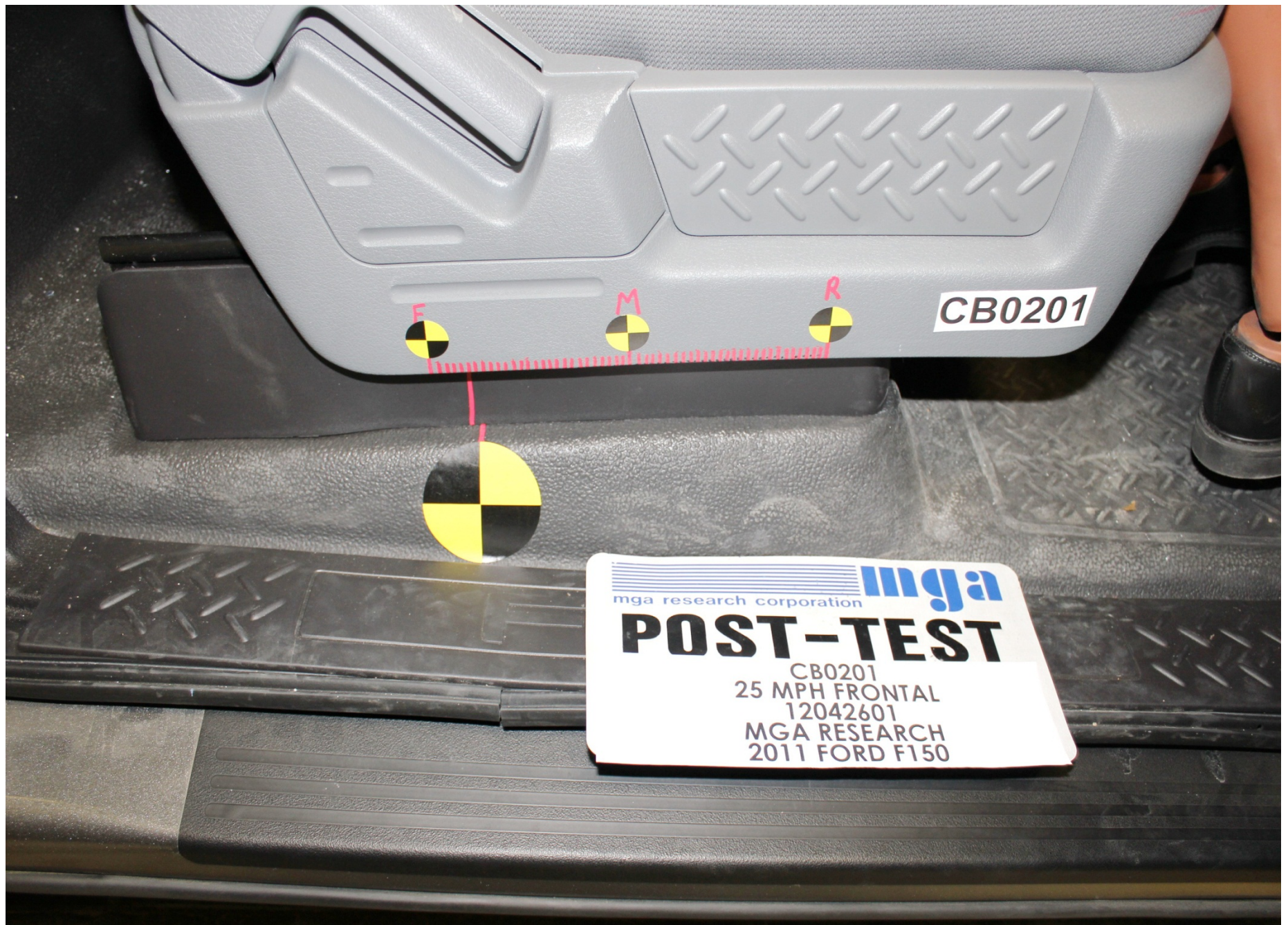
Post-Test Passenger Dummy Seat Position
