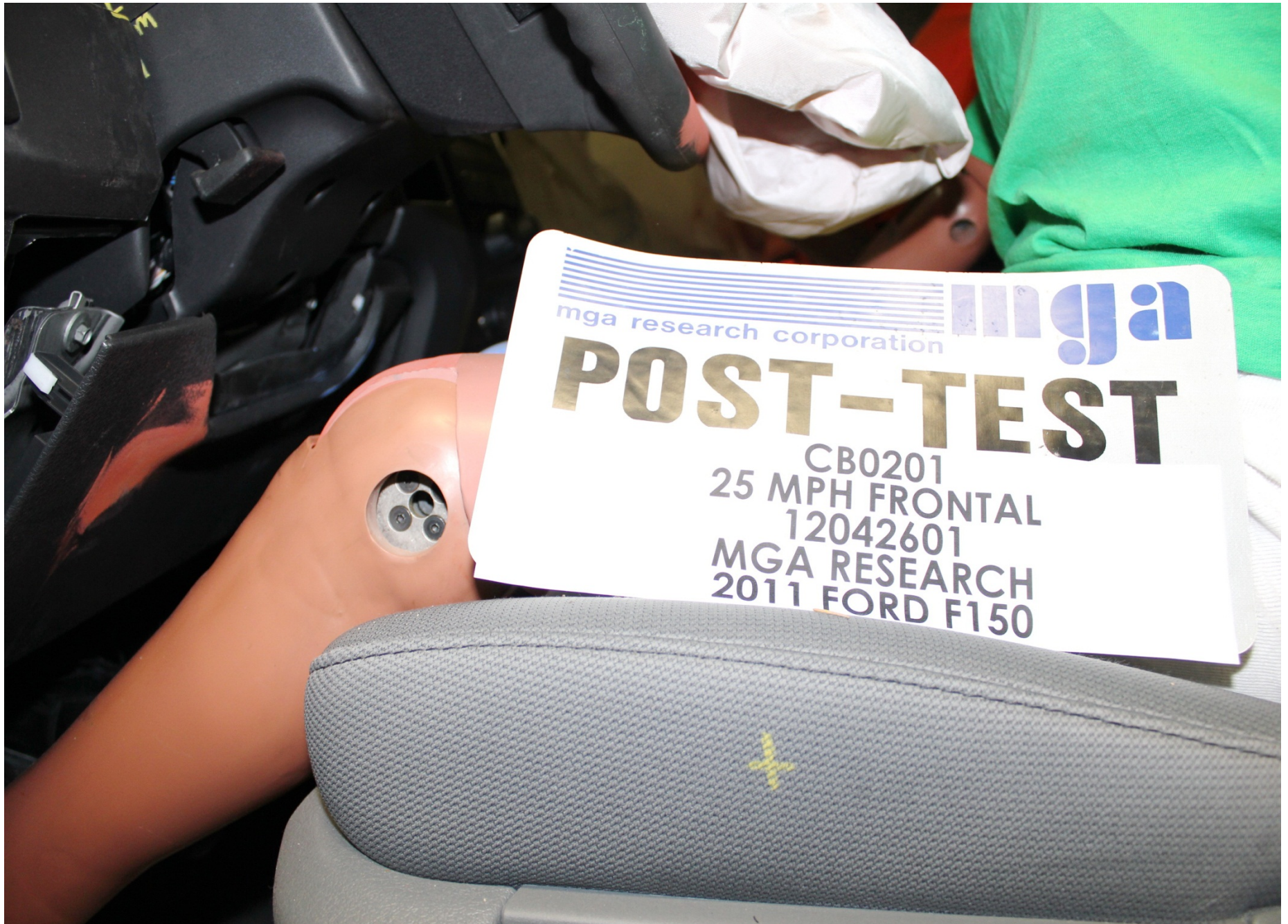
Post-Test Driver Side Knee Bolster View
