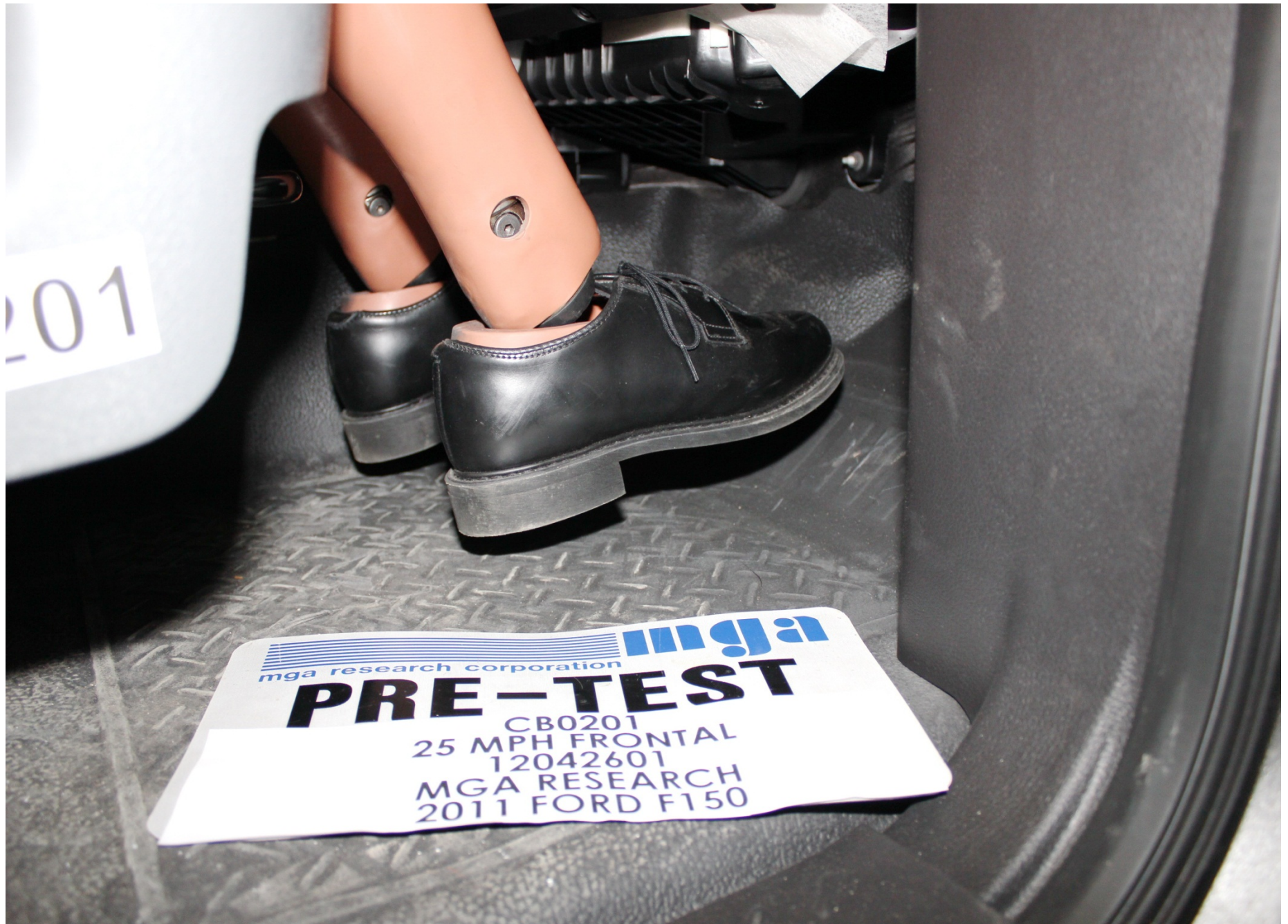
Pre-Test Passenger Dummy Feet Position
