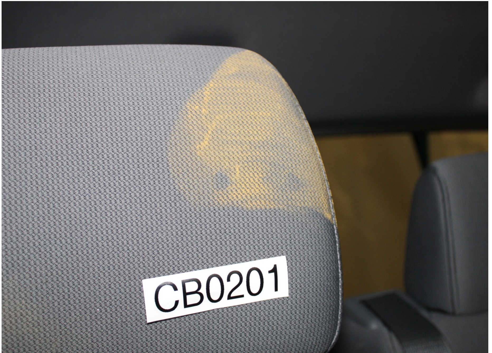
Post-Test Passenger Dummy Head Contact (headrest)
