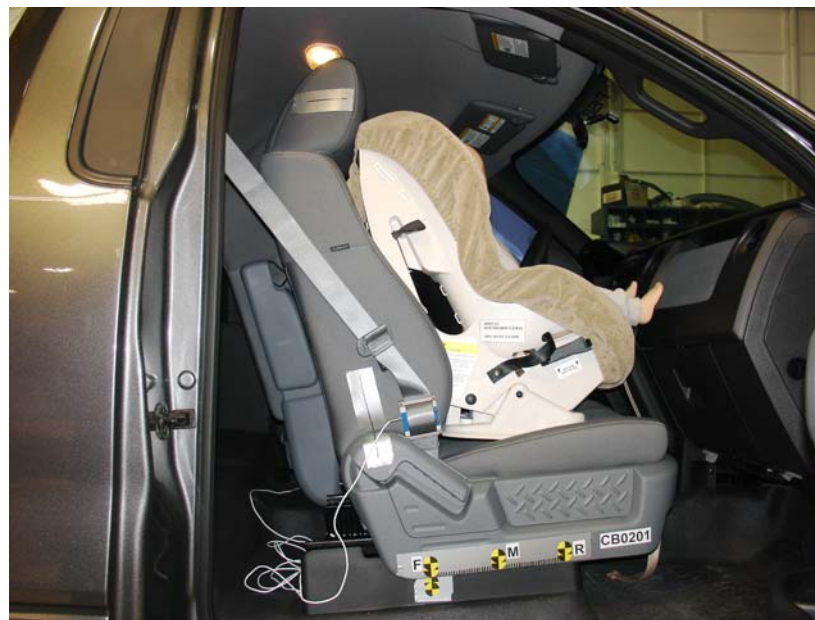
Britax Roundabout Forward Facing Unbelted, Forward Seat Track
