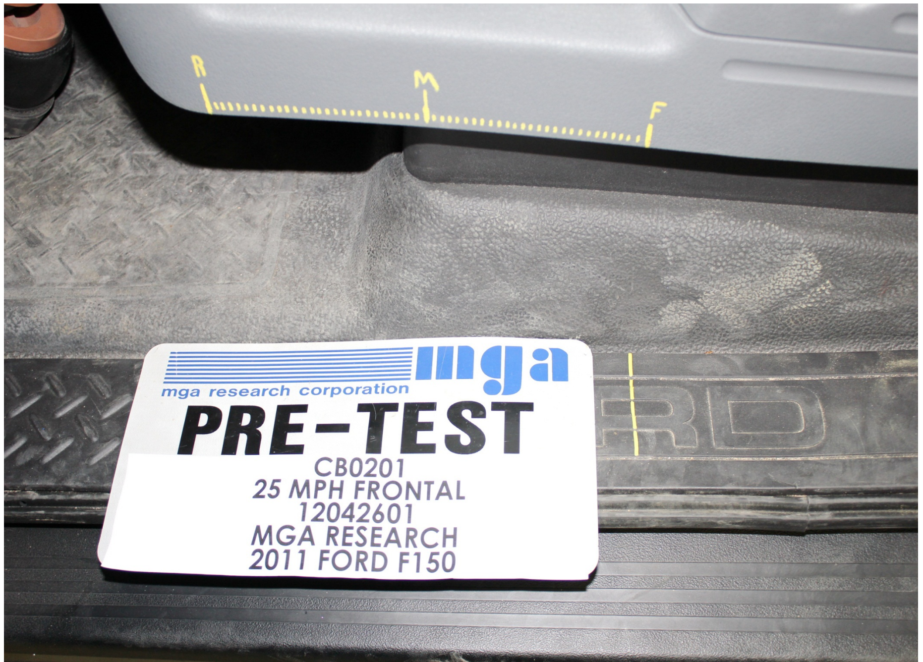
Pre-Test Driver Dummy Seat Position
