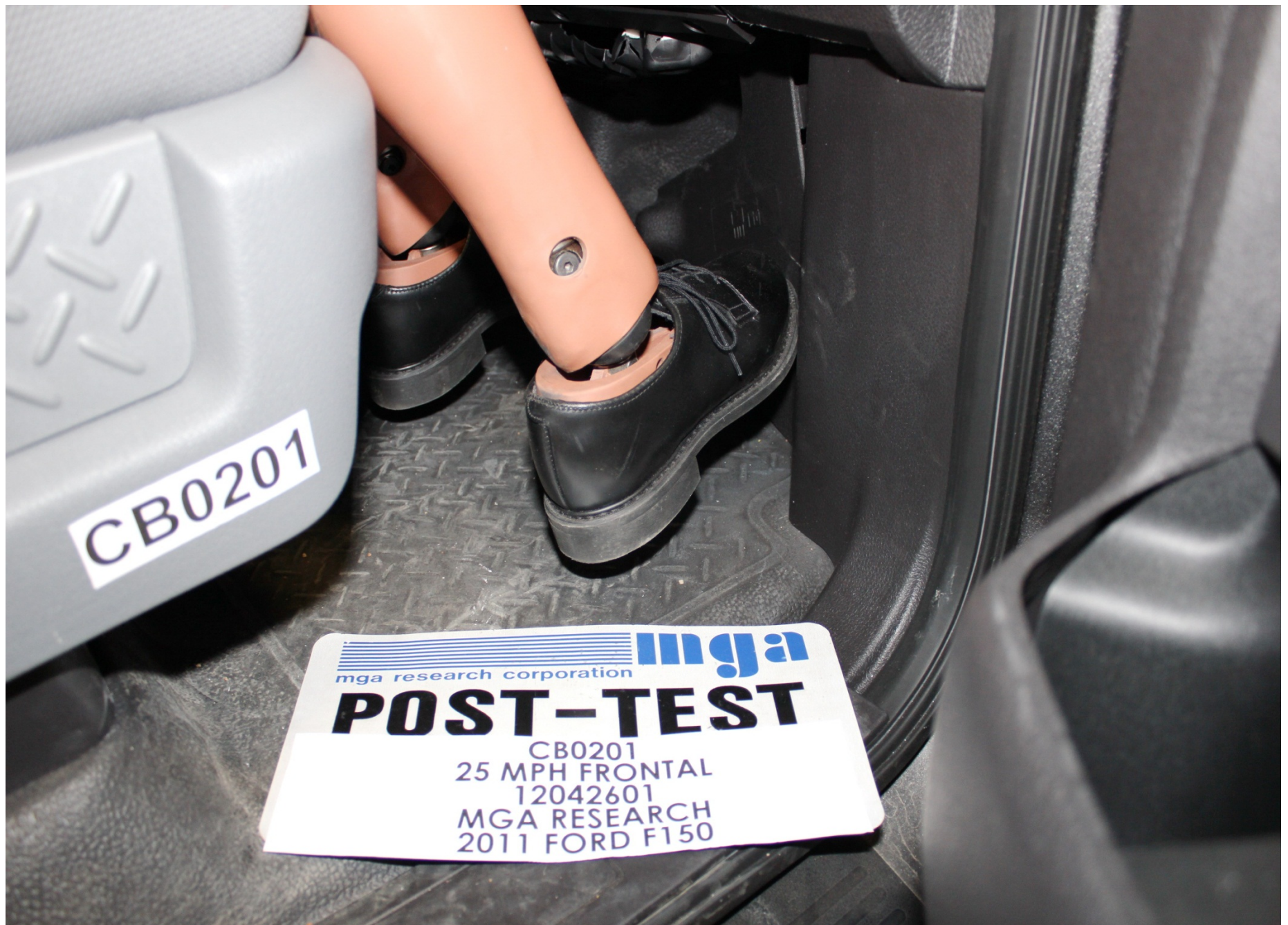
Post-Test Passenger Dummy Feet Position
