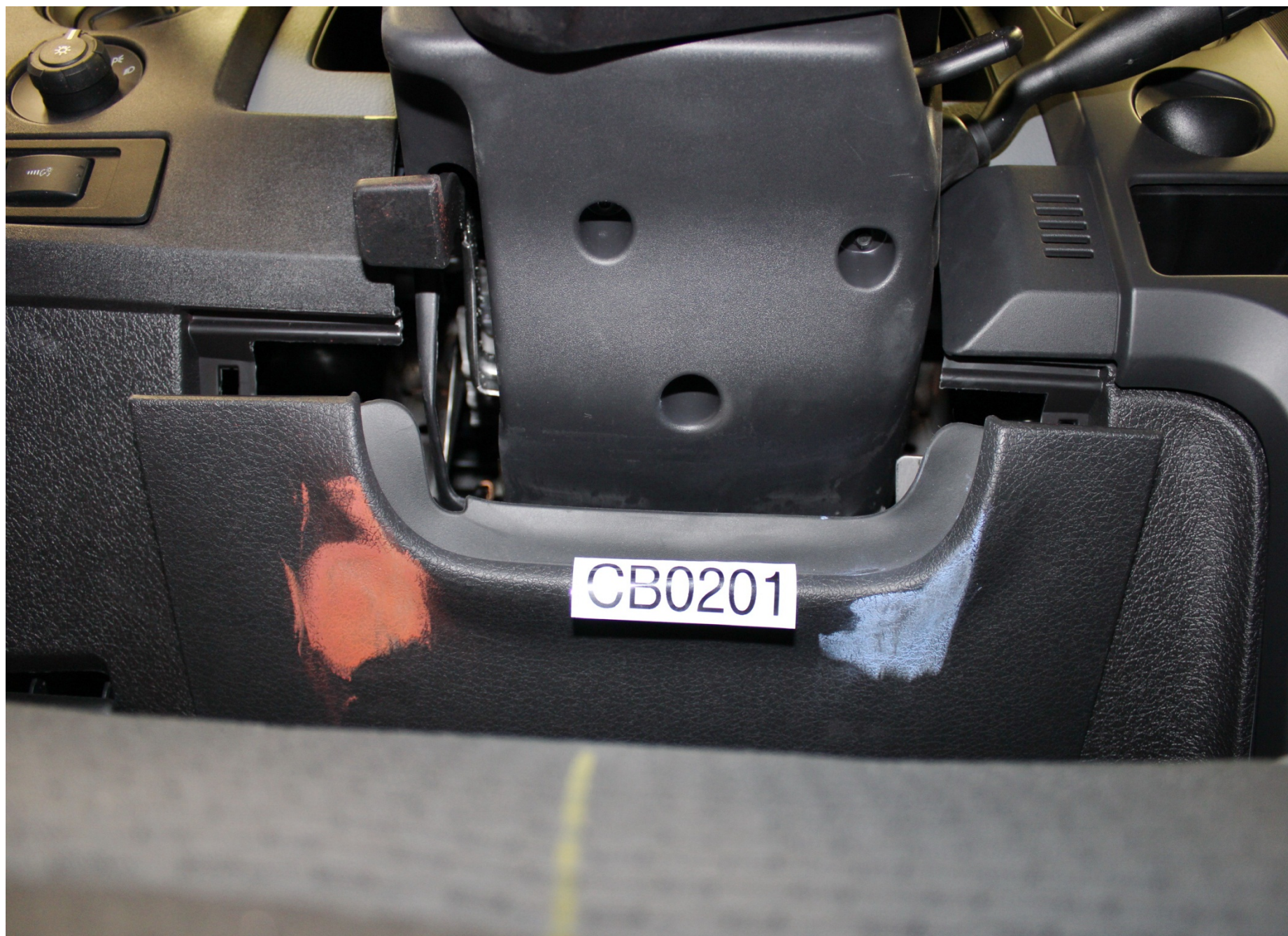
Post-Test Driver Dummy Knee Contact
