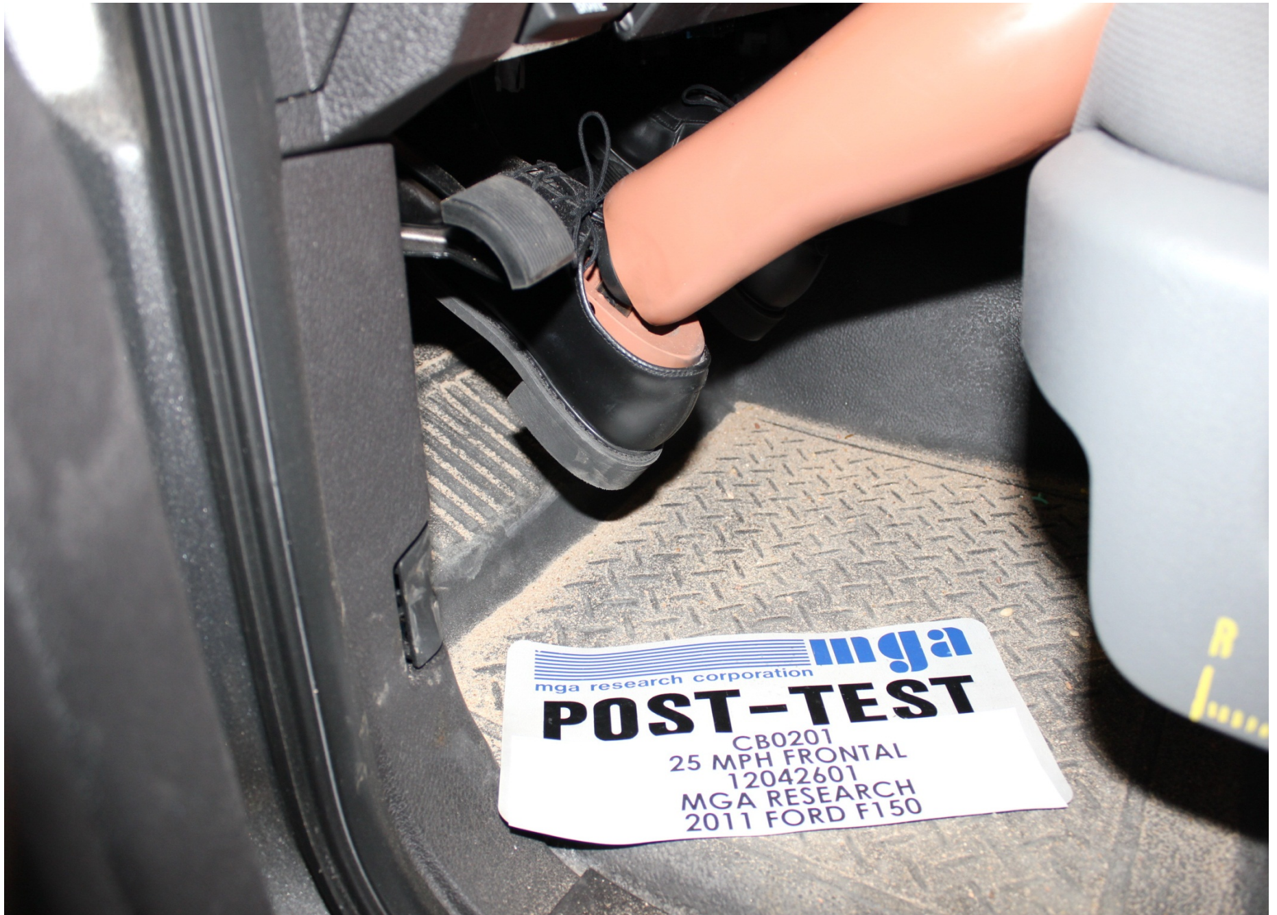
Post-Test Driver Dummy Feet Position
