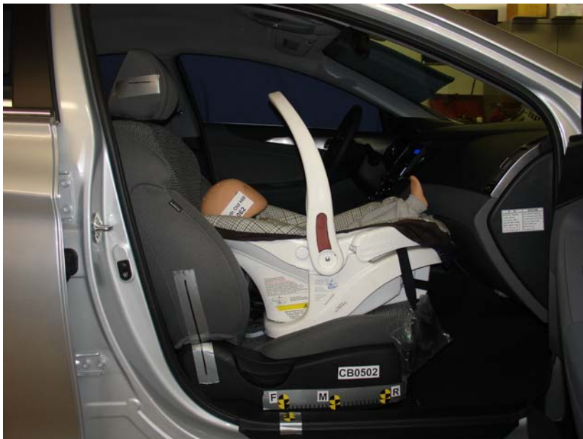
Cosco Arriva WBase, Unbelted, Forward Facing, Forward Seat Track
