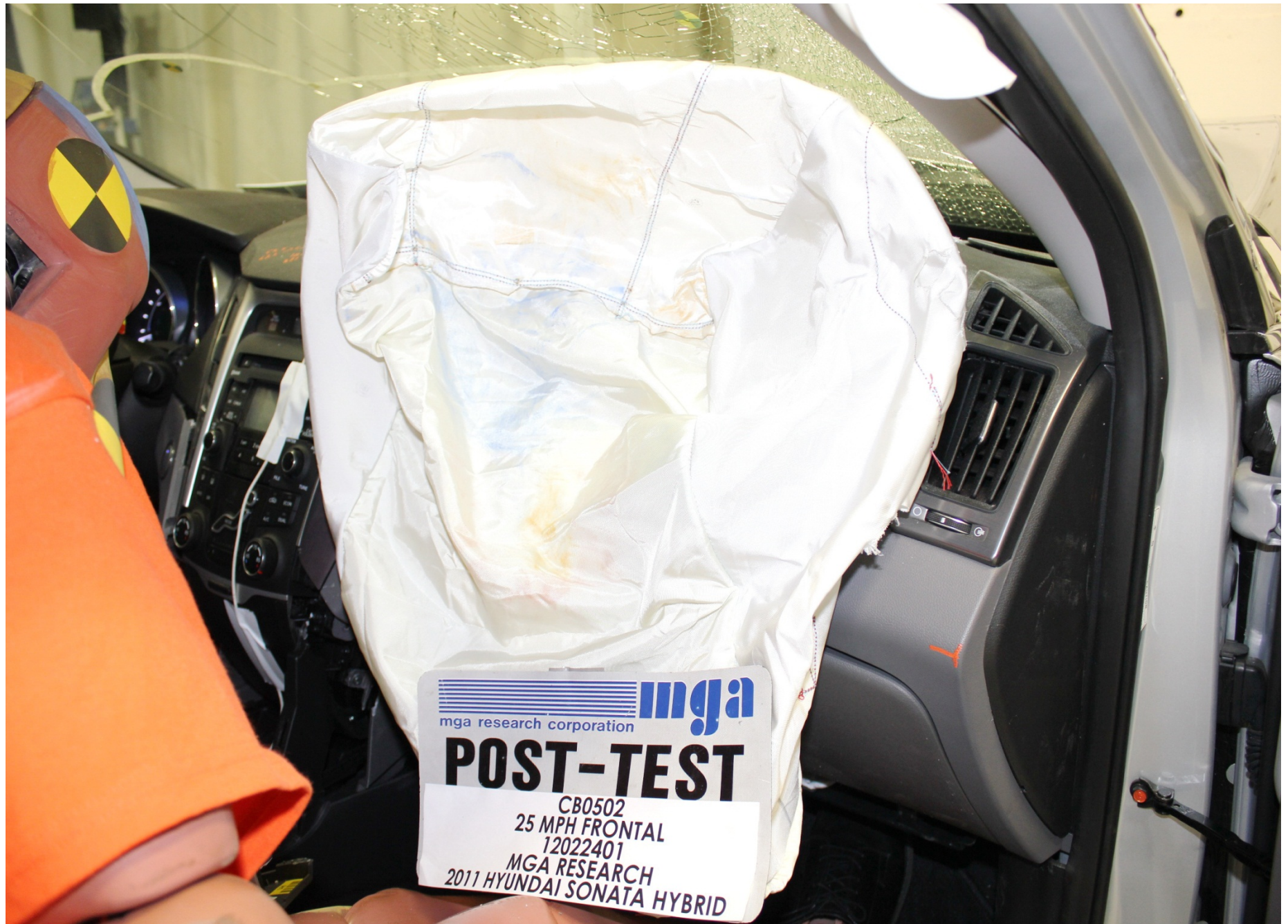
Post-Test Passenger Dummy Airbag Contact
