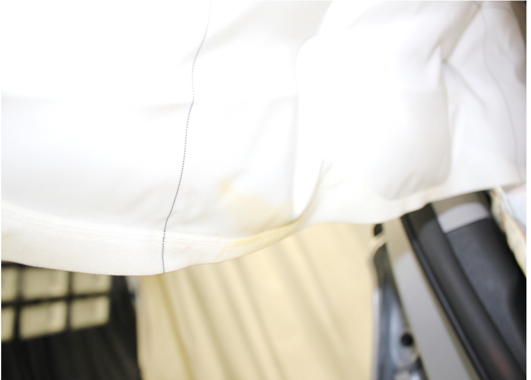
Post-Test Passenger Dummy Head Contact (side airbag)
