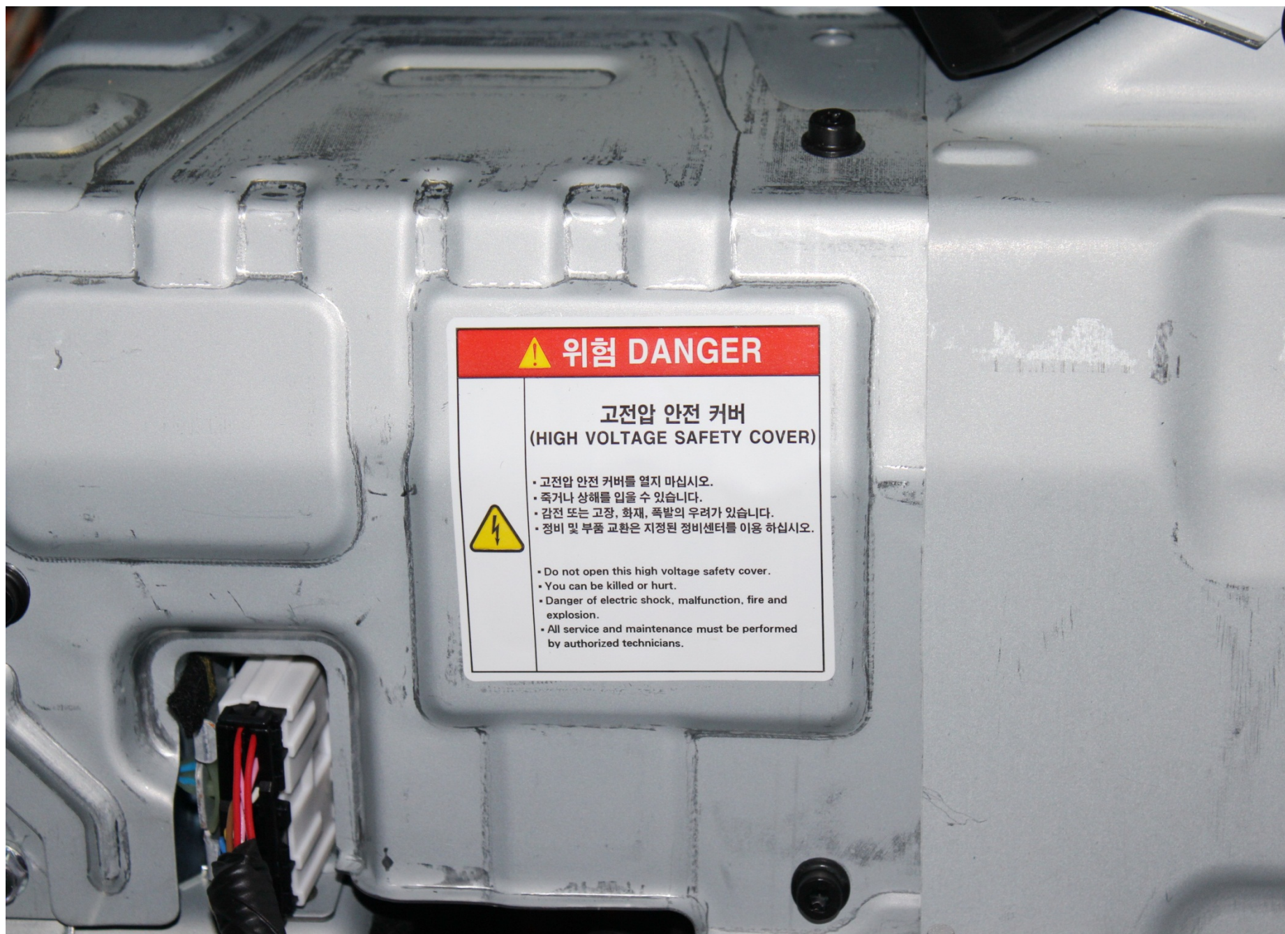
High Voltage Warning Label
