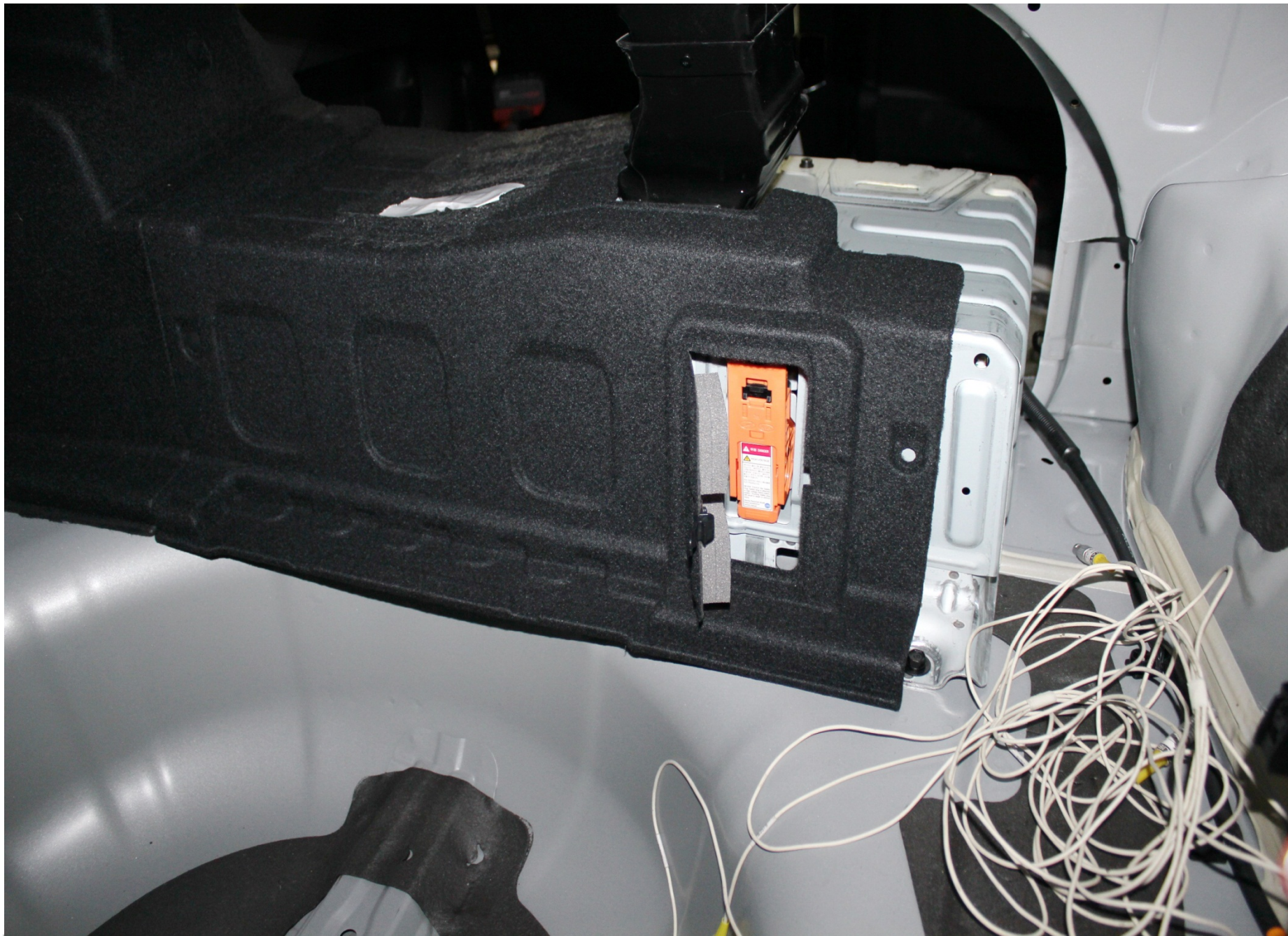
Manual High Voltage Service Disconnect Plug
