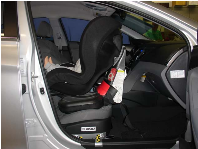
Graco Safeseat Rear Facing Unbelted, Rearward Seat Track
