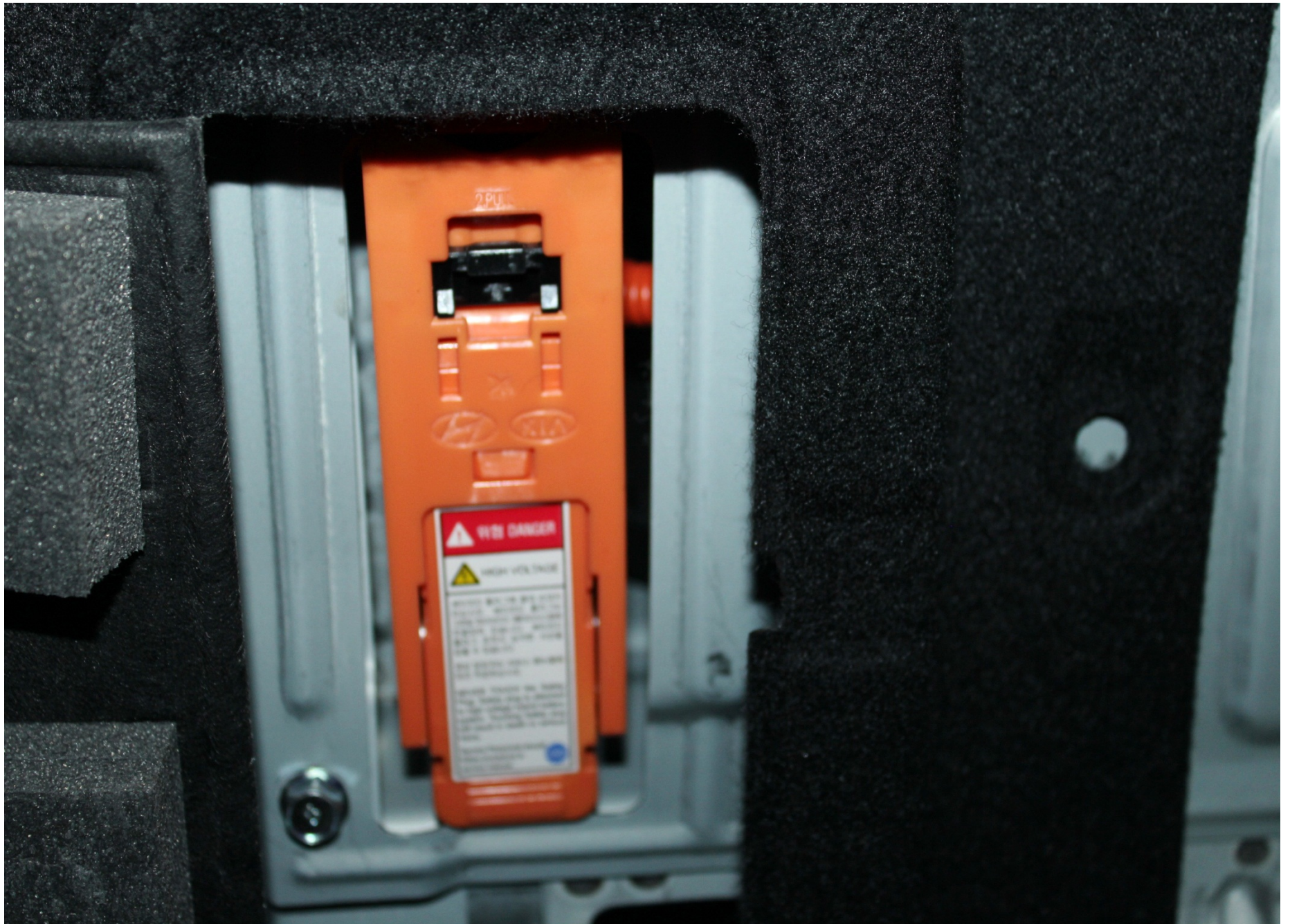
Manual High Voltage Service Disconnect Plug Close Up View
