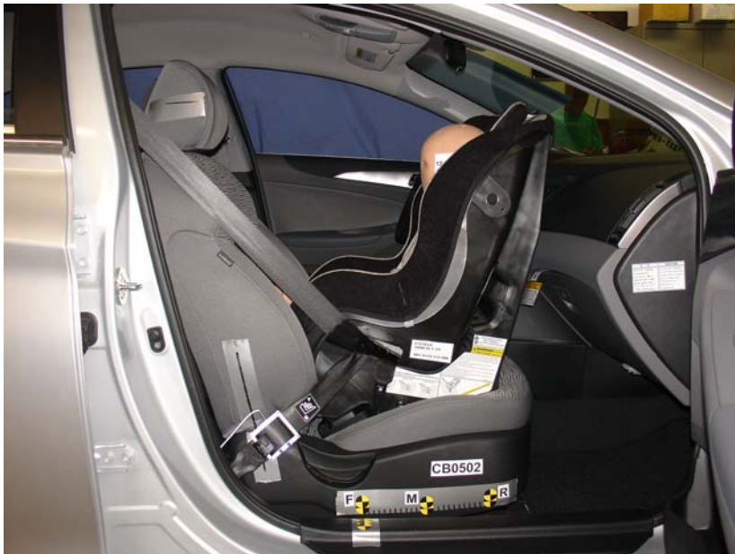
Evenflo Tribute Rear Facing Belted, Forward Seat Track
