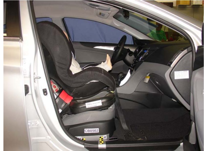
Graco Safeseat Forward Facing Unbelted, Rearward Seat Track
