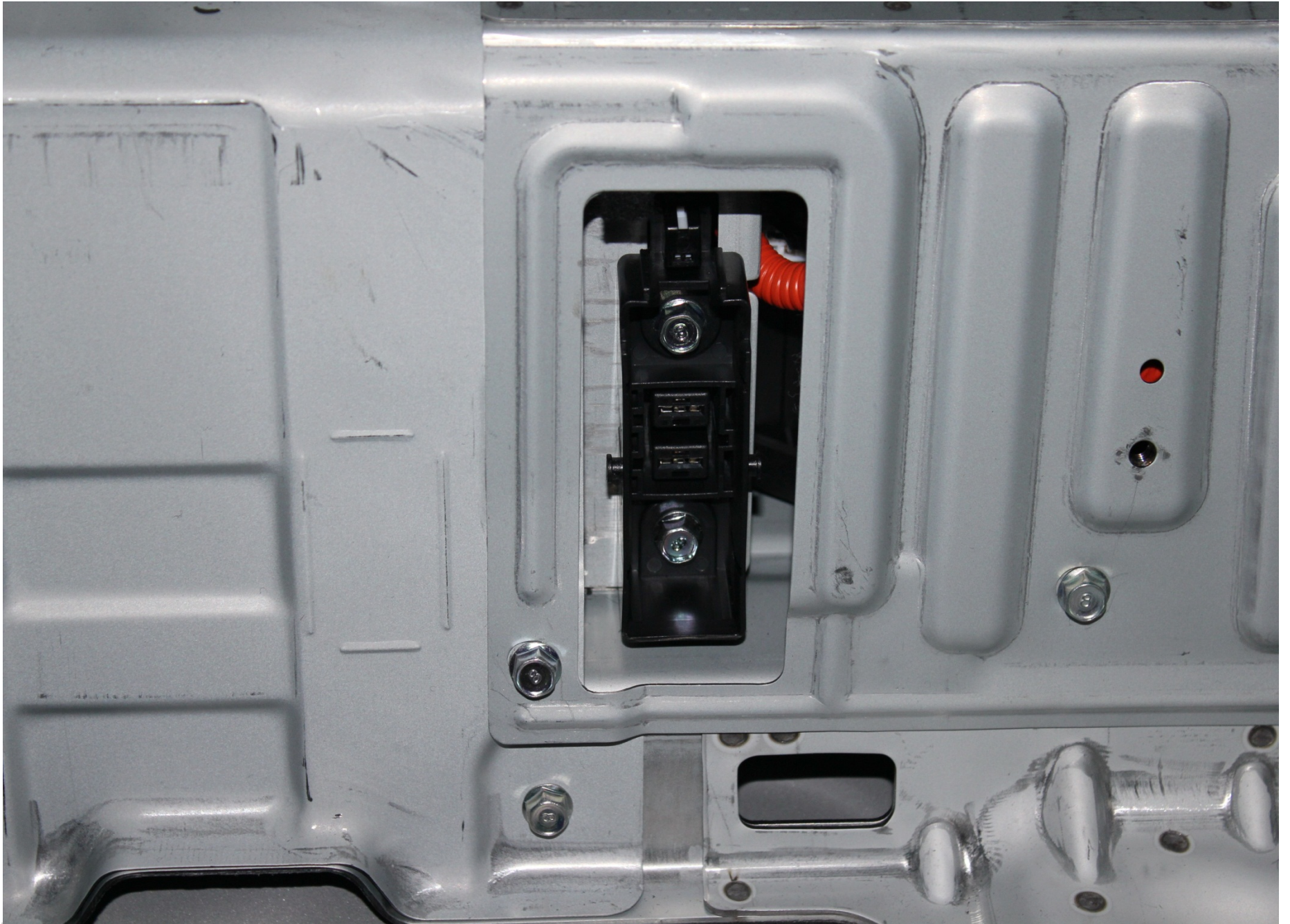
Manual High Voltage Service Disconnect Plug Removed
