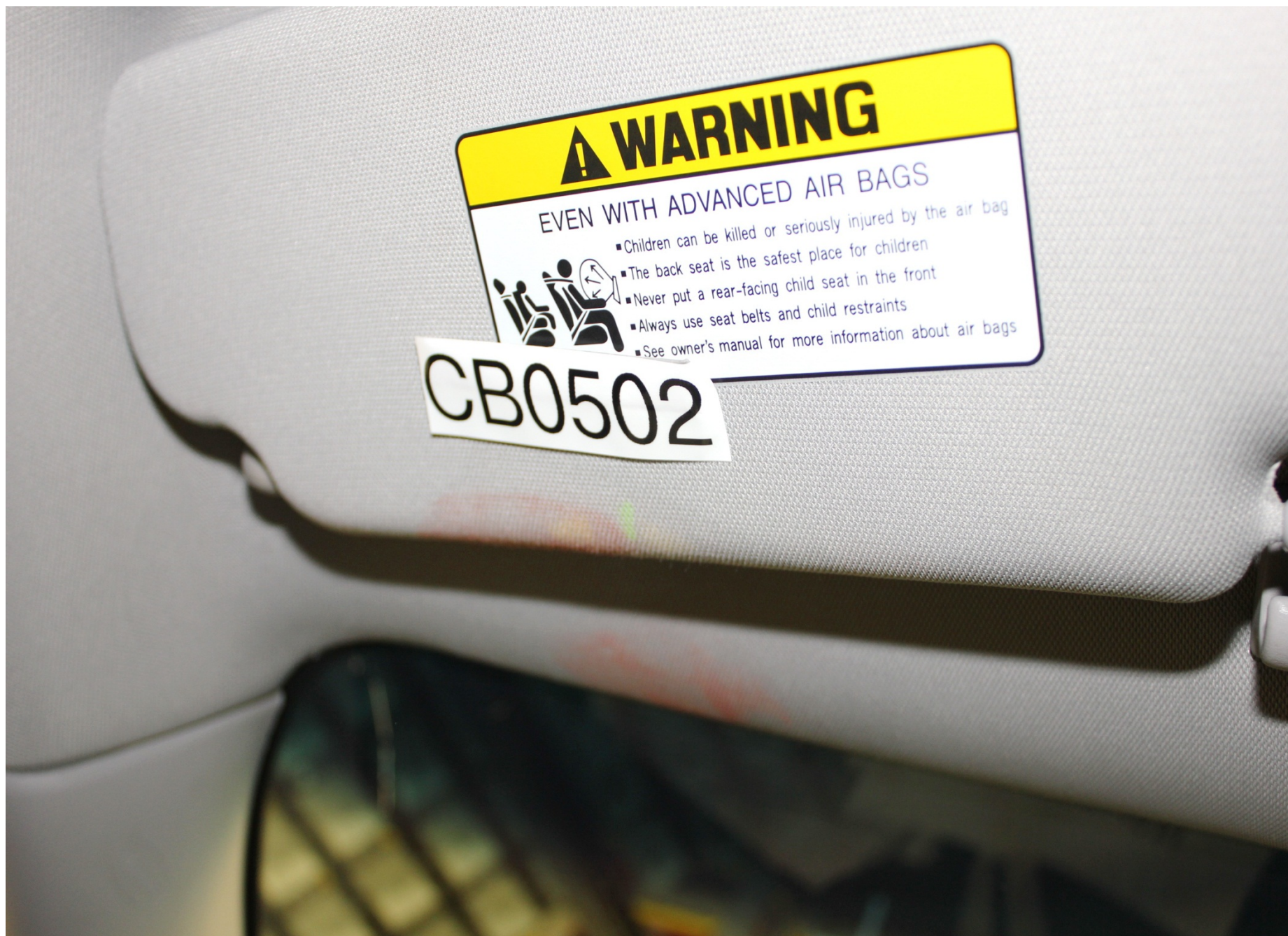
Post-Test Driver Dummy Head Contact (visor)
