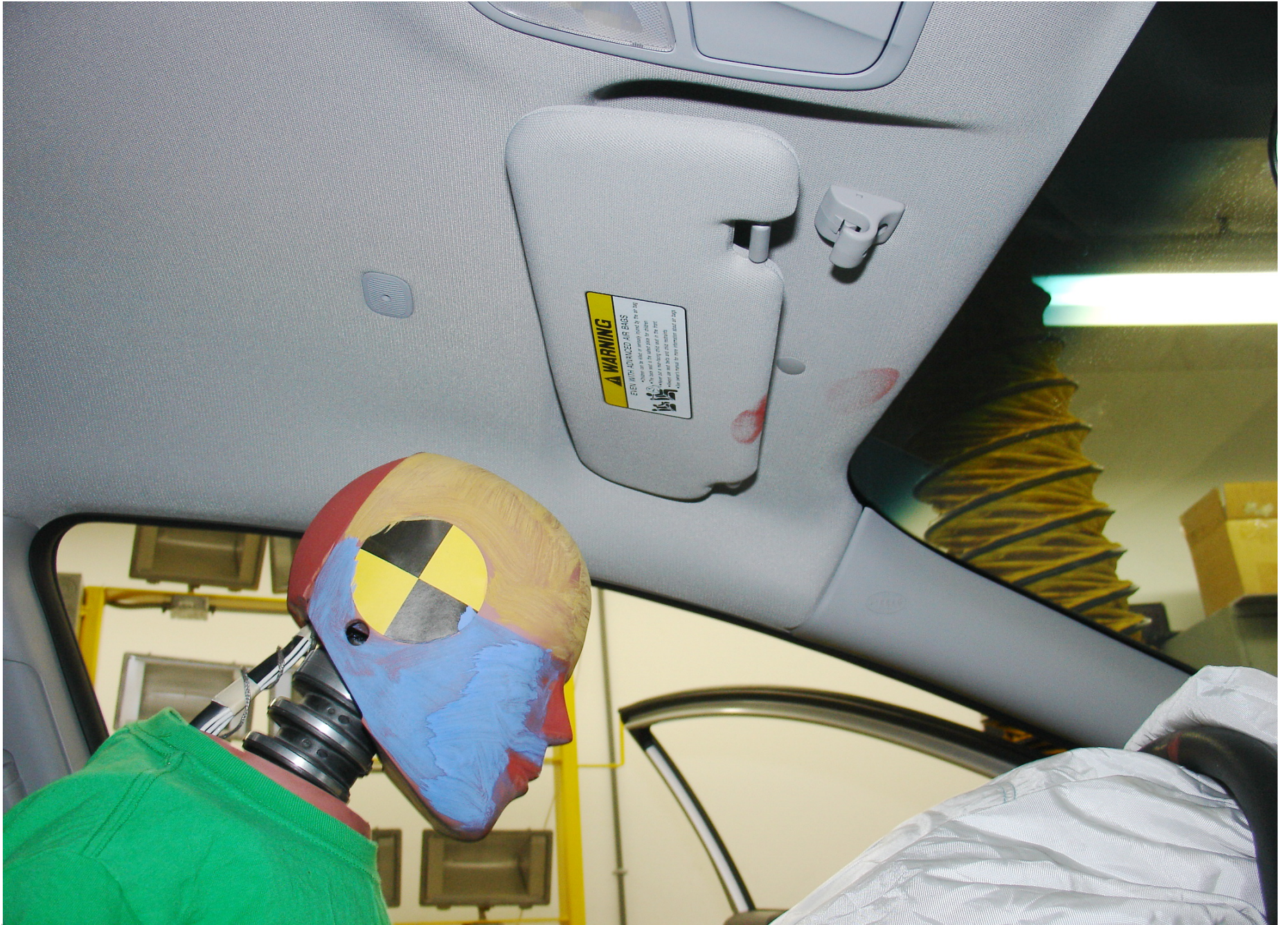
Post-Test 5th Fem. P2 Driver Dummy Head Contact (visor)
