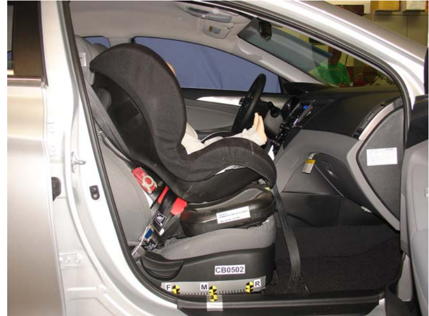
Graco Safeseat Forward Facing Belted, Middle Seat Track
