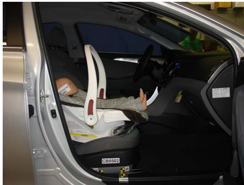
Cosco Arriva WOut Base, Unbelted, Forward Facing, Rearward Seat Track
