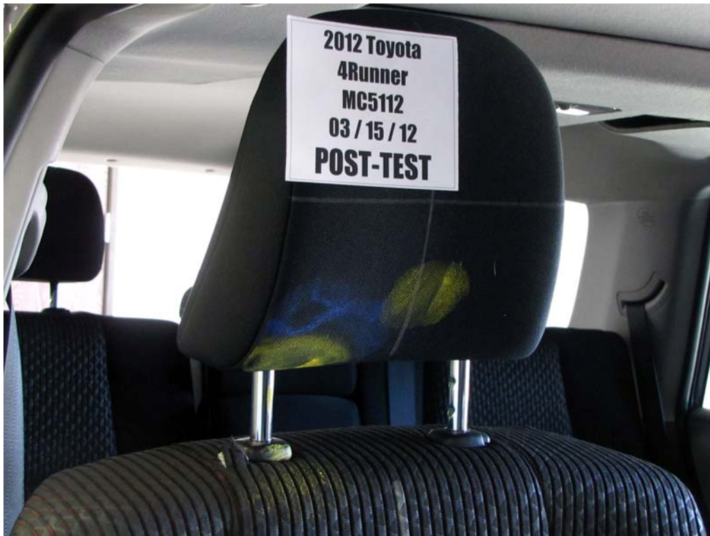
FIGURE 62a. Post-Test Passenger Dummy Contact With Headrest
