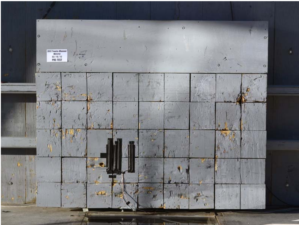
FIGURE 2. Load Cell Wall
