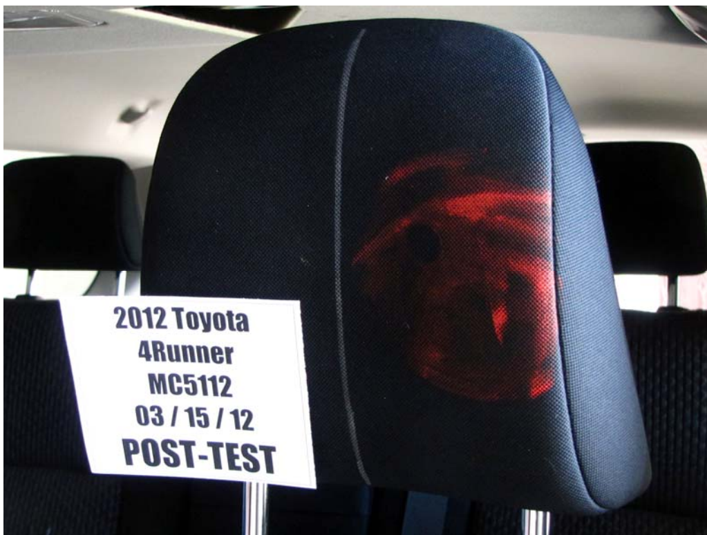
FIGURE 45. Post-Test Driver Dummy Contact With Headrest
