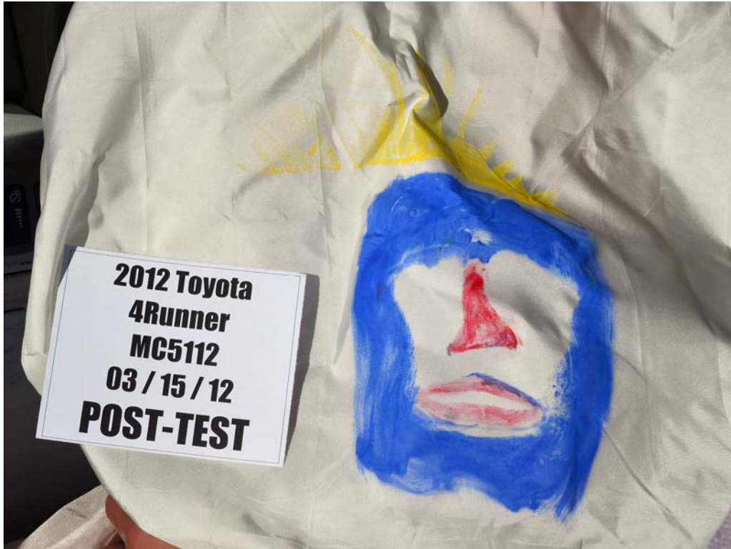
FIGURE 44. Post-Test Driver Dummy Contact With Airbag
