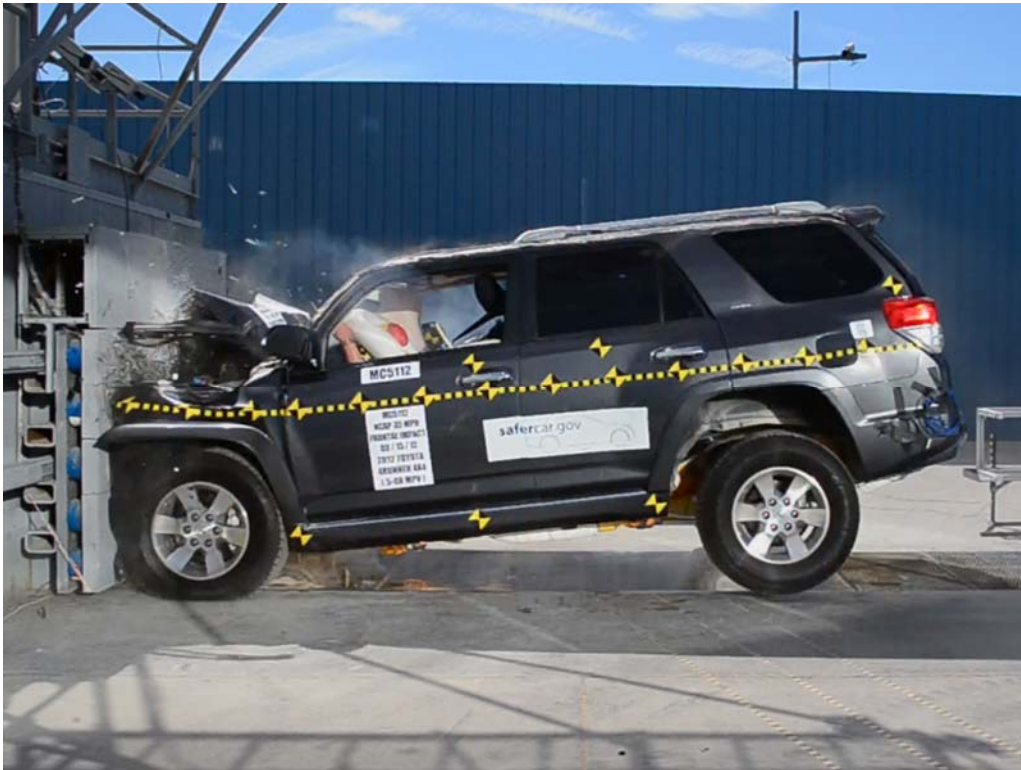
FIGURE 71. Toyota 4Runner Frontal Impact Event
