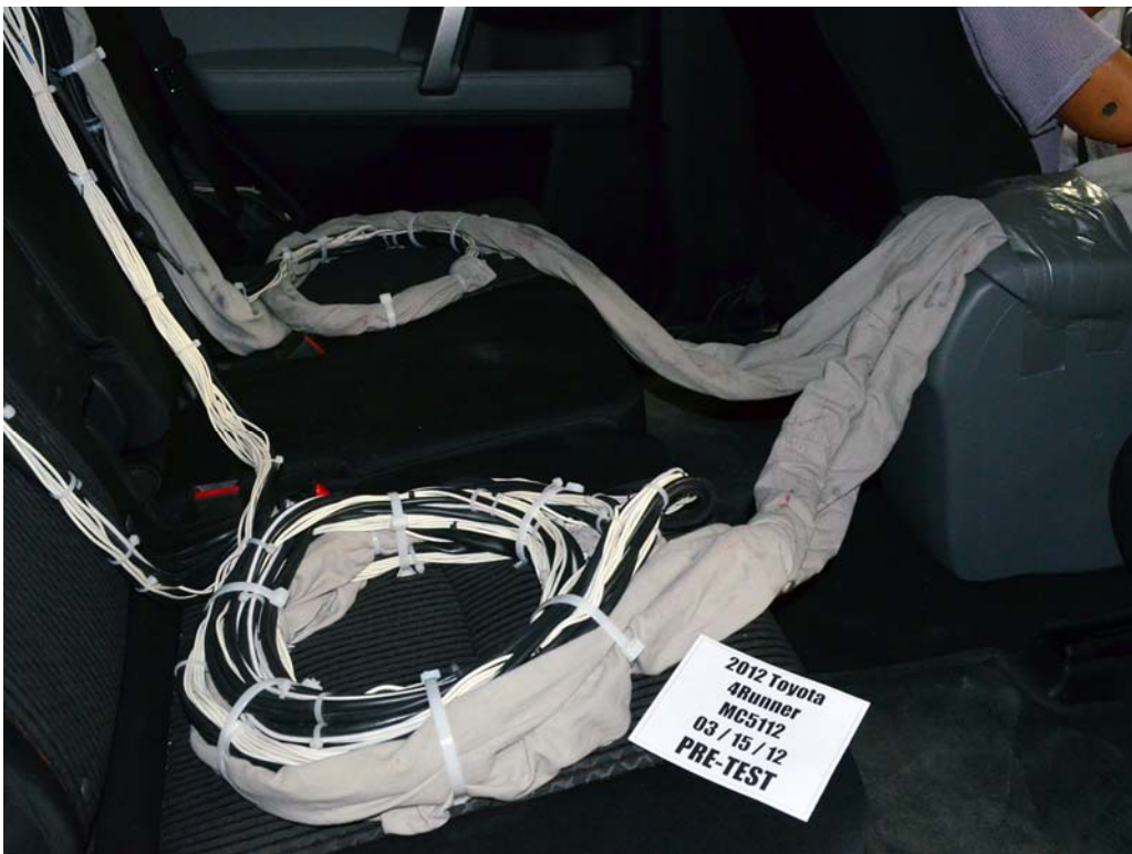
FIGURE 27. Pre-Test Dummy Cable Routing
