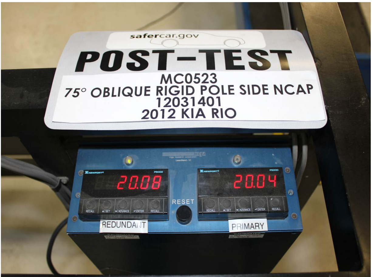
Post-Test Primary and Redundant Speed Trap Read-Out
