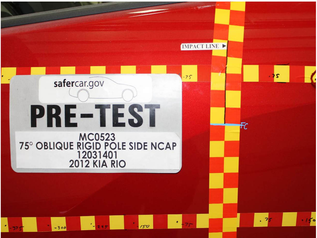
Pre-Test Close-Up View of Impact Point Target
