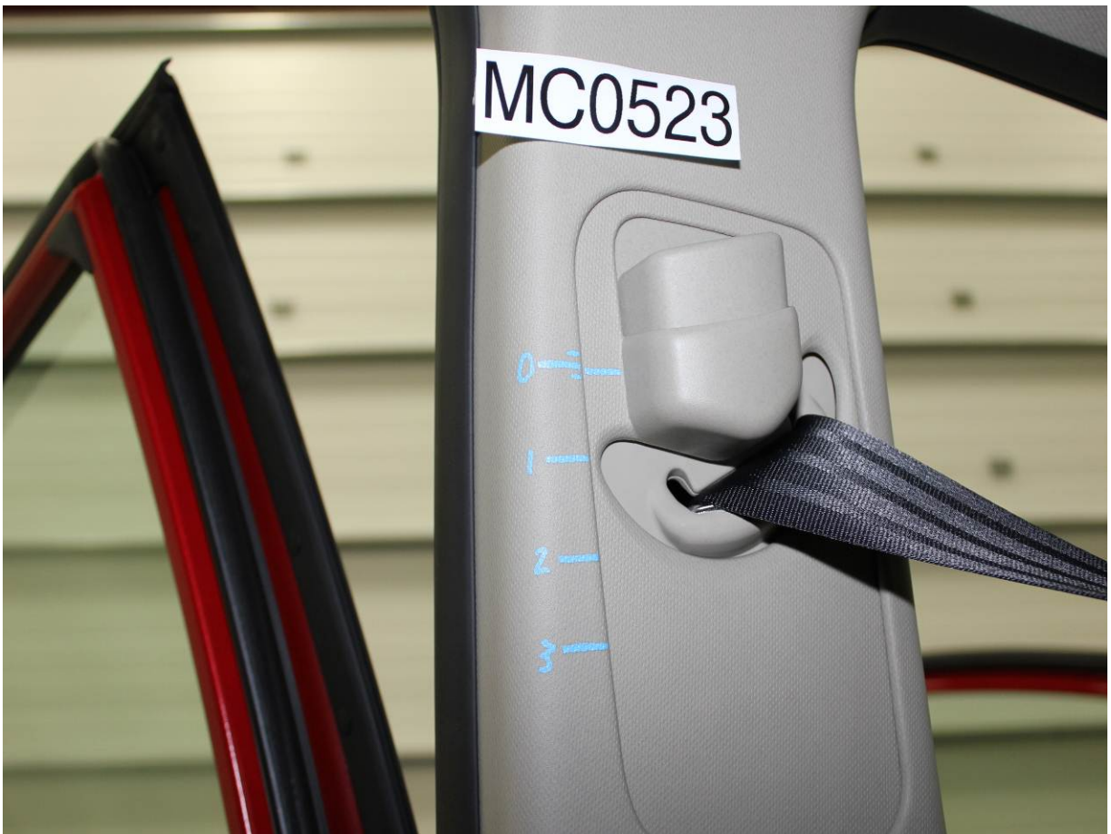
Pre-Test View of Belt Anchorage for Dummy
