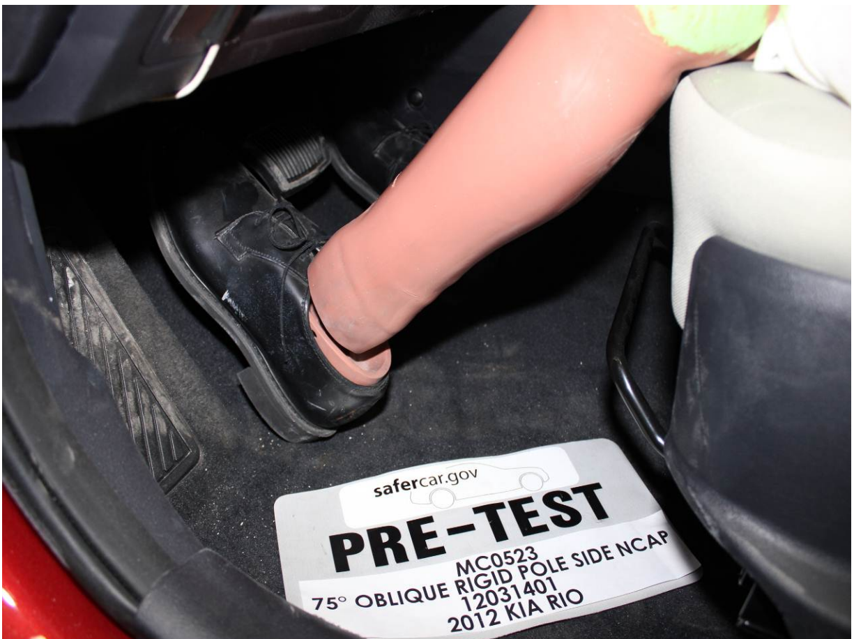
Pre-Test Placement of Dummy's Feet
