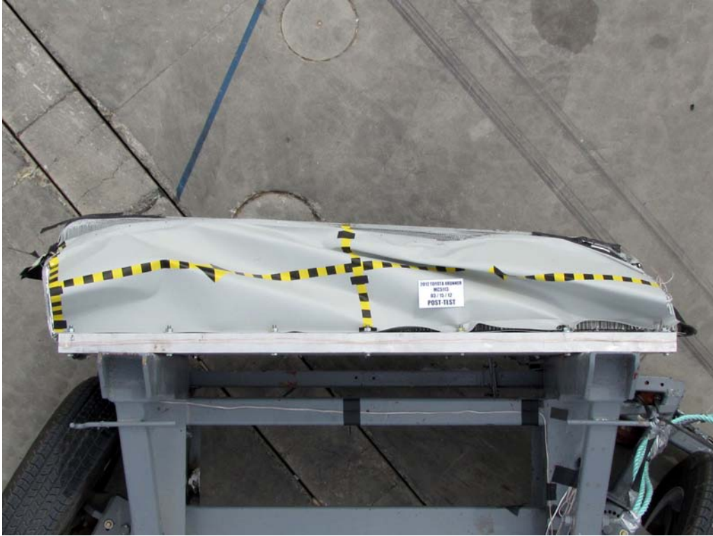
FIGURE 85. Post-Test Top View of MDB Impactor Face
