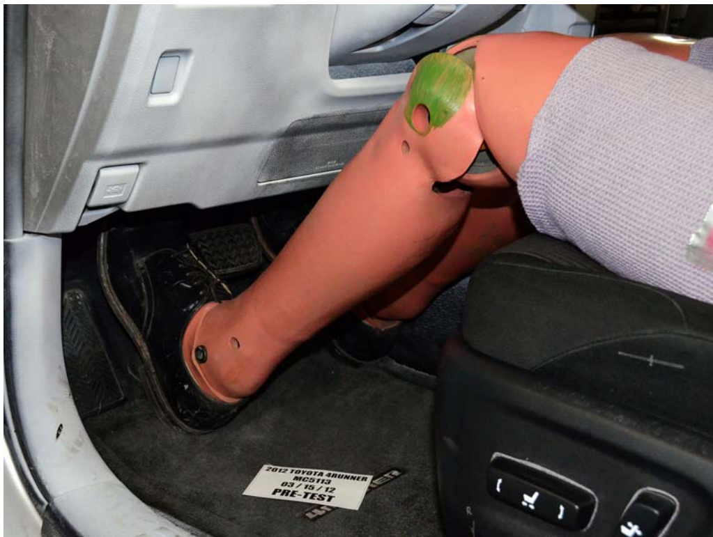
FIGURE 34. Pre-Test Placement of Driver Dummy's Feet
