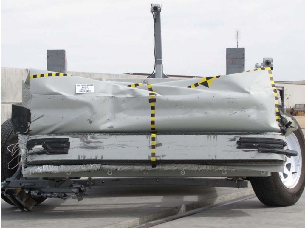
FIGURE 83. Post-Test Front View of MDB Impactor Face
