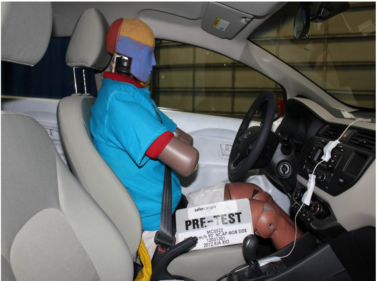
Pre-Test Right Side View of Driver Dummy and Front Seat of Occupant Compartment
