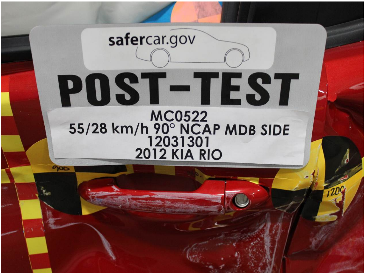
Post-Test Left Front Door Latch Close-Up
