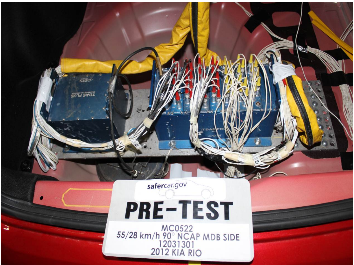
Pre-Test Ballast View
