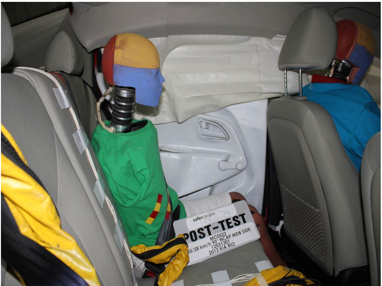
Post-Test Right Side View of Rear Passenger Dummy and Rear Seat Occupant Compartment
