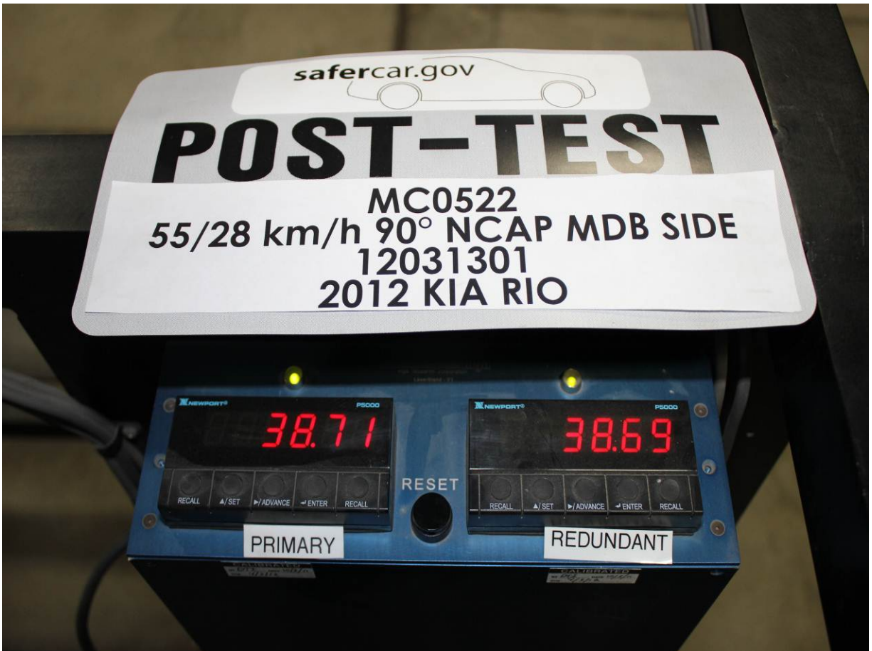
Post-Test Primary and Redundant Speed Trap Read-Out
