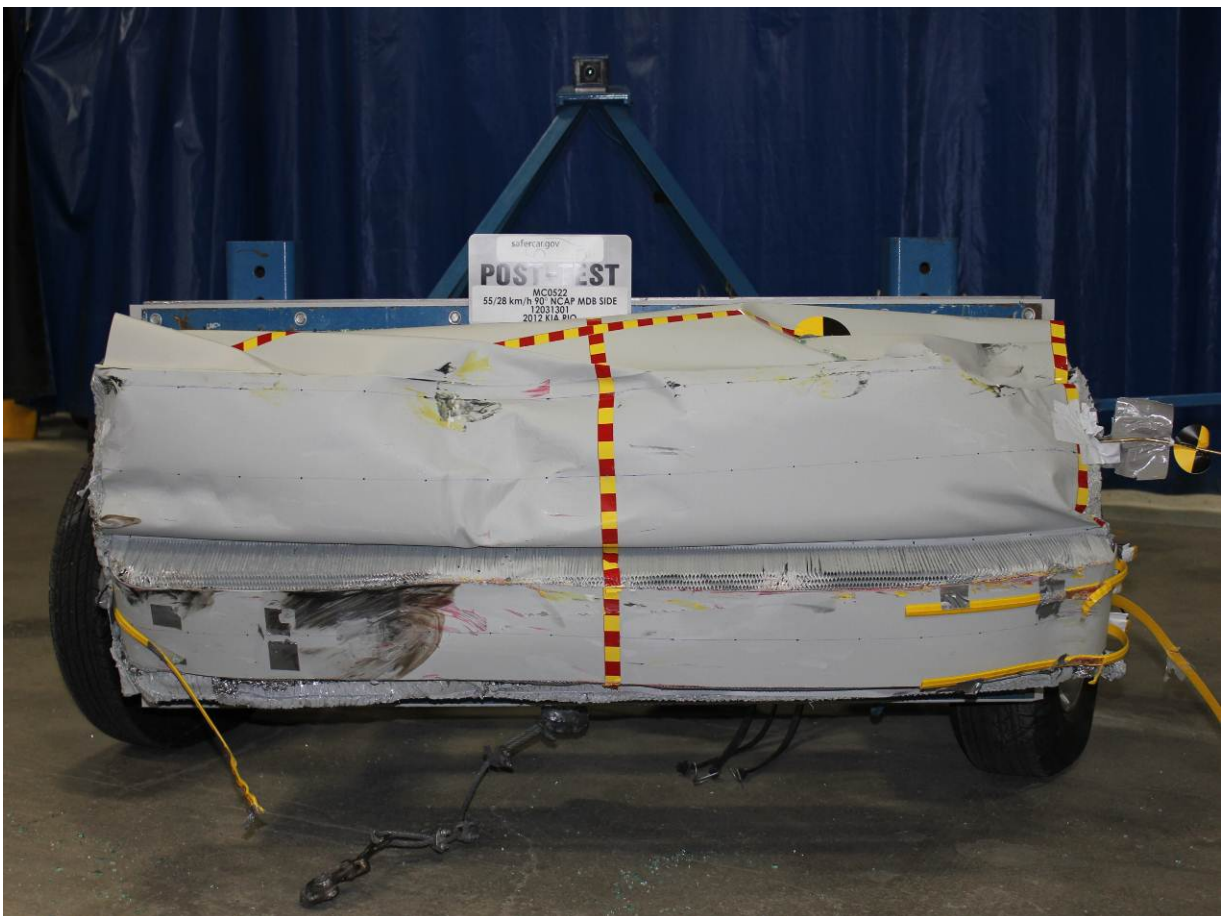
Post-Test Front View of MDB Impactor Face
