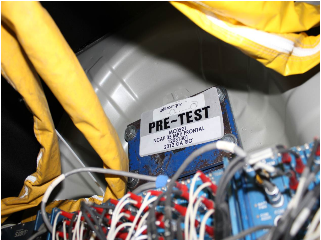
Ballast Installed in Vehicle
