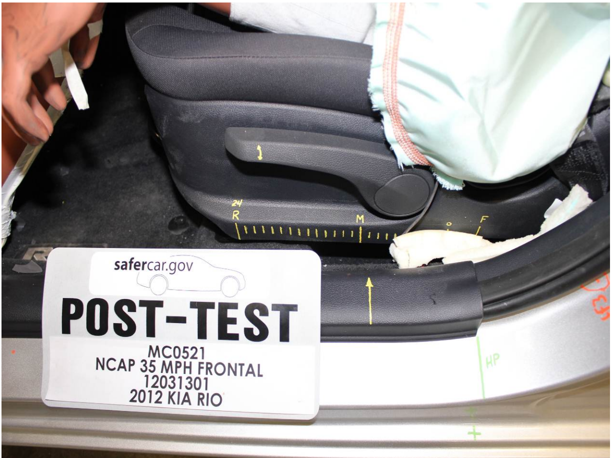
Post-Test Driver's Seat Fore-Aft Markings
