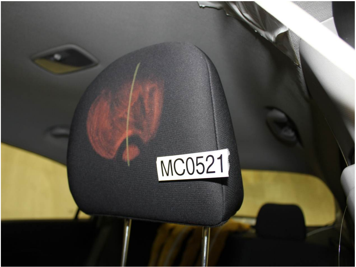
Post-Test Driver Dummy Contact with Headrest
