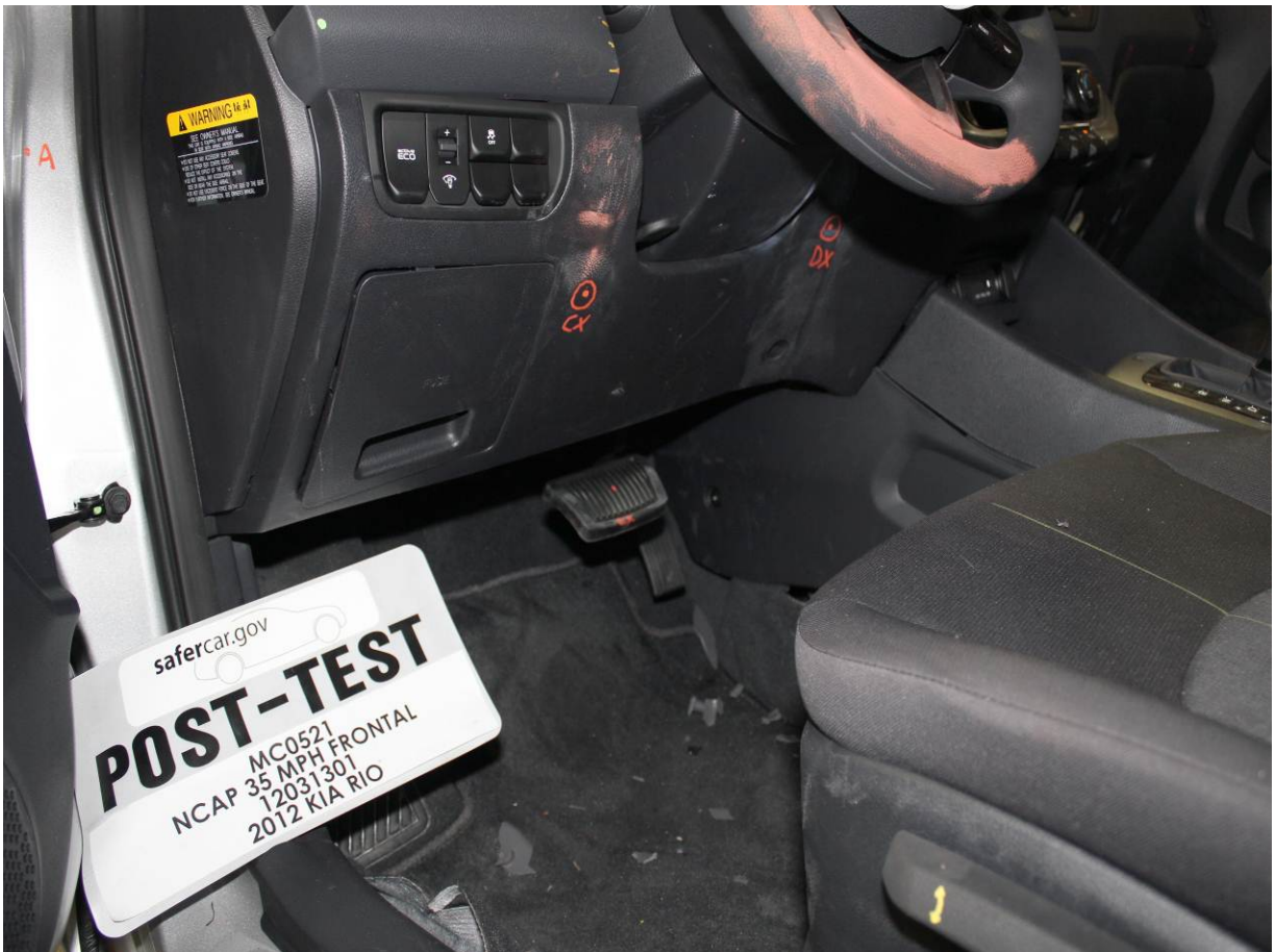
Post-Test Driver's Side Knee Bolster (without dummy)
