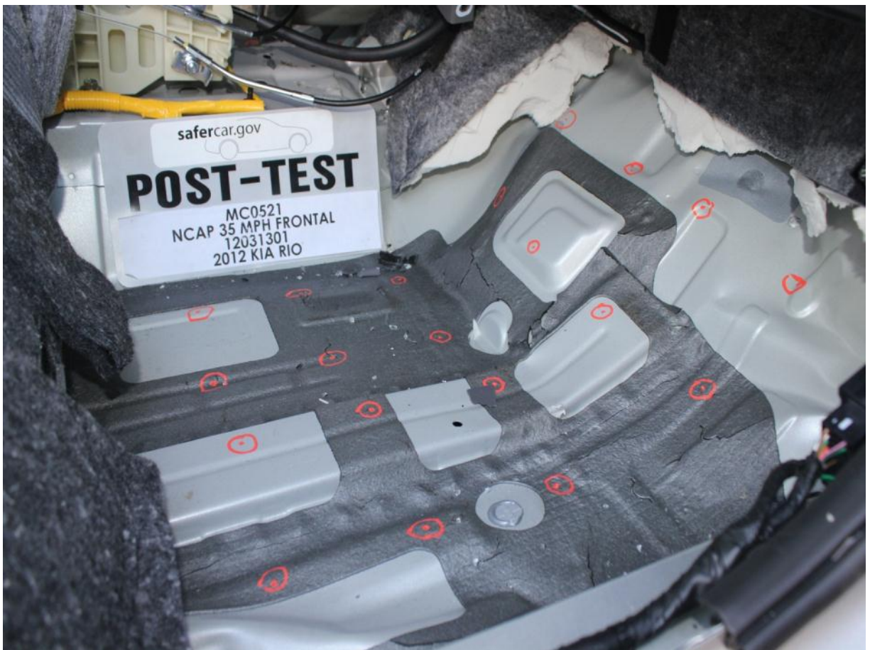
Post-Test Passenger's Side Floorpan
