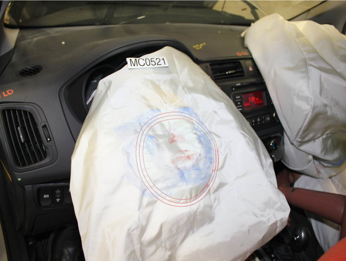
Post-Test Driver Dummy Contact with Airbag
