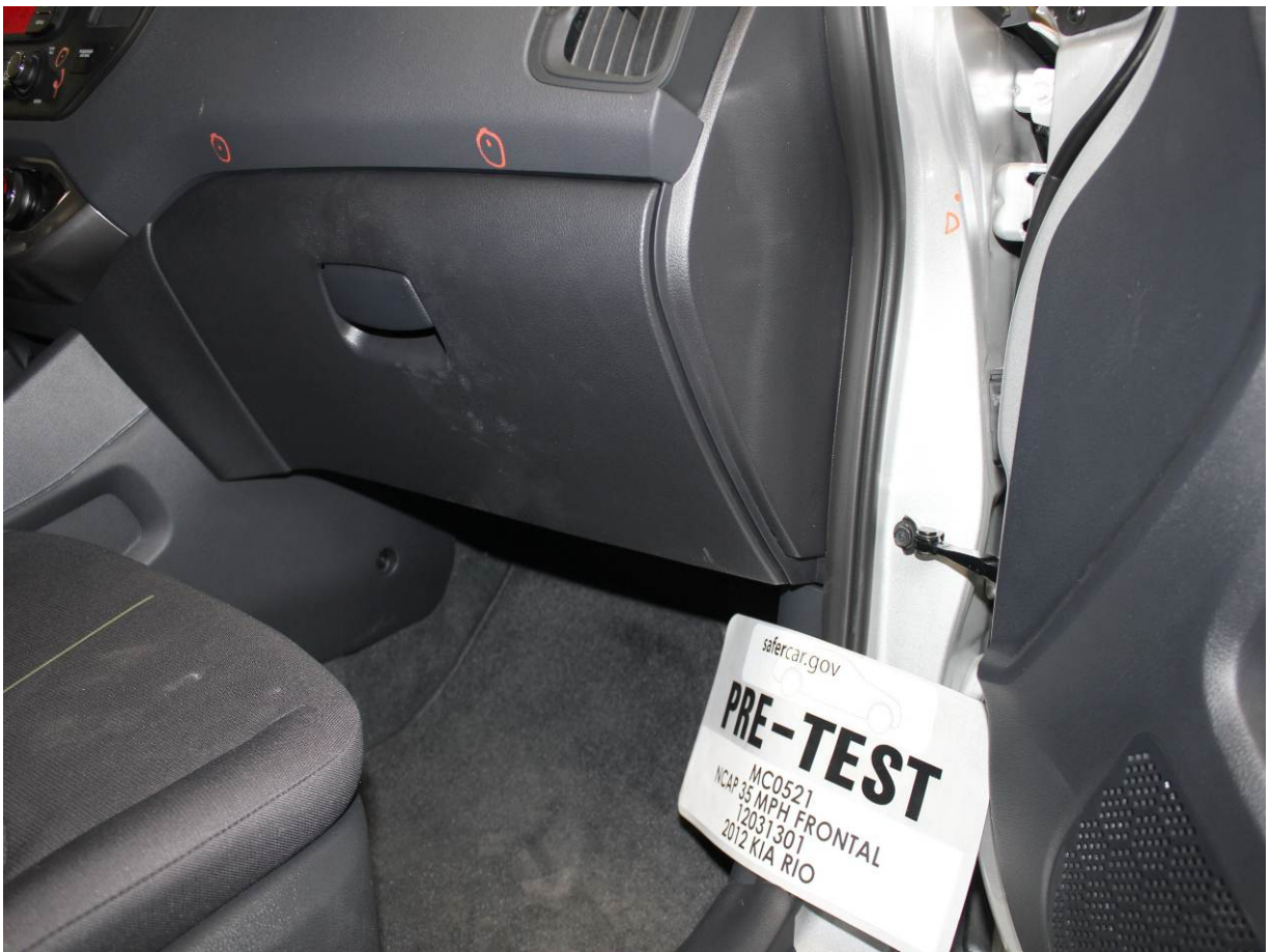
Pre-Test Passenger's Side Knee Bolster (without dummy)
