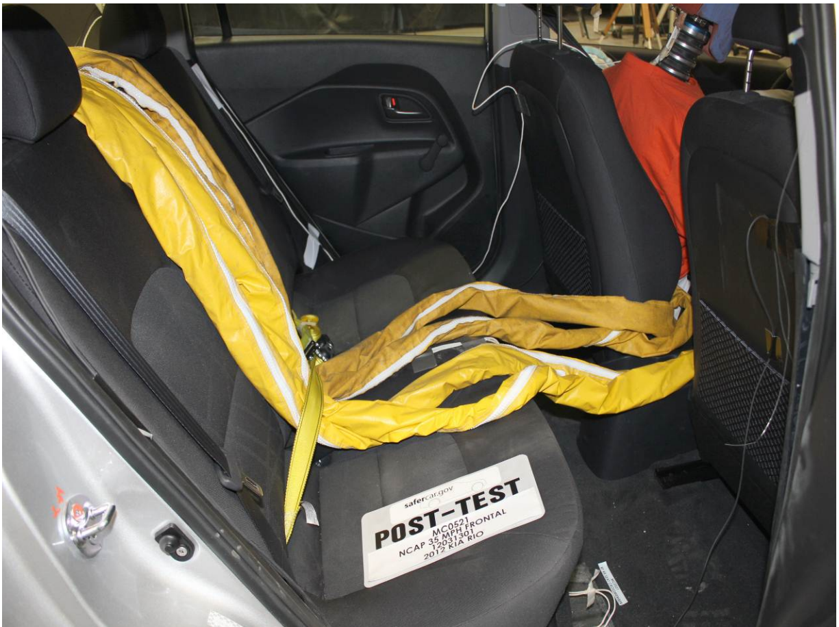
Post-Test Dummy Cable Routing
