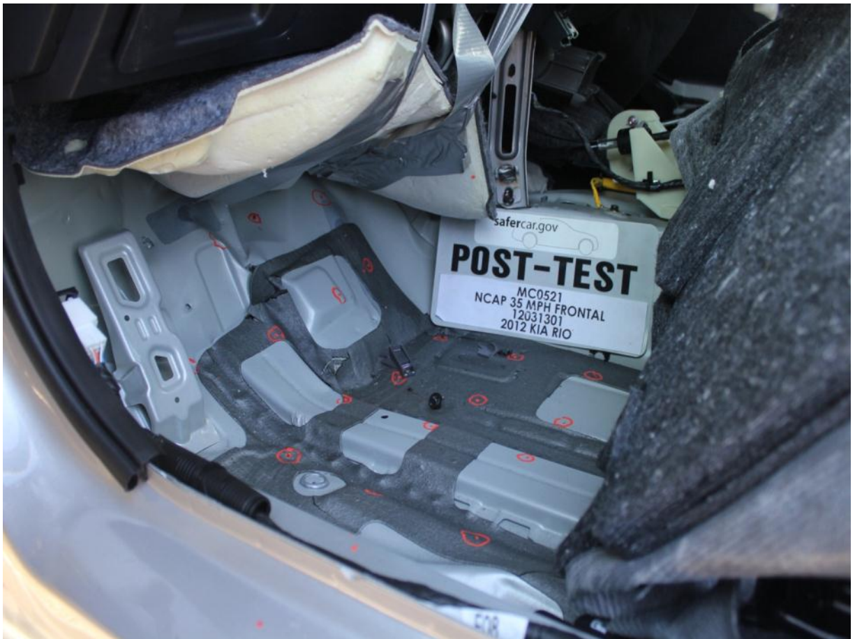
Post-Test Driver's Side Floorpan
