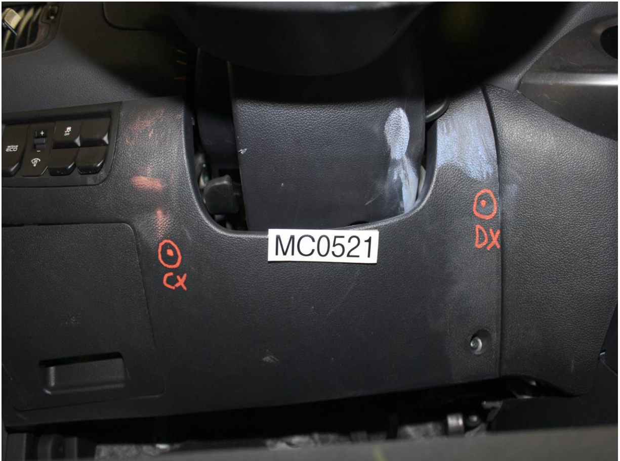
Post-Test Driver Dummy Contact with Knee Bolster
