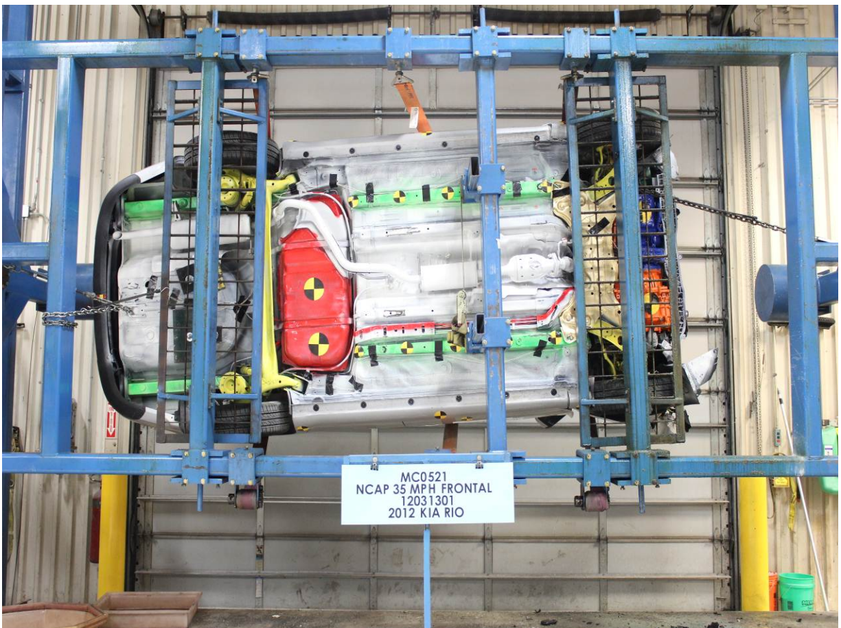
Vehicle at 90 Degrees on Static Rollover Device
