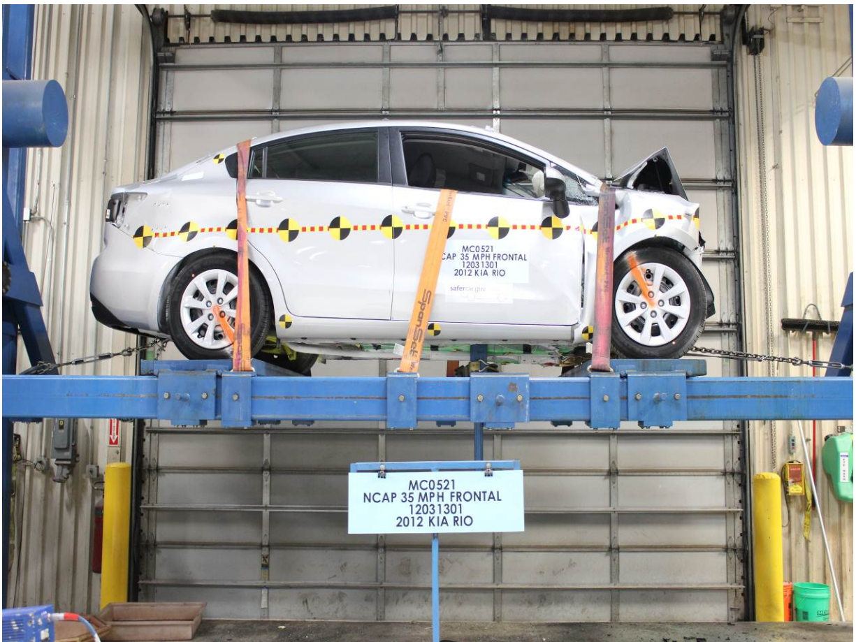
Vehicle at 0 Degrees on Static Rollover Device
