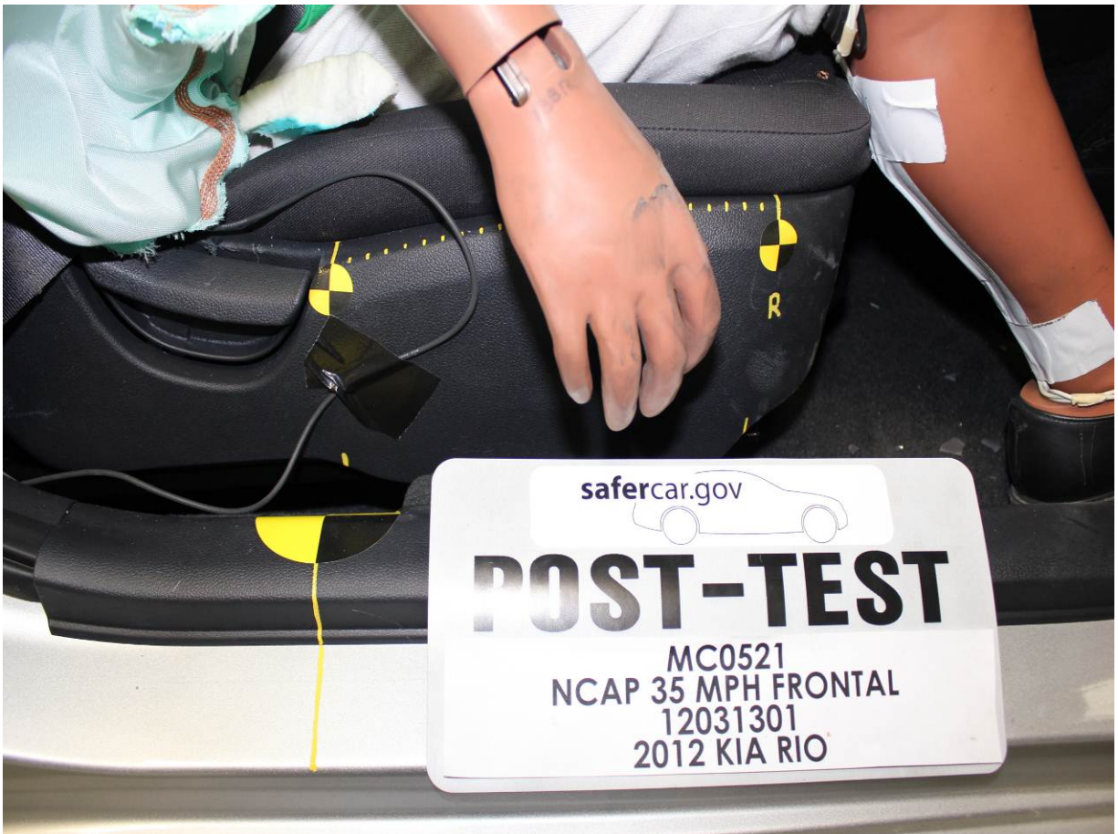
Post-Test Passenger's Seat Fore-Aft Markings
