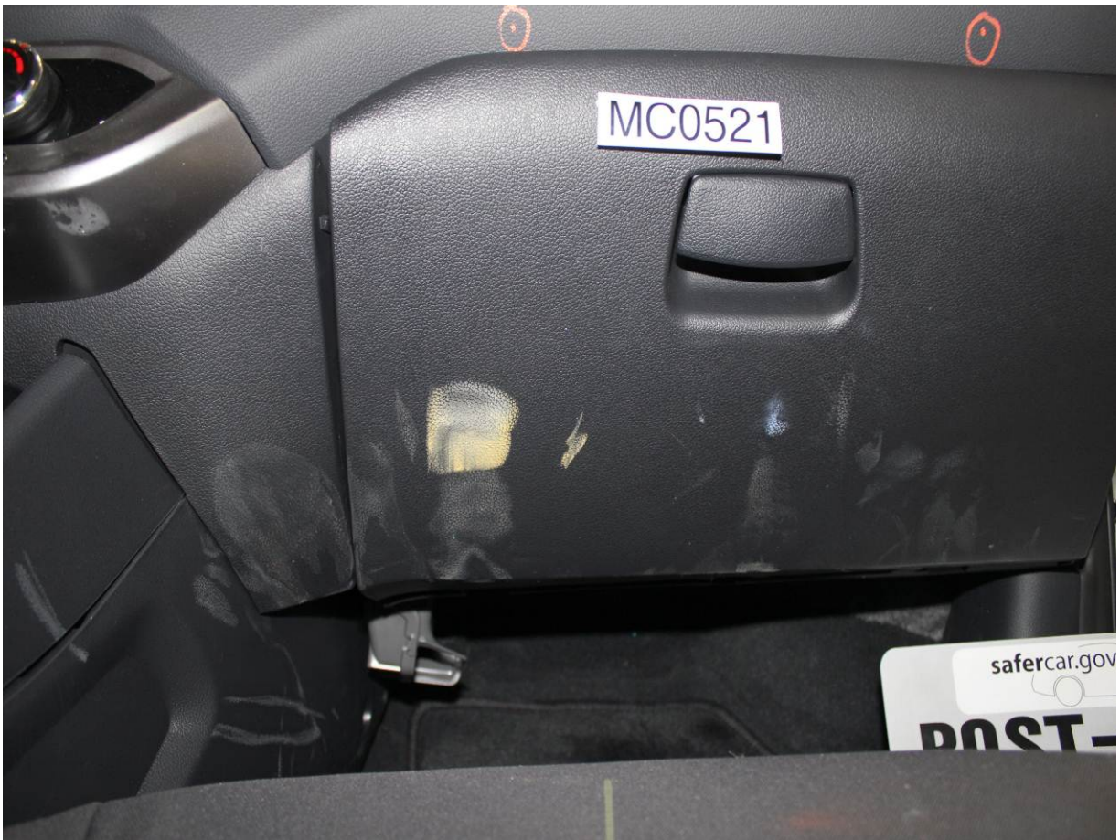
Post-Test Passenger Dummy Contact with Glovebox
