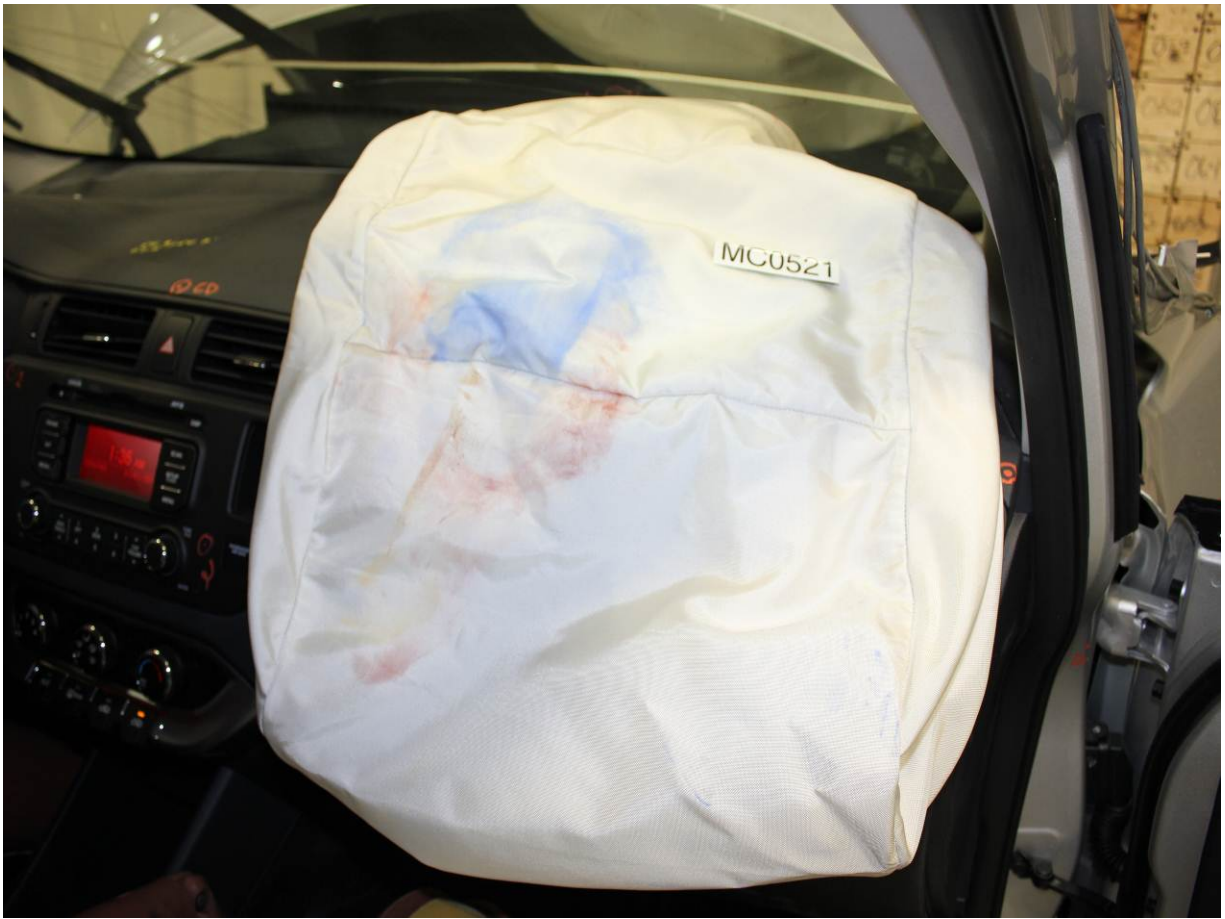
Post-Test Passenger Dummy Contact with Airbag
