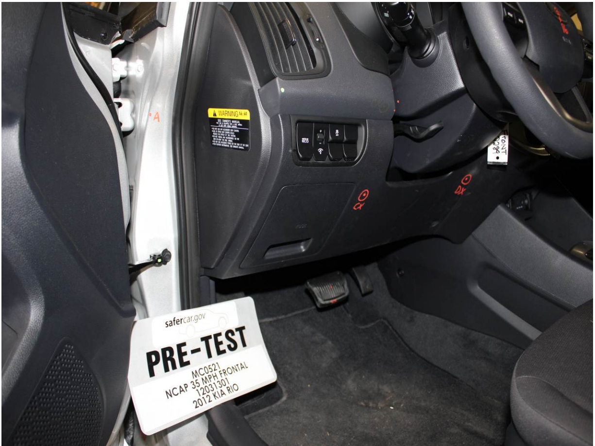
Pre-Test Driver's Side Knee Bolster (without dummy)
