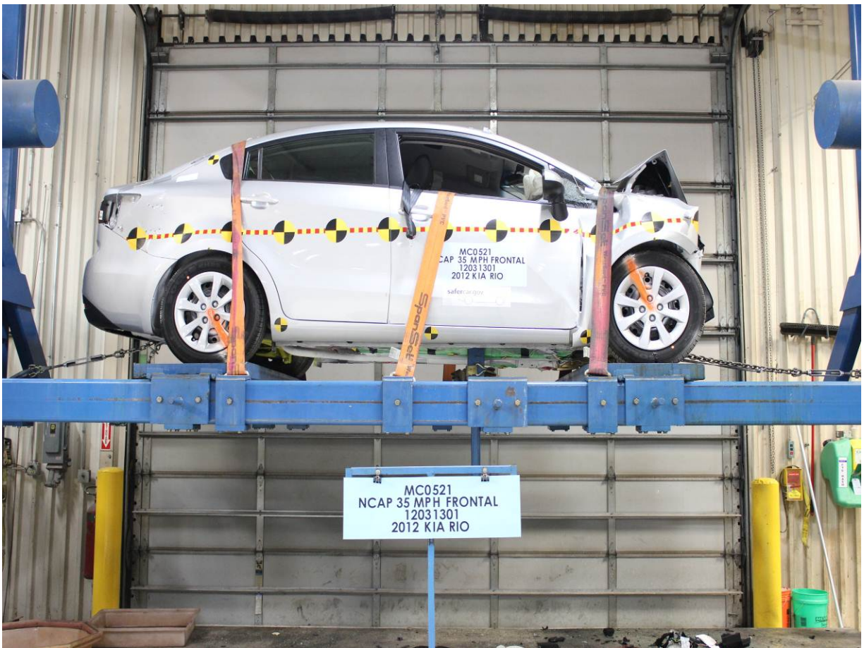
Vehicle at 360 Degrees on Static Rollover Device
