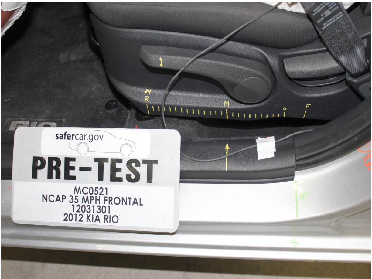
Pre-Test Driver's Seat Fore-Aft Markings
