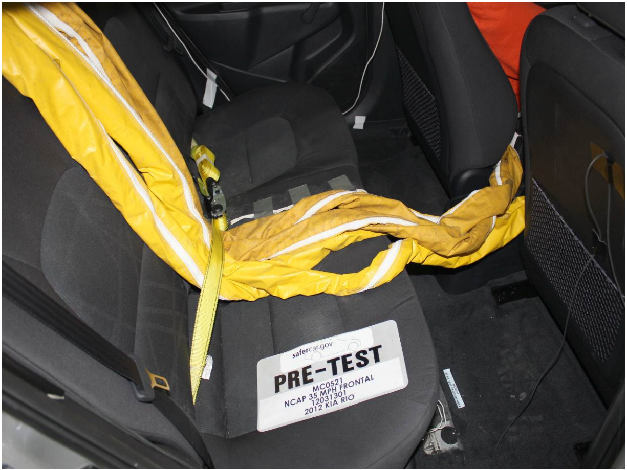
Pre-Test Dummy Cable Routing
