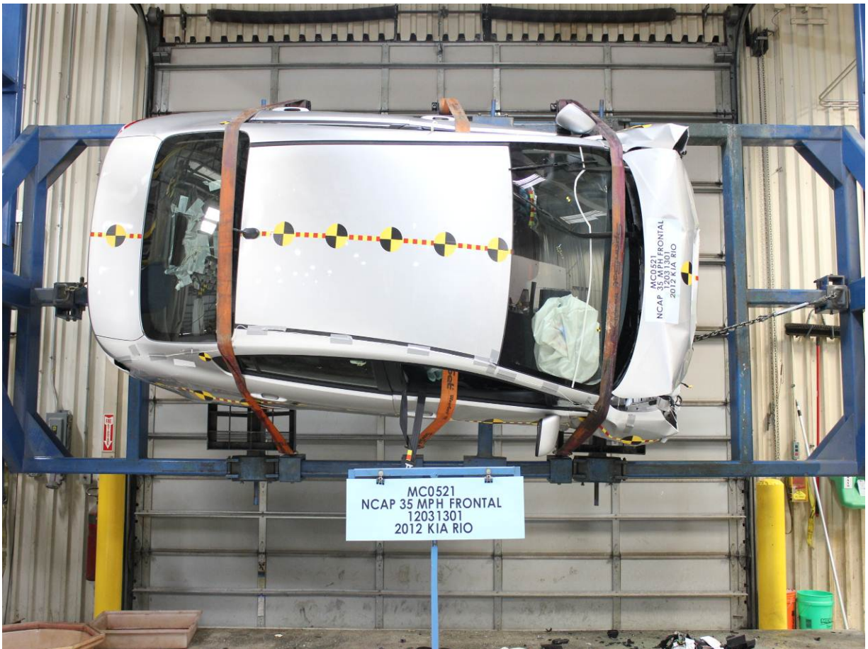
Vehicle at 270 Degrees on Static Rollover Device
