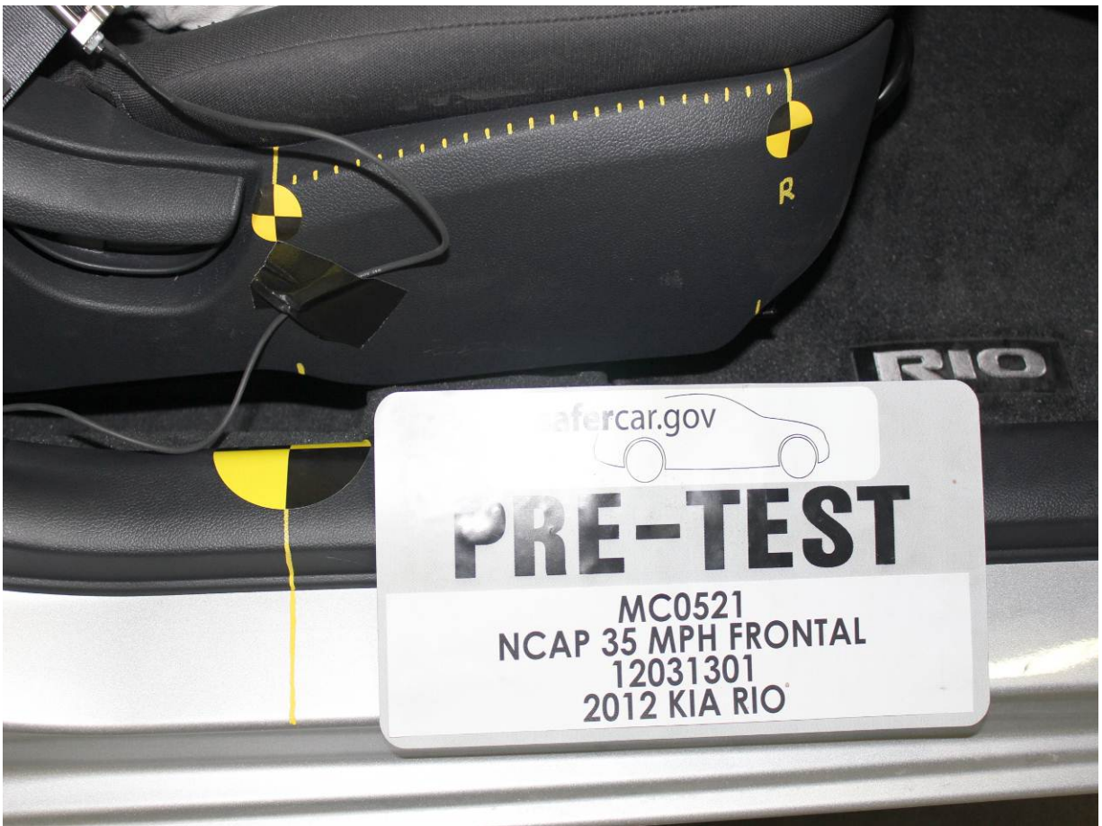
Pre-Test Passenger's Seat Fore-Aft Markings
