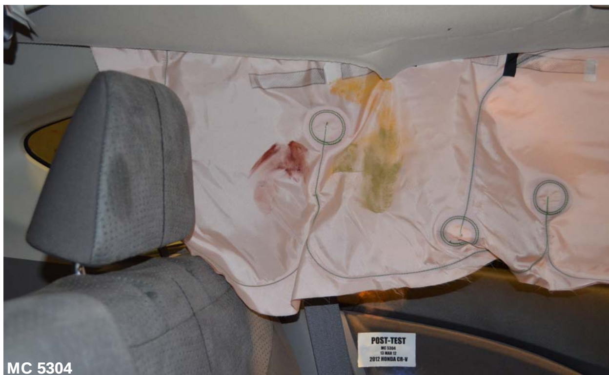
Figure A-74: Post-Test Rear Passenger Dummy Close-Up Head Contact with Vehicle Interior View
