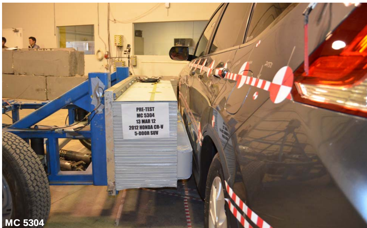
Figure A-18: Pre-Test Right Side View of MDB Positioned Against Side of Test Vehicle
