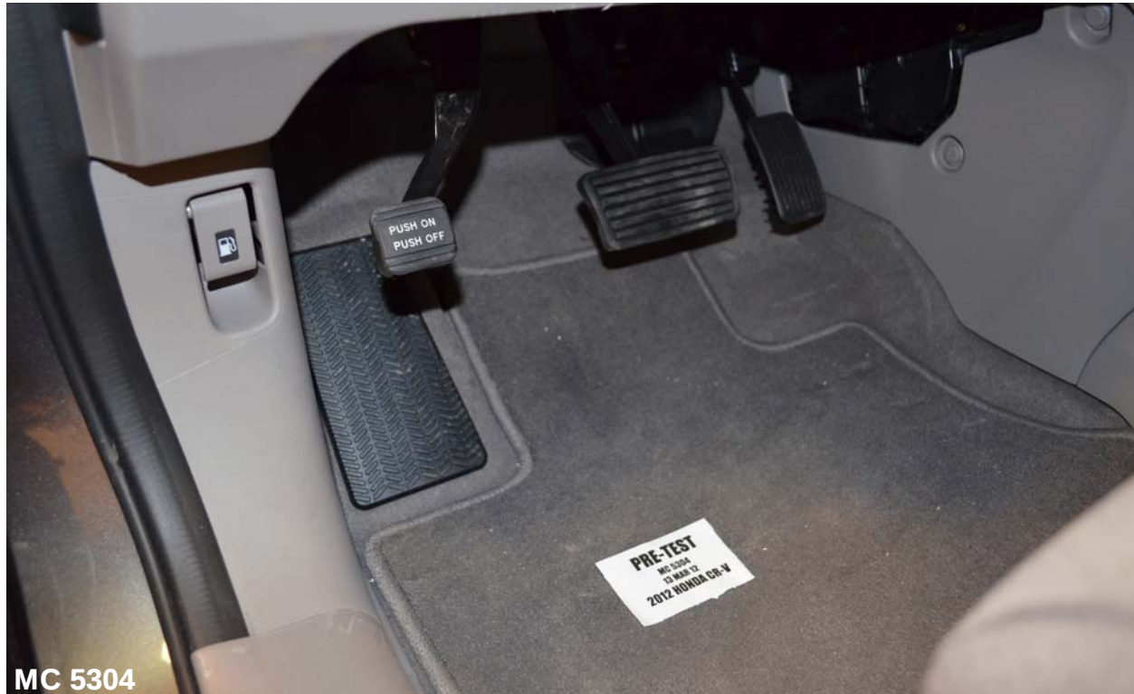
Figure A-37: View of Disengaged Parking Brake
