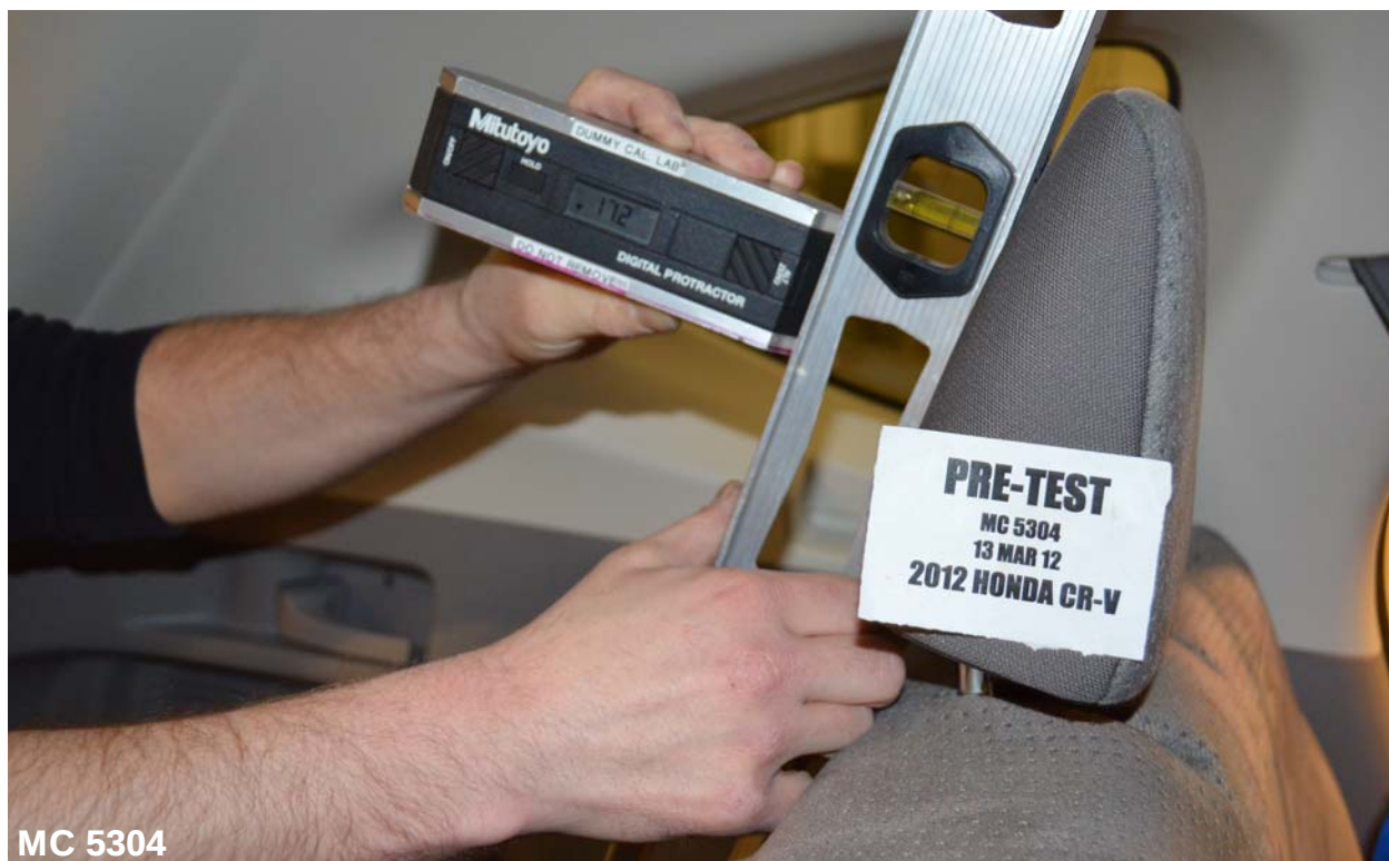
Figure A-67: Pre-Test Close-Up View of Rear Passenger Seat Back or Head Restraint
