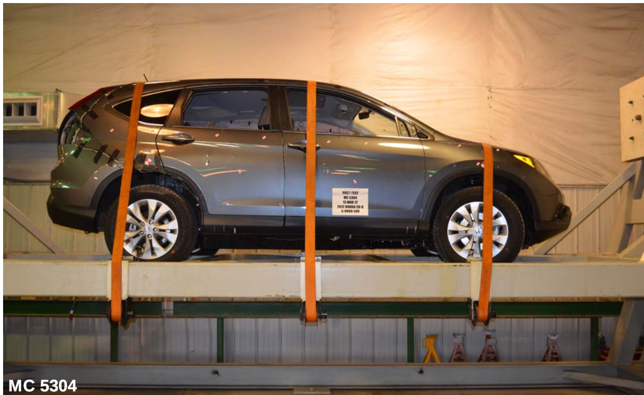
Figure A-94: FMVSS No. 301 Static Rollover 0 Degrees
