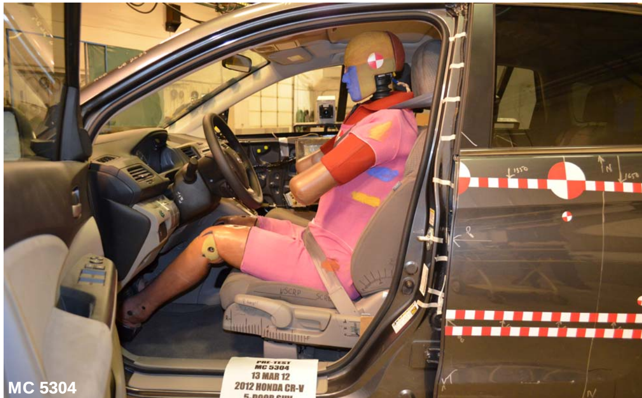
Figure A-27: Pre-Test Left Side View of Driver Dummy Showing Belt and Chalking
