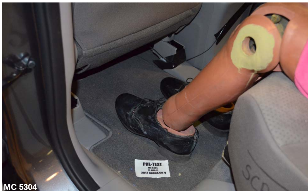
Figure A-63: Pre-Test Placement of Rear Passenger Dummy's Feet
