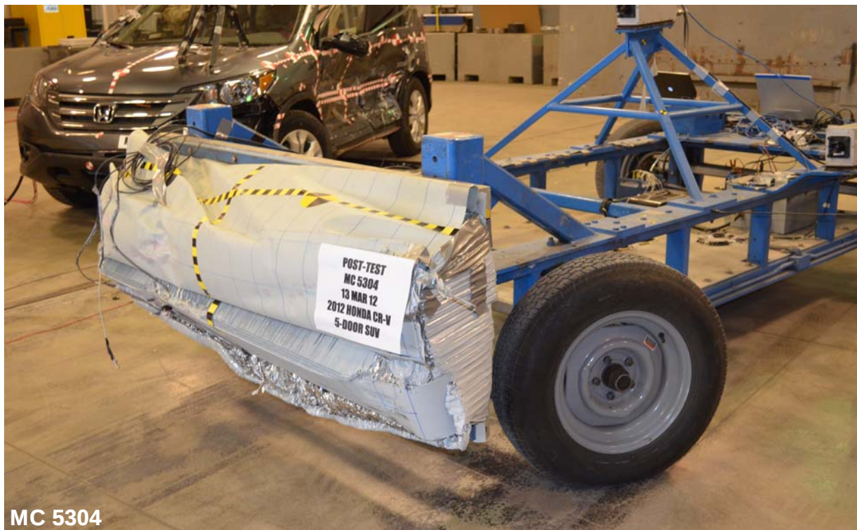
Figure A-87: Post-Test Left Side View of MDB Impactor Face
