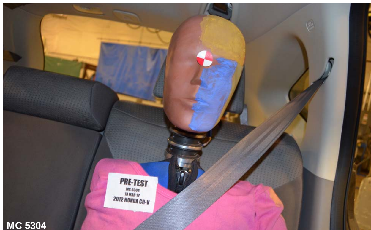
Figure A-58: Pre-Test Frontal View of Rear Passenger Dummy Head and Shoulders in Relation to Head Restraint
