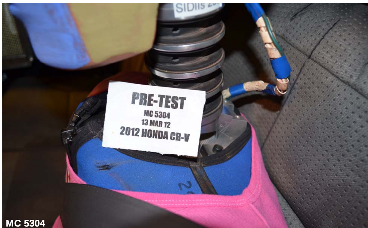
Figure A-61: Pre-Test View of Rear Passenger Dummy's Neck Showing Position of Adjustable Neck Bracket
