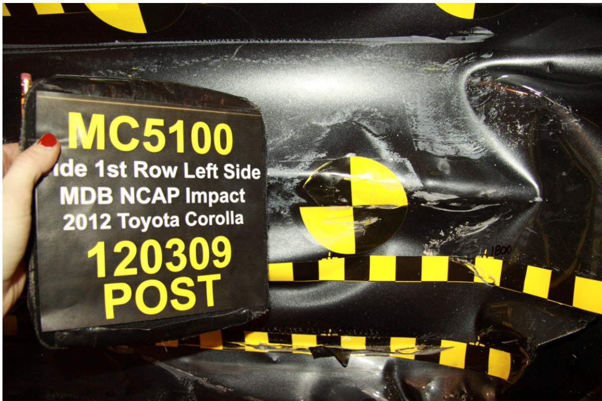
020 Post-Test Close-up View of Impact Point Target
